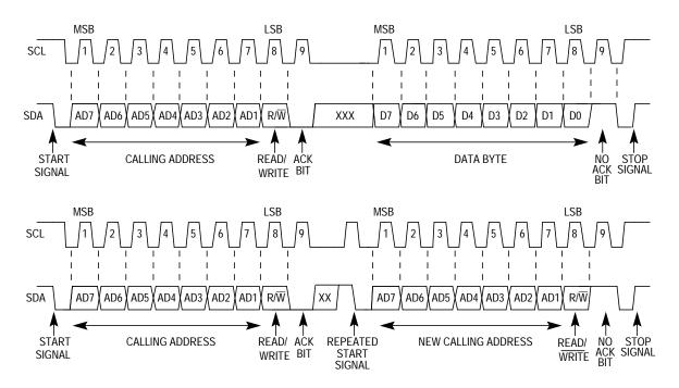
Figure 12-9. IIC Bus Transmission Signals
