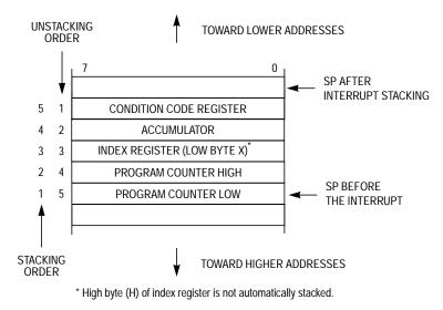
Figure 5-1. Interrupt Stack Frame
