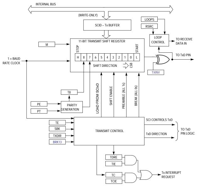
Figure 14-3. SCI Transmitter Block Diagram
