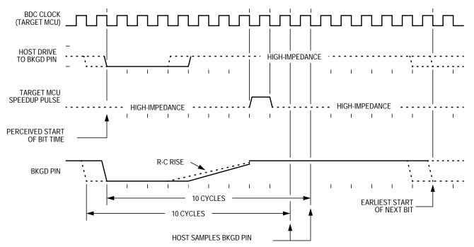
Figure 17-3. BDC Target-to-Host Serial Bit Timing (Logic 1)
