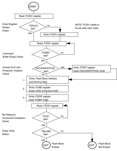
Figure 4-16. Example Erase Verify Command Flow
