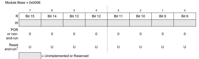
Figure 18-8. Debug FIFO High Register (DBGFH)
