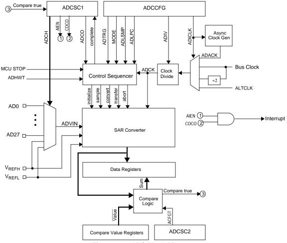
Figure 10-2. ADC Block Diagram
