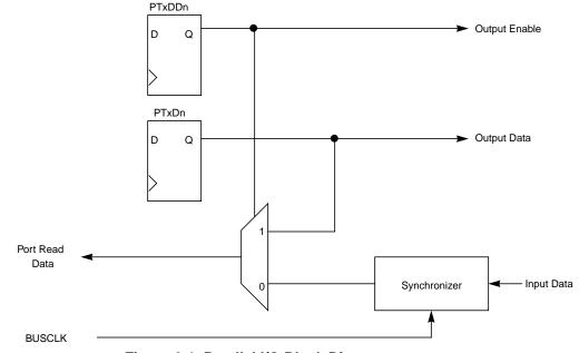
Figure 6-1. Parallel I/O Block Diagram
