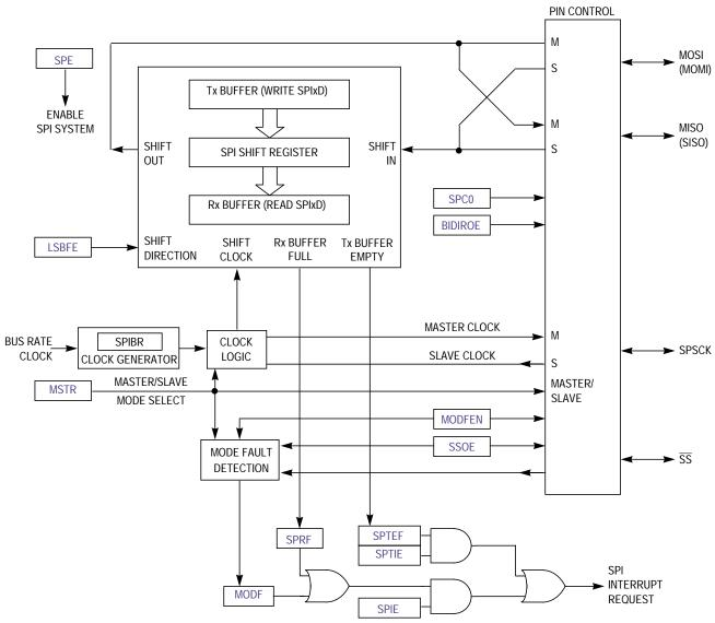
Figure 15-3. SPI Module Block Diagram
