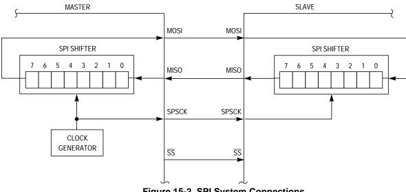
Figure 15-2. SPI System Connections
