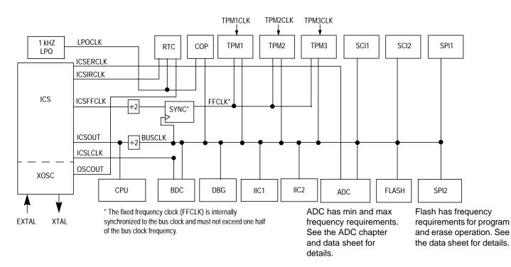
Figure 1-2. System Clock Distribution Diagram
