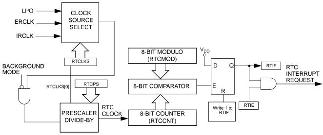
Figure 13-2. Real-Time Counter (RTC) Block Diagram
