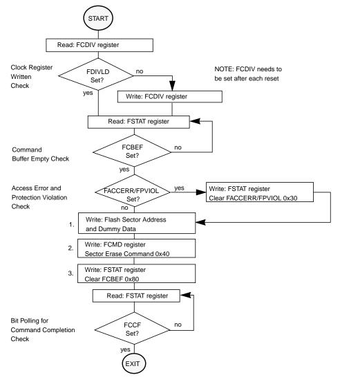
Figure 4-19. Example Sector Erase Command Flow
