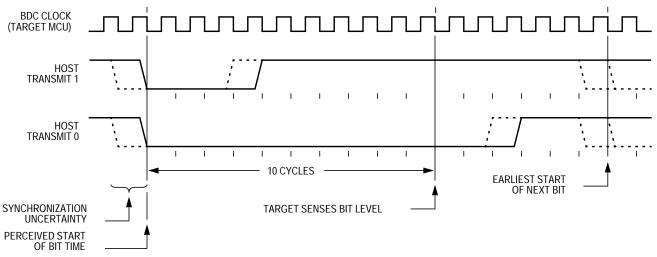
Figure 17-2. BDC Host-to-Target Serial Bit Timing
