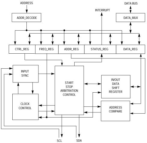
Figure 12-2. IIC Functional Block Diagram
