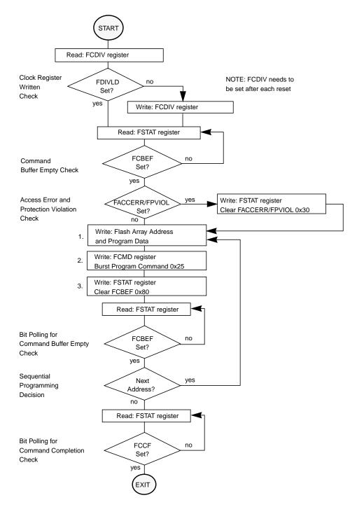
Figure 4-18. Example Burst Program Command Flow
