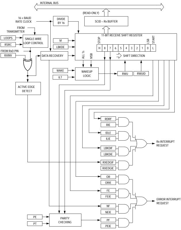
Figure 14-4. SCI Receiver Block Diagram
