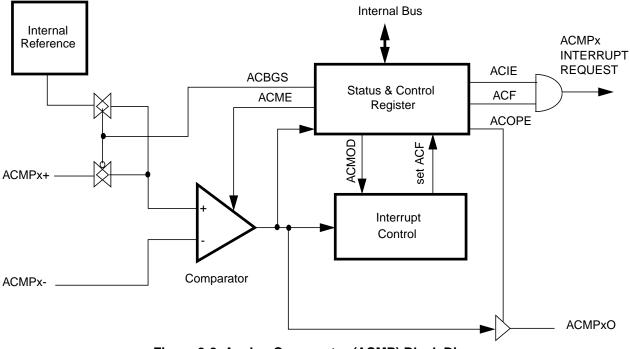
Figure 9-2. Analog Comparator (ACMP) Block Diagram
