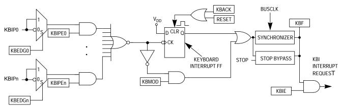
Figure 7-1. KBI Block Diagram
