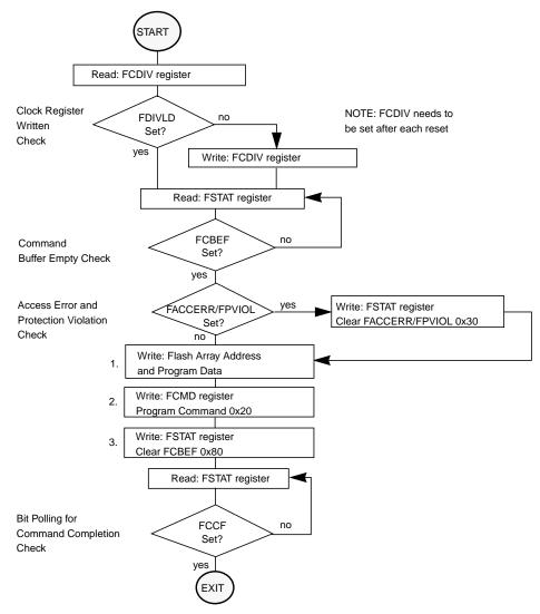
Figure 4-17. Example Program Command Flow
