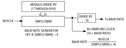
Figure 14-13. SCI Baud Rate Generation
