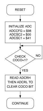
Figure 10-14. Initialization Flowchart for Example
