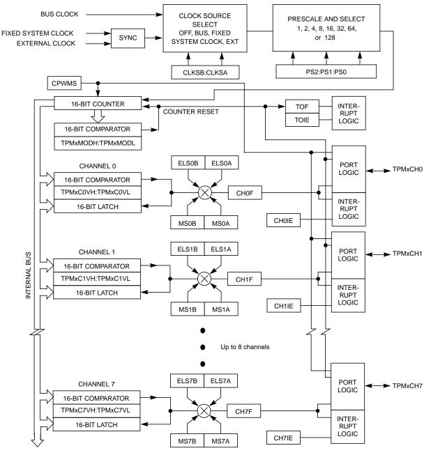
Figure 16-2. TPM Block Diagram
