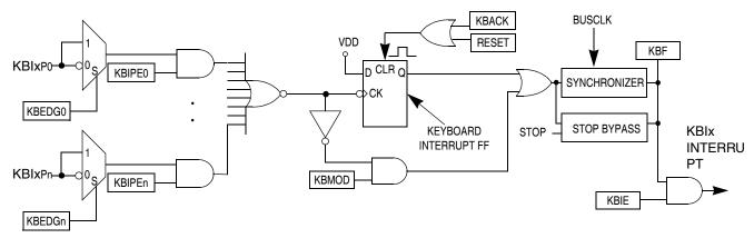
Figure 7-2. Keyboard Interrupt (KBI) Block Diagram
