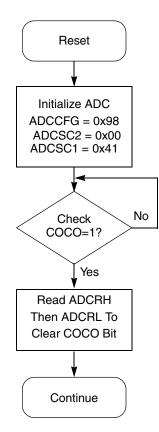
Figure 10-13. Initialization Flowchart for Example
