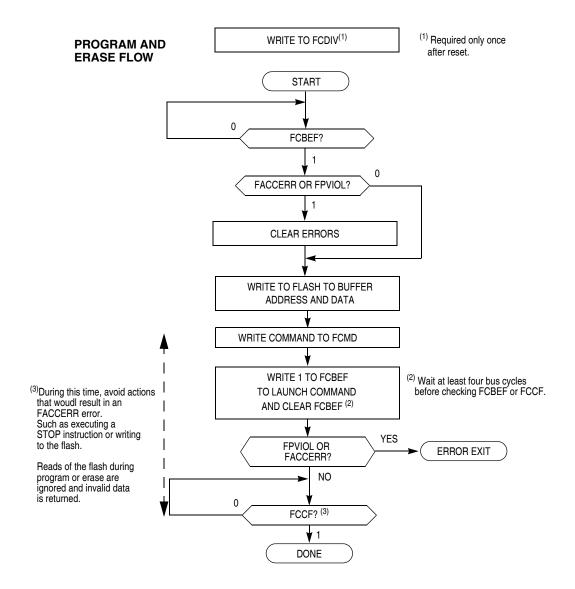
Figure 4-2. Flash Program and Erase Flowchart
