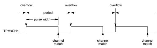
Figure 16-15. EPWM period and pulse width (ELSnA=0)
