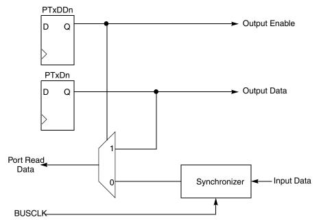
Figure 6-1. Parallel I/O Block Diagram
