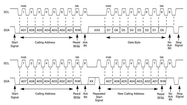
Figure 12-9. IIC Bus Transmission Signals
