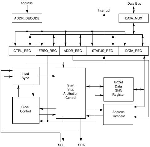
Figure 12-2. IIC Functional Block Diagram
