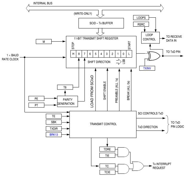
Figure 14-3. SCI Transmitter Block Diagram
