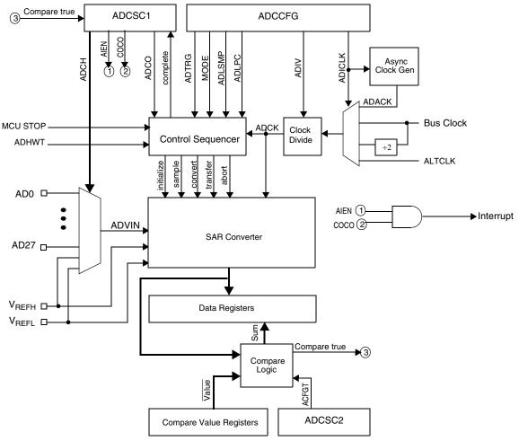
Figure 10-2. ADC Block Diagram
