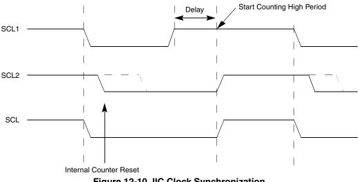
Figure 12-10. IIC Clock Synchronization
