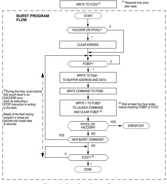
Figure 4-3. Flash Burst Program Flowchart
