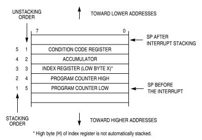
Figure 5-1. Interrupt Stack Frame
