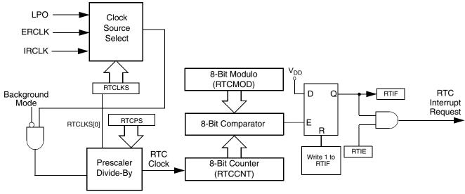
Figure 13-2. Real-Time Counter (RTC) Block Diagram
