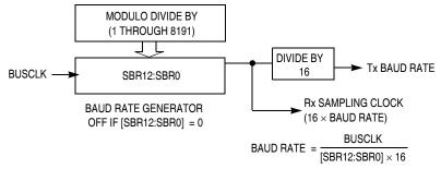
Figure 14-13. SCI Baud Rate Generation
