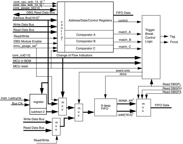
1. In 64K versions of this module there are only 16 address lines [15:0], there are no core\_cpu\_aob\_14\_t2, core\_cpu\_aob\_15\_t2, core\_ppage\_t2[2:0], and ppage\_sel signals.
