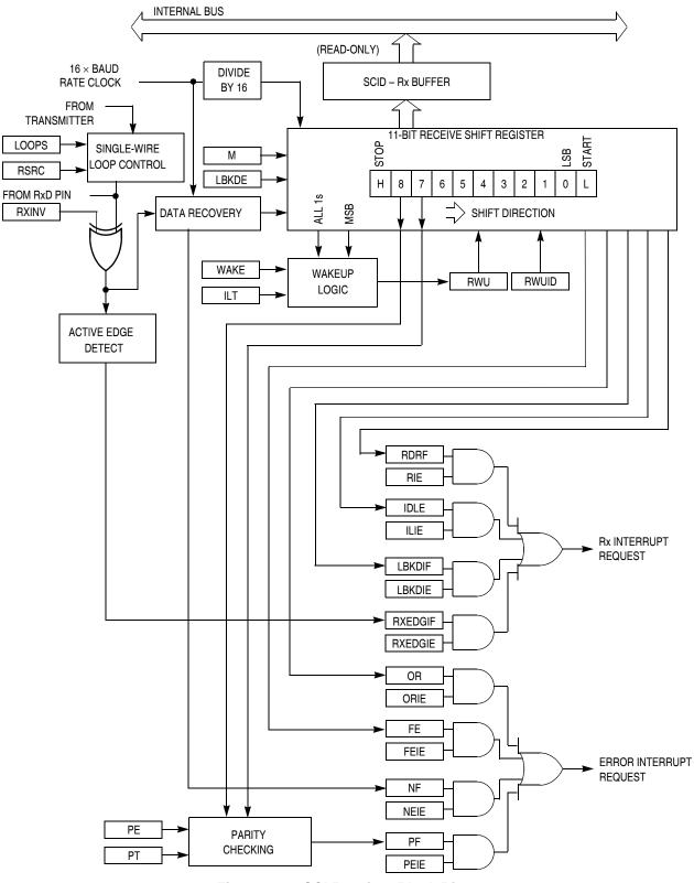
Figure 14-4. SCI Receiver Block Diagram
