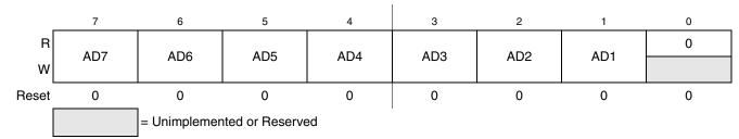
Figure 12-3. IIC Address Register (IICA)
