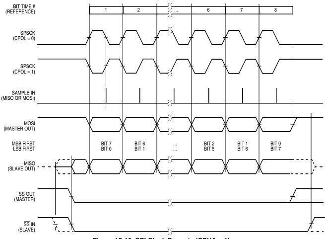
Figure 15-10. SPI Clock Formats (CPHA = 1)
