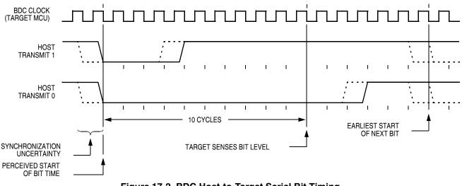
Figure 17-2. BDC Host-to-Target Serial Bit Timing
