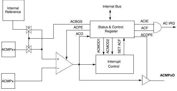
Figure 9-2. Analog Comparator Module Block Diagram
