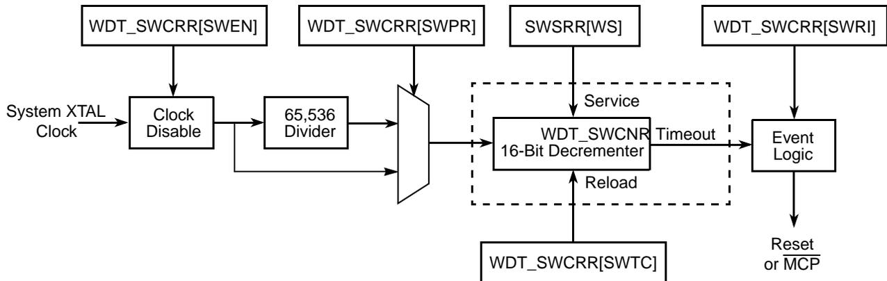
**Figure 35-5. Software Watchdog Timer Functional Block Diagram**
