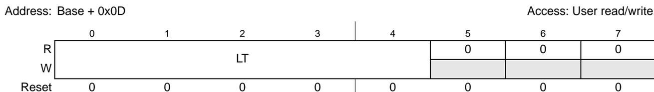
**Figure 28-25. Latency Timer Configuration (PCI\_LATENCYTMFG) Register**
