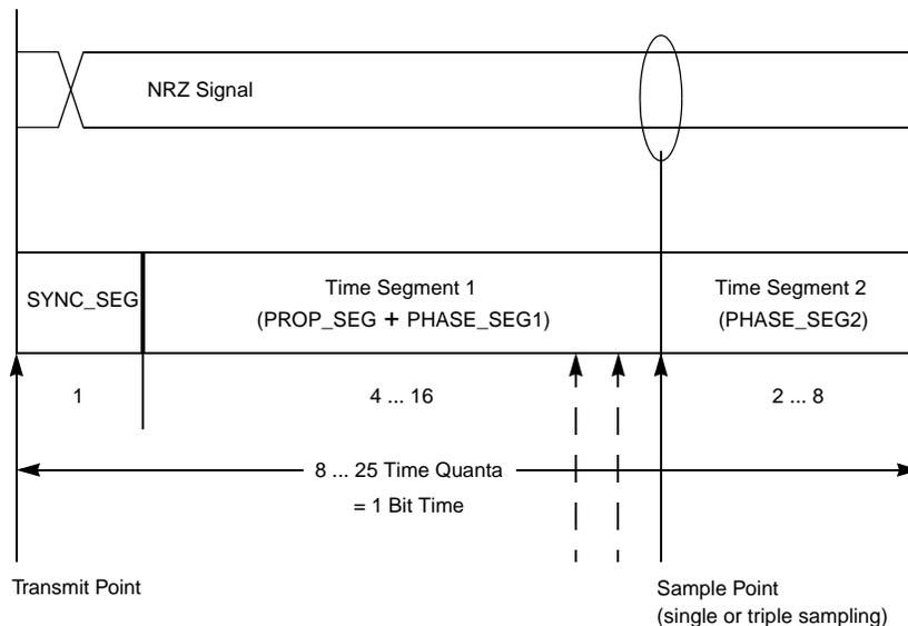
**Figure 25-38. Segments within the Bit Time**
