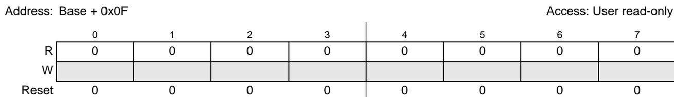
Figure 28-27. BIST Control Configuration (PCI\_BISTCTLCFG) Register
