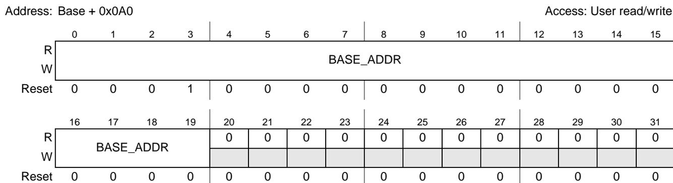
**Figure 2-6. DDR Local Access Window Base Address Register (DDRLAWBAR)**
