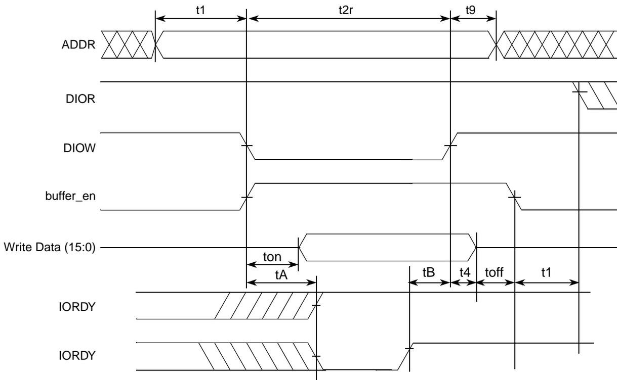
**Figure 27-17. PIO Write Mode Timing**
