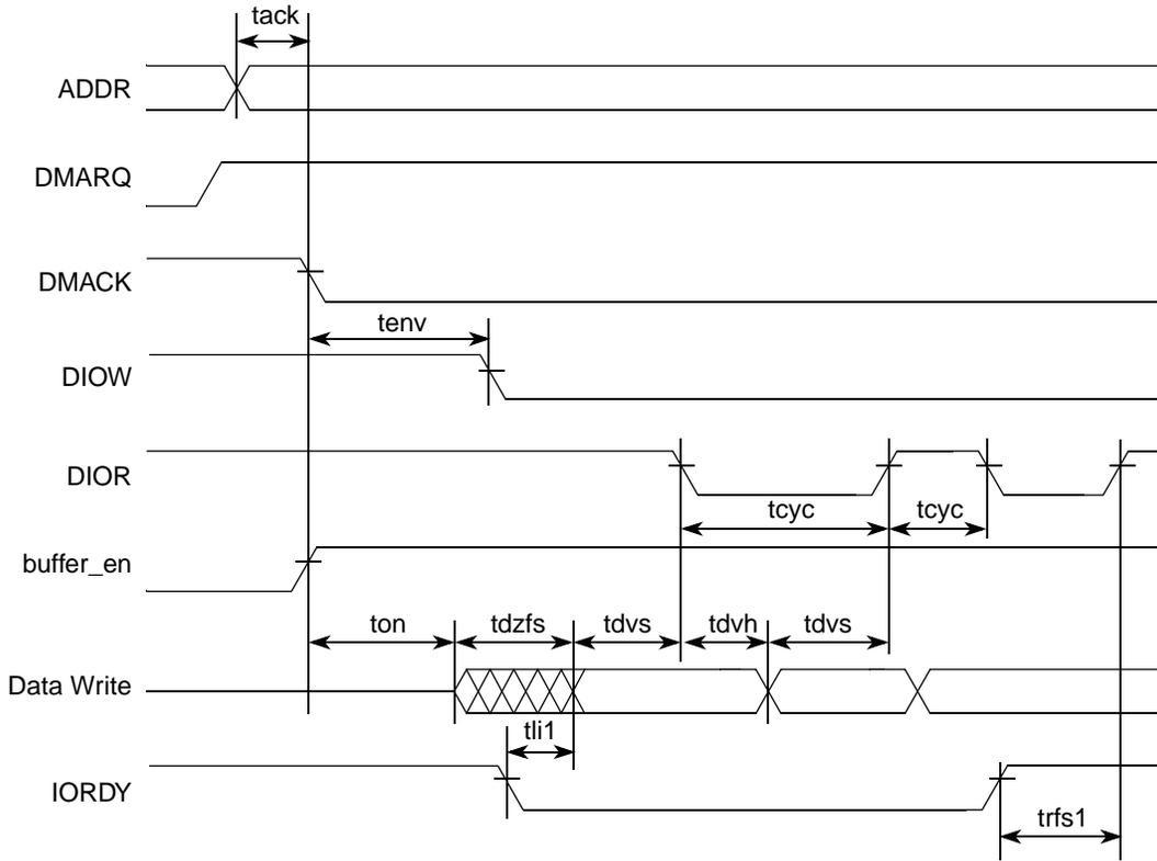
Figure 27-23. UDMA Out Transfer Start Timing Diagram
