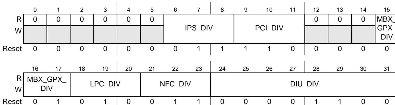
**Figure 5-12. System Clock Frequency Register 1 (SCFR1)**
