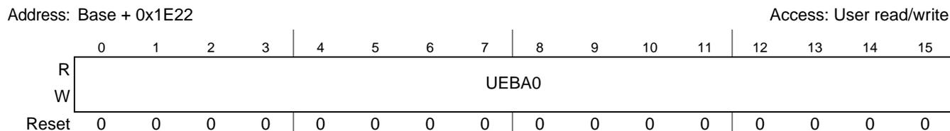
**Figure 26-14. End Block Address to Unlock in Write Protection Mode Register 0 (NFC\_UEBA0)**
