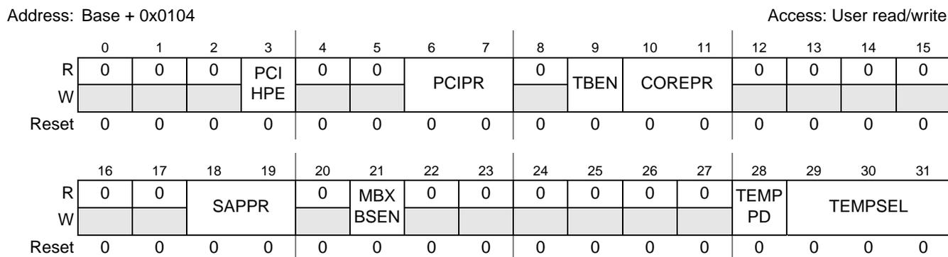
Figure 2-13. System Priority Configuration Register (SPCR)
