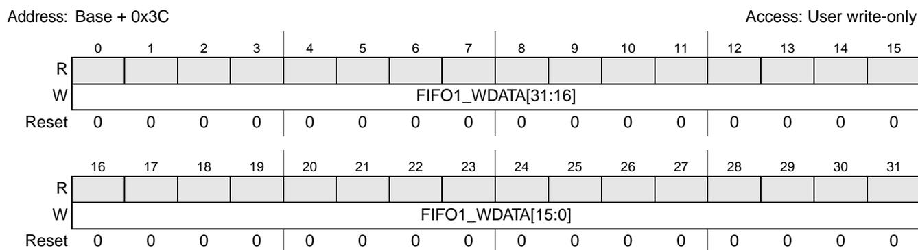
Figure 6-16. FIFO1 Write Data Register
