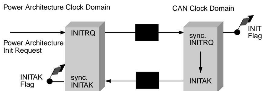
Figure 25-41. Initialization Request/Acknowledge Cycle
