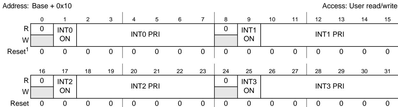
**Figure 6-6. Interrupt Priority Register 0 (INTPRI0)**
