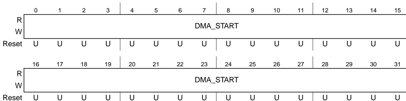
Figure 33-27. DMA Start Address Register (DMA\_START)
