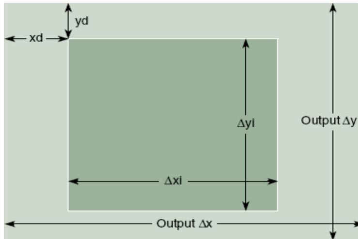
**Figure 12-32. Display Parameters**
