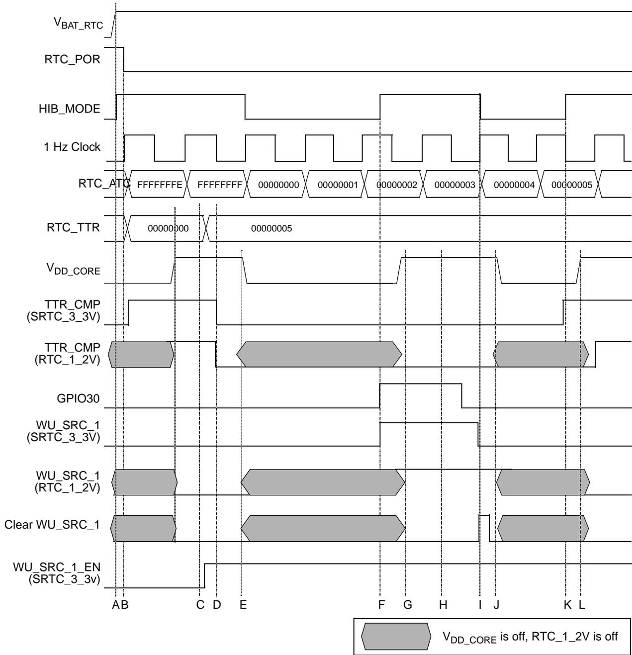
**Figure 32-14. Timing Diagram of the RTC\_TTR and the Positive Edge of GPIO30**
