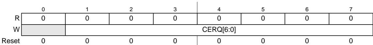
**Figure 11-8. DMA Clear Enable Request Register (DMACERQ)**
