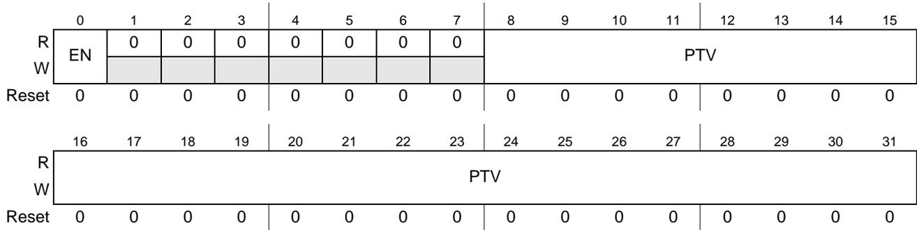
Figure 28-57. PCI Discard Timer Control Register (PCI\_DISCARD\_TIMER\_CNTRL)
