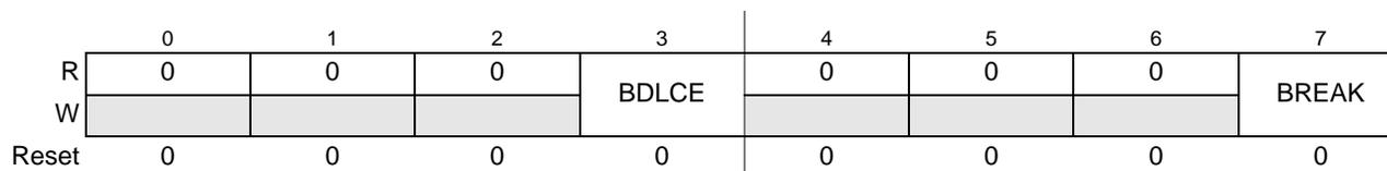
**Figure 7-9. BDLC Control Register (BDLC\_DLCSCR)**
