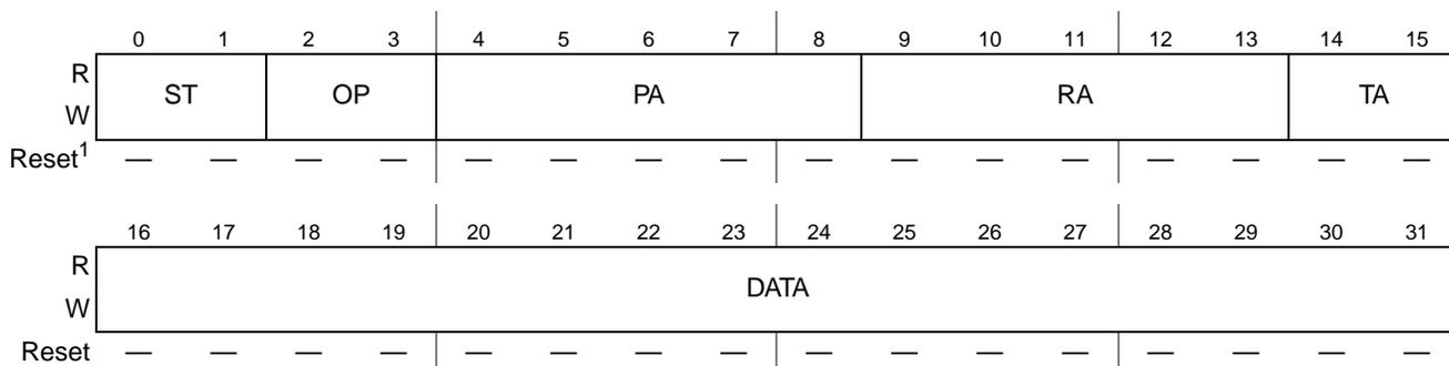
**Figure 16-9. MII Management Frame (ETH\_MII\_DATA) Register**
