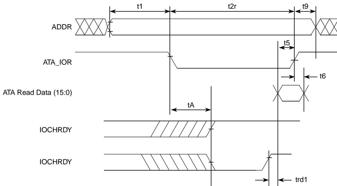
**Figure 27-16. PIO Read Mode Timing**
