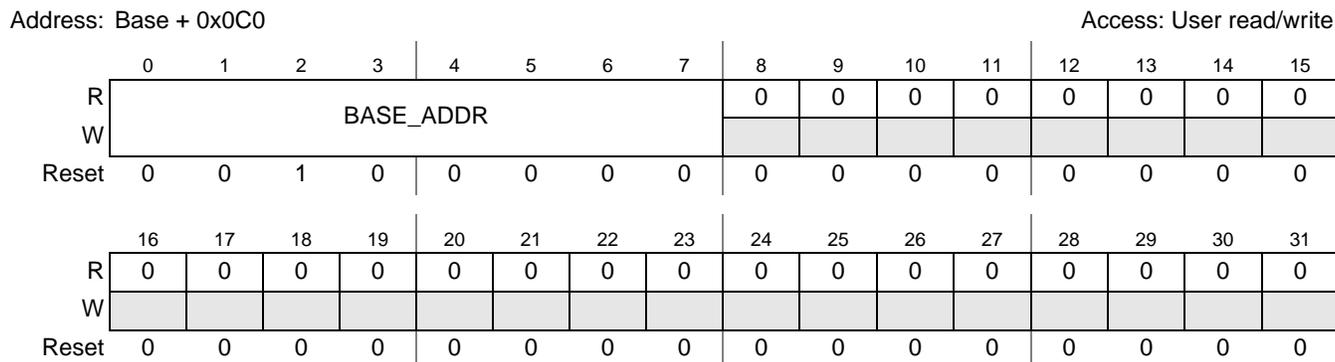
Figure 2-8. MBX Base Address Register (MBXBAR)
