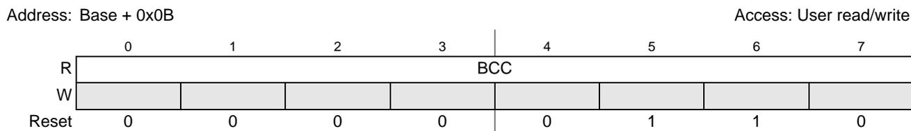
Figure 28-23. Base Class Code Configuration (PCI\_BASECLSCODCFG) Register
