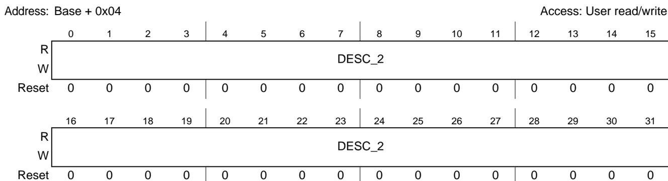
**Figure 12-2. Plane 2 Area Descriptor Pointer Register (DESC\_2)**
