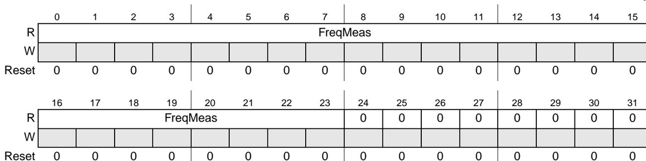
Figure 36-15. SPDIF Frequency Measurement Register (SRFM)
