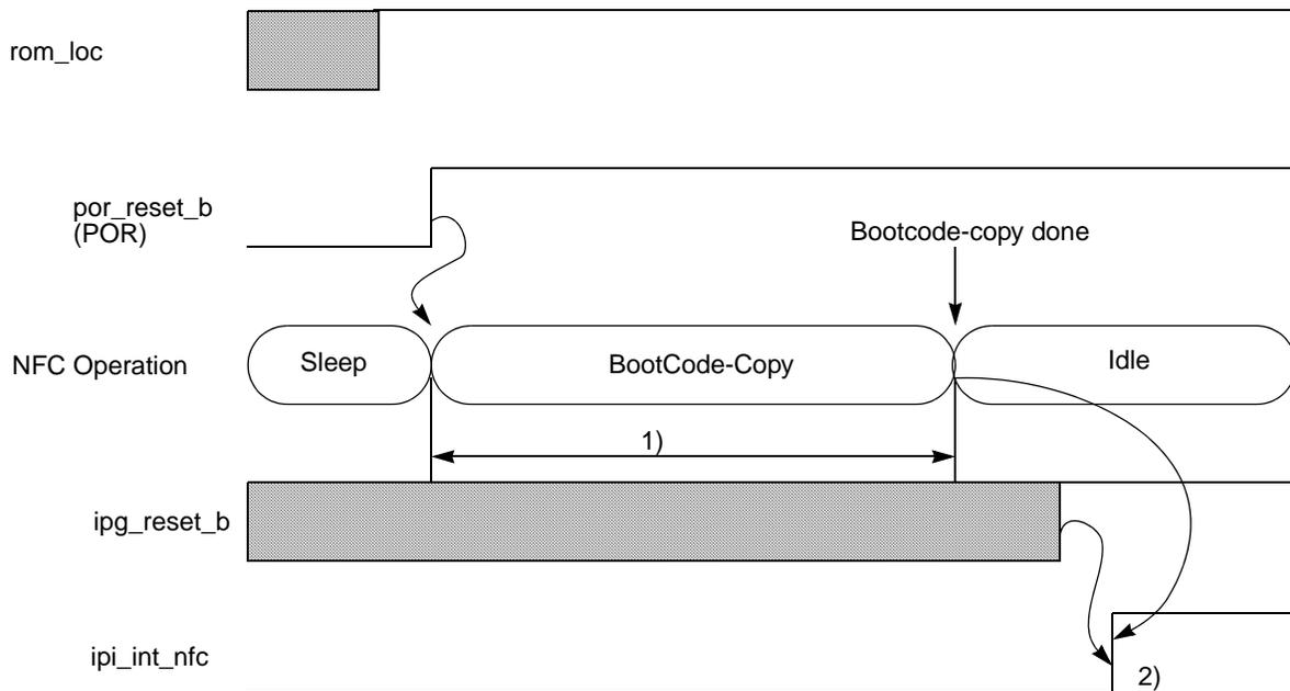
Figure 26-21. Boot Mode Operation
