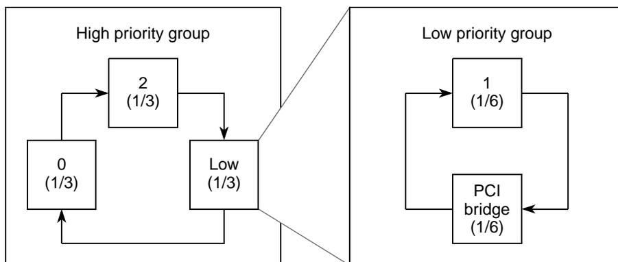
Figure 28-44. PCI Arbitration Example
