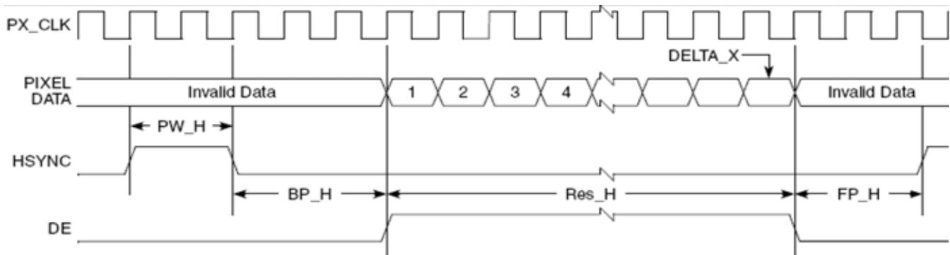
Figure 12-48. Horizontal Sync Signals
