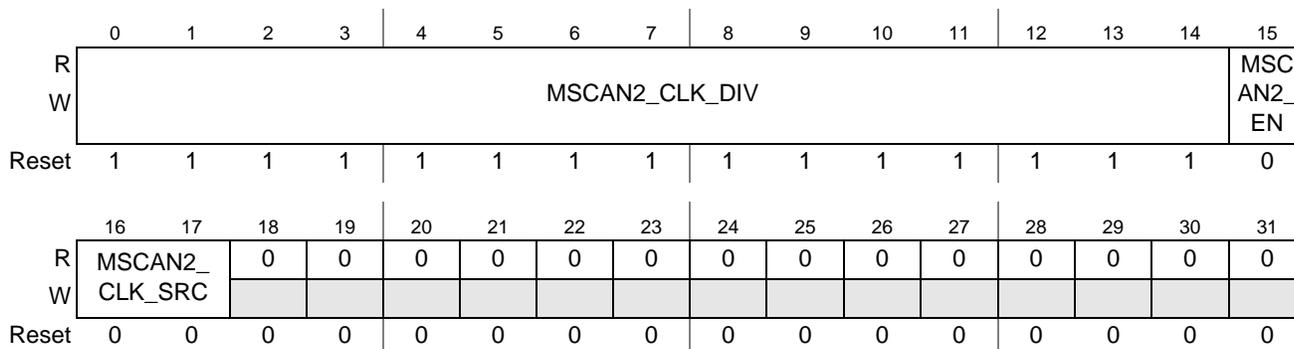
Figure 5-32. MSCAN2 Clock Control Register (M2CCR)
