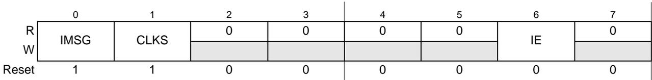
**Figure 7-2. BDLC Control Register 1 (BDLC\_DLCBCR1)**
