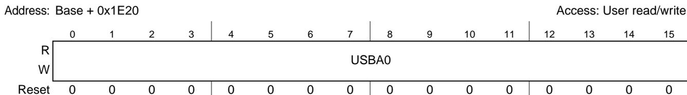
**Figure 26-13. Start Block Address to Unlock in Write Protection Mode Register 0 (NFC\_USBA0)**
