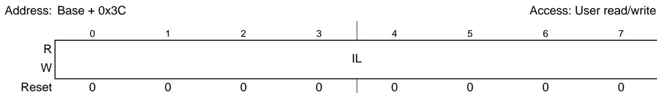
**Figure 28-34. Interrupt Line Configuration (PCI\_INTERRLINECFG) Register**
