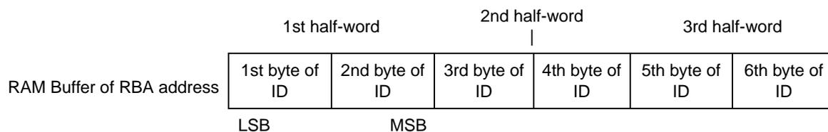
**Figure 26-38. x8 Assignment of NAND Flash ID Data**
