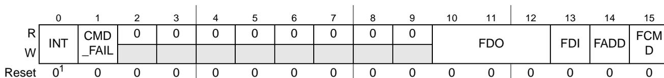
**Figure 26-12. NAND Flash Operation Configuration Register 2 (NF\_CFG2)**
