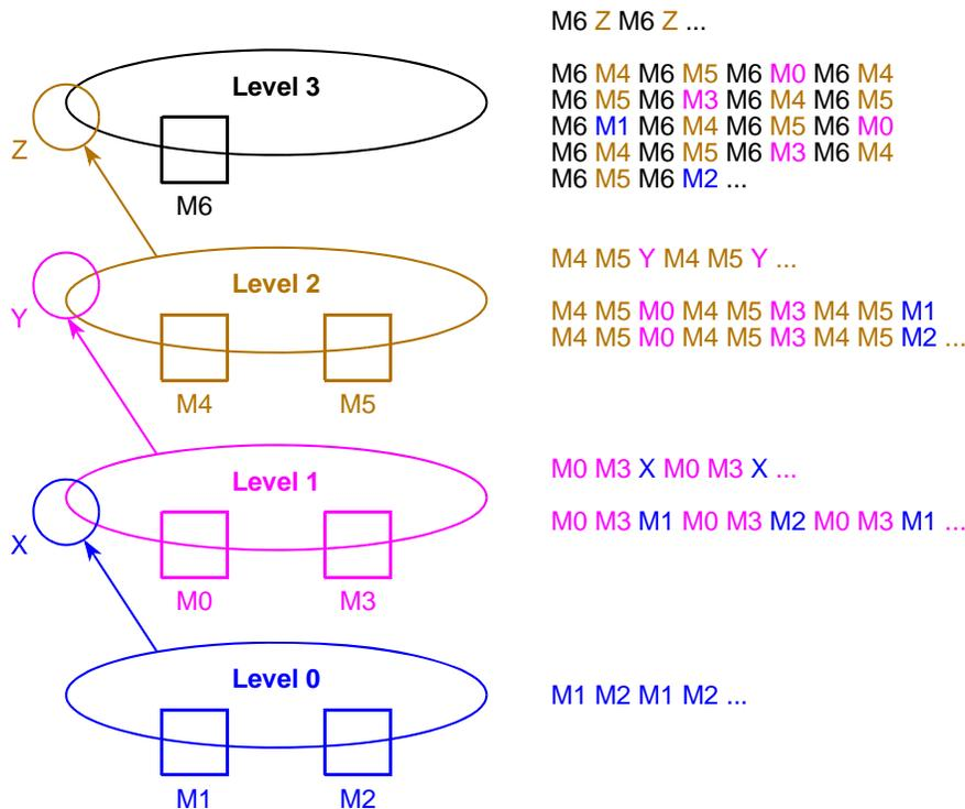
Figure 10-11. Example of Priority Based Arbitration Algorithm
