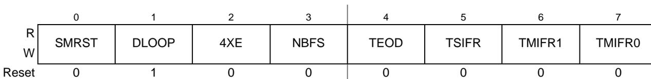
**Figure 7-4. BDLC Control Register 2 (BDLC\_DLCBCR2)**
