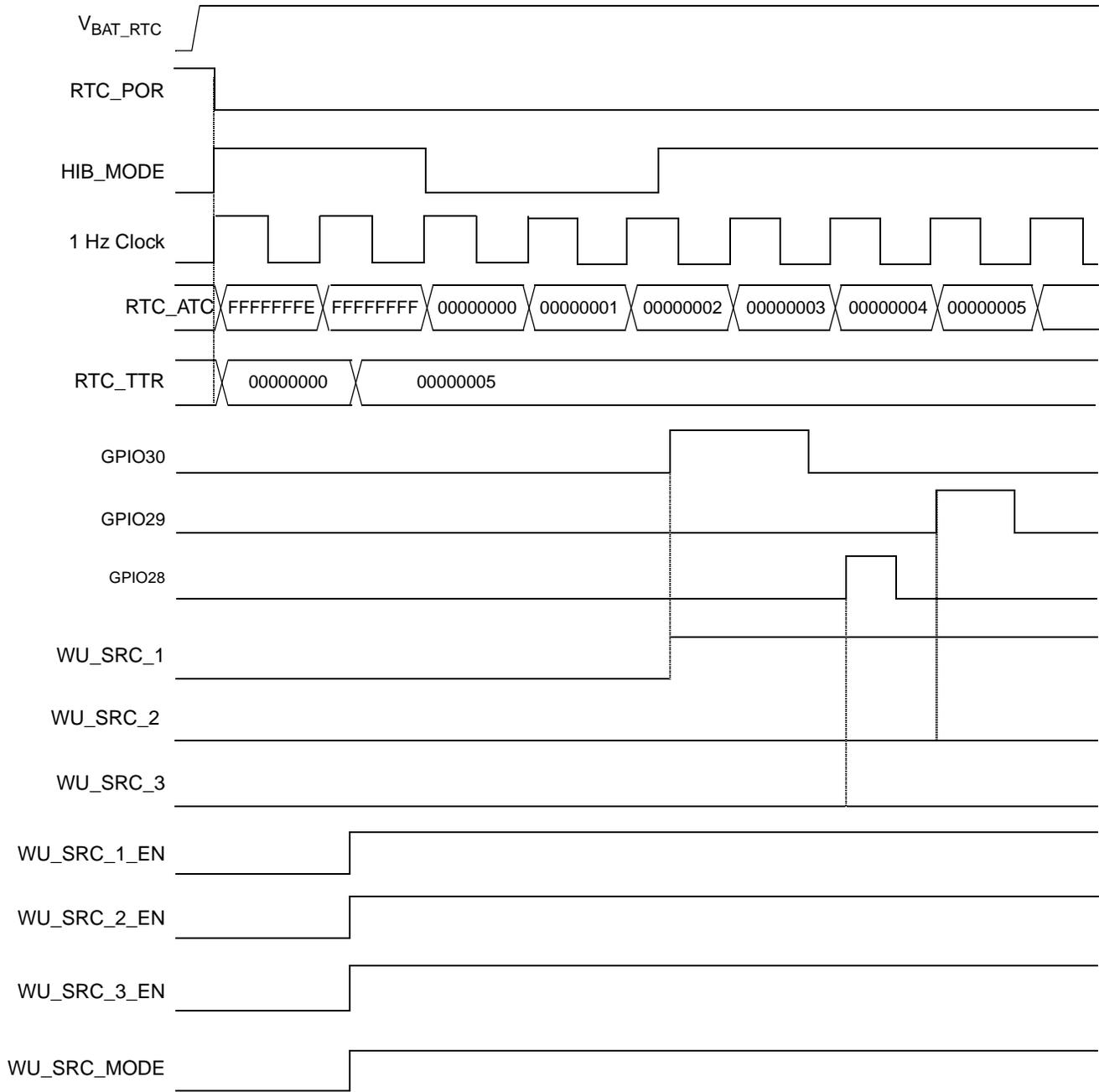
**Figure 32-16. Timing Diagram Illustrating the Functionality of Detecting GPIO[30:28] with WU\_SRC\_MODE Enabled**
