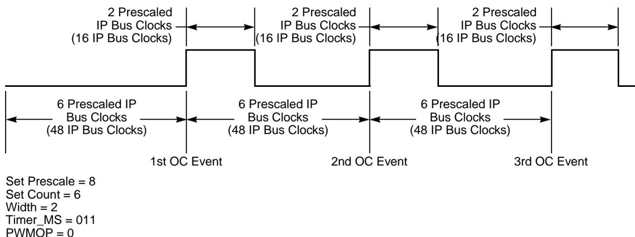
**Figure 17-8. PWM Example with OFF TIME = LOW**
