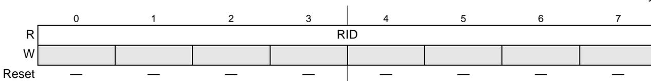
**Figure 28-20. Revision ID Configuration (PCI\_REVIDCFG) Register**
