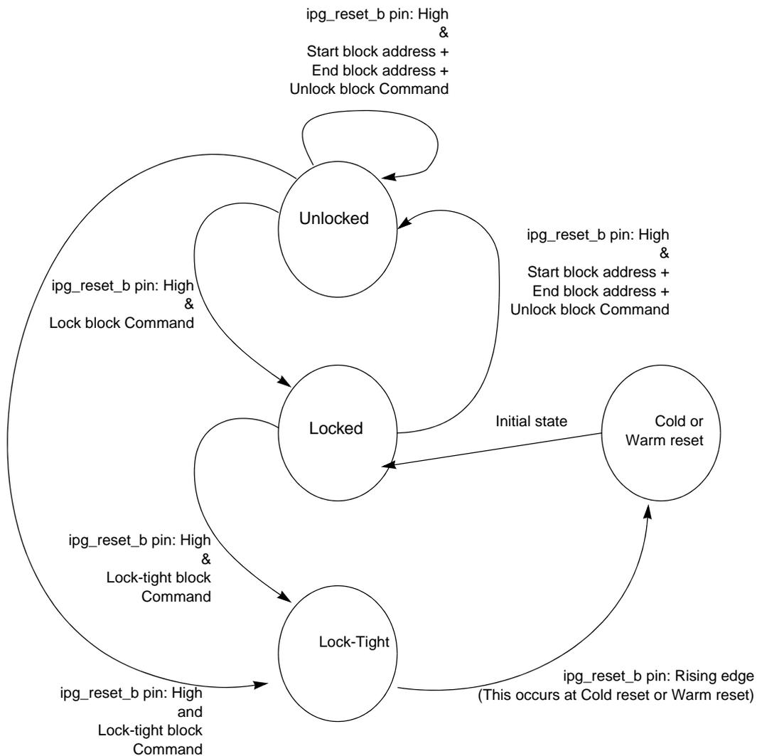
Figure 26-50. State Diagram of NAND Flash Write Protection
