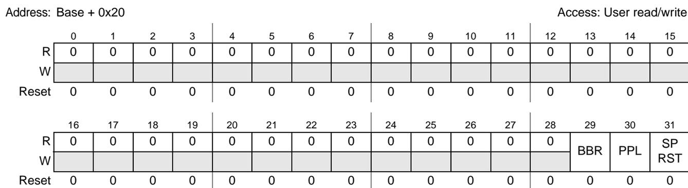
**Figure 28-9. PCI General Control Register (PCI\_PCIGCR)**
