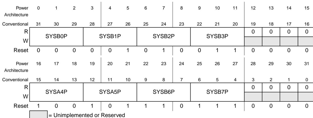
Figure 20-7. System Internal Interrupt Group B Priority Register (SIPRR\_B)
