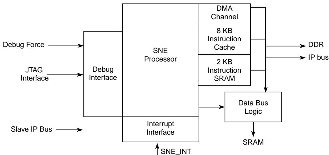
**Figure 6-1. Block Diagram of the Auxiliary Execution Engine**
