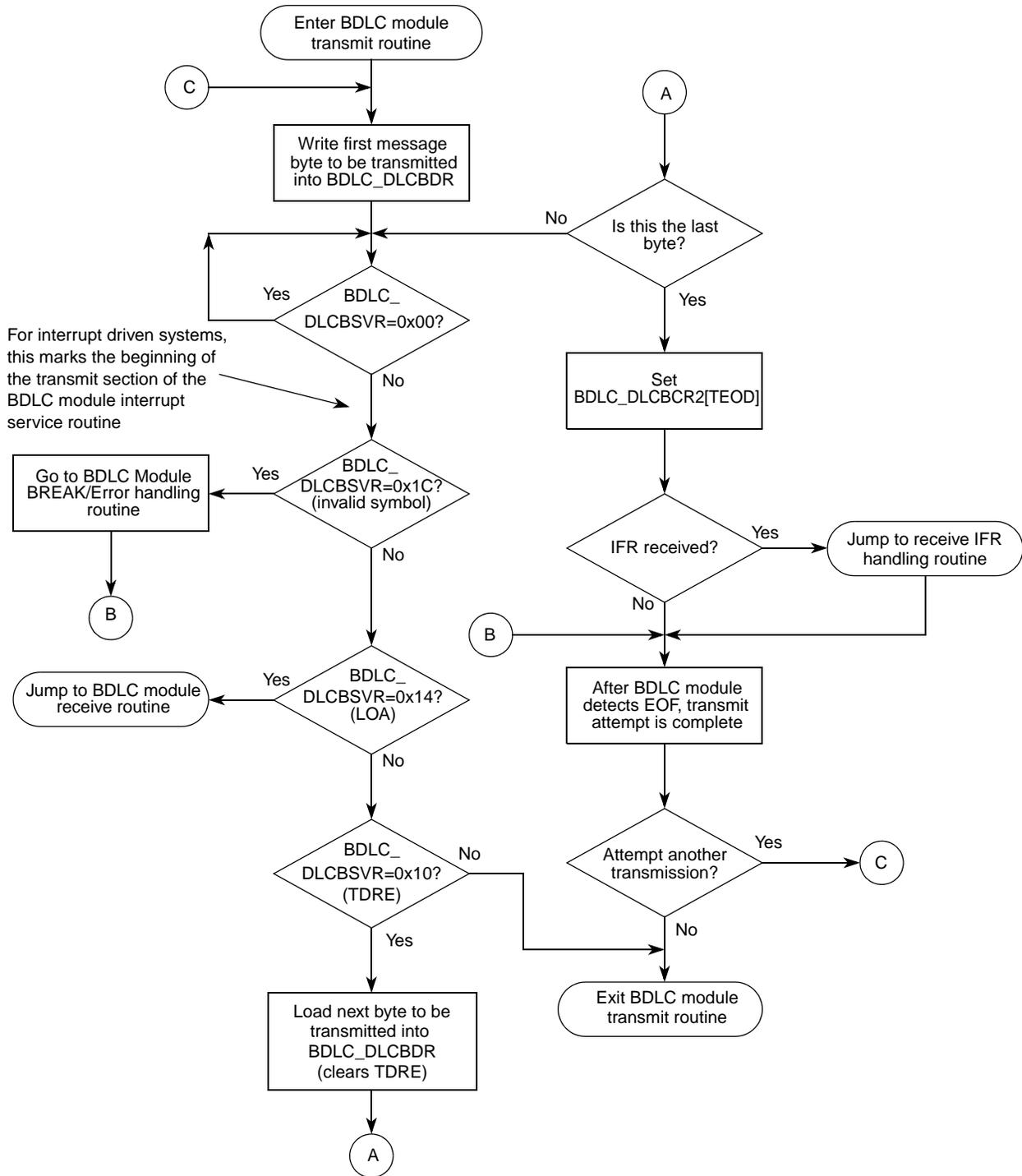
NOTE: The EOF and CRC Error Interrupts are handled in the BDLC Module Receive Routine
