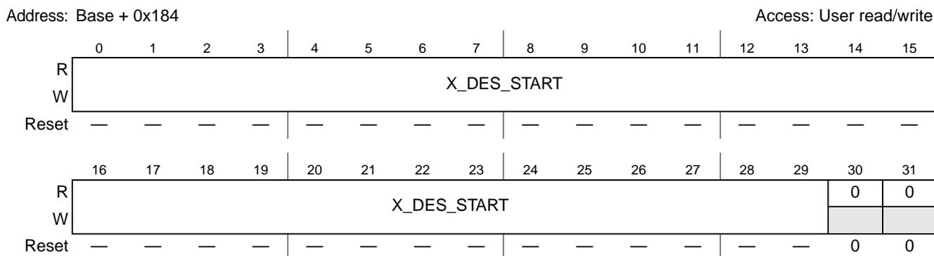
**Figure 16-26. Beginning of Transmit Descriptor Ring (ETH\_X\_DES\_START) Register**
