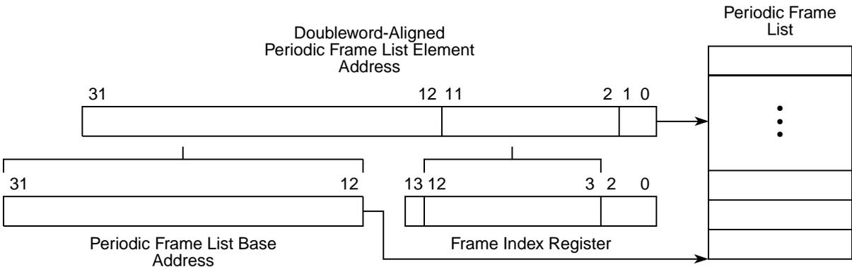
**Figure 39-53. Derivation of Pointer into Frame List Array**
