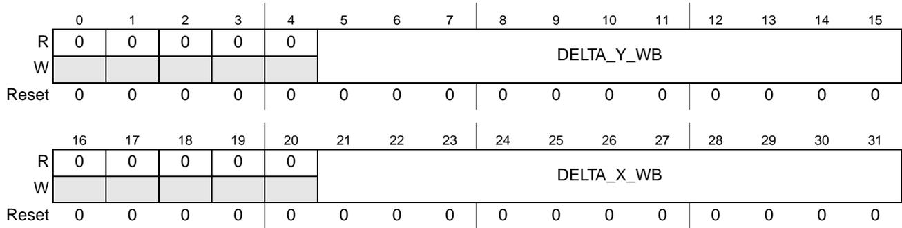
Figure 12-12. Writeback Plane Size Register (WB\_SIZE)
