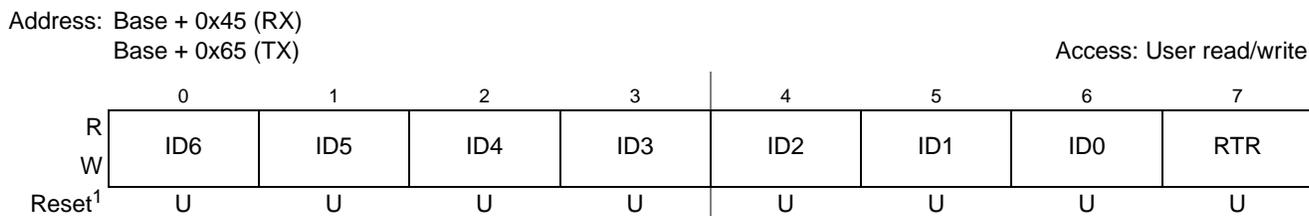
**Figure 25-25. Identifier Register 3 (IDR3)—Extended Identifier Mapping**
