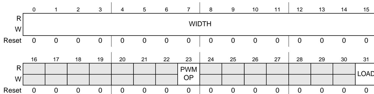
Figure 17-3. GPT0–GPT7 PWM (GPT<sub>n</sub>\_PWM) Configuration Registers
