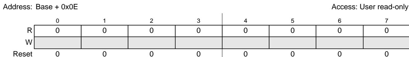
**Figure 28-26. Header Type Configuration (PCI\_HDRTYPECFG) Register**
