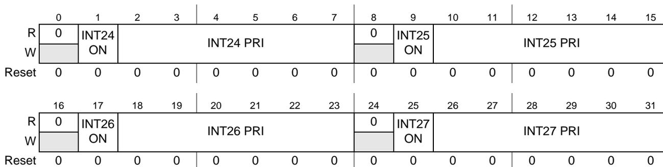
**Figure 6-12. Interrupt Priority Register 6 (INTPRI6)**
