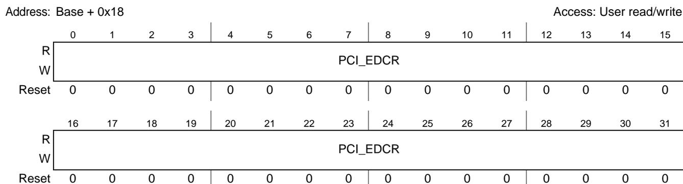
**Figure 28-8. PCI Error Data Capture Register (PCI\_PCIEDCR)**
