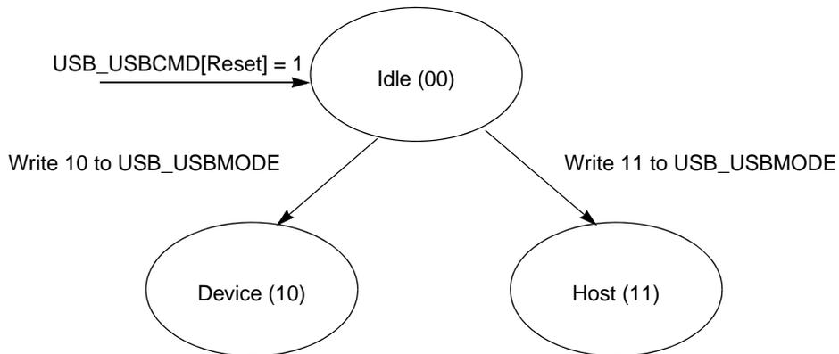
**Figure 39-44. Controller Mode**
