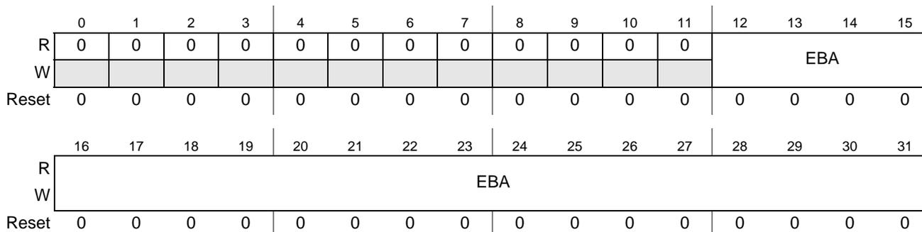
Figure 28-14. PCI Inbound Extended Base Address Registers (PCI\_PCIPIEBAR $n$ )
