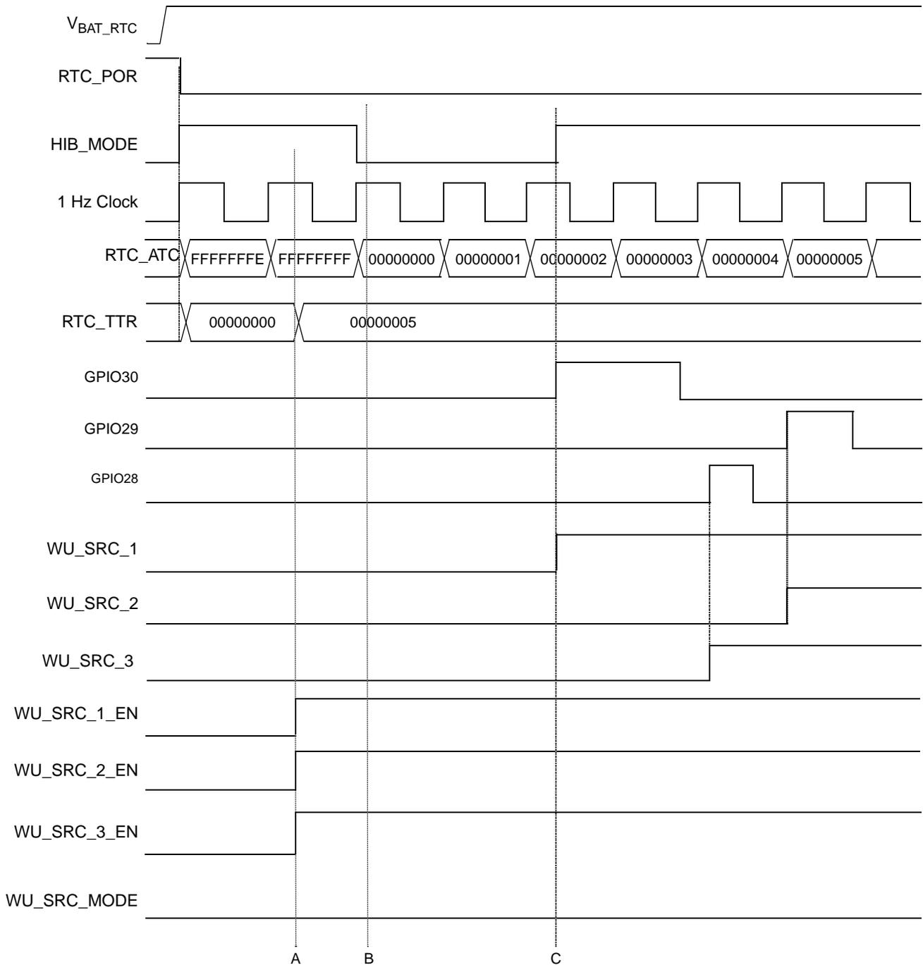
**Figure 32-15. Timing Diagram Showing the Functionality of Detecting GPIO[30:28] with WU\_SRC\_MODE Disabled**
