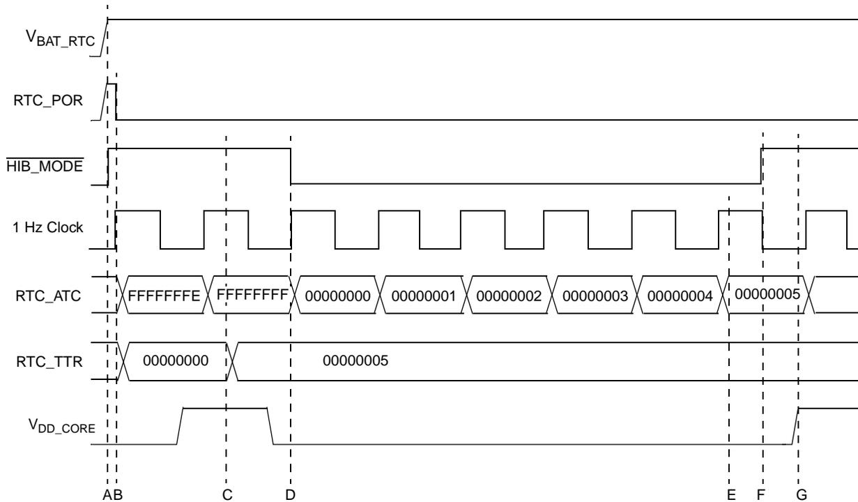
**Figure 32-13. Timing Diagram of the RTC in Deep Sleep Mode**
