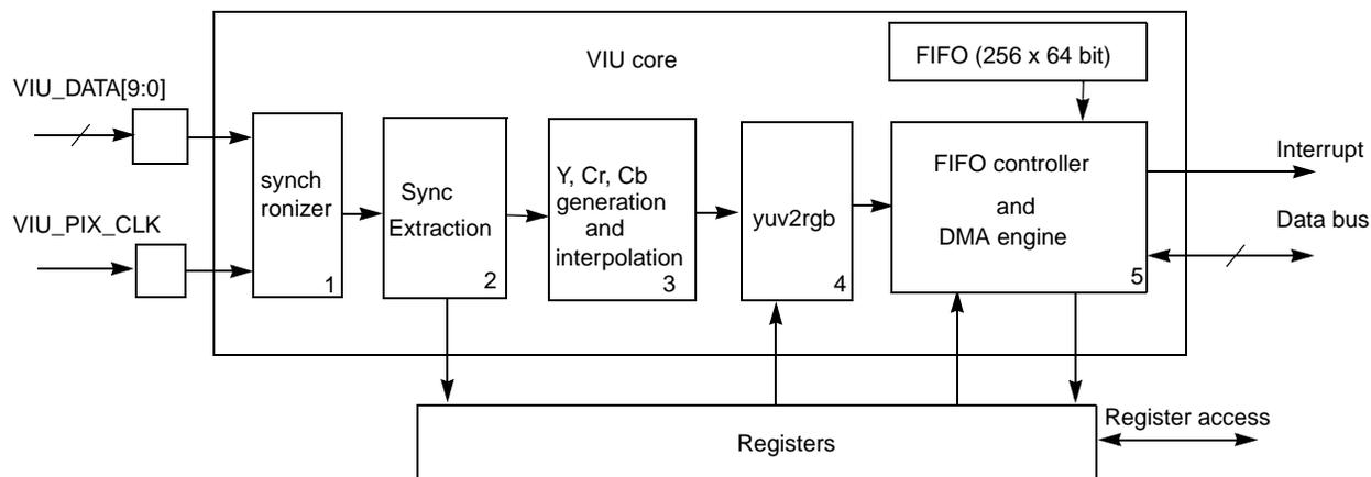
**Figure 40-1. Video In Block Diagram**
