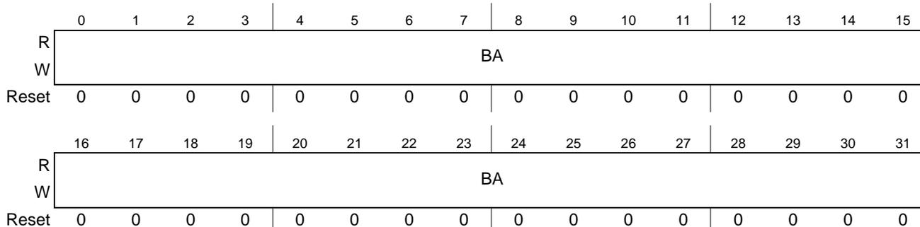
Figure 28-13. PCI Inbound Base Address Registers (PCI\_PCIPIBAR $n$ )
