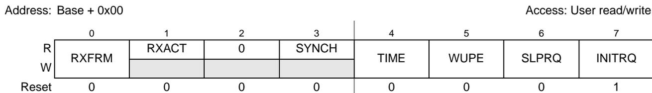
Figure 25-3. MSCAN Control 0 Register (CANCTL0)
