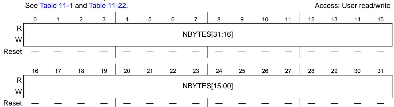
**Figure 11-26. TCD<sub>n</sub> Word 2 (TCD<sub>n</sub>.NBYTES) Field**
