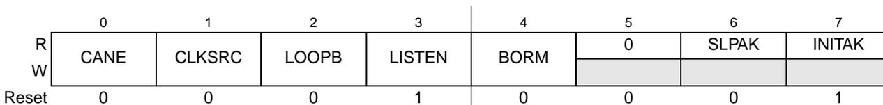
Figure 25-4. MSCAN Control 1 Register (CANCTL1)
