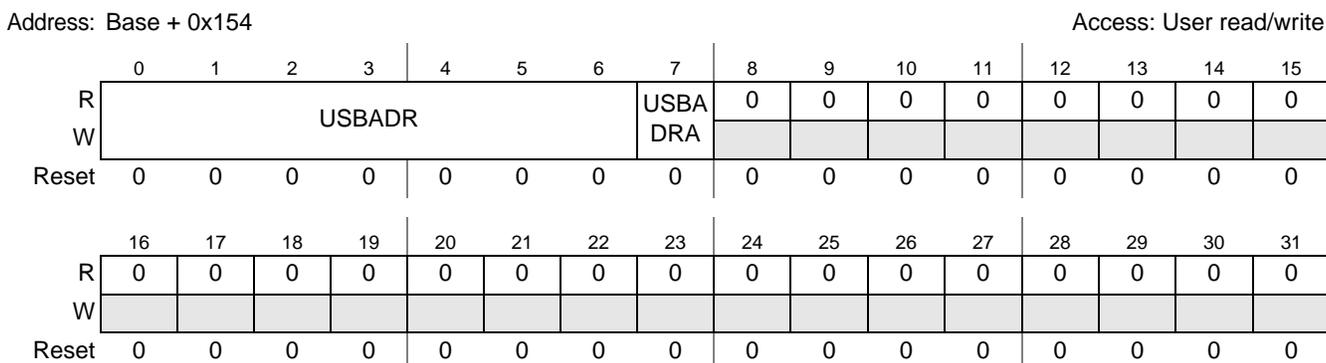
**Figure 39-22. Device Address (USB\_DEVICEADDR) Register**
