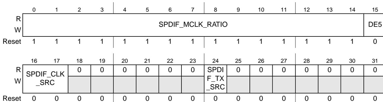
Figure 5-28. SPDIF Clock Control Register (SCCR)
