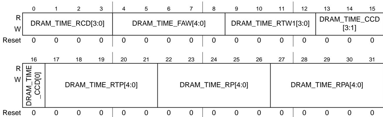
**Figure 13-6. DDR Time Configuration Register 2 (DDR\_TIME\_CONFIG2)**
