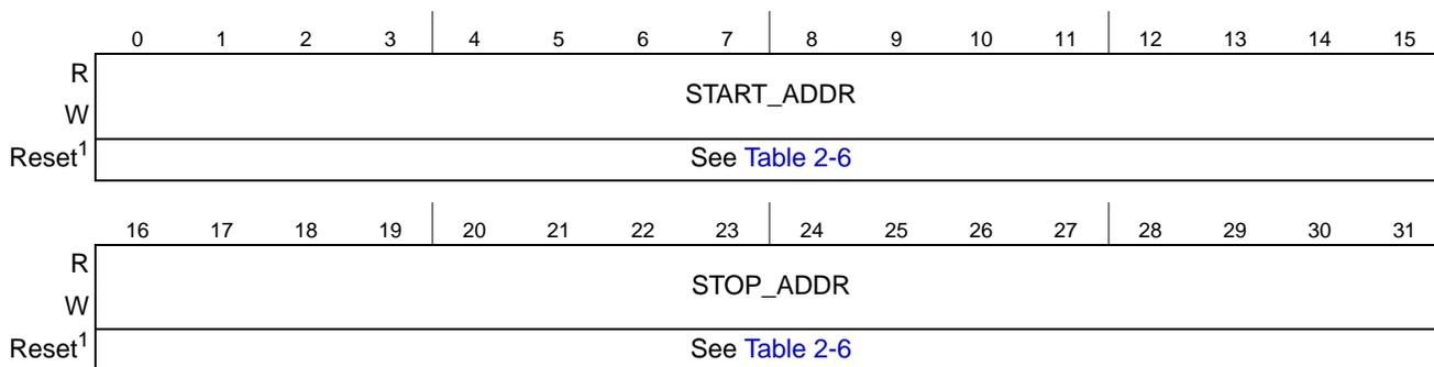
**Figure 2-2. LocalPlus Boot Access Window Register (LPBAW)**
