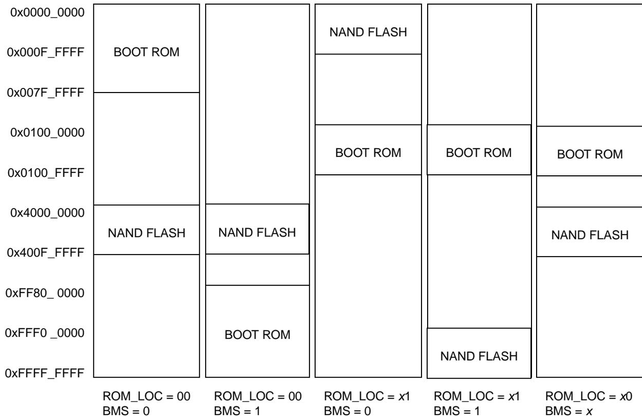
Figure 2-11. Initial Memory Map Configurations Immediately After the Release of  $\overline{\text{PORESET}}$
