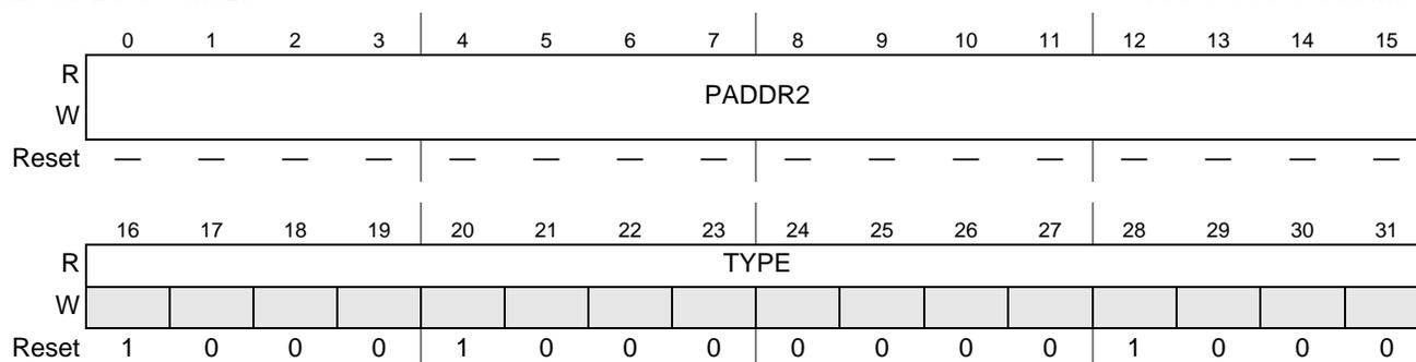
**Figure 16-16. Physical Address High (ETH\_PADDR2) Register**
