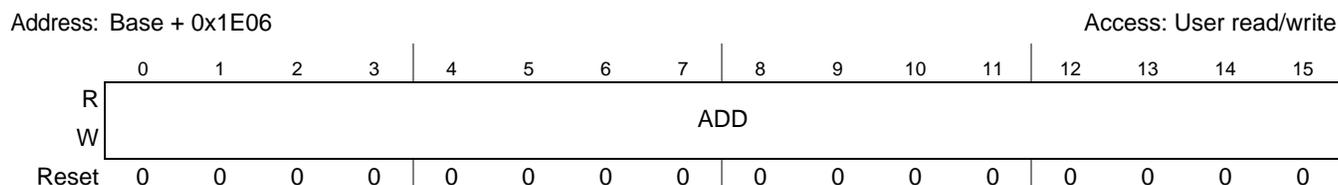
Figure 26-3. NAND Flash Address Register (FLASH\_ADDR)
