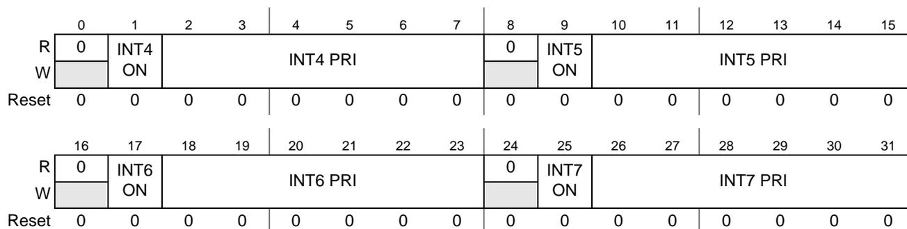
**Figure 6-7. Interrupt Priority Register 1 (INTPRI1)**
