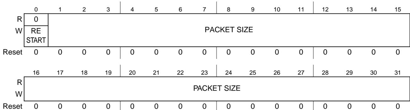
**Figure 23-10. SCLPC Packet Size (LPC\_SCLPC\_PS) Register**
