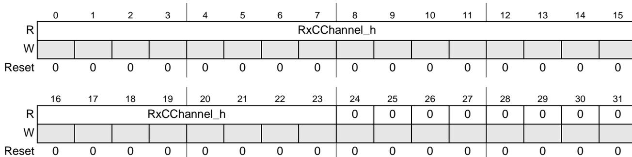
Figure 36-11. SPDIF Receive C Channel Register High (SRCSH)
