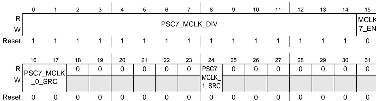
Figure 5-23. PSC7 Clock Control Register (P7CCR)
