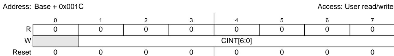
**Figure 11-11. DMA Clear Interrupt Request Register (DMACINT)**
