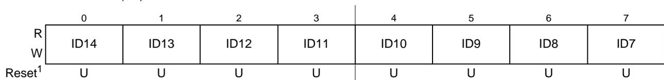
**Figure 25-24. Identifier Register 2 (IDR2)—Extended Identifier Mapping**
