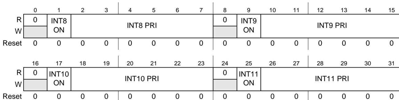
Figure 6-8. Interrupt Priority Register2 (INTPRI2)
