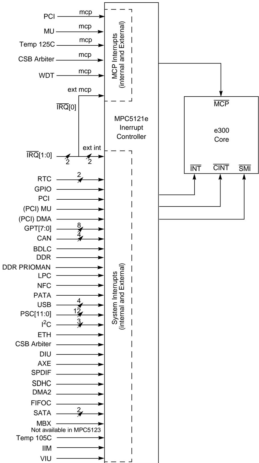
Figure 20-26. MPC5121e Interrupt Structure
