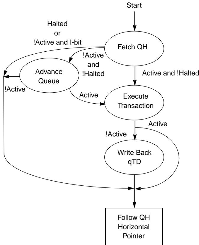
**Figure 39-63. Host Controller Queue Head Traversal State Machine**
