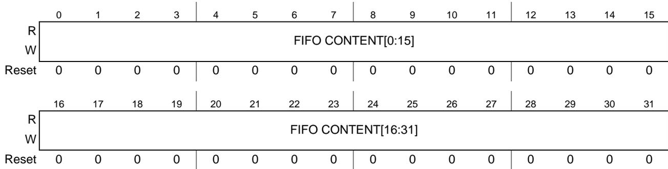
**Figure 34-15. SDHC Data Buffer Access (SDHC\_BUFFER\_ACCESS) Register**
