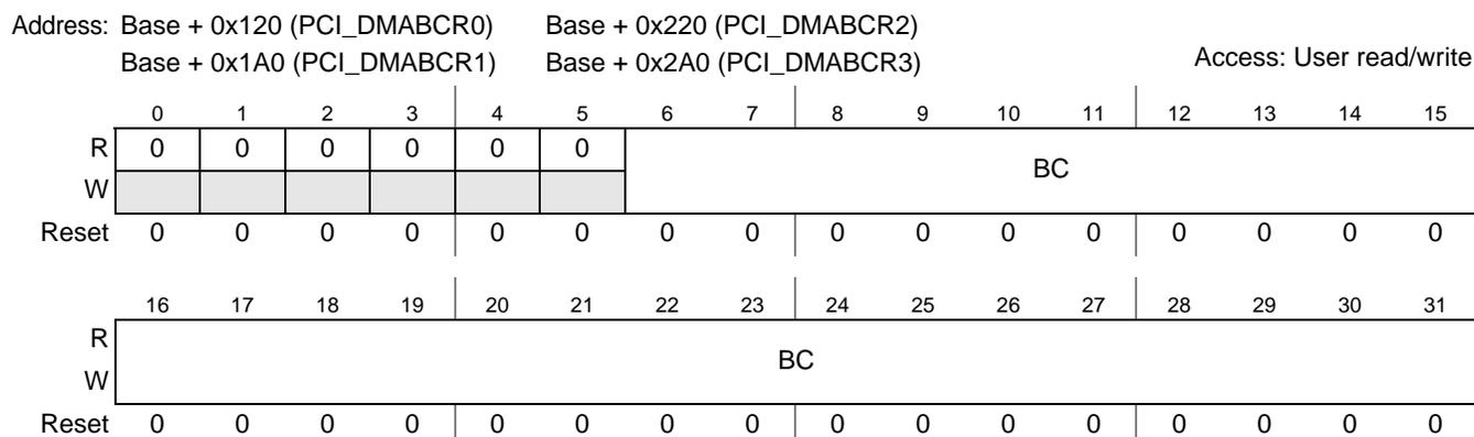
Figure 28-73. DMA Byte Count Register (DMABCR<sub>n</sub>)
