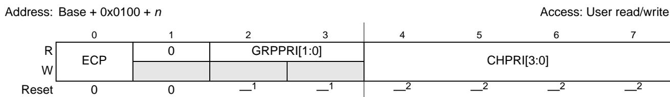
**Figure 11-23. DMA Channel  $n$  Priority Register (DCHPRI $n$ )**
