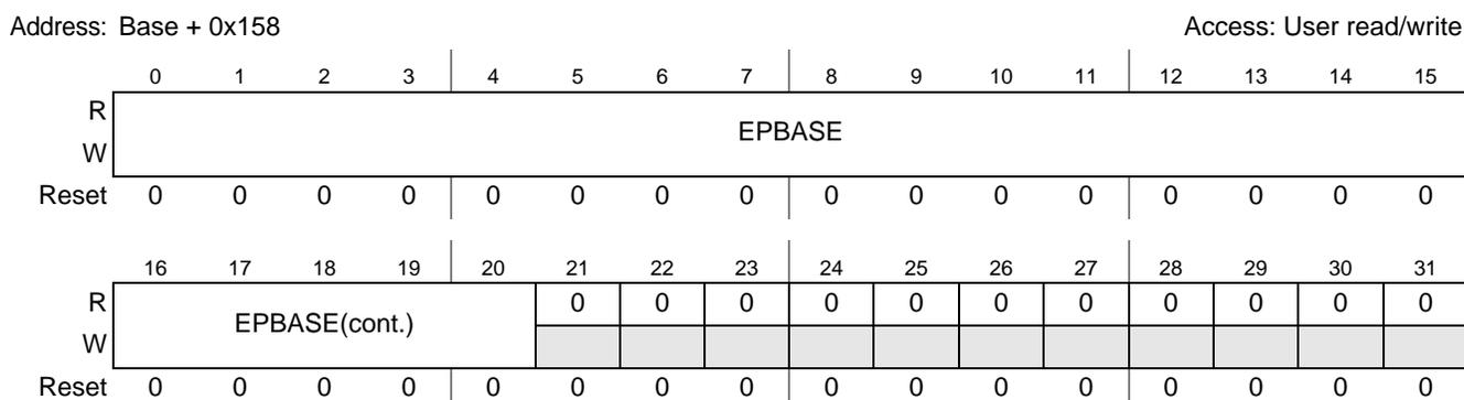
Figure 39-24. Endpoint List Address (USB\_ENDPOINTLISTADDR) Register
