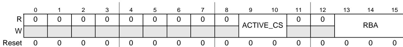
Figure 26-2. Buffer Number for Page Data Transfer Register (RAM\_BUF\_ADDR)
