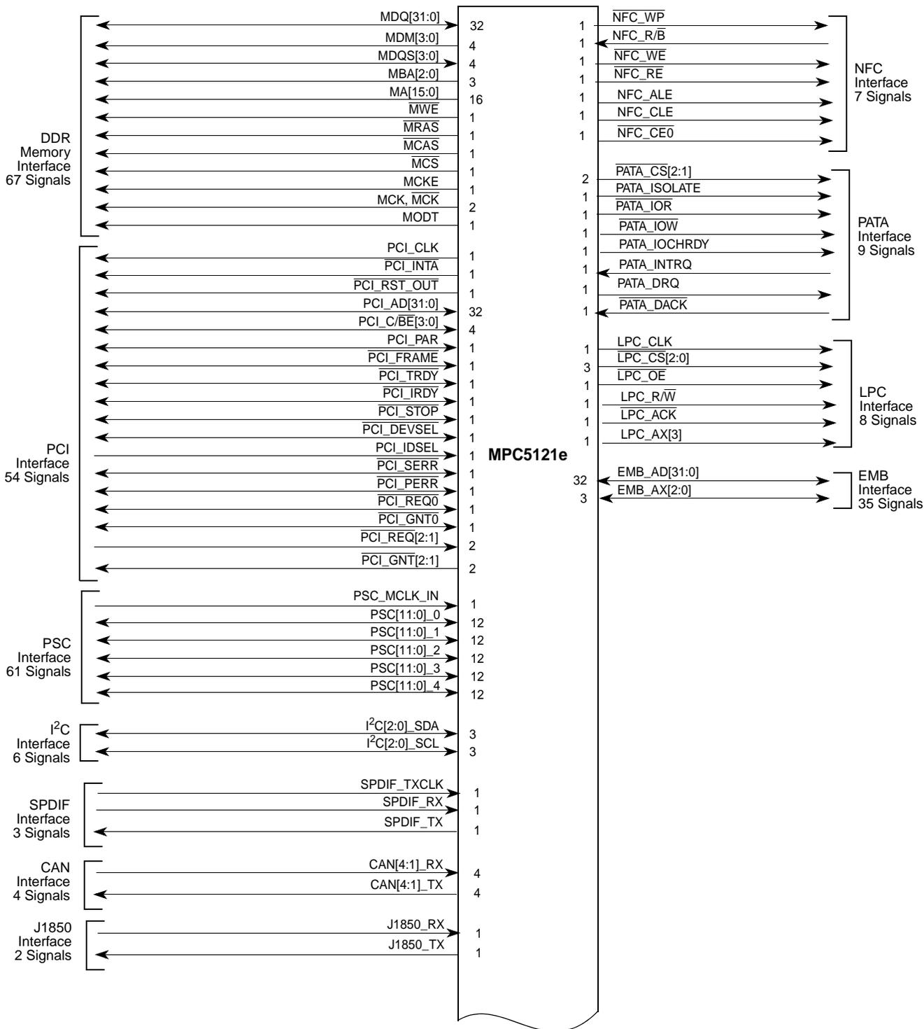
Figure 3-1. MPC5121e Signal Groupings
