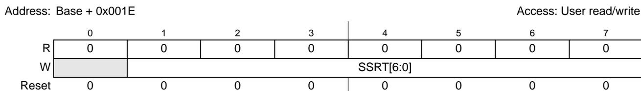
**Figure 11-13. DMA Set START Bit Register (DMASSRT)**
