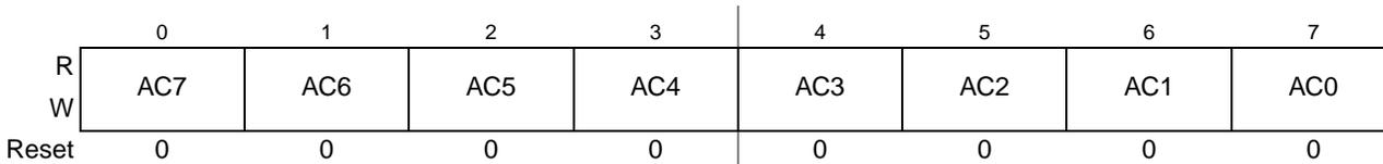
**Figure 25-18. MSCAN Identifier Acceptance Registers (CANIDAR0–CANIDAR7)**
