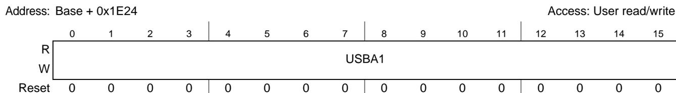
**Figure 26-15. Start Block Address to Unlock in Write Protection Mode Register 1 (NFC\_USBA1)**
