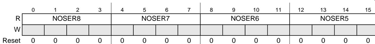
**Figure 26-7. Controller Status and the Result of Flash Operation Register 2 (ECC\_STATUS2)**
