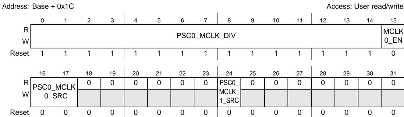
**Figure 5-16. PSC0 Clock Control Register (P0CCR)**
