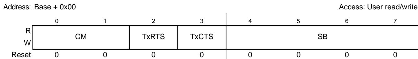
Figure 30-4. Mode Register 2 for UART Mode (MR2)
