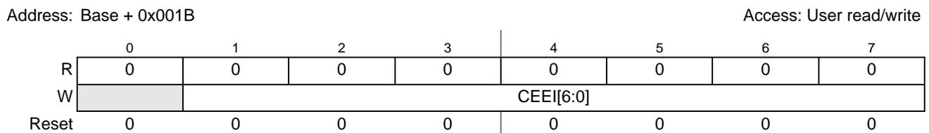
**Figure 11-10. DMA Clear Enable Error Interrupt Register (DMACEEI)**
