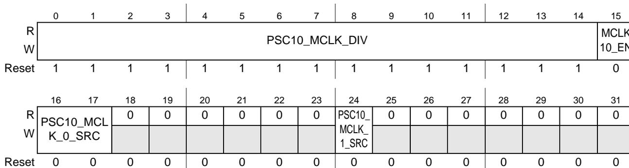
Figure 5-26. PSC10 Clock Control Register 10 (P10CCR)
