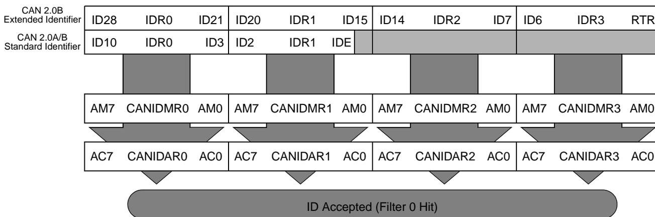
**Figure 25-34. 32-Bit Maskable Identifier Acceptance Filter**
