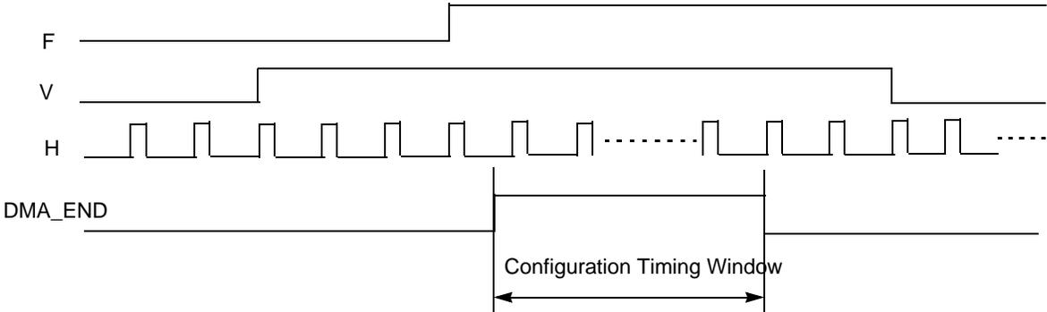
Figure 40-15. Register Configuration Timing Window
