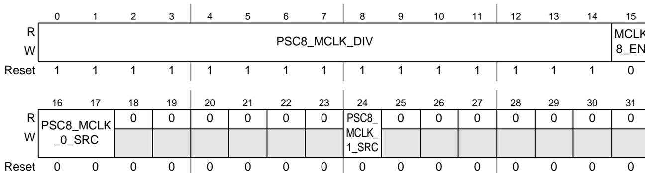
Figure 5-24. PSC8 Clock Control Register (P8CCR)
