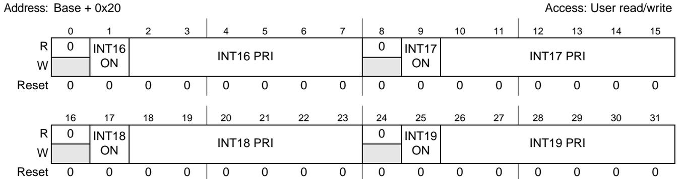
Figure 6-10. Interrupt Priority Register 4 (INTPRI4)
