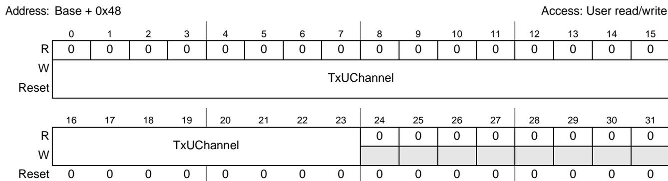
**Figure 36-20. SPDIF Transmit U Channel Register (STU)**
