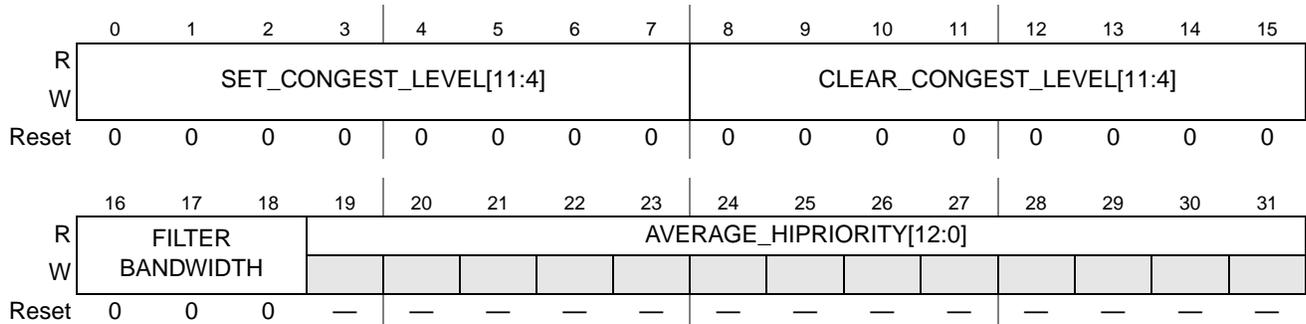
Figure 14-4. High Priority Configuration Register (HIPRIO\_CONFIG)
