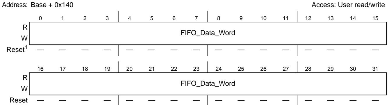
**Figure 23-18. LPC RX/TX FIFO Data Word (LPC\_SCLPC\_FIFOD) Register**
