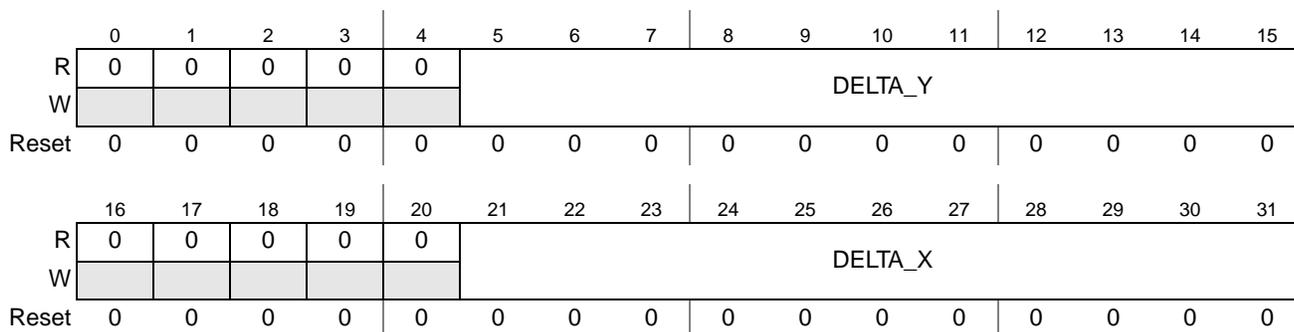
**Figure 12-11. Display Size Register (DISP\_SIZE)**
