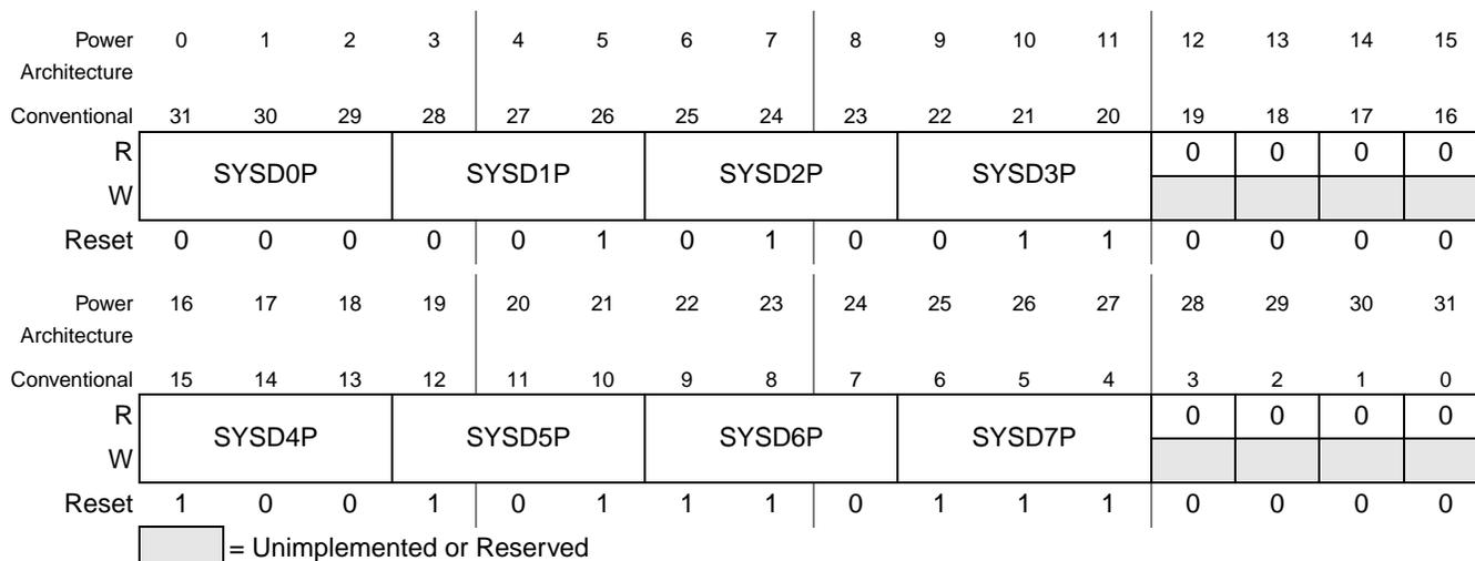
Figure 20-9. System Internal Interrupt Group D Priority Register (SIPRR\_D)
