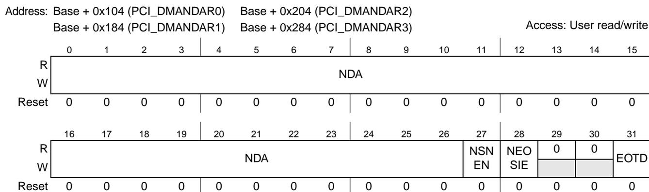
Figure 28-74. DMA Next Descriptor Address Register (PCI\_DMANDAR<sub>n</sub>)
