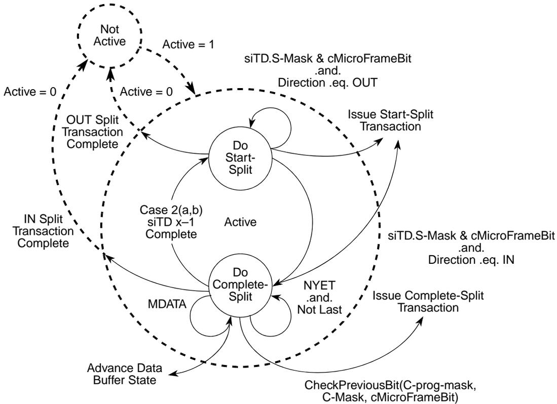
**Figure 39-72. Split Transaction State Machine for Isochronous**
