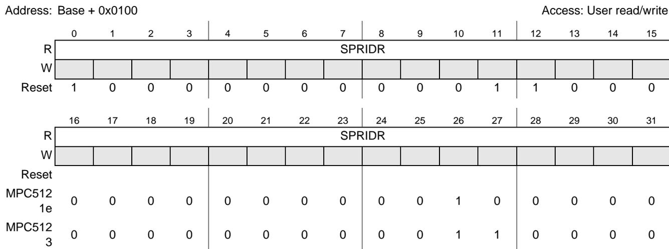
Figure 2-12. System Part and Revision ID Register (SPRIDR)
