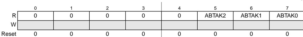
**Figure 25-12. MSCAN Transmitter Message Abort Acknowledge (CANTAACK)**
