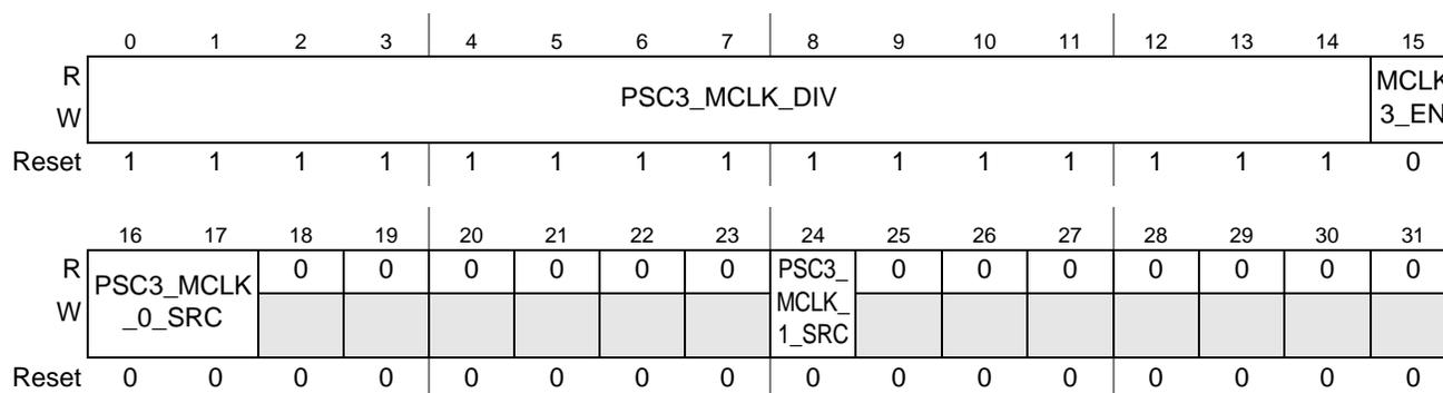
**Figure 5-19. PSC3 Clock Control Register (P3CCR)**
