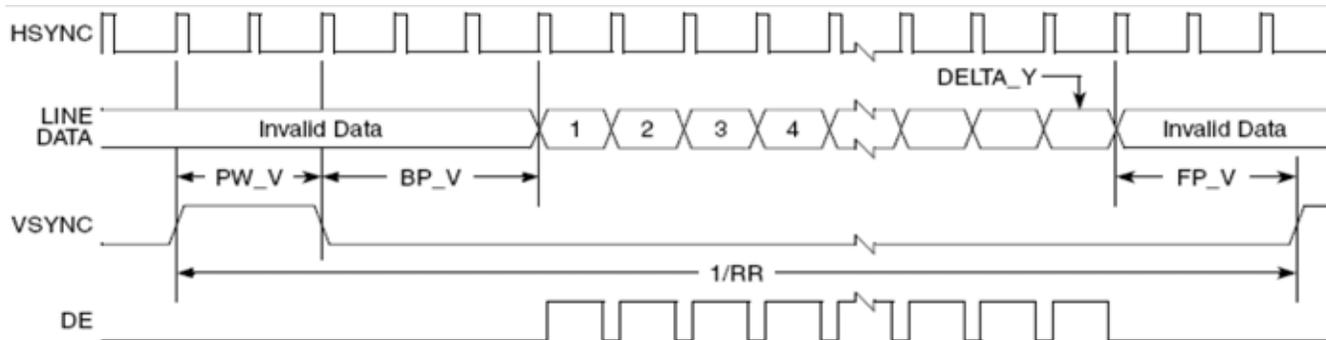
**Figure 12-49. Vertical Sync Signals**
