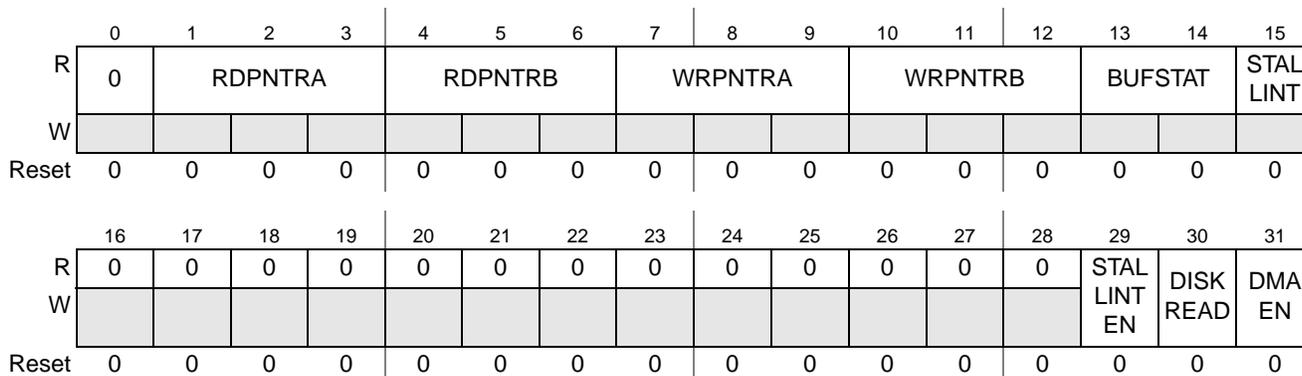
Figure 33-25. DMA Status/Control Register (DMA\_STAT\_CTRL)
