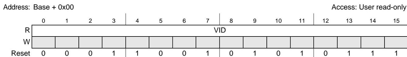
**Figure 28-16. Vendor ID Configuration (PCI\_VENDORIDCFG) Register**
