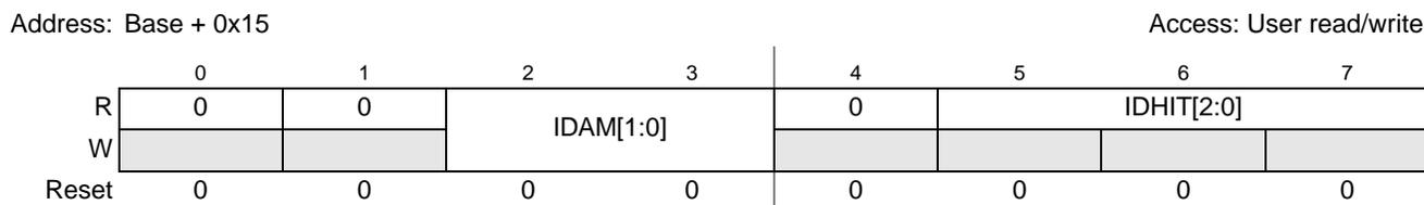
**Figure 25-14. MSCAN Identifier Acceptance Control Register (CANIDAC)**
