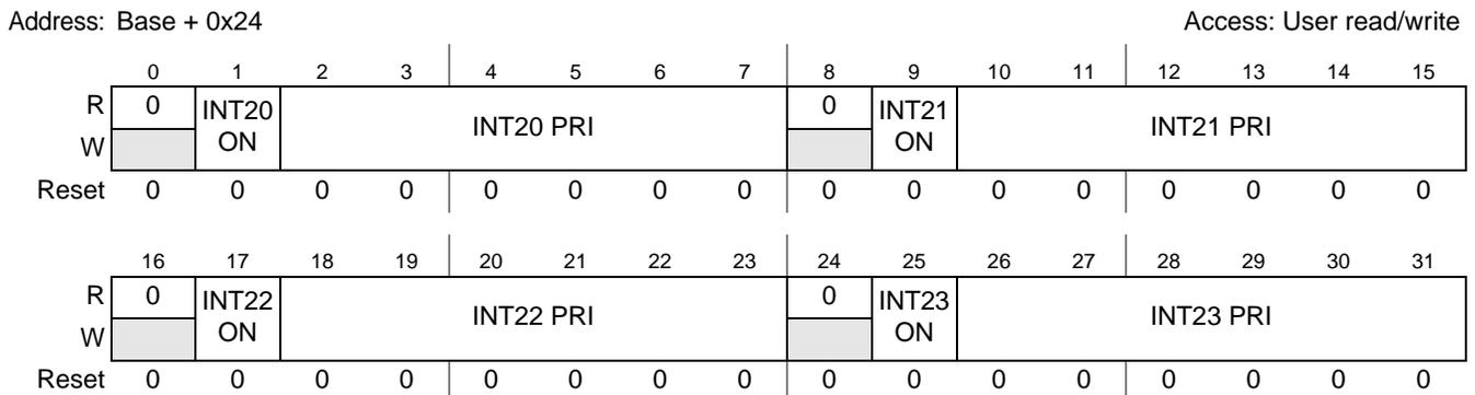
Figure 6-11. Interrupt Priority Register 5 (INTPRI5)
