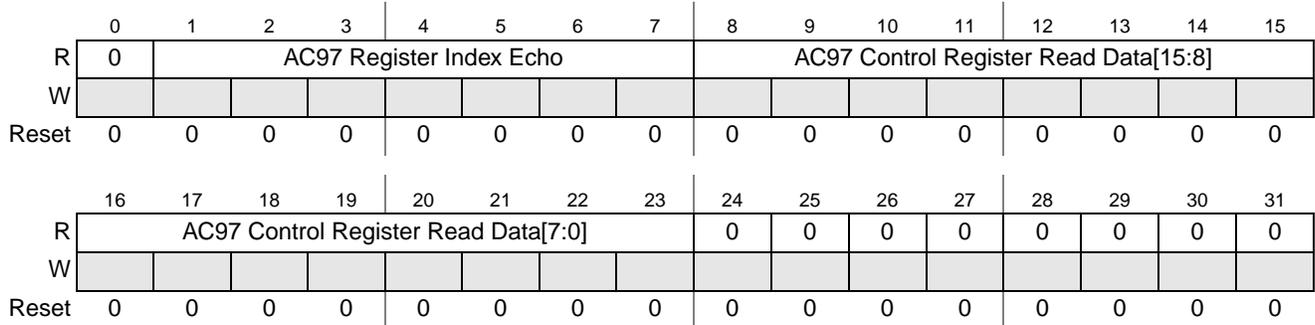
Figure 30-30. AC97 Status Register (AC97Data)
