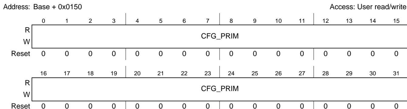
**Figure 33-8. Link Layer Configuration Register 2 (LINK\_CFG2)**
