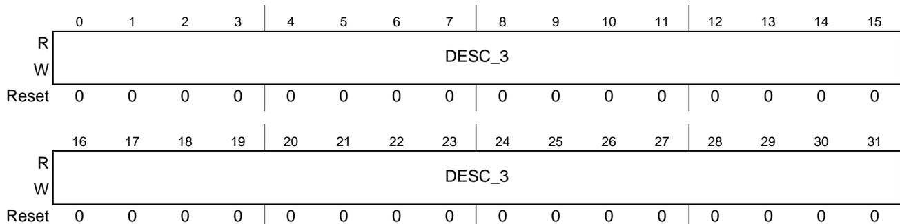
**Figure 12-3. Plane 3 Area Descriptor Pointer Register (DESC\_3)**
