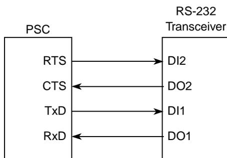
**Figure 30-39. Signal Configuration for a PSC/RS-232 Interface**
