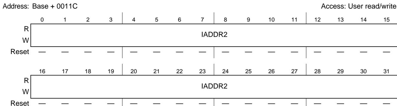
Figure 16-19. Descriptor Individual Address 2 (ETH\_IADDR2) Register
