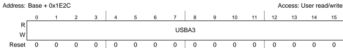
Figure 26-19. Start Block Address to Unlock in Write Protection Mode Register 3 (NFC\_USBA3)
