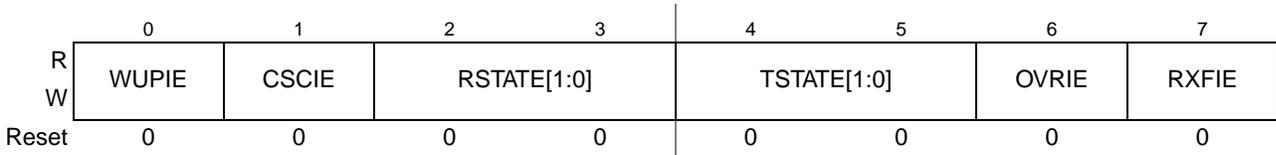
**Figure 25-8. MSCAN Receiver Interrupt Enable Register (CANRIER)**
