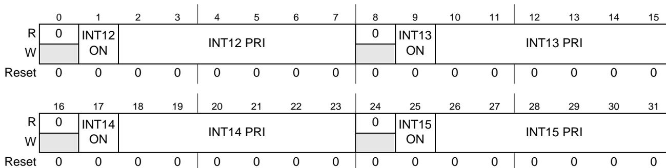
Figure 6-9. Interrupt Priority Register 3 (INTPRI3)
