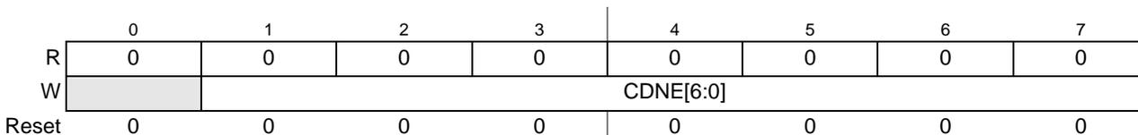
**Figure 11-14. DMA Clear DONE Status Register (DMACDNE)**
