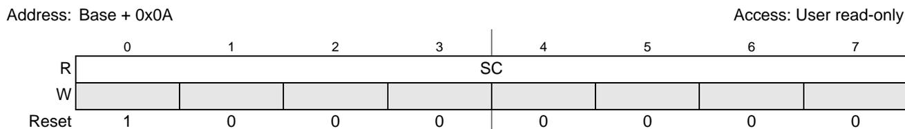
Figure 28-22. Subclass Code Configuration (PCI\_SUBCLSCODCFG) Register
