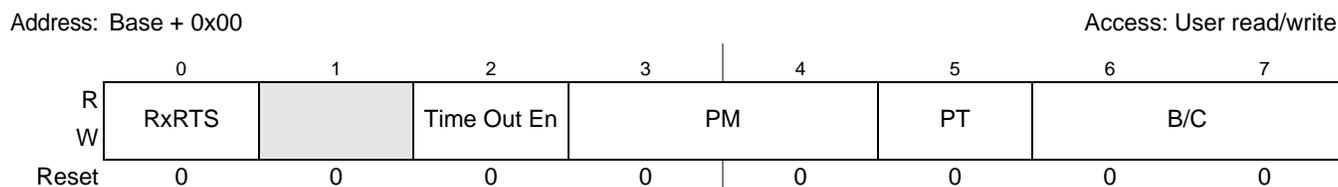
Figure 30-2. Mode Register 1 for UART Mode (MR1)
