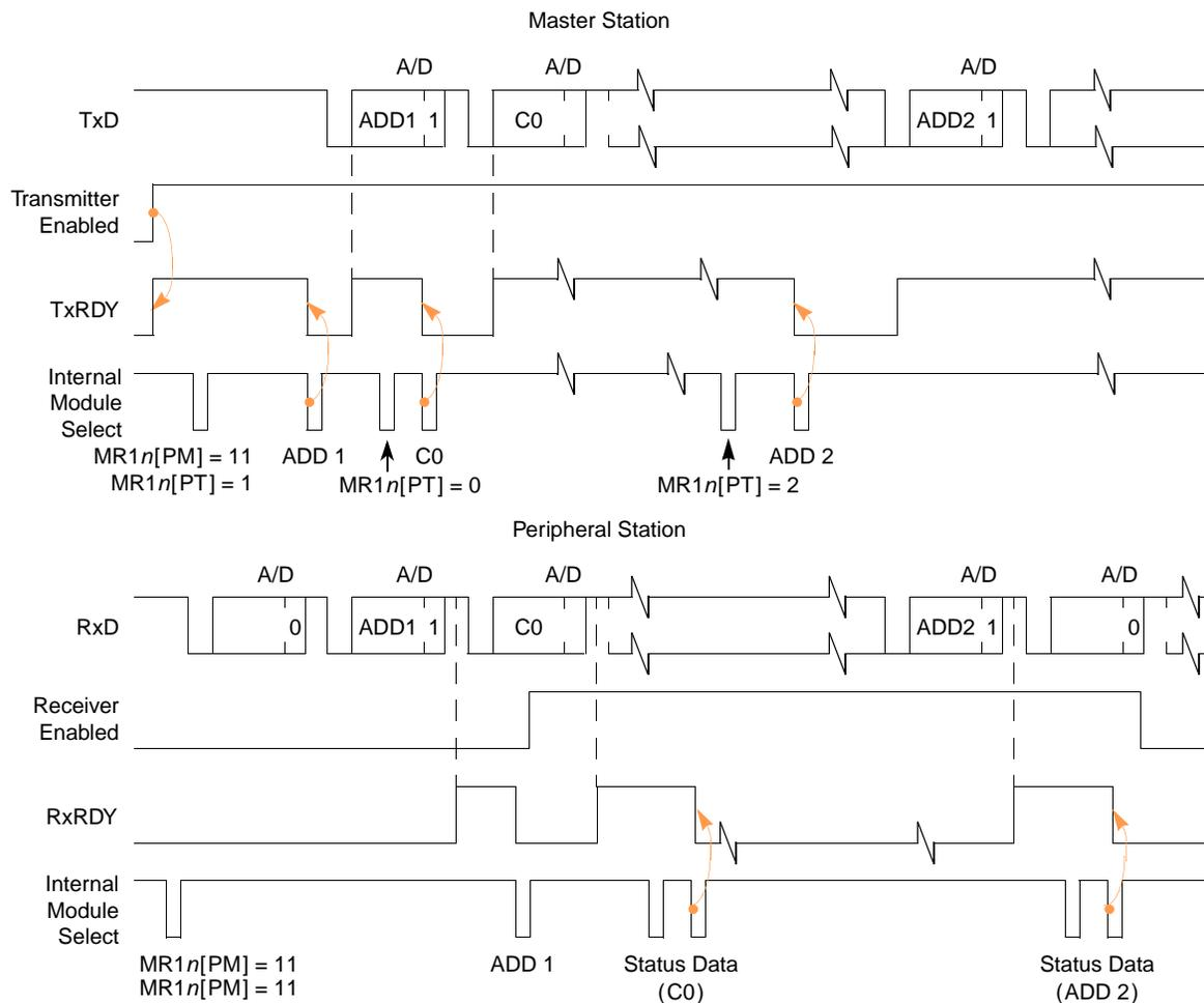
Figure 30-43. Timing Diagram – Multidrop Mode
