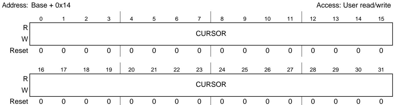
Figure 12-6. Cursor Bitmap Table Pointer Register (CURSOR)
