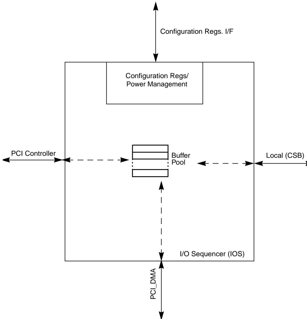
Figure 28-52. PCI Block Diagram
