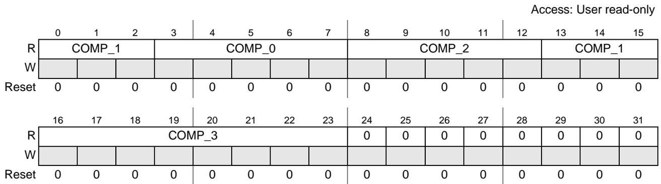
**Figure 12-43. Example of 24-bit ARGB 8:5:6:5 Pixel Structure Definition when BYTE\_F = 0**
