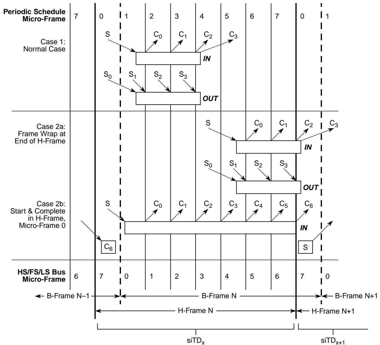
**Figure 39-70. Split Transaction and Isochronous Scheduling Boundary Conditions**
