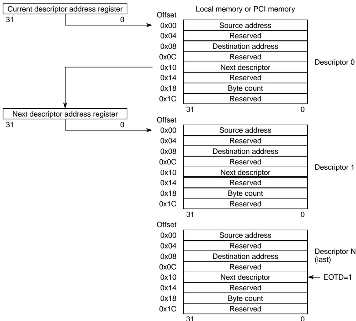
Figure 28-77. DMA Chain of Segment Descriptors
