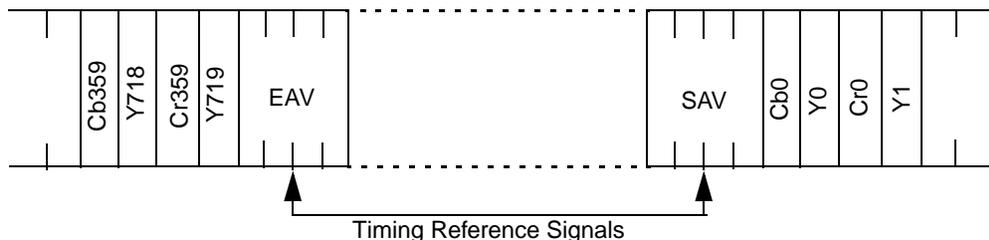
**Figure 40-12. Interface Data Stream of ITU-R BT.656-4**
