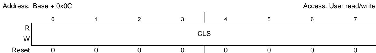
**Figure 28-24. Cache Line Size Configuration (PCI\_CACHELINESZCFG) Register**
