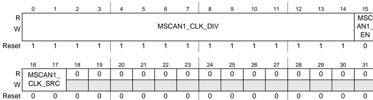
Figure 5-31. MSCAN1 Clock Control Register (M1CCR)
