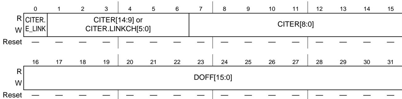
**Figure 11-29. TCD<sub>n</sub> Word 5 (TCD<sub>n</sub>.{CITER,DOFF}) Field**
