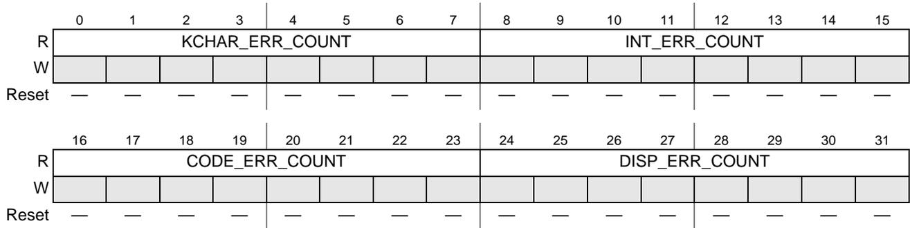
Figure 33-10. Link Layer Status Register 1 (LINK\_STATUS1)
