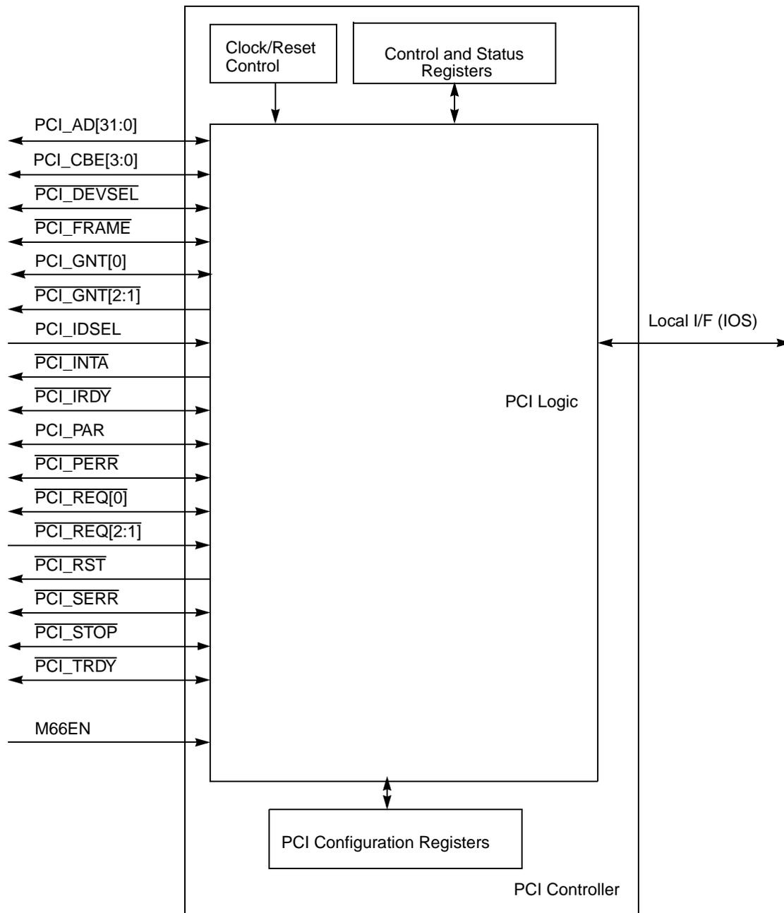
Figure 28-1. PCI Block Diagram
