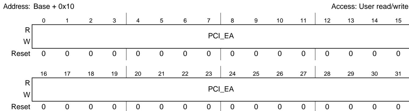
**Figure 28-6. PCI Error Address Capture Register (PCI\_PCIEACR)**
