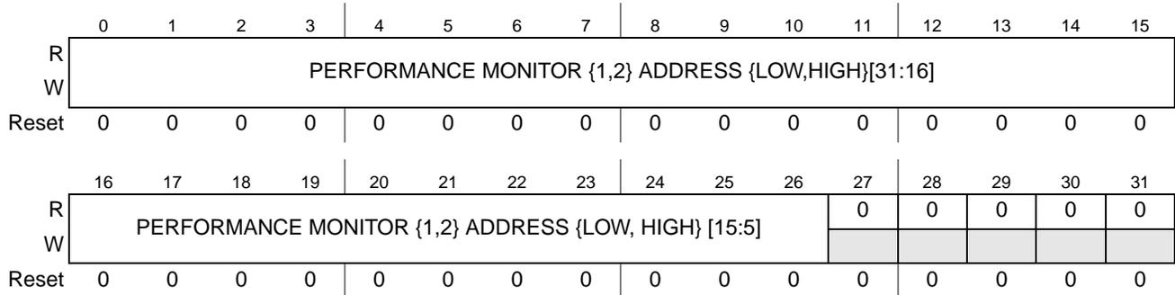
Figure 14-12. Performance Monitor Address Registers
