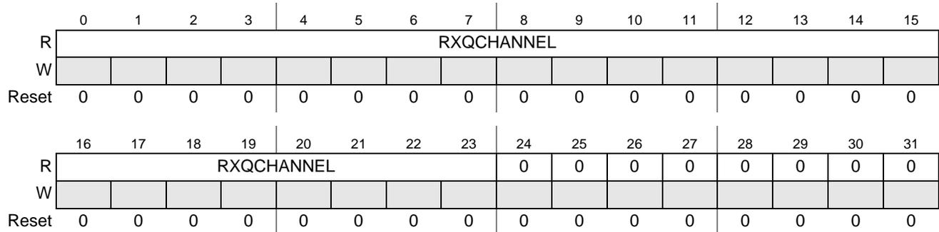
**Figure 36-14. SPDIF Receive Q Channel Register (SRQ)**
