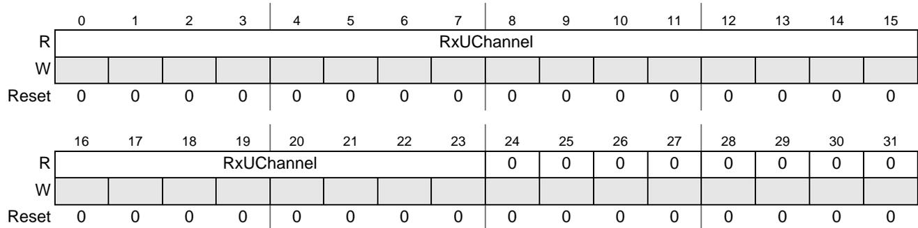
**Figure 36-13. SPDIF Receive U Channel Register (SRU)**
