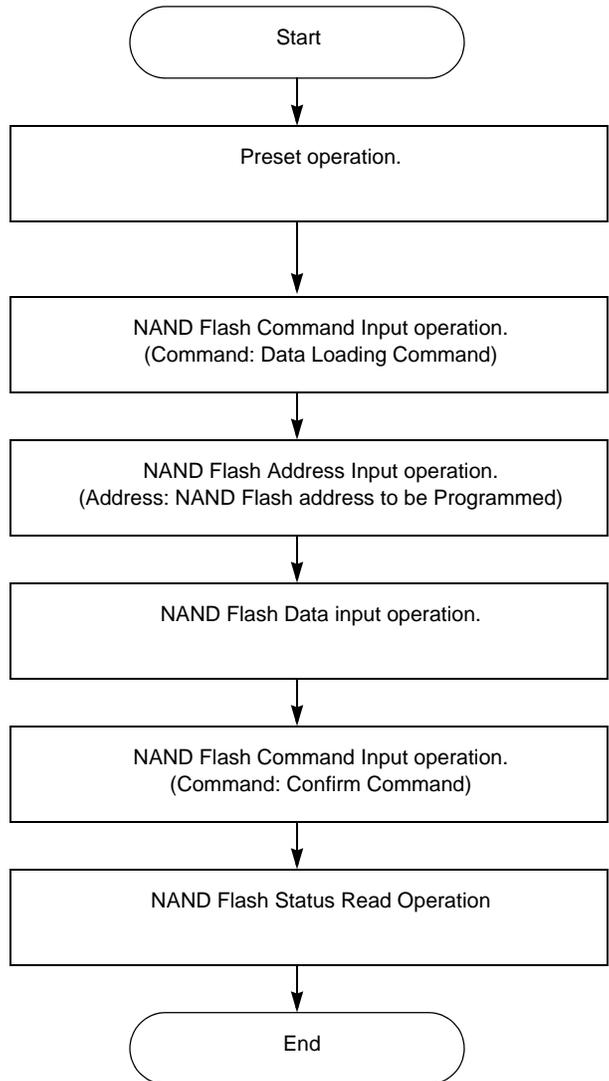
Figure 26-42. Flow Chart of Program NAND Flash Data Operation
