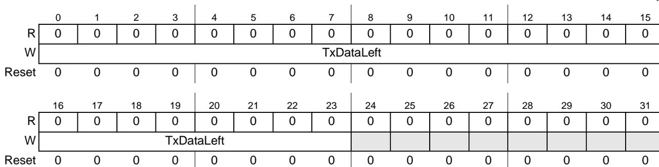
Figure 36-16. SPDIF Transmit Left Channel Register (STXL)
