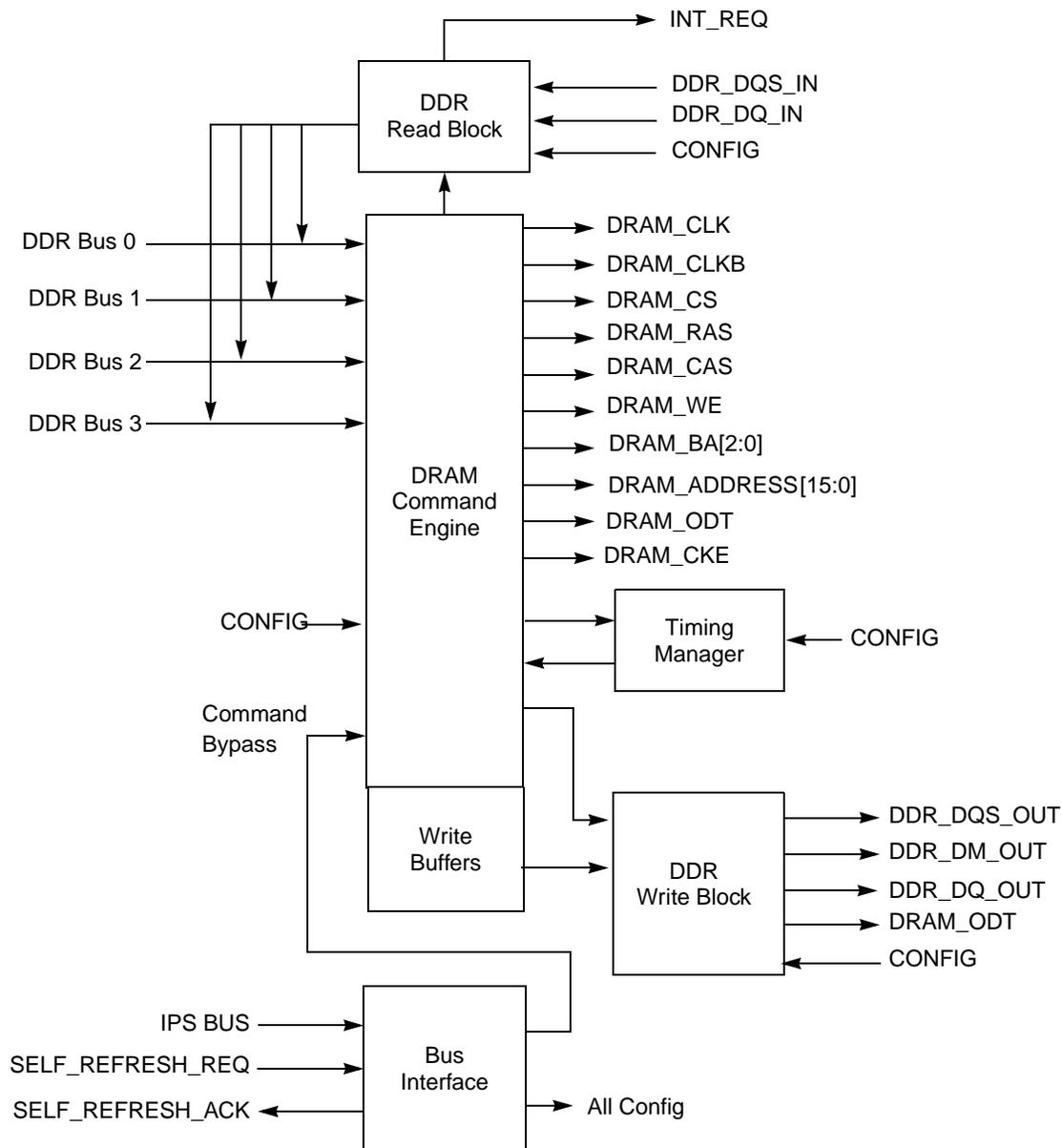
**Figure 13-1. Block Diagram of the Multi-port DRAM Controller**
