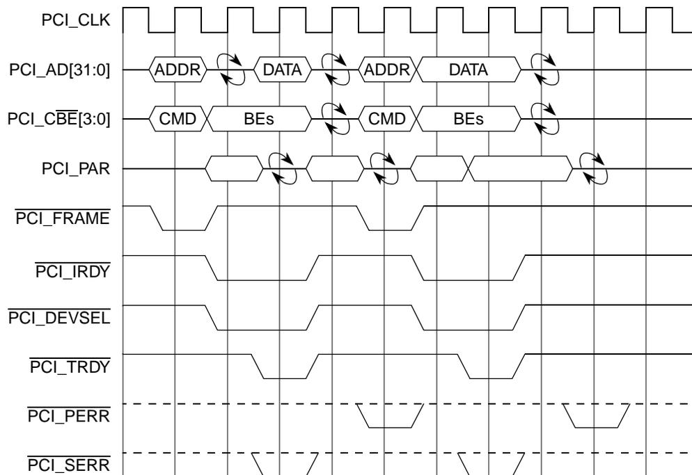
**Figure 28-50. PCI Parity Operation**
