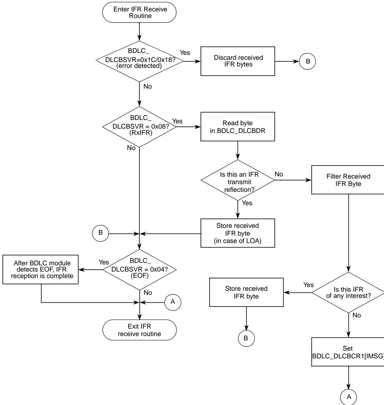
**Figure 7-25. Receiving An IFR with the BDLC Module**
