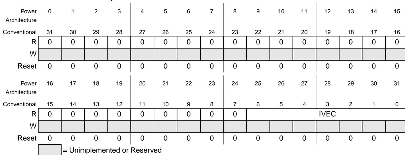
Figure 20-3. System Global Interrupt Vector Register (SIVCR)
