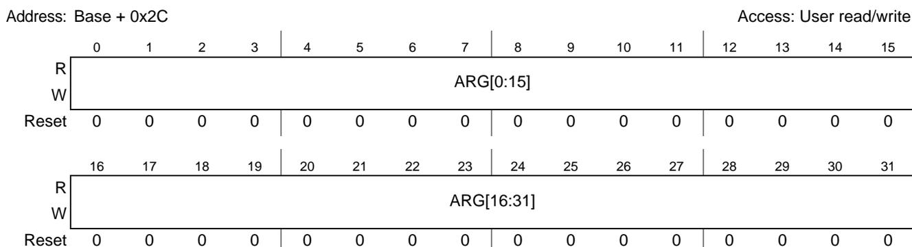
**Figure 34-13. SDHC Command Argument (SDHC\_ARG) Register**
