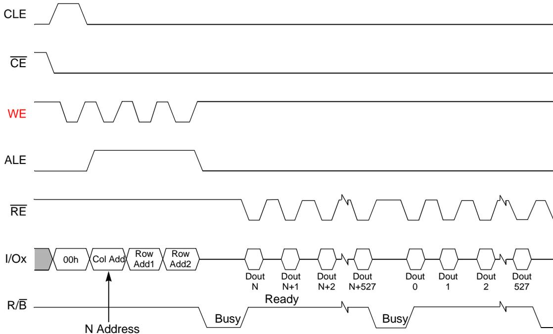
Figure 26-22. Read Operation A (Without Command 30H)
