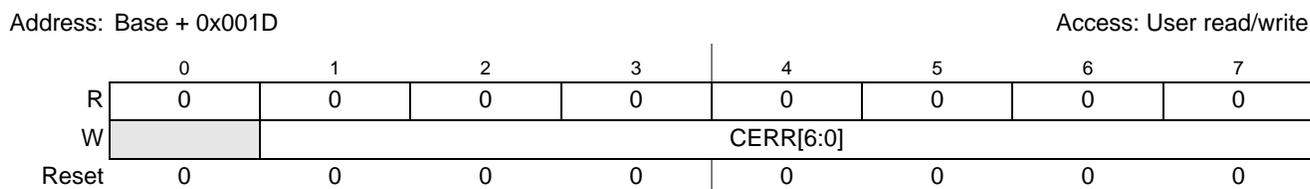
**Figure 11-12. DMA Clear Error Register (DMACERR)**
