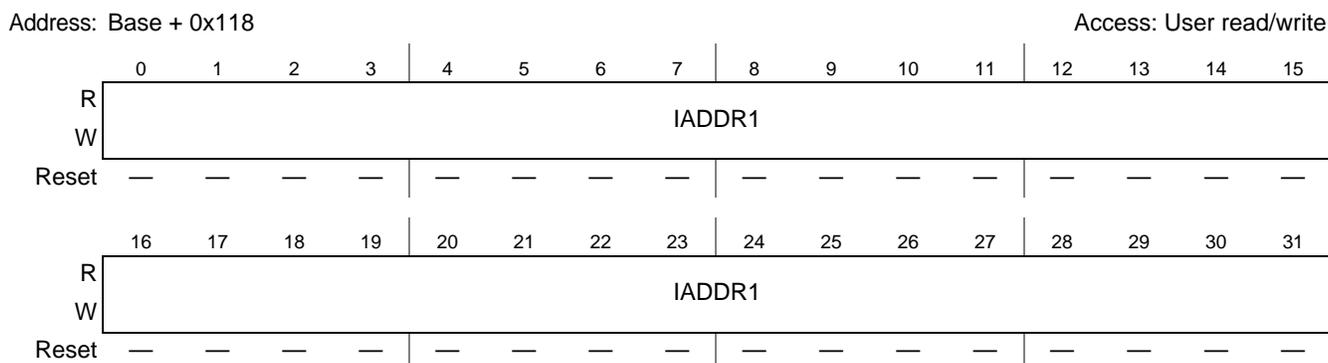
**Figure 16-18. Descriptor Individual Address 1 (ETH\_IADDR1) Register**
