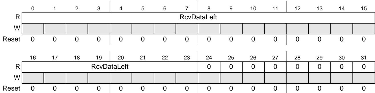
**Figure 36-6. SPDIF Receive Data Left Channel Register (SRXL)**
