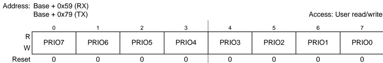
**Figure 25-30. Transmit Buffer Priority Register (TBPR)**
