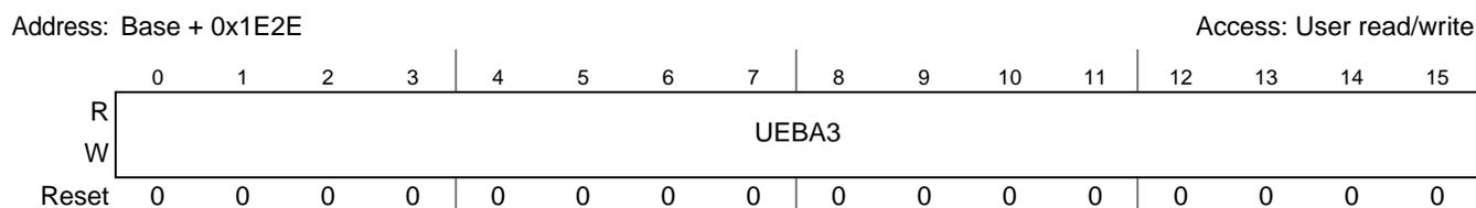
Figure 26-20. End Block Address to Unlock in Write Protection Mode Register 3 (NFC\_UEBA3)
