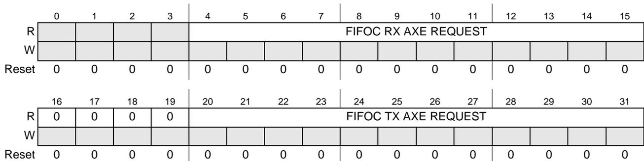
Figure 31-14. FIFOC AXE Request Register (FIFOC\_AXE)
