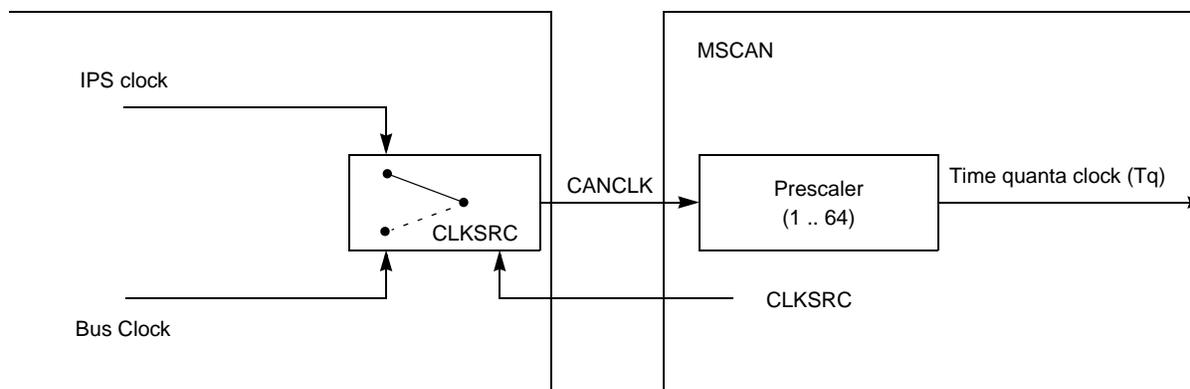
**Figure 25-37. MSCAN Clocking Scheme**
