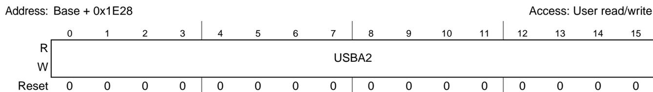
**Figure 26-17. Start Block Address to Unlock in Write Protection Mode Register 2 (NFC\_USBA2)**
