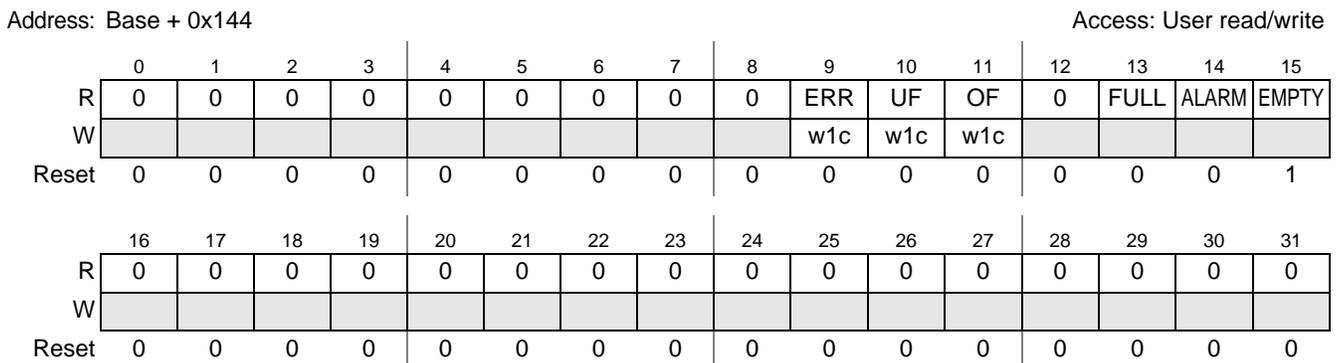
**Figure 23-19. LPC RX/TX FIFO Status (LPC\_SCLPC\_FIFOS) Register**
