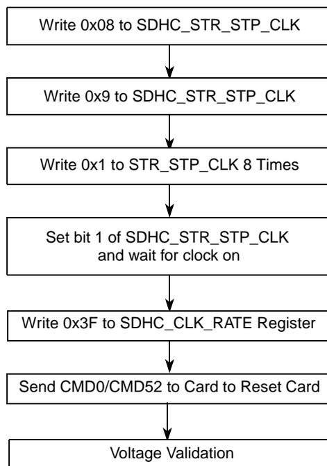
**Figure 34-24. Flow Chart for Reset of SDHC and SD I/O Card**
