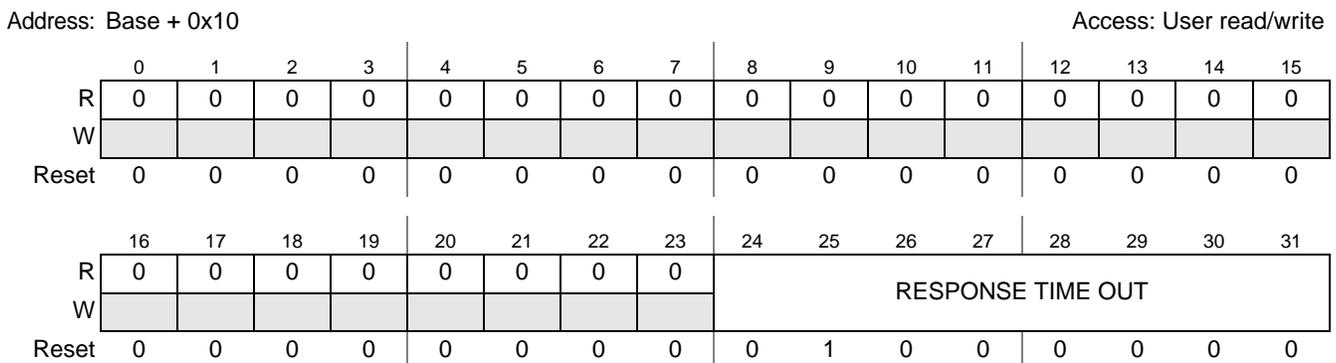
**Figure 34-6. SDHC Response Time Out (SDHC\_RES\_TO) Register**
