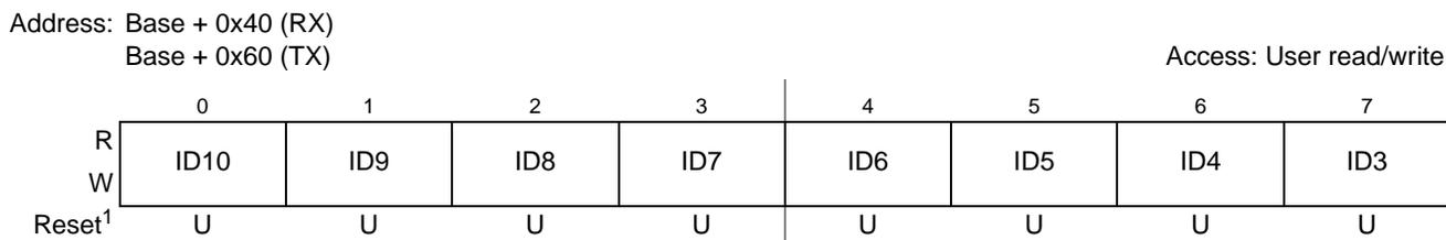
**Figure 25-26. Identifier Register 0 (IDR0)—Standard Mapping**
