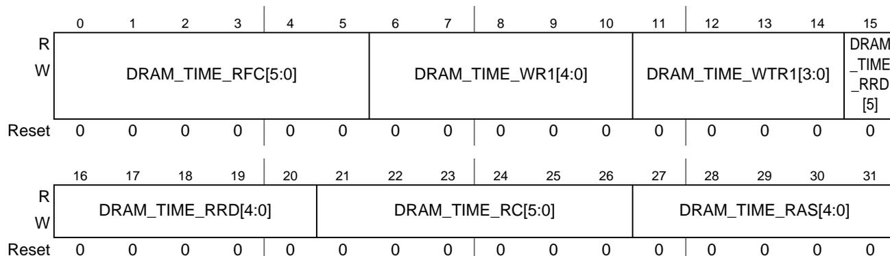
**Figure 13-5. DDR Time Configuration Register 1 (DDR\_TIME\_CONFIG1)**
