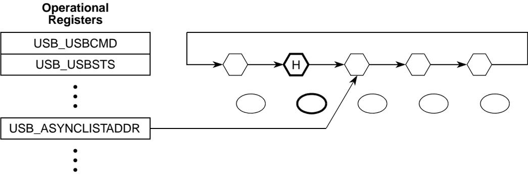
**Figure 39-54. General Format of Asynchronous Schedule List**
