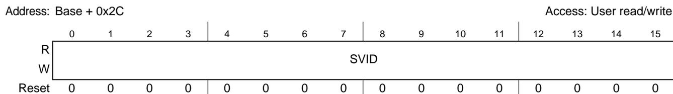
**Figure 28-31. Sub-System Vendor ID Configuration (PCI\_SUBSYSVENDORIDCFG) Register**
