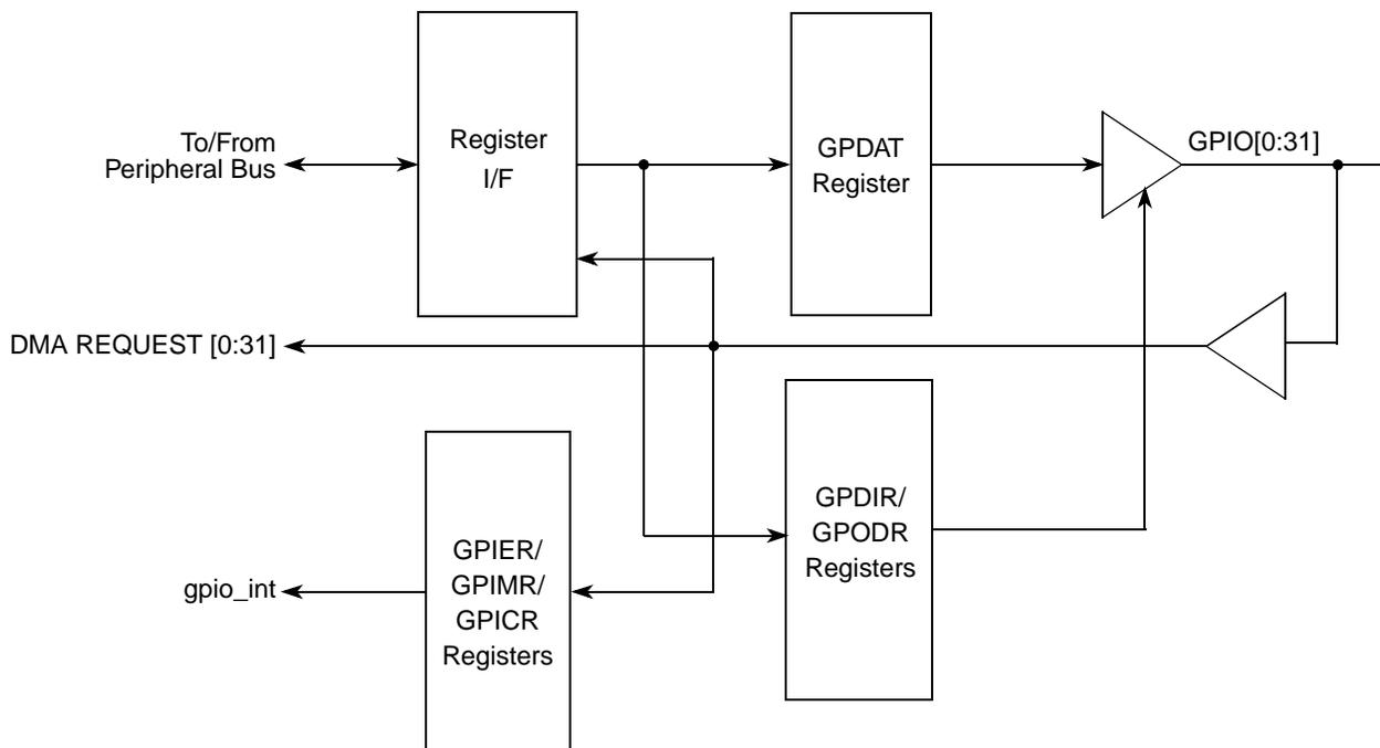
Figure 18-1. GPIO Module Block Diagram
