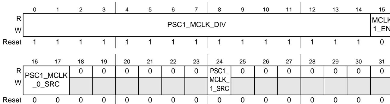
**Figure 5-17. PSC1 Clock Control Register (P1CCR)**
