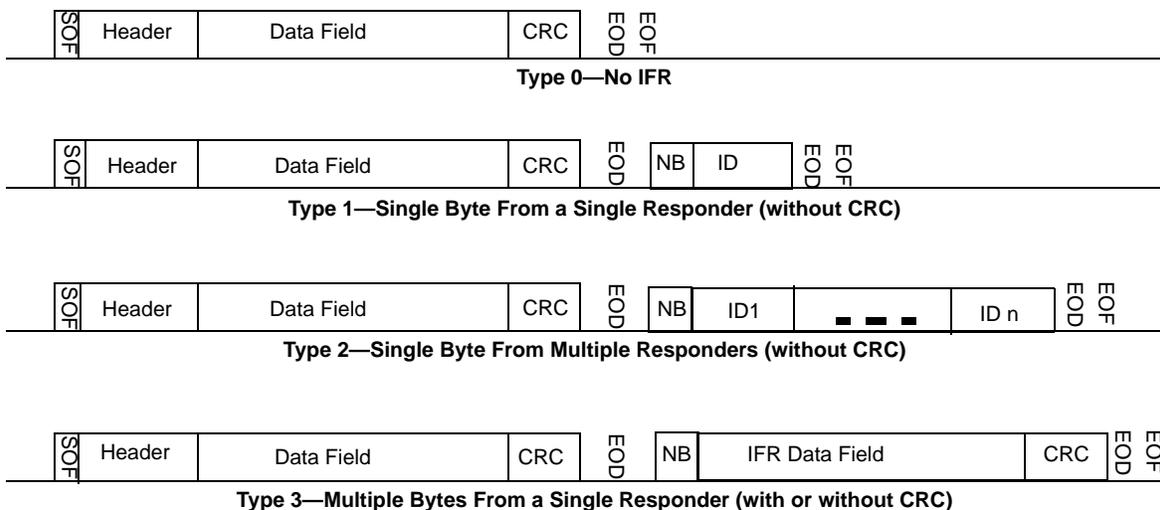
**Figure 7-5. Types of In-Frame Response**
