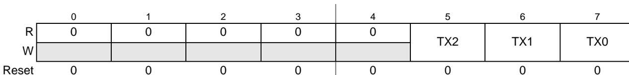
Figure 25-13. MSCAN Transmitter Buffer Selection (CANTBSEL)
