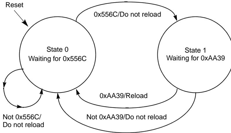
**Figure 35-4. Software Watchdog Timer Service State Diagram**
