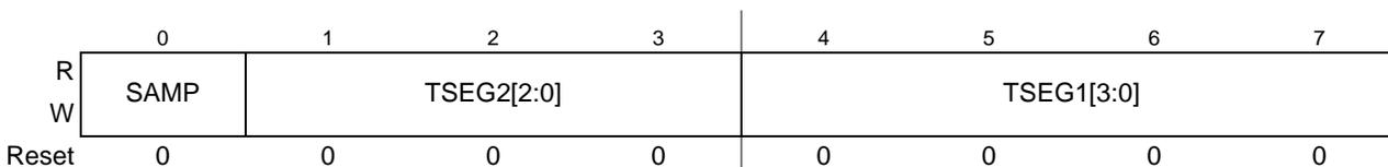
Figure 25-6. MSCAN Bus Timing Register 1 (CANBTR1)
