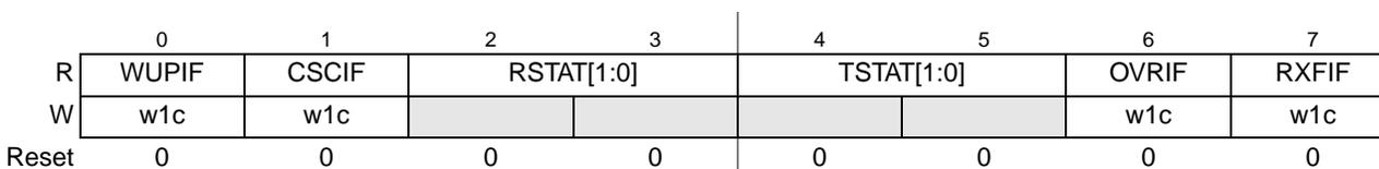
Figure 25-7. MSCAN Receiver Flag Register (CANRFLG)
