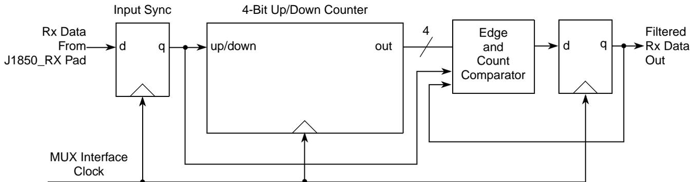
**Figure 7-18. BDLC Module Rx Digital Filter Block Diagram**
