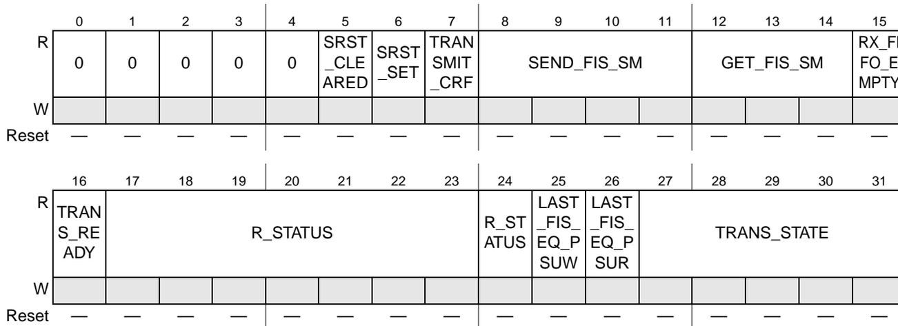
Figure 33-5. Transport Layer Status Register 0 (TRANS\_STATUS0)
