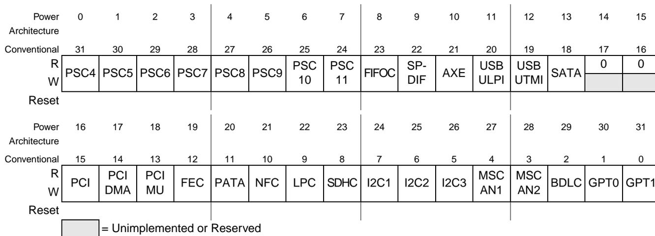
**Figure 20-20. System Internal Interrupt Force Register (SIFCR\_H)**
