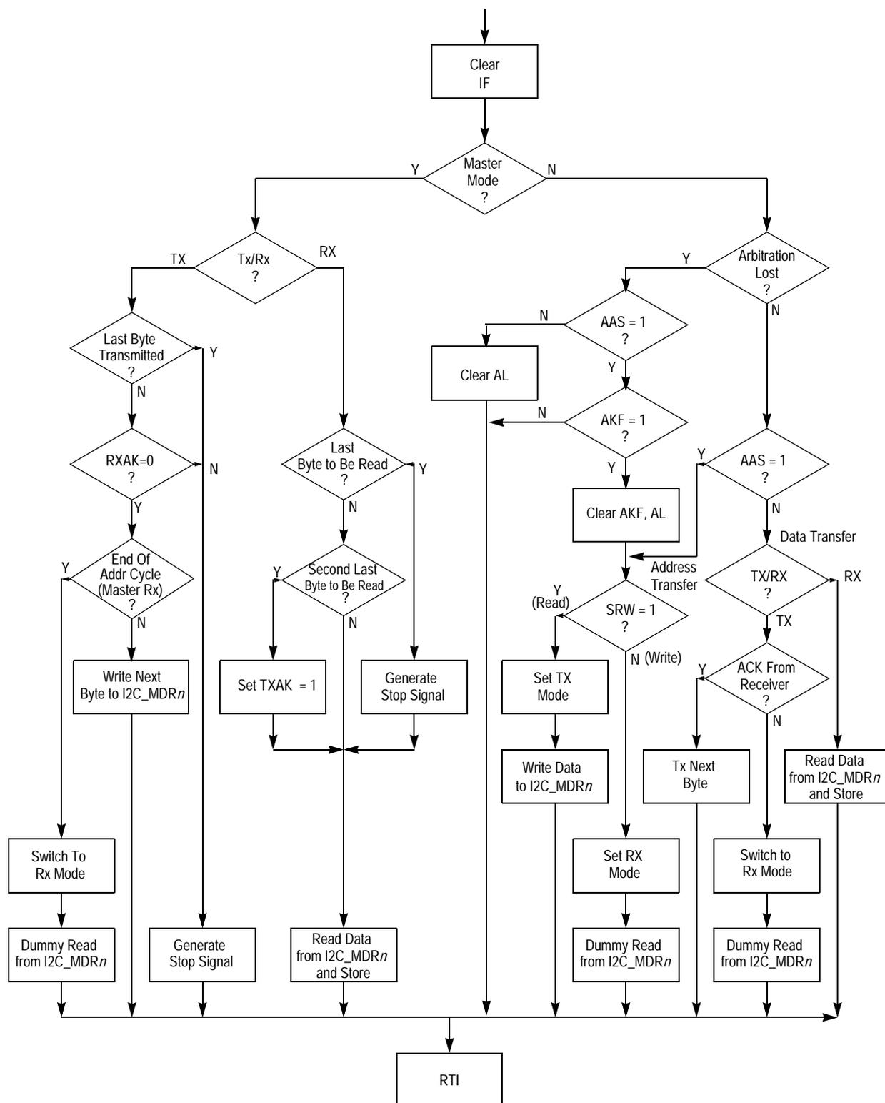
Figure 21-16. Software Flowchart of Typical I<sup>2</sup>C Interrupt Routine
