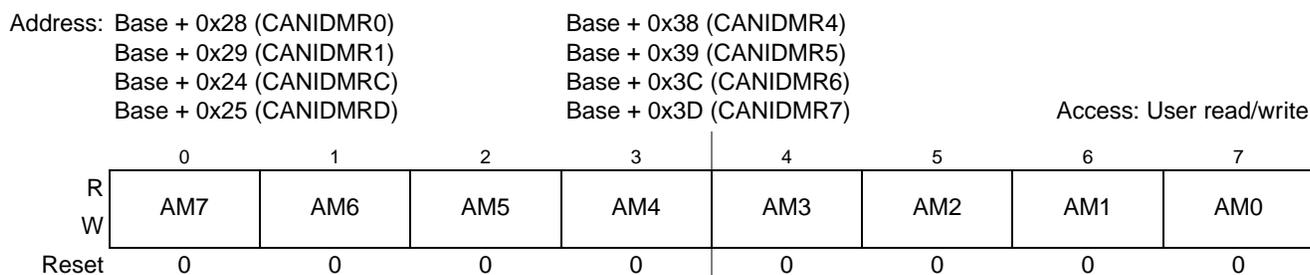
**Figure 25-19. MSCAN Identifier Mask Registers (CANIDMR0–CANIDMR7)**
