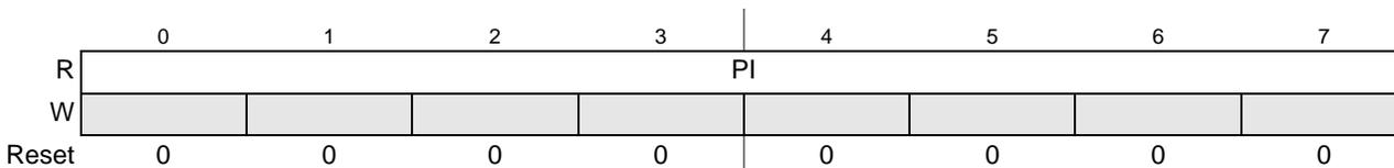
**Figure 28-21. Standard Programming Interface Configuration (PCI\_STDPROGIFCFG) Register**
