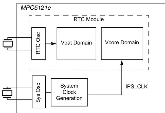
**Figure 5-6. RTC Clock Generation**
