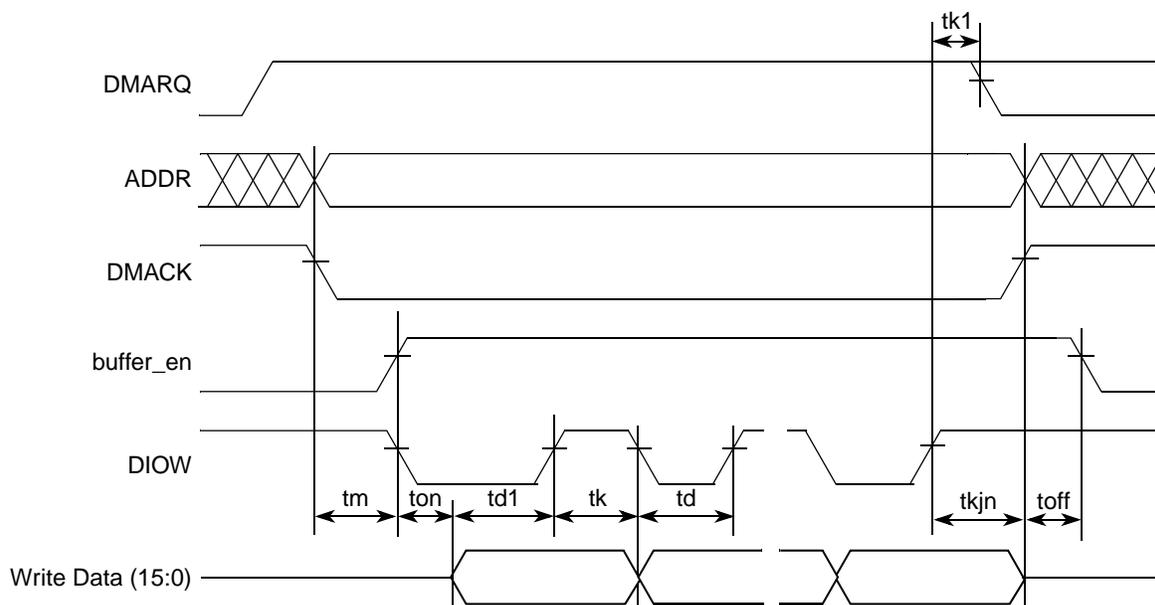
Figure 27-19. MDMA Write Timing
