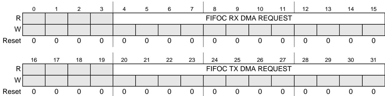
Figure 31-13. FIFOC DMA Request Register (FIFOC\_DMA)
