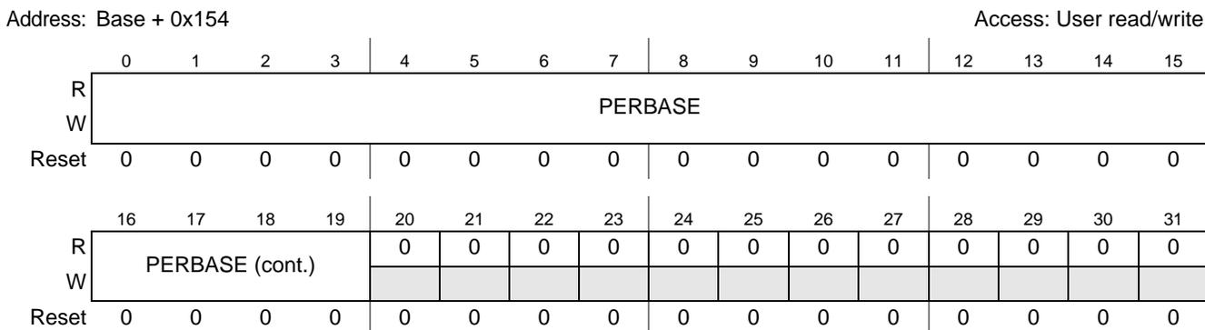
**Figure 39-21. Periodic Frame List Base Address (USB\_PERIODICLISTBASE) Register**
