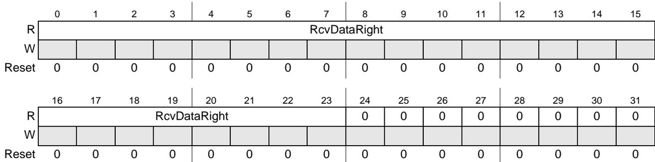
**Figure 36-7. SPDIF Receive Data Right Channel Register (SRXR)**
