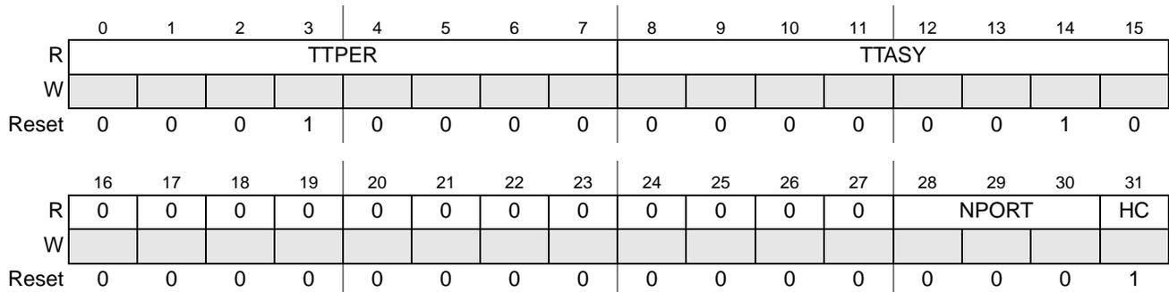
**Figure 39-5. Host Hardware Parameters (USB\_HWHOST) Register**
