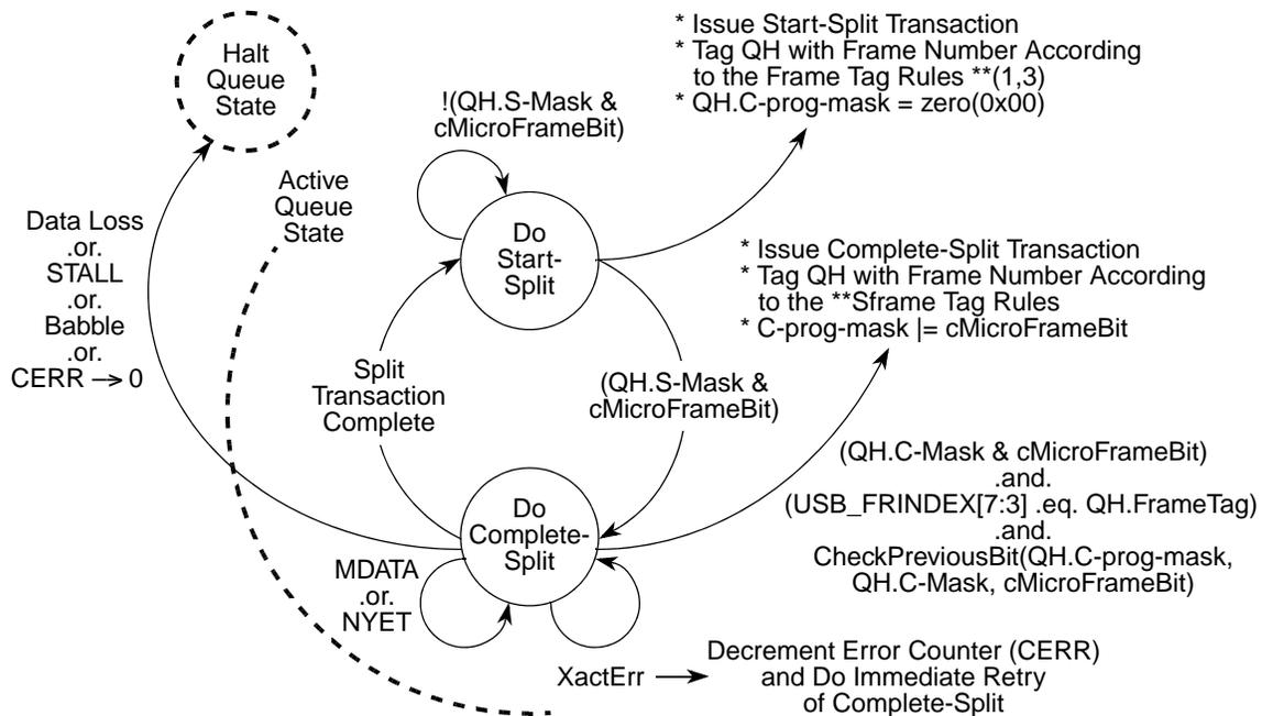
**Figure 39-69. Split Transaction State Machine for Interrupt**
