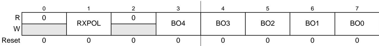
Figure 7-7. BDLC Analog Round Trip Delay Register (BDLC\_DLCBARD)
