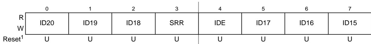
**Figure 25-23. Identifier Register 1 (IDR1)—Extended Identifier Mapping**
