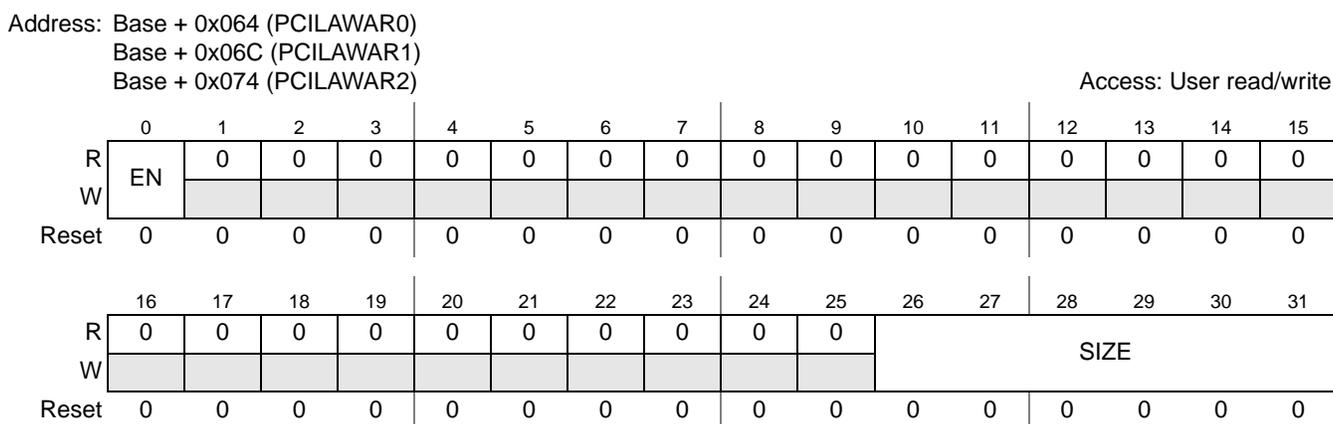
**Figure 2-5. PCI Local Access Window *n* Base Address Registers (PCILAWAR[0:2])**
