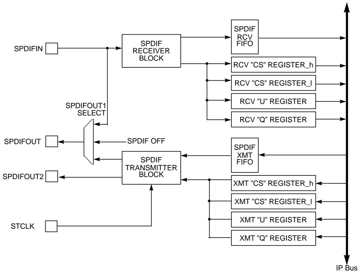
Figure 36-1. SPDIF Transceiver Data Interface Block Diagram
