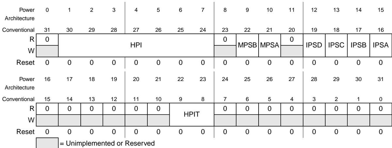
**Figure 20-2. System Global Interrupt Configuration Register (SICFR)
