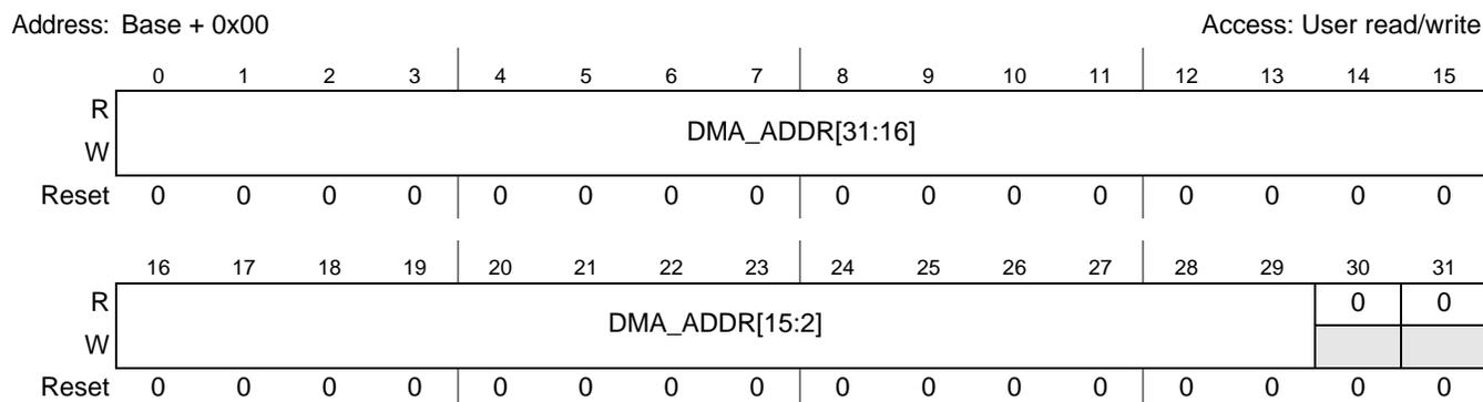
Figure 6-2. DMA Address Register (DMA\_ADDR)
