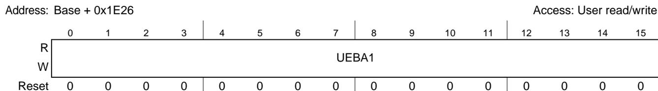
**Figure 26-16. End Block Address to Unlock in Write Protection Mode Register 1 (NFC\_UEBA1)**
