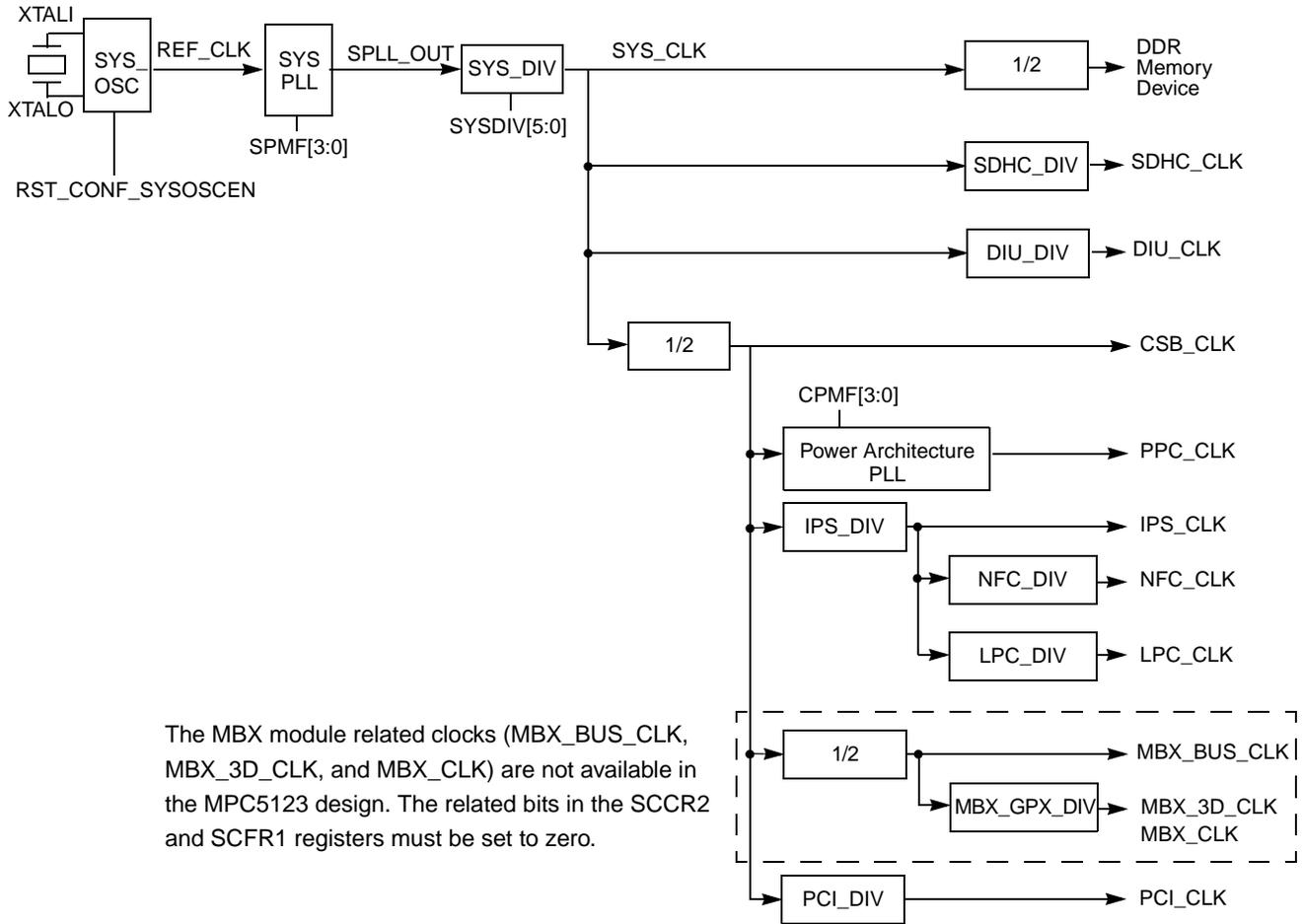
**Figure 5-1. MPC5121e Clock System**
