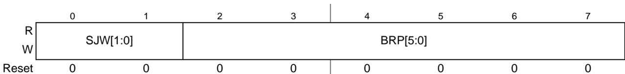
**Figure 25-5. MSCAN Bus Timing Register 0 (CANBTR0)**
