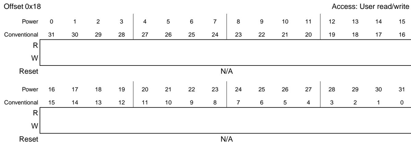
**Figure 5-15. Bread Crumb Register (BCR)**
