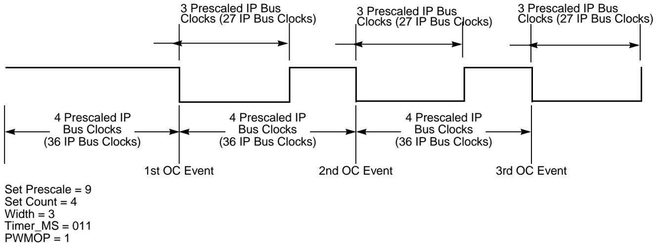
**Figure 17-9. PWM Example with OFF TIME = HIGH**
