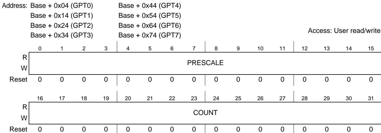
Figure 17-2. GPT0–GPT7 Input and Up/Down Counter Output (GPT<sub>n</sub>\_COUNTER) Registers
