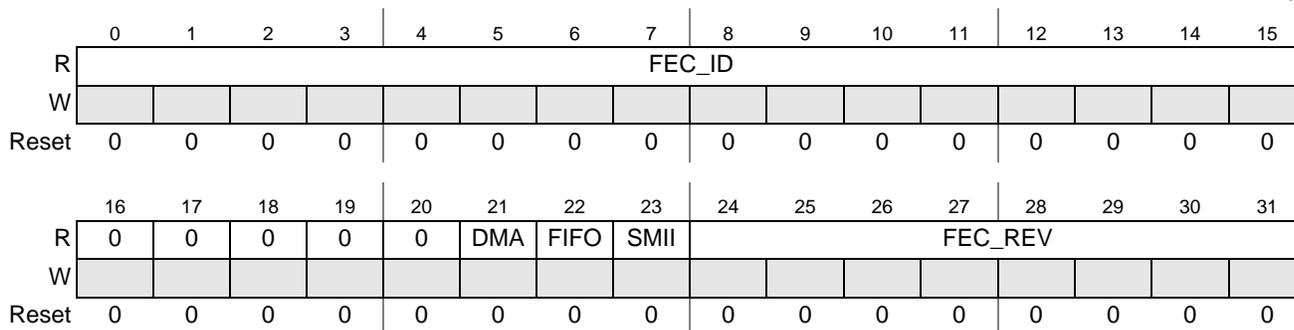
**Figure 16-3. FEC ID Register (ETH\_FEC\_ID)**
