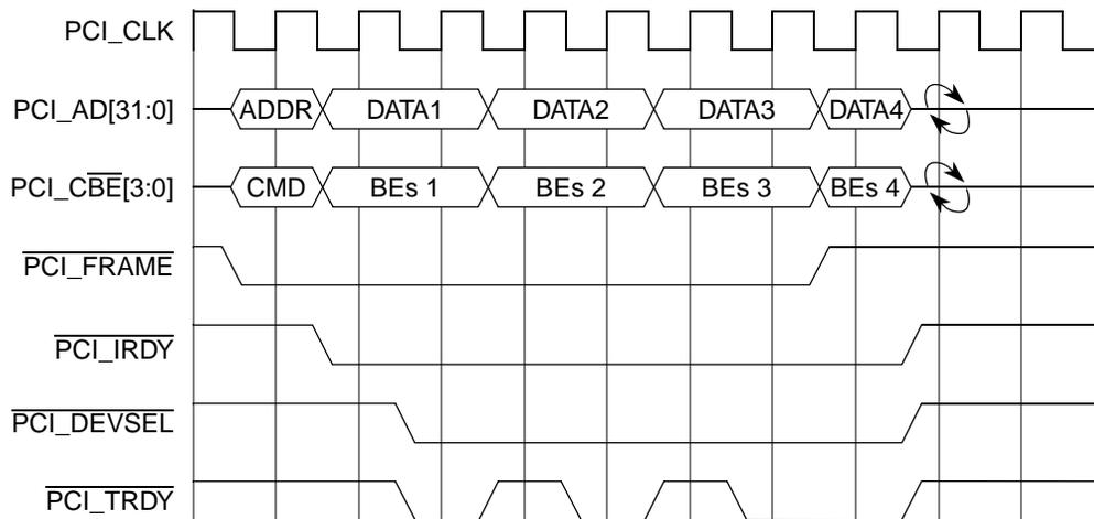
Figure 28-48. Burst Write Example
