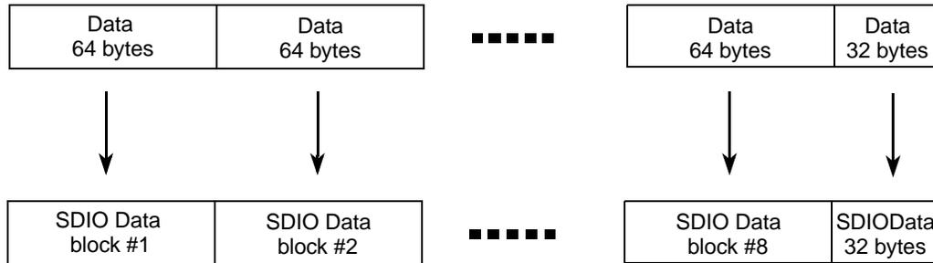
Eight 64-byte blocks are sent in block transfer mode and the remainder remove carriage return/line feed. The 32 bytes are sent in byte transfer mode.
