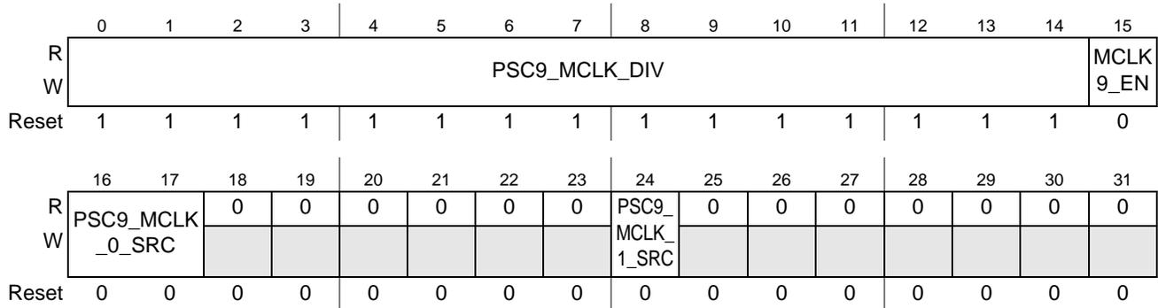
Figure 5-25. PSC9 Clock Control Register 9 (P9CCR)
