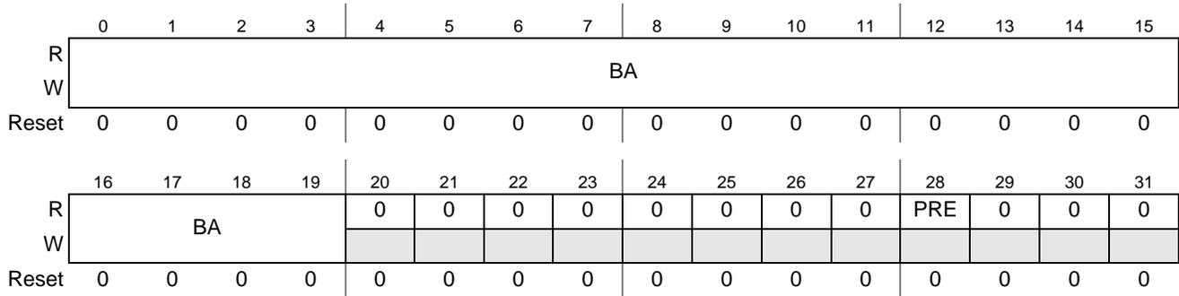
Figure 28-29. GPL Base Address Register 0 (PCI\_GPLBAR0CFG)
