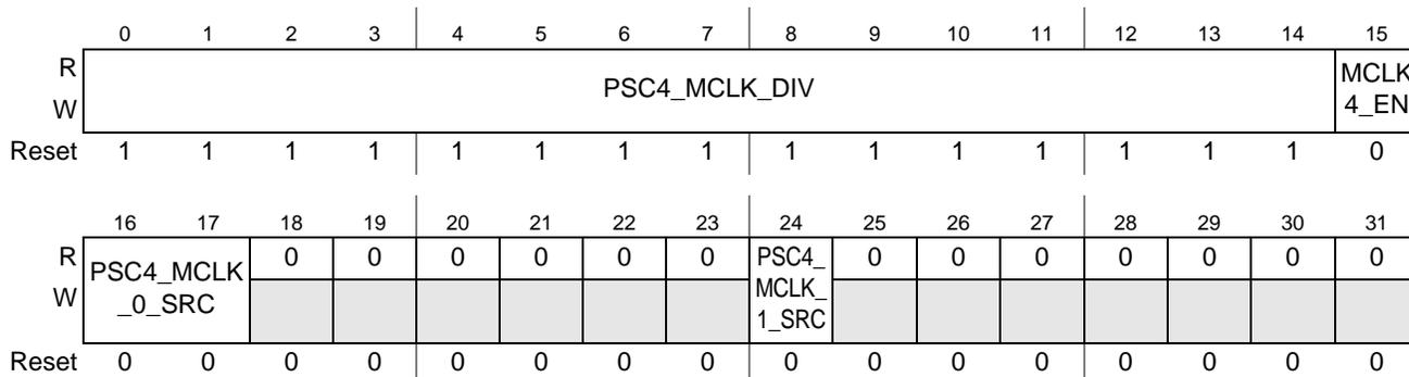
Figure 5-20. PSC4 Clock Control Register (P4CCR)
