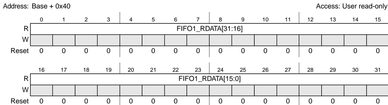
Figure 6-17. FIFO1 Read Data Register
