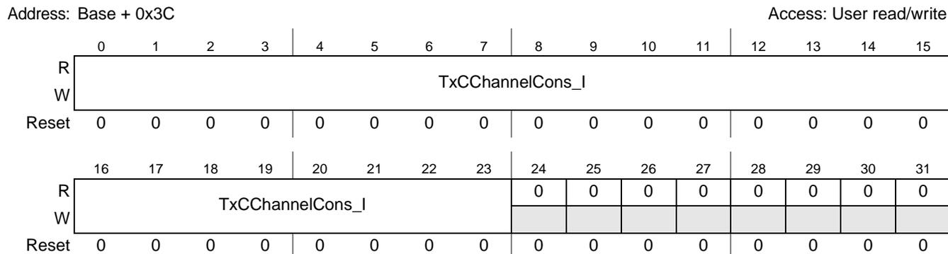
**Figure 36-19. SPDIF Transmit Consumer Channel Status Register Low (STCSL)**
