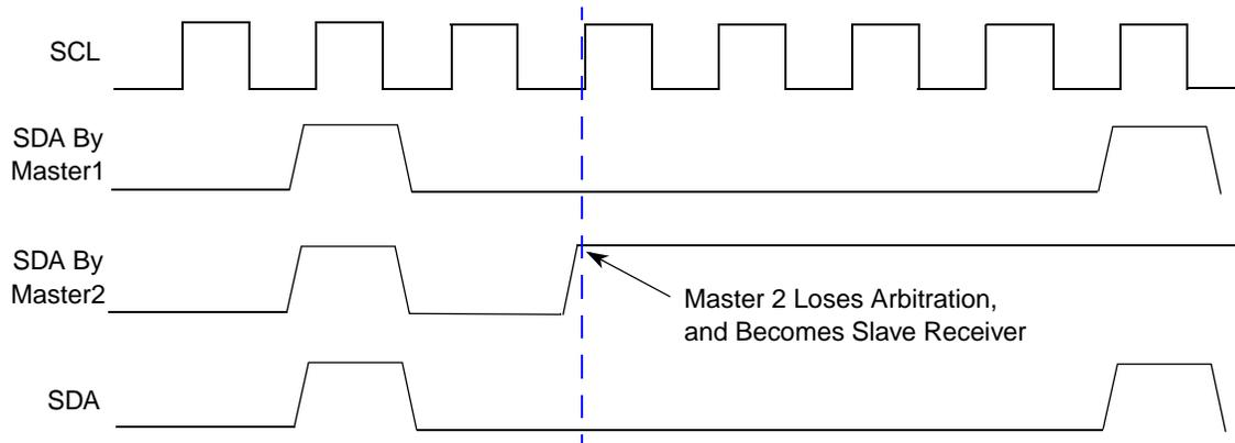
Figure 21-7. Timing Diagram – Arbitration Procedure
