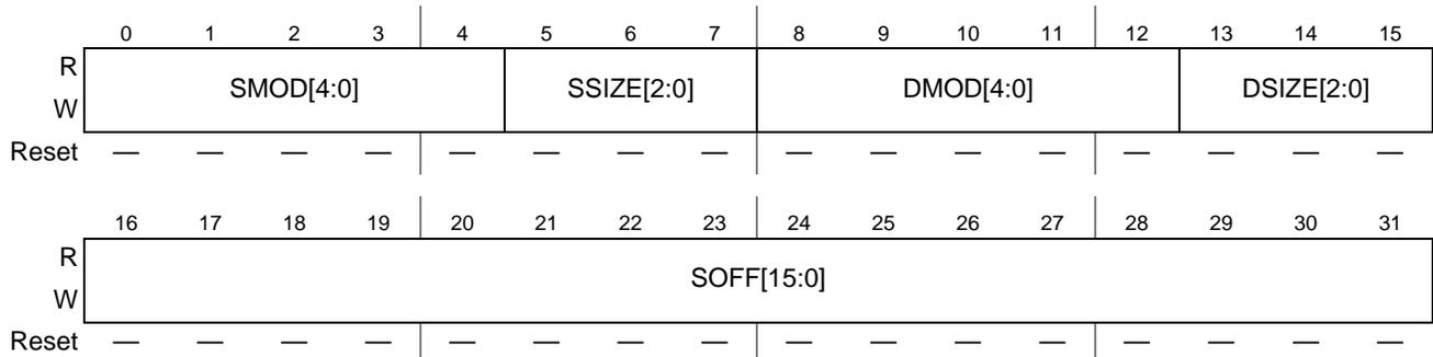
**Figure 11-25. TCDn Word 1 (TCDn.{SOFF,SMOD,SSIZE,DMOD,DSIZE}) Field**
