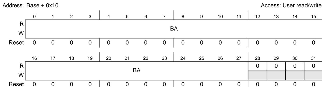
Figure 28-28. PIMMR Base Address Configuration (PCI\_PIMMRBACFG) Register
