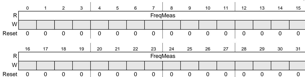
**Figure 8-3. Frequency Measurement Result Register (FMS)**
