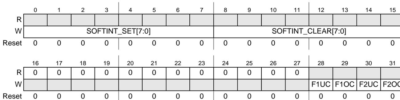
**Figure 6-23. Interrupt Clear/Set Register**
