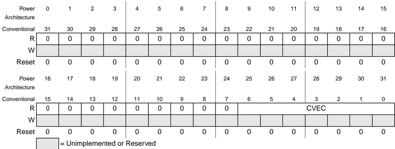
Figure 20-24. System Critical Interrupt Vector Register (SCVCR)
