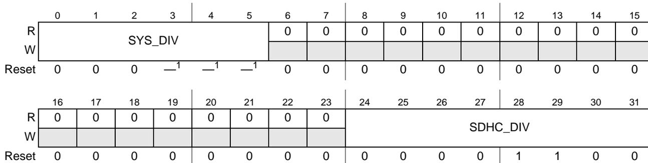
Figure 5-13. System Clock Frequency Register (SCFR2)
