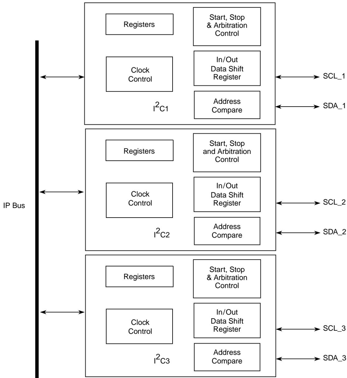
Figure 21-1. Block Diagram – I<sup>2</sup>C Module
