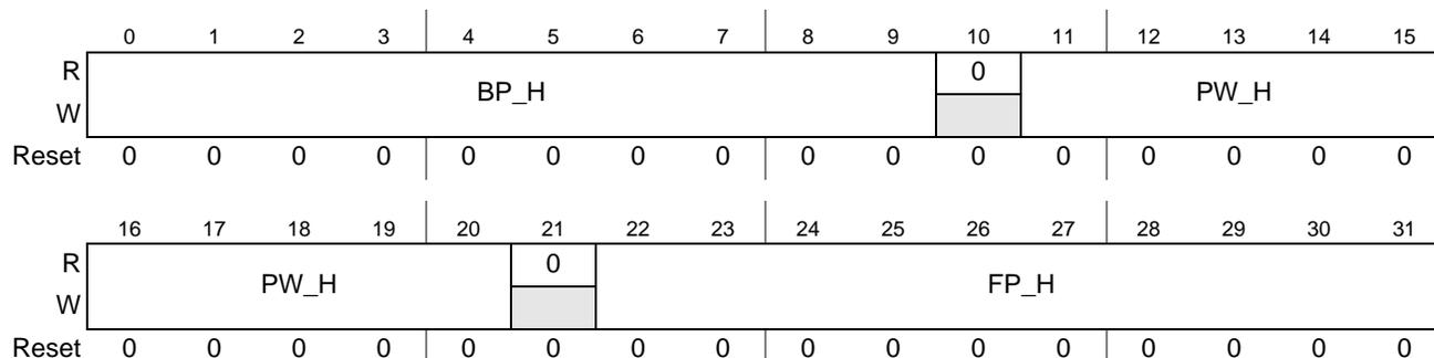
Figure 12-14. Horizontal Sync Pulse Parameters Register (HSYN\_PARA)
