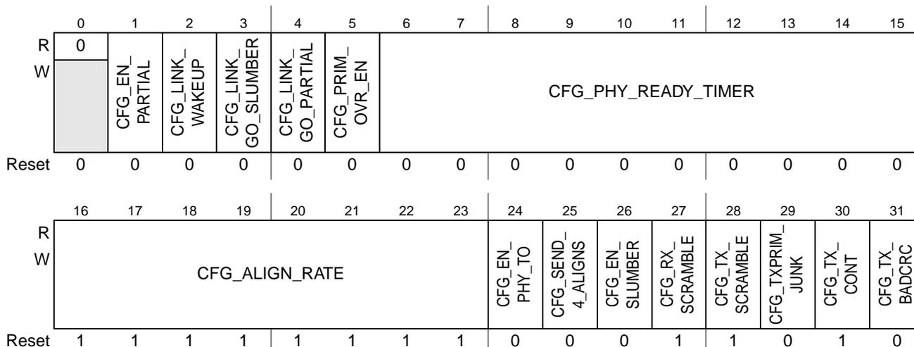
Figure 33-6. Link Layer Configuration Register 0 (LINK\_CFG0)
