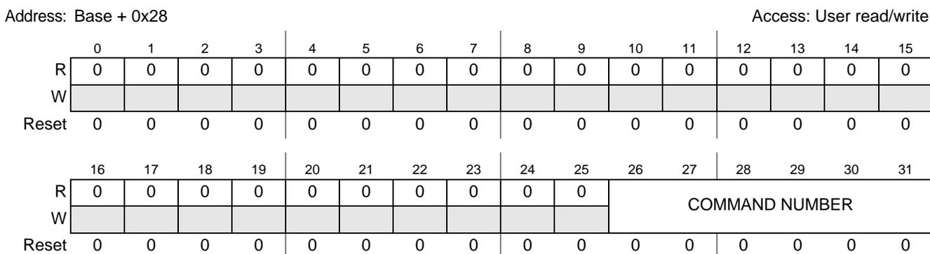
**Figure 34-12. SDHC Command Number (SDHC\_CMD) Register**
