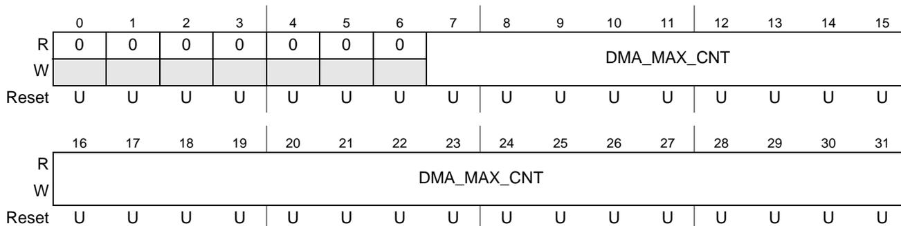
Figure 33-26. DMA Maximum Count Register (DMA\_MAX\_CNT)
