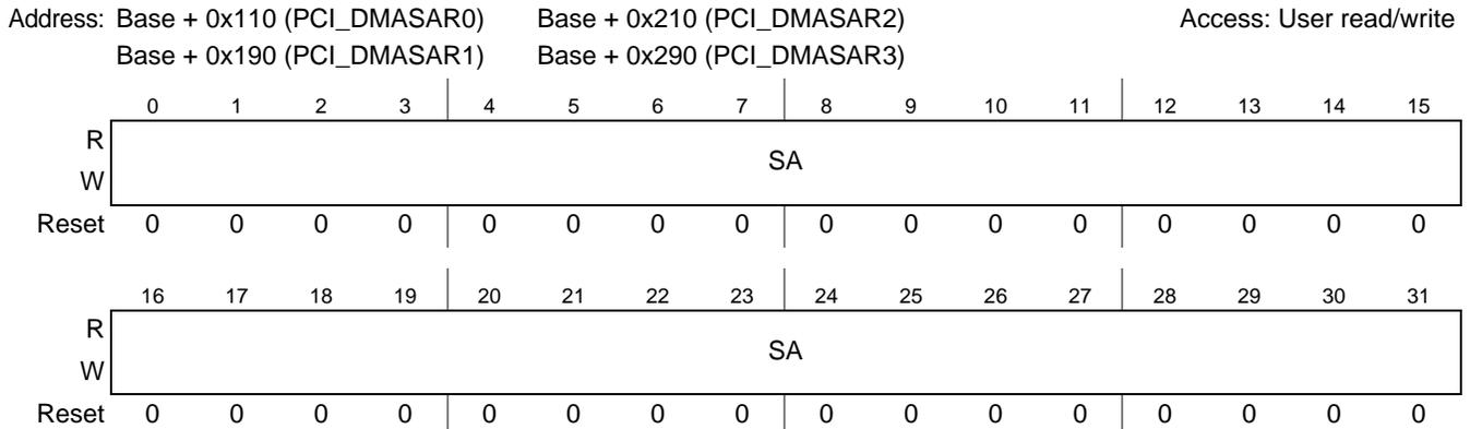
Figure 28-71. DMA Source Address Register (PCI\_DMASAR $n$ )
