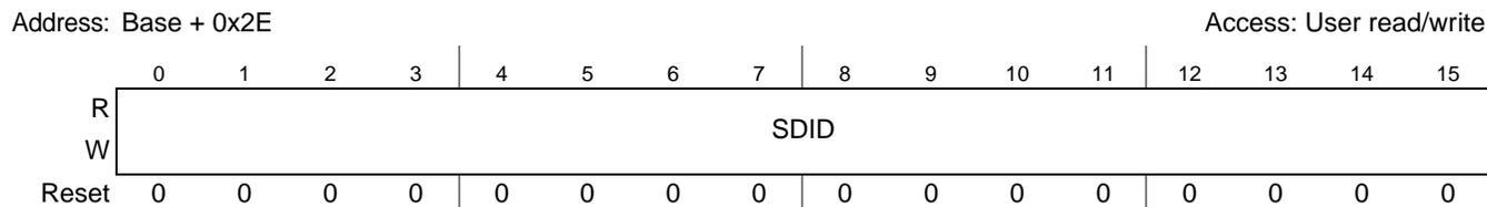
**Figure 28-32. Sub-System Device ID Configuration (PCI\_SUBSYSDEVICEIDCFG) Register**
