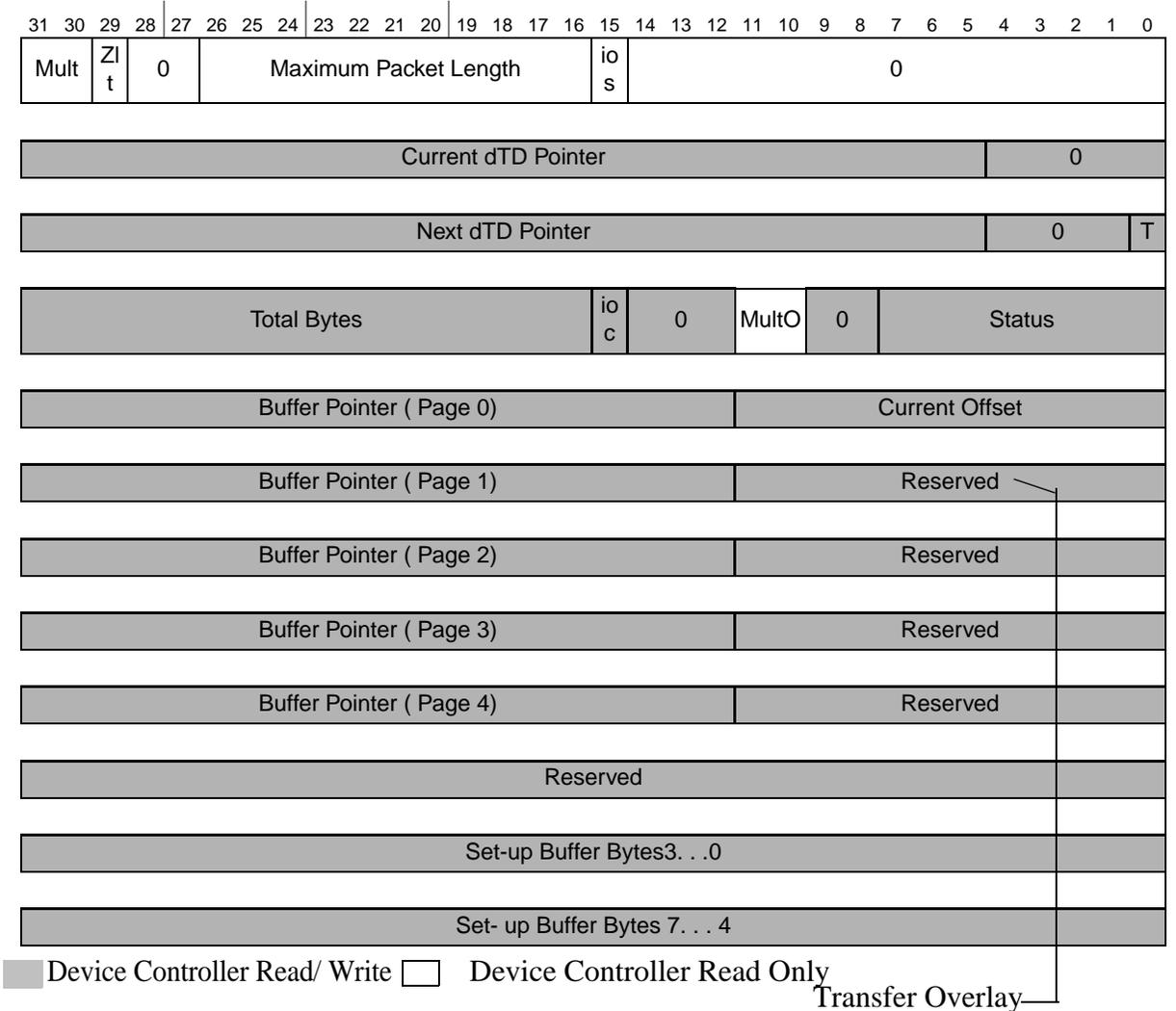
**Figure 39-74. Endpoint Queue Head**
