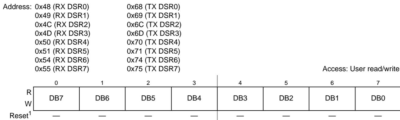
**Figure 25-28. Data Segment Registers (DSR0–DSR7)—Extended Identifier Mapping**
