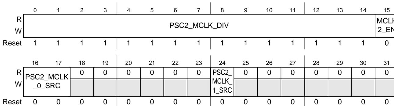
**Figure 5-18. PSC2 Clock Control Register (P2CCR)**
