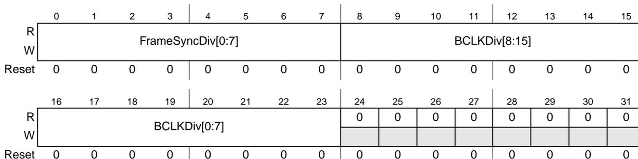
Figure 30-26. Codec Clock Register for Codec Mode (CCR)
