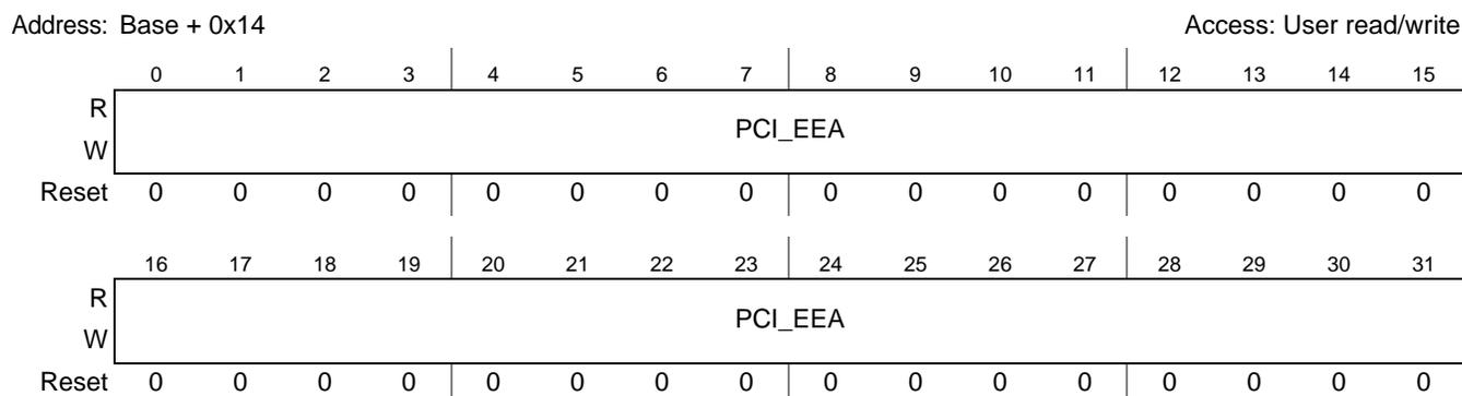
**Figure 28-7. PCI Error Extended Address Capture Register (PCI\_PCIEEACR)**
