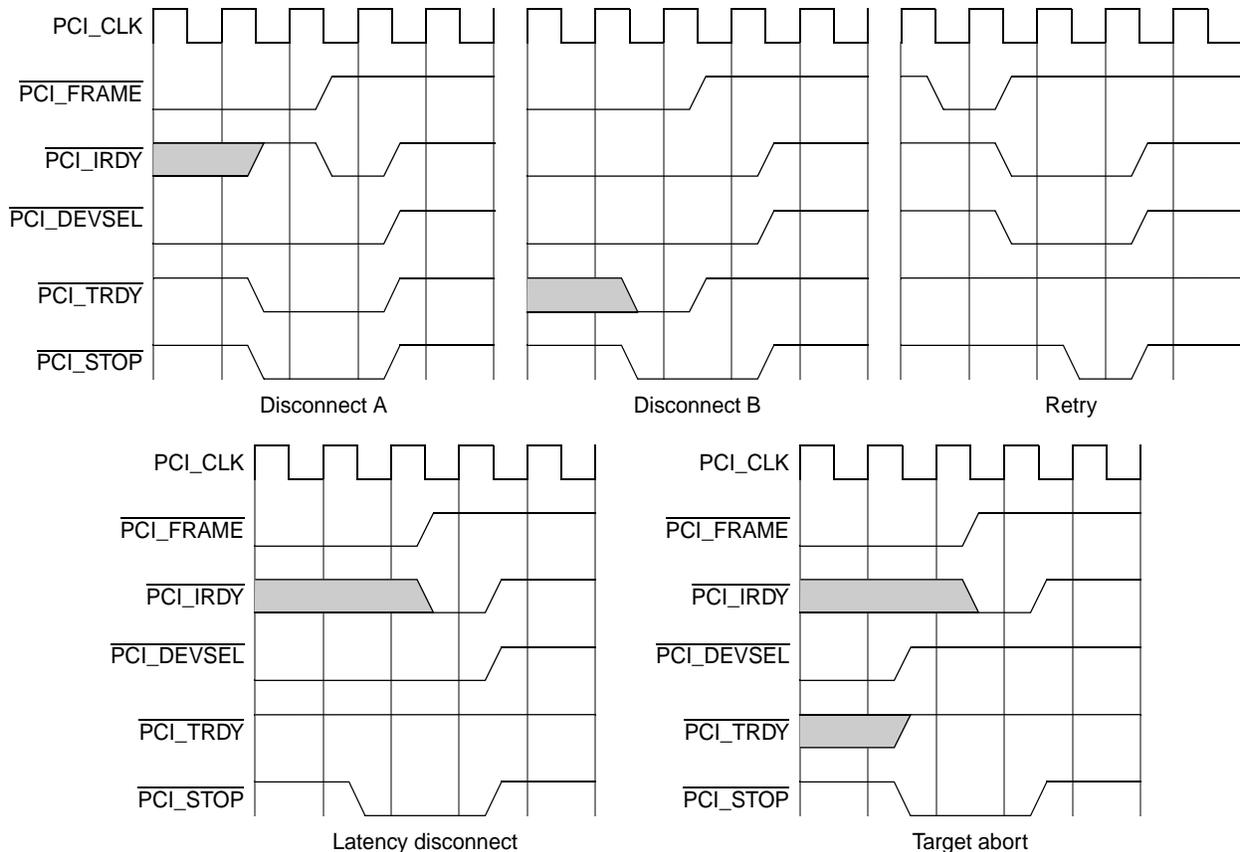
**Figure 28-49. Target-Initiated Terminations**
