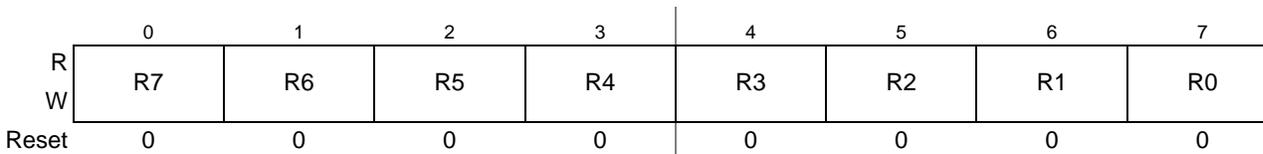
**Figure 7-8. BDLC Rate Select Register (BDLC\_DLCBRSR)**
