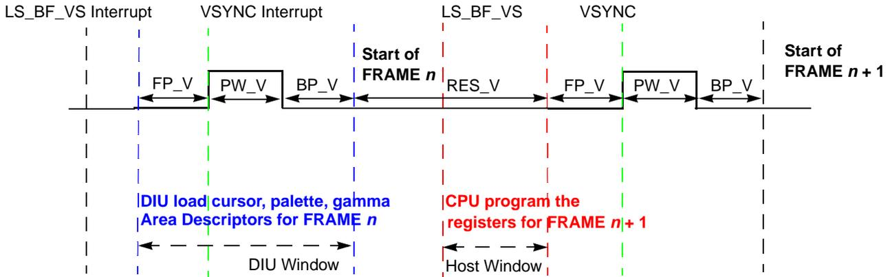
**Figure 12-50. Synchronizing the Host and the DIU**
