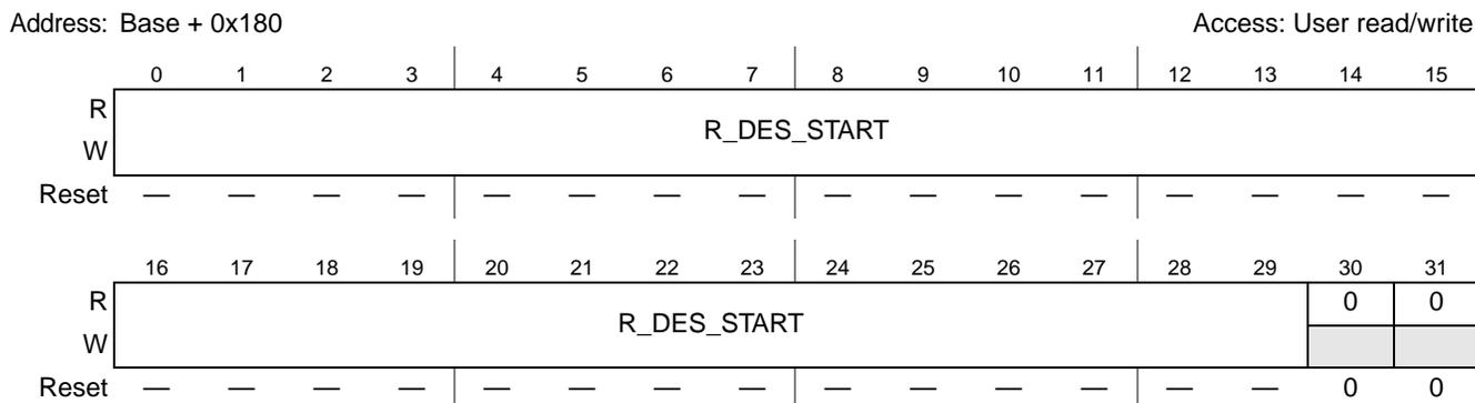
**Figure 16-25. Beginning of Receive Descriptor Ring (ETH\_R\_DES\_START) Register**
