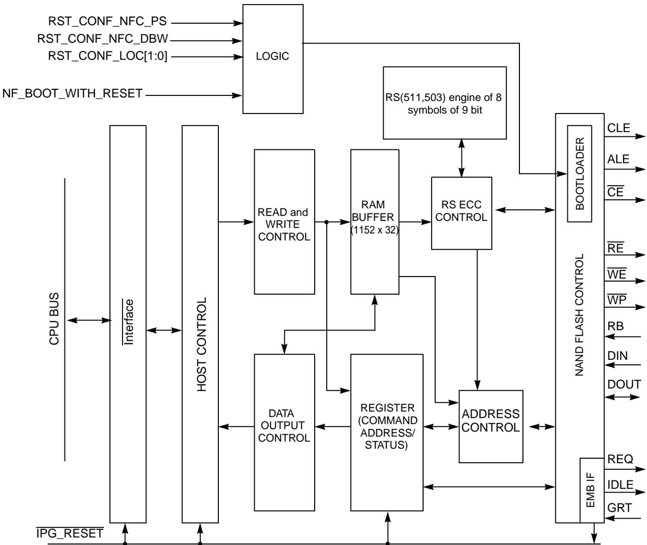
Figure 26-1. NAND Flash Controller Block Diagram
