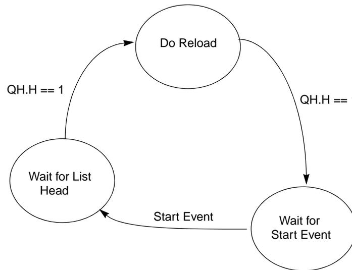
**Figure 39-62. Example HC State Machine for Controlling Nak Counter Reloads**
