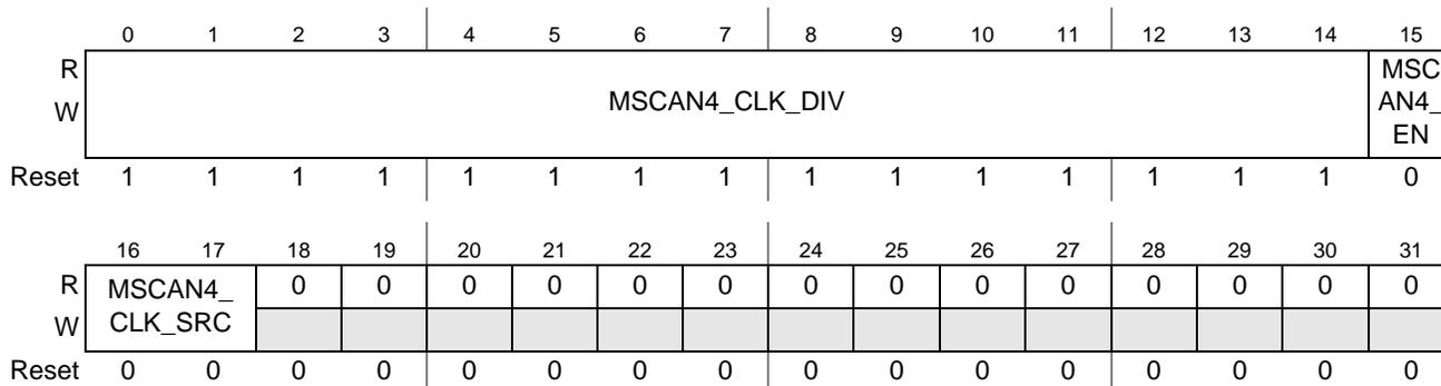
**Figure 5-34. MSCAN4 Clock Control Register (M2CCR)**
