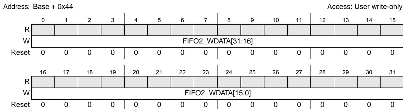
Figure 6-18. FIFO2 Write Data Register
