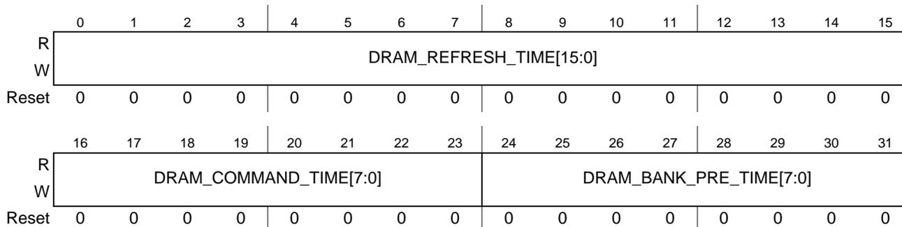
**Figure 13-4. DDR Time Configuration Register 0 (DDR\_TIME\_CONFIG0)**
