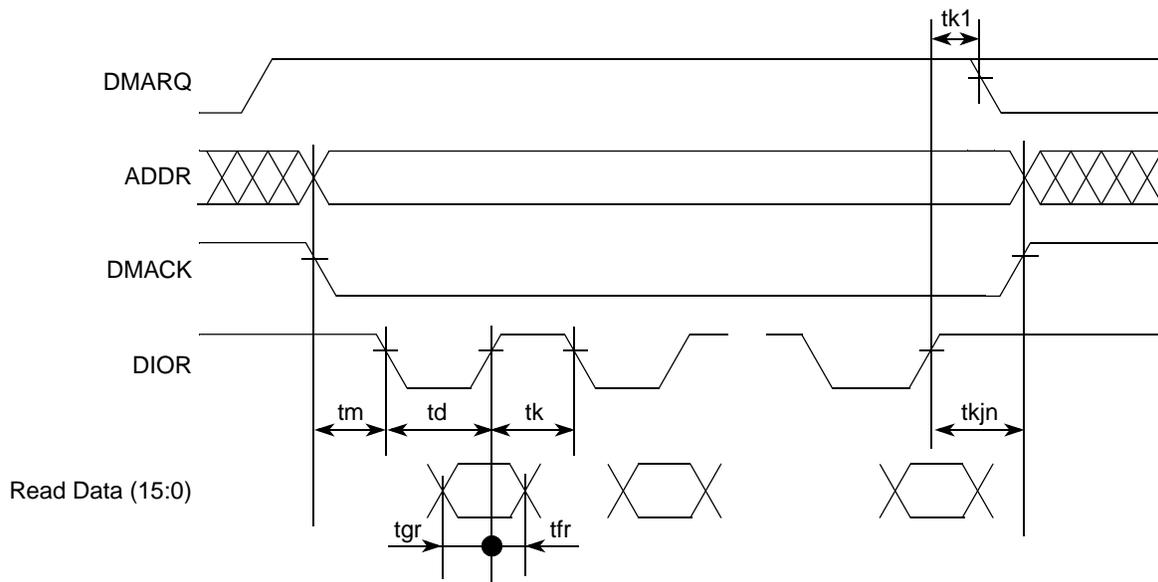
**Figure 27-18. MDMA Read Timing**
