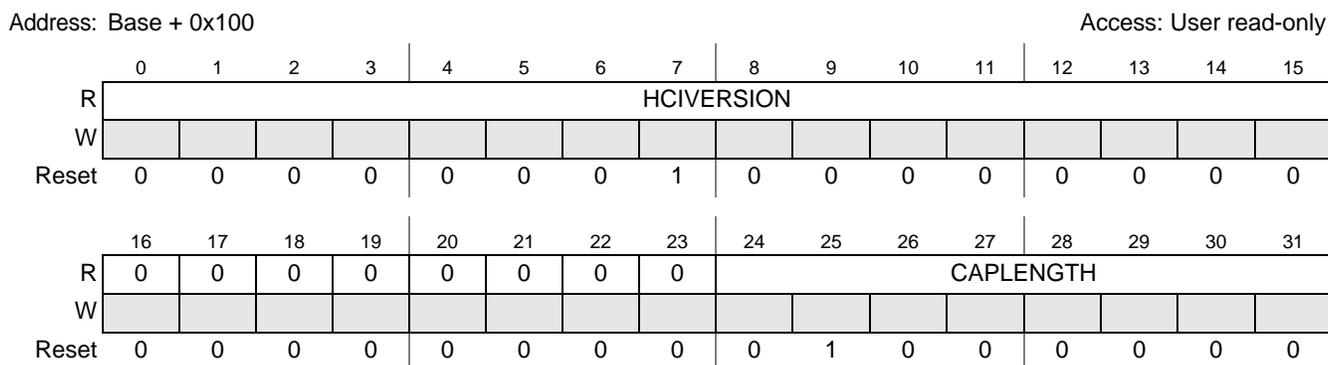
Figure 39-10. Capability Registers Length (USB\_CAPLENGTH)
