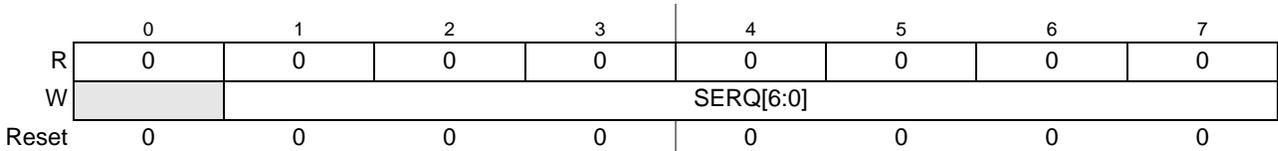
**Figure 11-7. DMA Set Enable Request Register (DMASERQ)**
