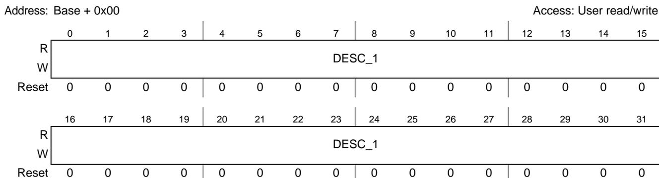
**Figure 12-1. Plane 1 Area Descriptor Pointer Register (DESC\_1)**
