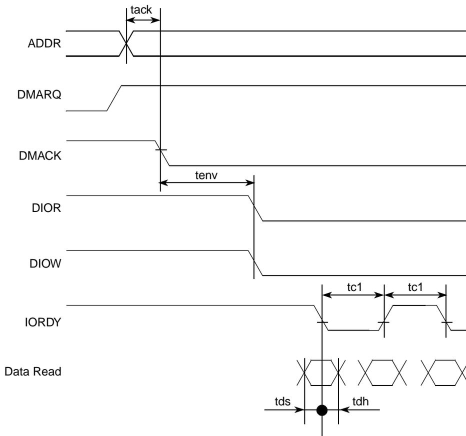
**Figure 27-20. UDMA In Transfer Start Timing Diagram**
