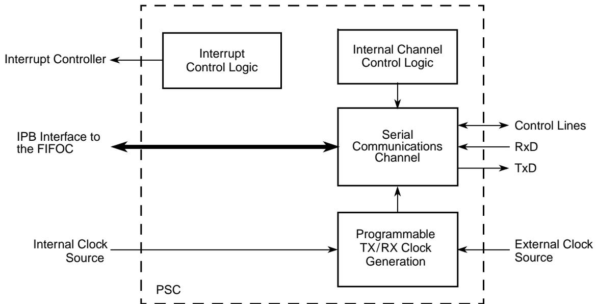
NOTE: In Codec mode, the number of available TxD and RxD lines depends on the configuration of the RX-TX channels fields of register MR2.
