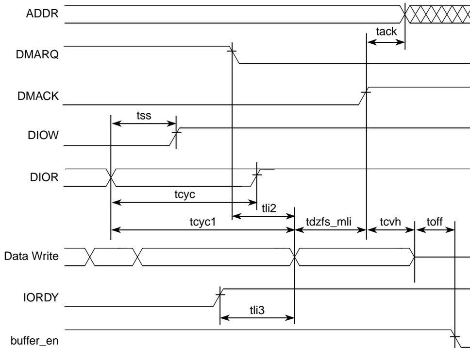
Figure 27-24. UDMA Out Host Terminates Transfer
