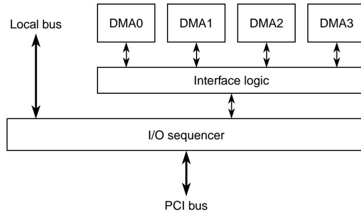
**Figure 28-76. DMA Controller Block Diagram**
