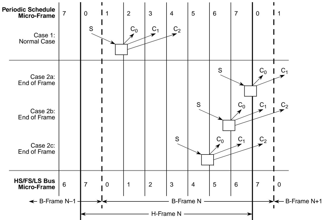
**Figure 39-66. Split Transaction and Interrupt Scheduling Boundary Conditions**
