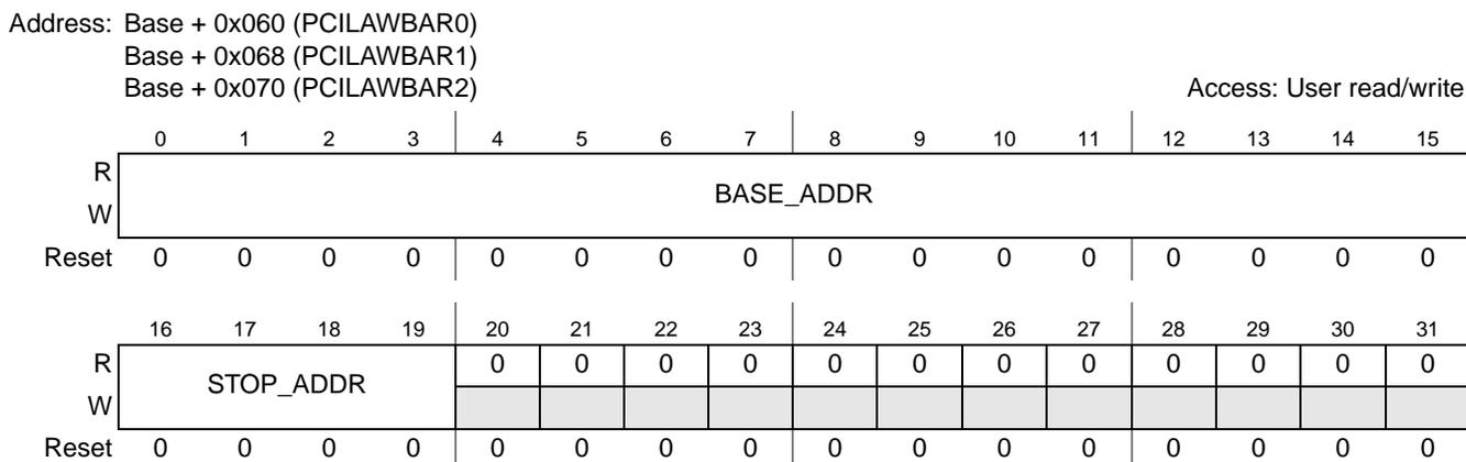
**Figure 2-4. PCI Local Access Window *n* Base Address Registers (PCILAWBAR[0:2])**
