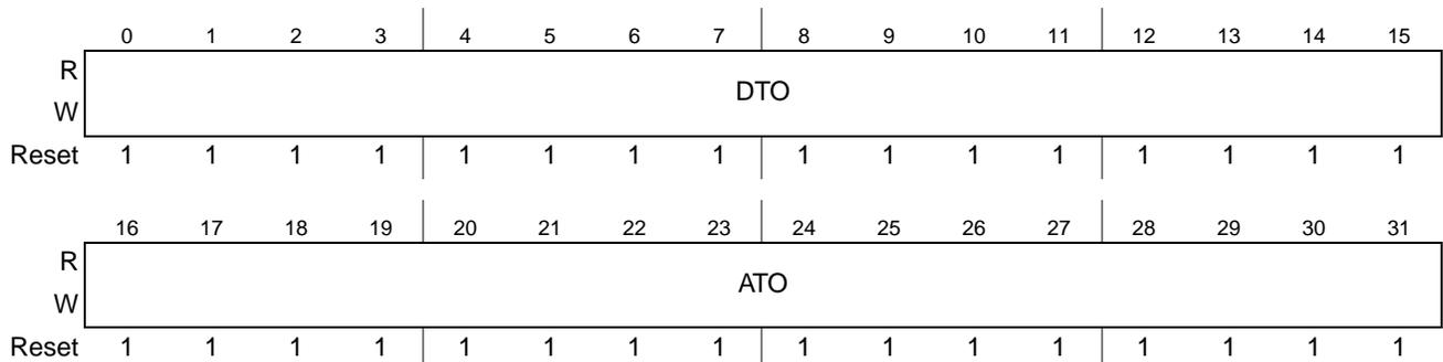
**Figure 10-2. Arbiter Timers Register (ATR)**
