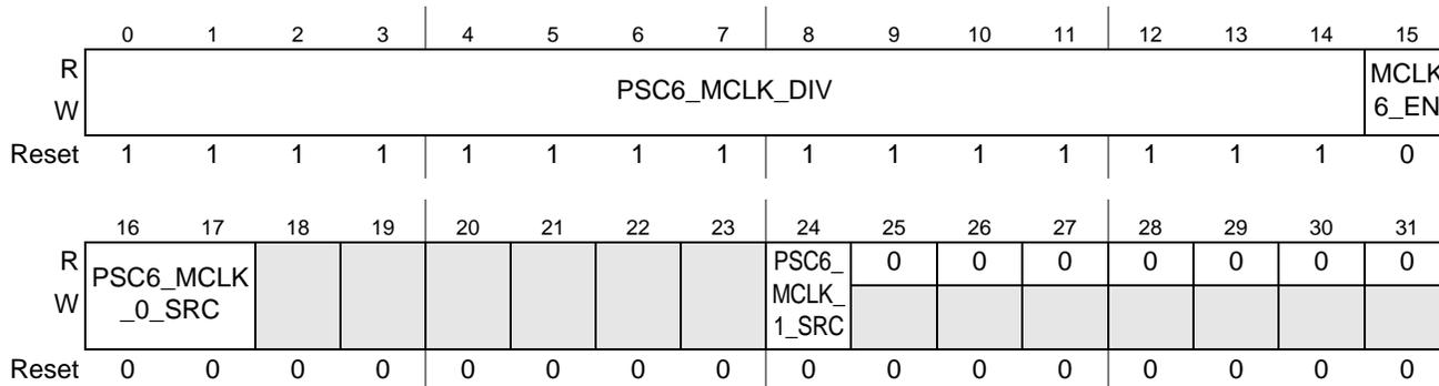
Figure 5-22. PSC6 Clock Control Register (P6CCR)
