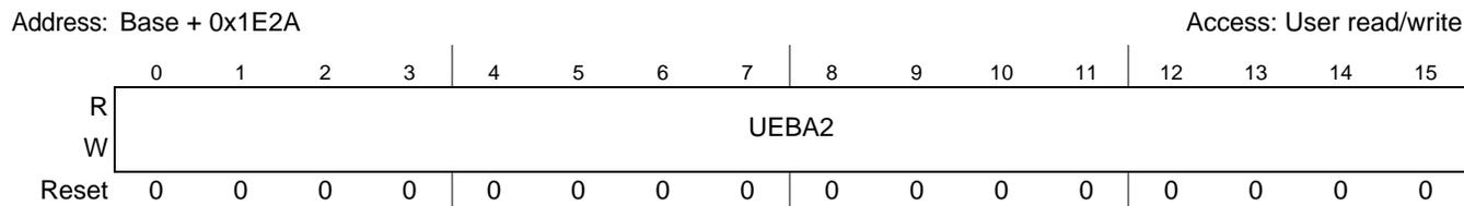
**Figure 26-18. End Block Address to Unlock in Write Protection Mode Register 2 (NFC\_UEBA2)**
