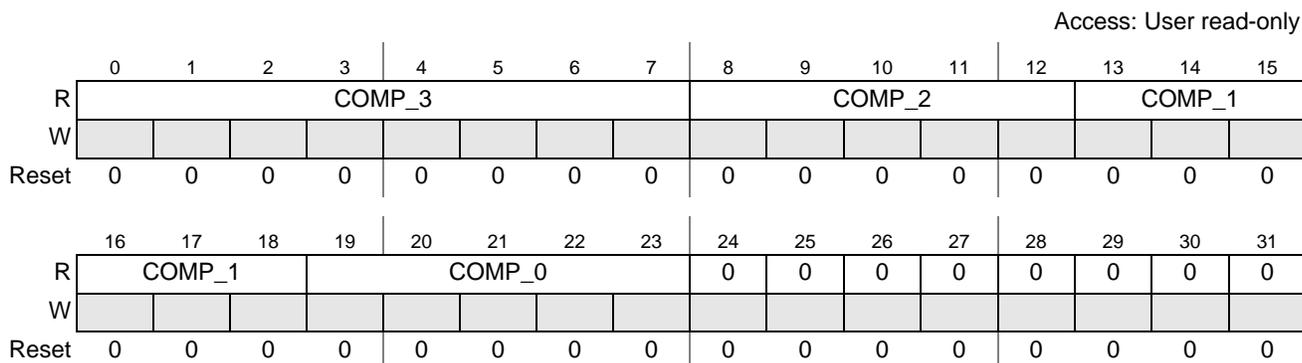
**Figure 12-42. Example of 24-bit ARGB 8:5:6:5 Pixel Structure Definition when BYTE\_F = 1**
