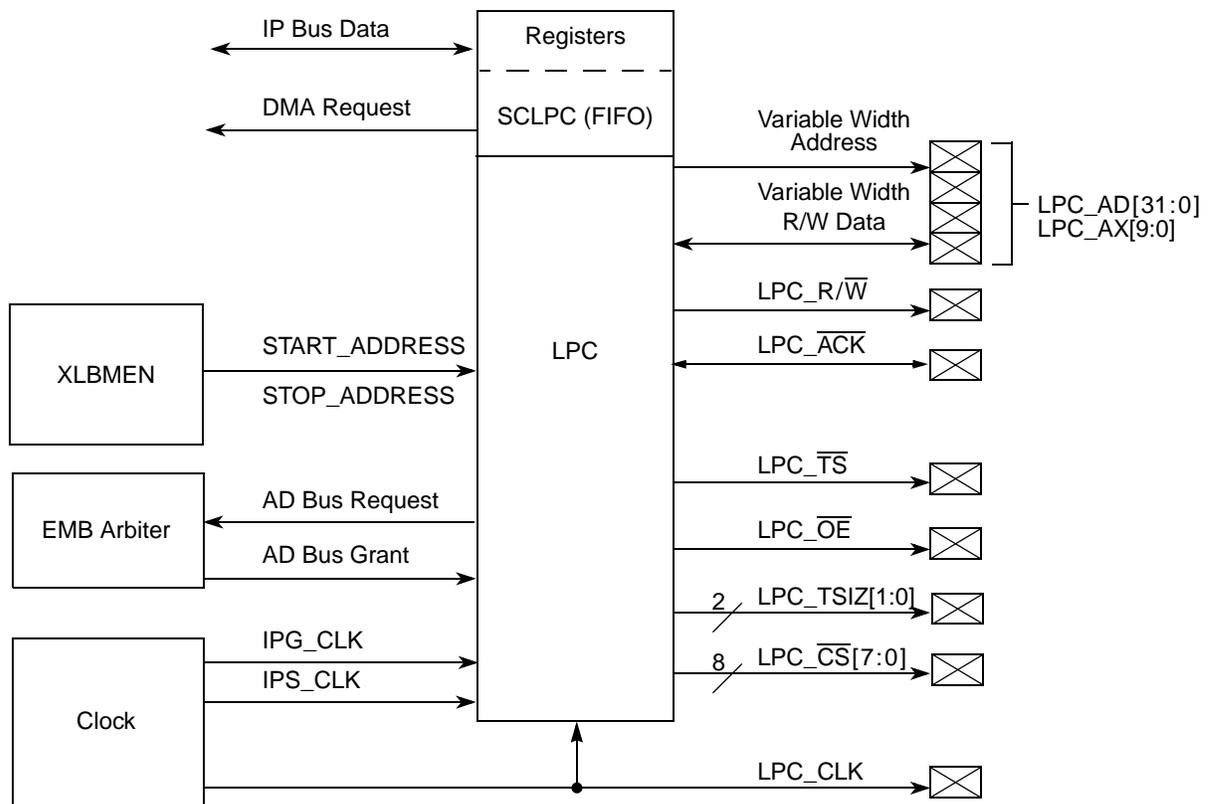
Figure 23-1. LPC Block Diagram
