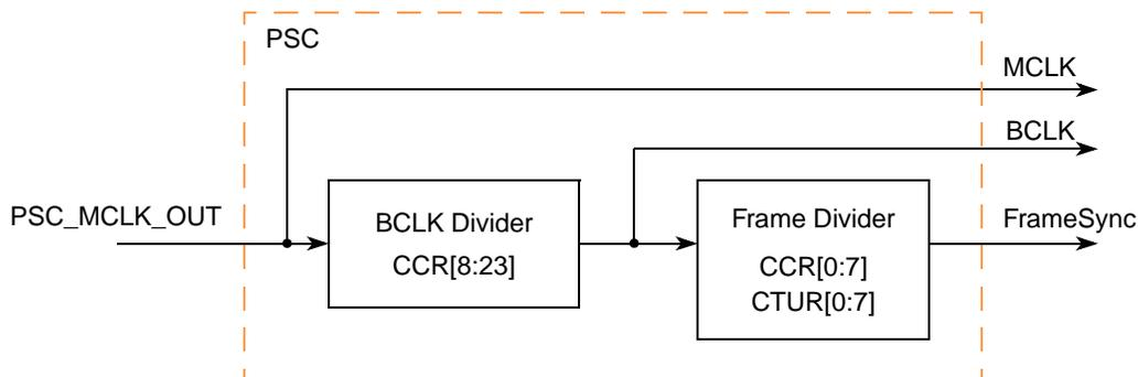
**Figure 30-45. Clock Generation Diagram for Codec Mode**
