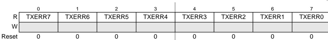
**Figure 25-17. MSCAN Transmit Error Counter Register (CANTXERR)**
