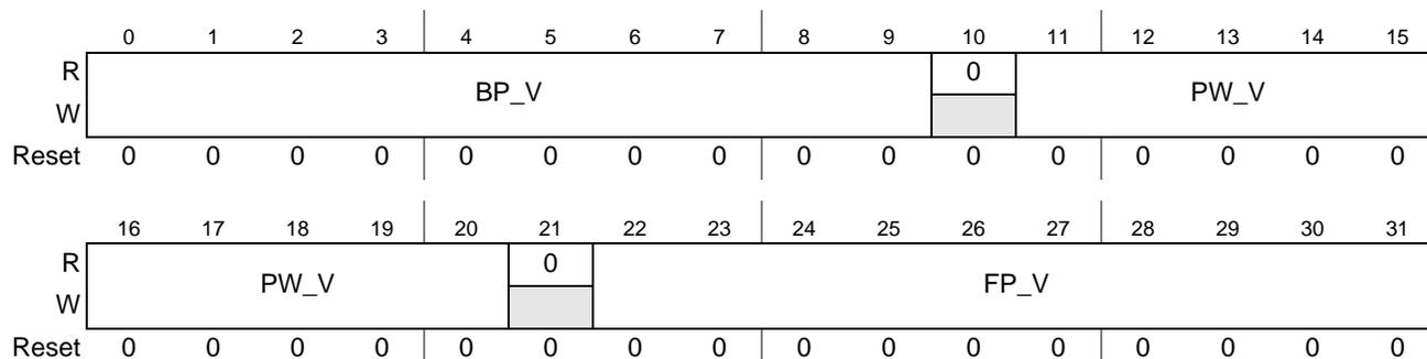
Figure 12-15. Vertical Sync Pulse Parameters Register (VSYN\_PARA)
