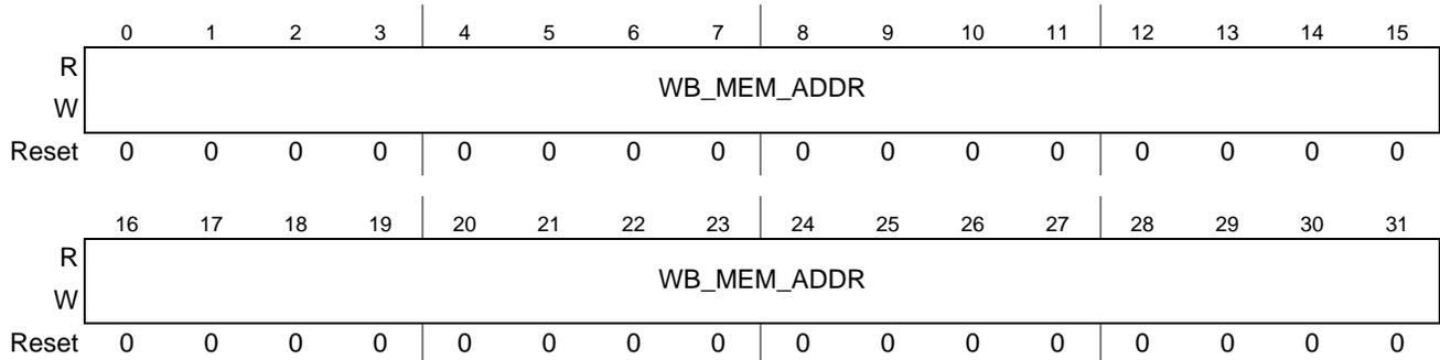
Figure 12-13. Writeback Plane Address Register (WB\_MEM\_ADDR)
