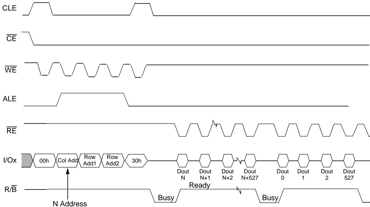
Figure 26-23. Read Operation B (With Command 30H)
