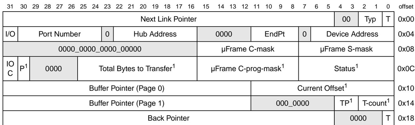
**Figure 39-49. Split-Transaction Isochronous Transaction Descriptor (siTD)**
