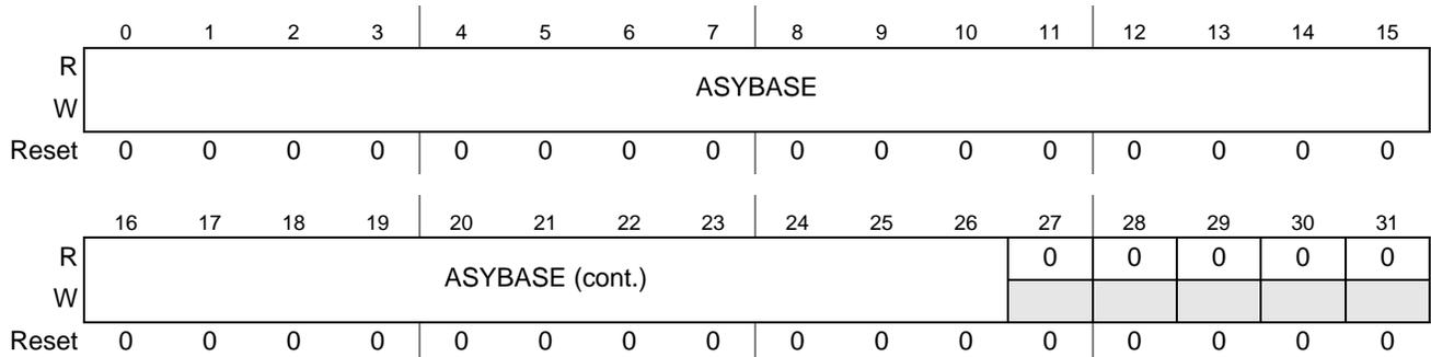
**Figure 39-23. Current Asynchronous List Address Register (USB\_ASYNCLISTADDR)**
