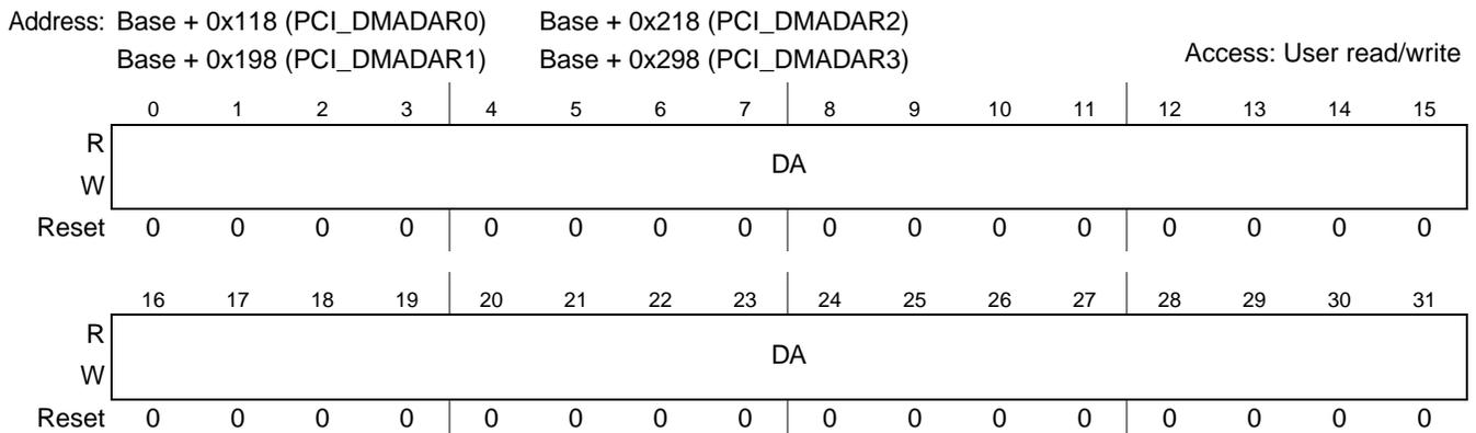
Figure 28-72. DMA Destination Address Register (PCI\_DMADAR $n$ )
