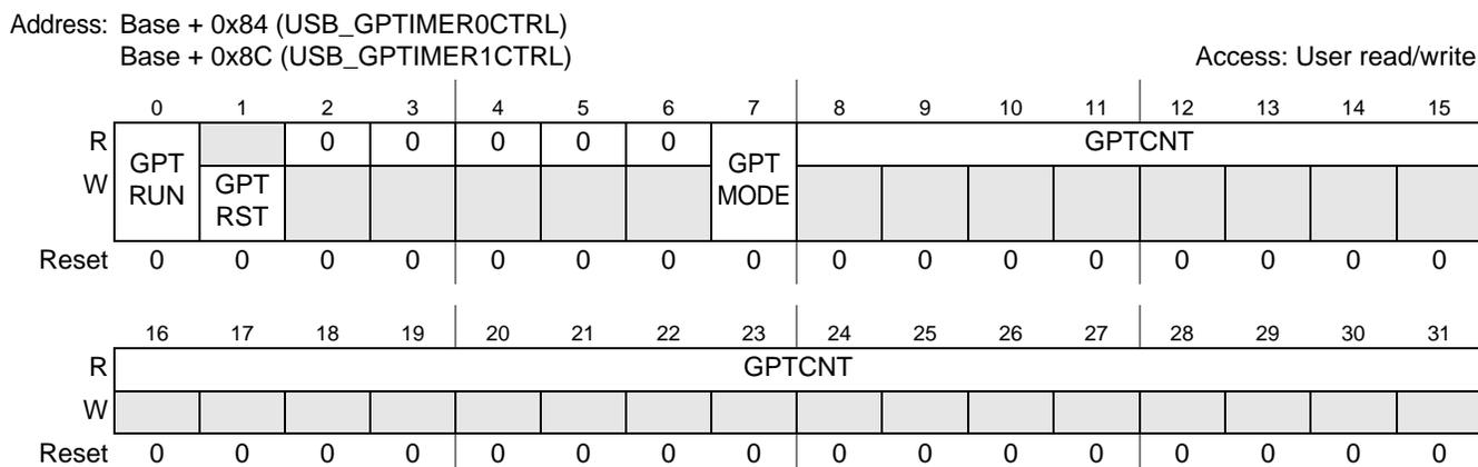
Figure 39-16. General Purpose Timer Control Register USB\_GPTIMERxCTRL)
