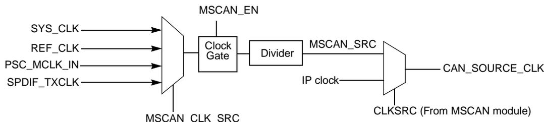
**Figure 5-5. MSCAN Source Clock Generation<sup>1</sup>**
