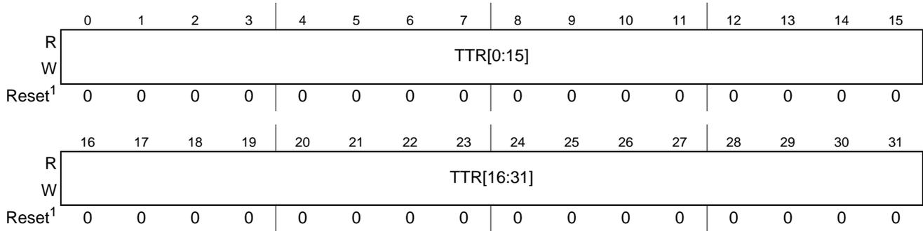
**Figure 32-10. RTC Target Time Register (RTC\_TTR)**
