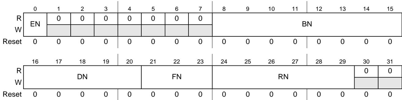
Figure 28-41. Configuration Address (PCI\_CONFIG\_ADDR) Register
