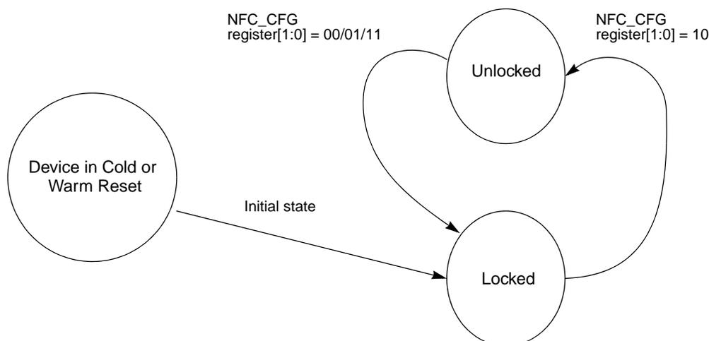
Figure 26-49. State Diagram of RAMbuffer Write Protection
