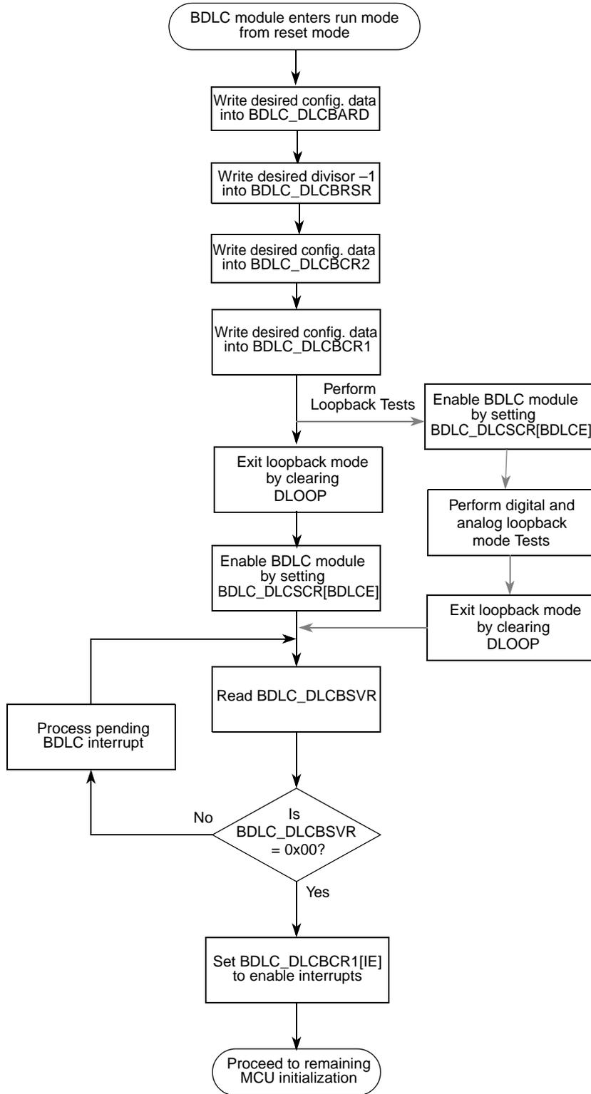
**Figure 7-27. Basic BDLC Module initialization Flowchart**
