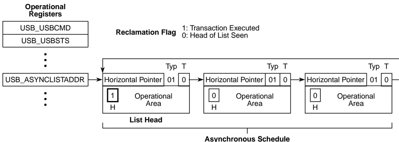
Figure 39-60. Asynchronous Schedule List with Annotation to Mark Head of List
