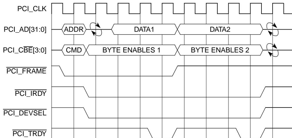
Figure 28-46. Burst Read Example
