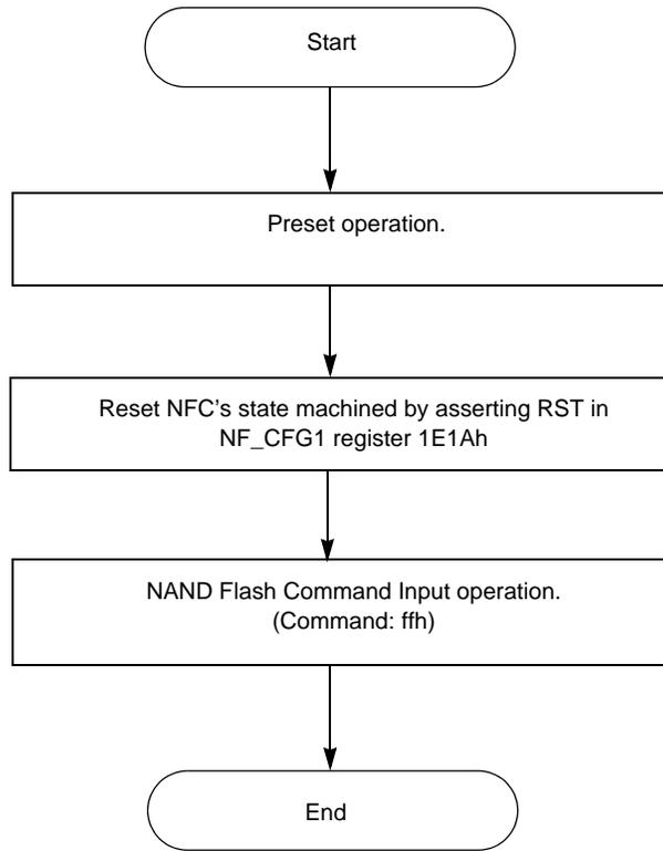
Figure 26-44. Flow Chart of Hot Reset Operation
