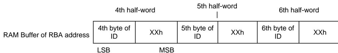
**Figure 26-39. x16 Assignment of NAND Flash ID Data**
