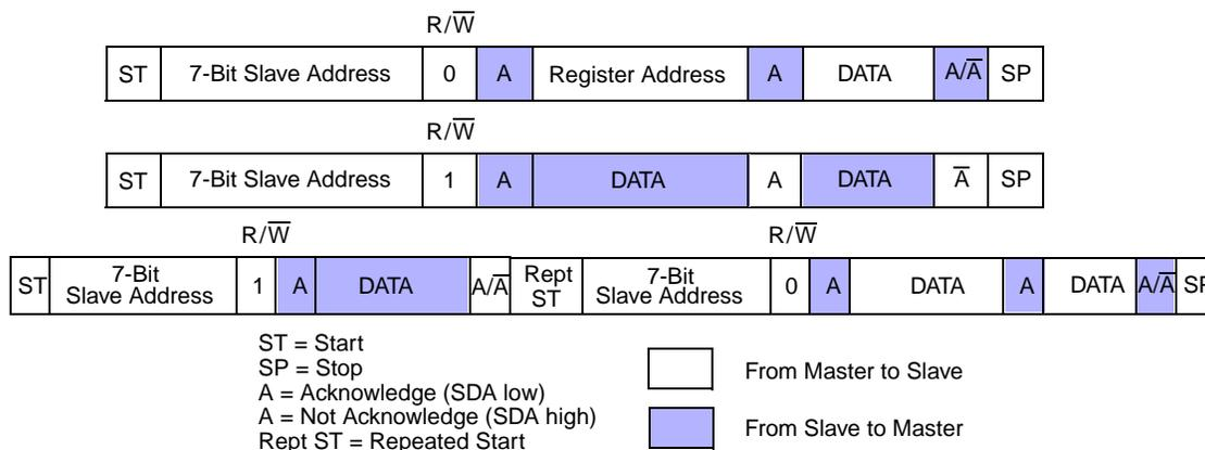
**Figure 21-5. Data Transfer, Combined Format**
