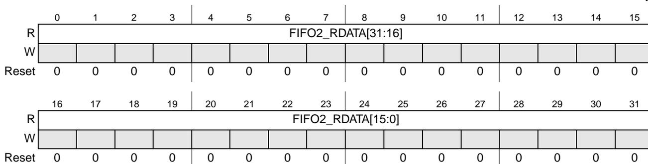
**Figure 6-19. FIFO2 Read Data Register**
