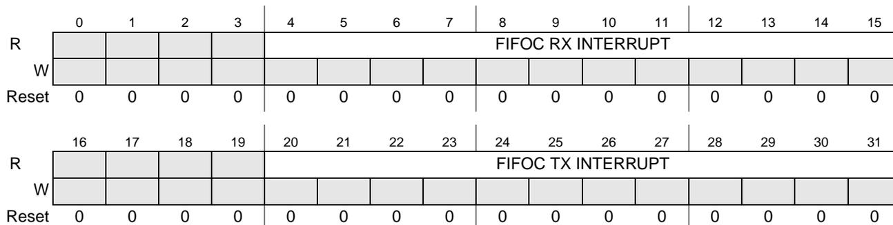
**Figure 31-12. FIFOC Interrupt Register (FIFOC\_INT)**
