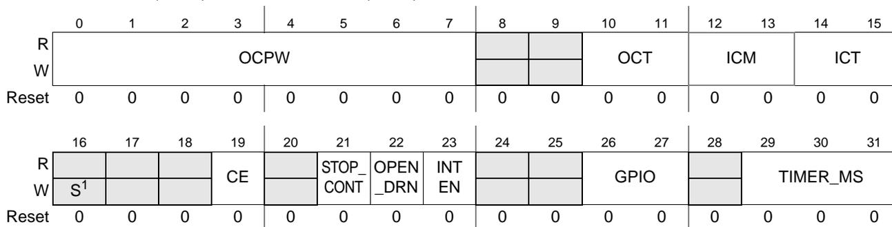
**Figure 17-1. GPT0–GPT7 Enable and Mode Select (GPT<sub>n</sub>\_MODE) Registers**
