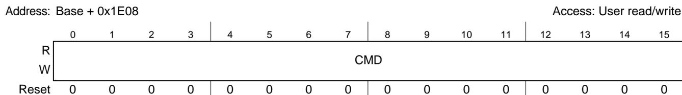
Figure 26-4. NAND Flash Command Register (FLASH\_CMD)
