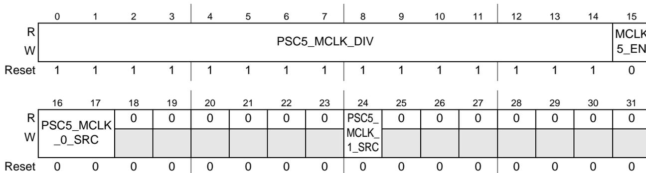
Figure 5-21. PSC5 Clock Control Register (P5CCR)
