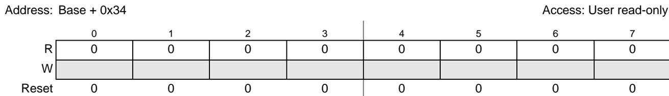
**Figure 28-33. Capabilities Pointer Configuration (PCI\_CAPABILITYPTR) Register**
