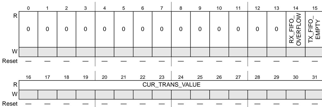
Figure 33-12. Transport Layer Status Register 1 (TRANS\_STATUS1)
