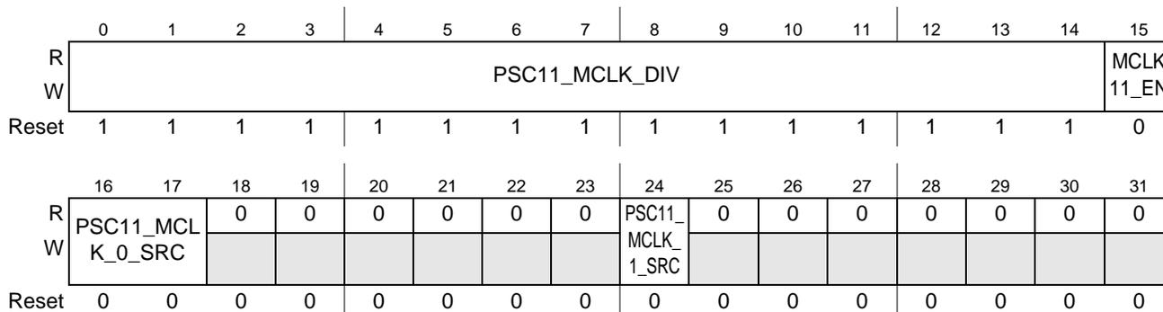
Figure 5-27. PSC11 Clock Control Register 11 (P11CCR)
