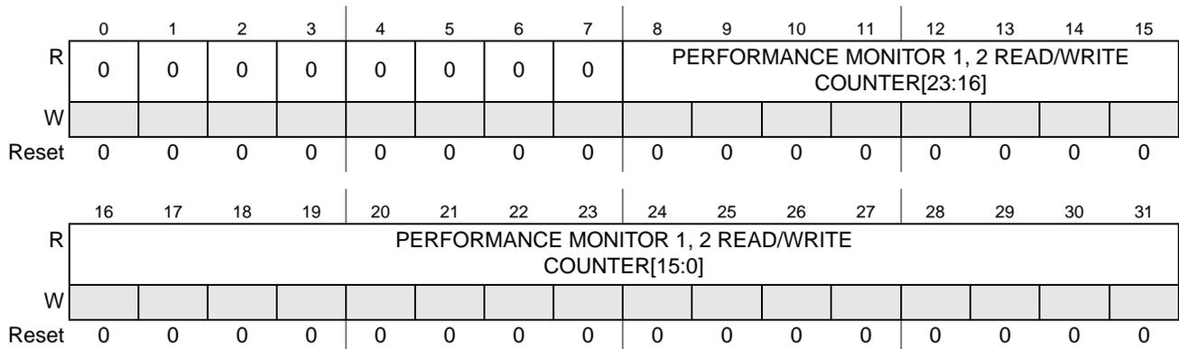
Figure 14-13. Performance Monitor Counter Registers
