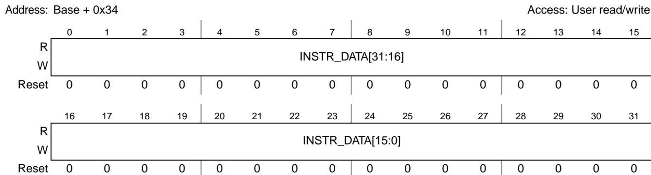
Figure 6-15. Instruction SRAM Data Register
