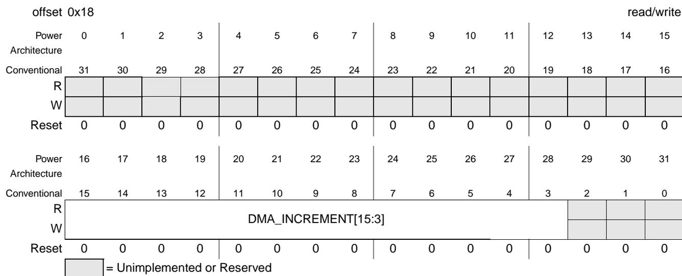
**Figure 40-8. DMA\_INCREMENT Register**
