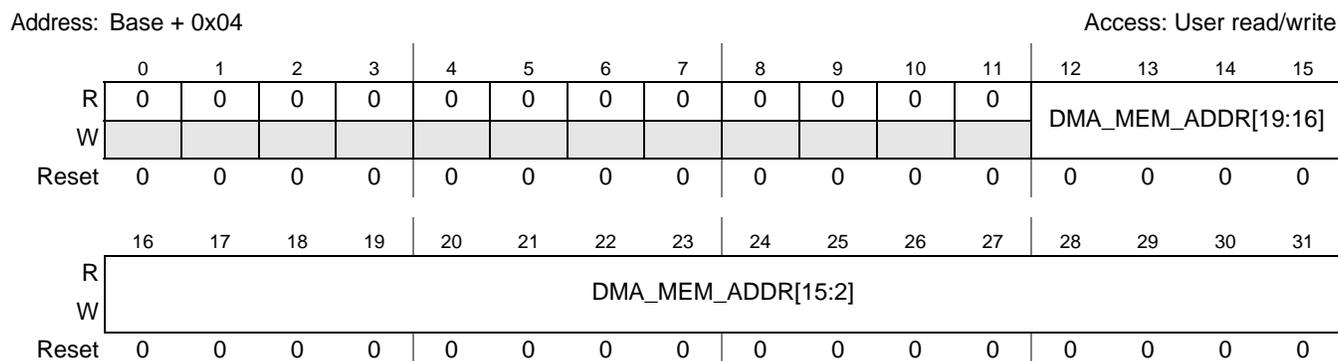
Figure 6-3. DMA Memory Address Register (DMA\_MEM\_ADDR)
