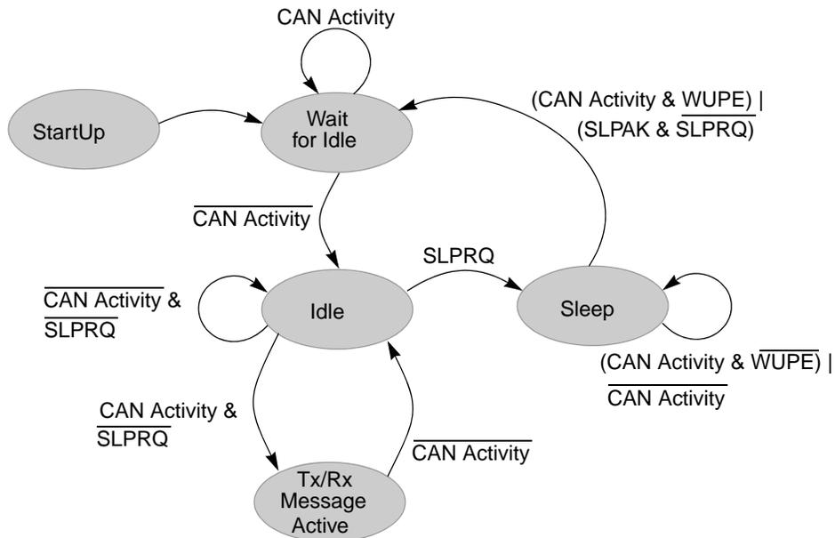
**Figure 25-40. Simplified State Transitions for Entering/Leaving Sleep Mode**
