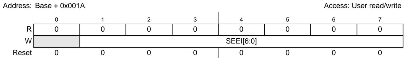
**Figure 11-9. DMA Set Enable Error Interrupt Register (DMASEEI)**
