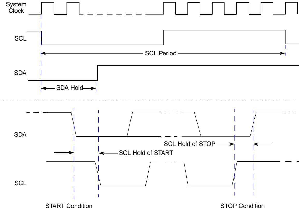
**Figure 21-10. Timing Diagram of I<sup>2</sup>C Signal Relationships**
