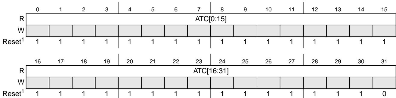
**Figure 32-11. RTC Actual Time Counter (RTC\_ATC) register**
