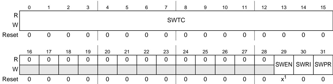
**Figure 35-1. Software Watchdog Control Register (WDT\_SWCRR)**
