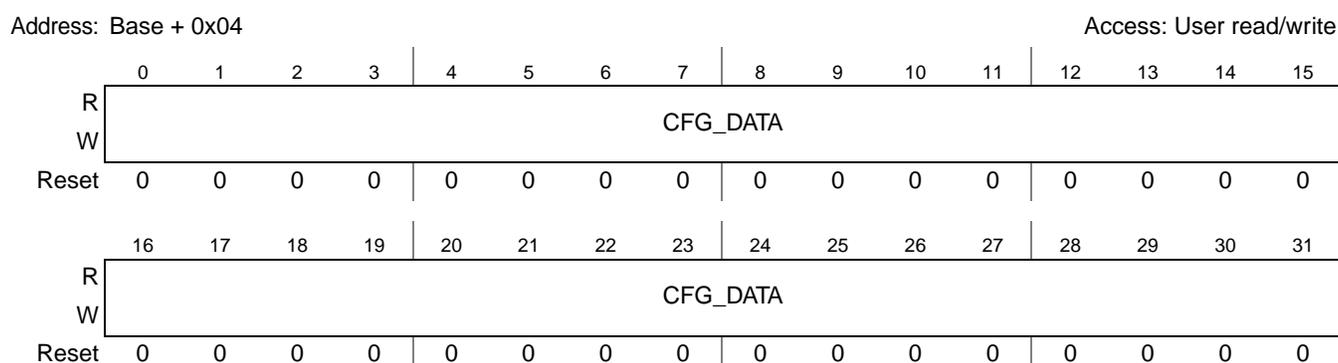
**Figure 28-42. Configuration Data (PCI\_CONFIG\_DATA) Register**
