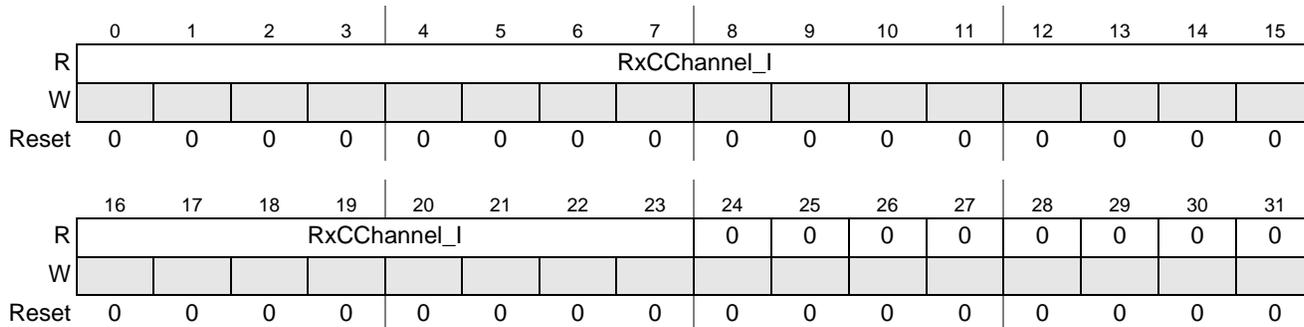
Figure 36-12. SPDIF Receive C Channel Register Low (SRCSL)
