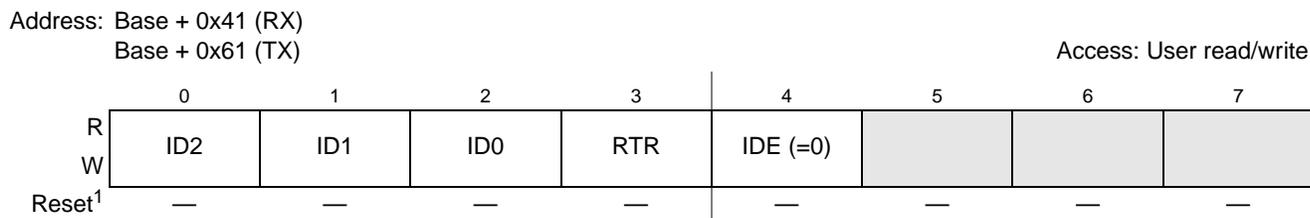
**Figure 25-27. Identifier Register 1 (IDR1)—Standard Mapping**
