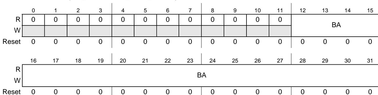
**Figure 28-54. PCI Outbound Base Address Register  $x$  (PCI\_OUTBOUND\_BASE\_ADDR $x$ )**
