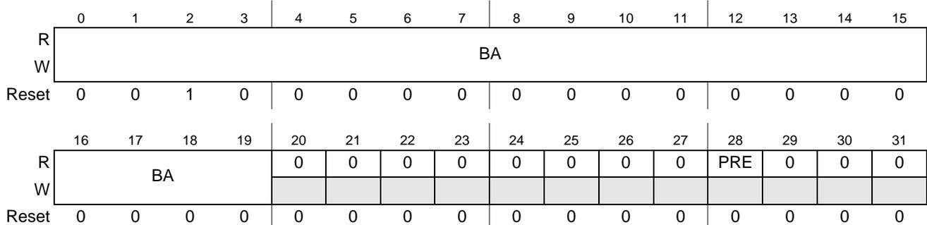
Figure 28-30. GPL Base Address Registers *n* (PCI\_GPLBAR<sub>*n*</sub>)
