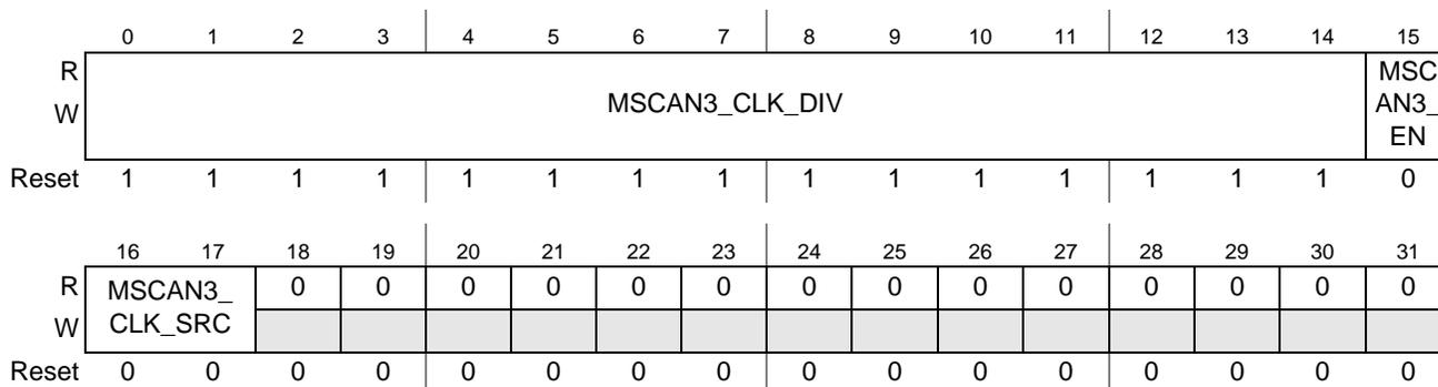
**Figure 5-33. MSCAN3 Clock Control Register (M2CCR)**
