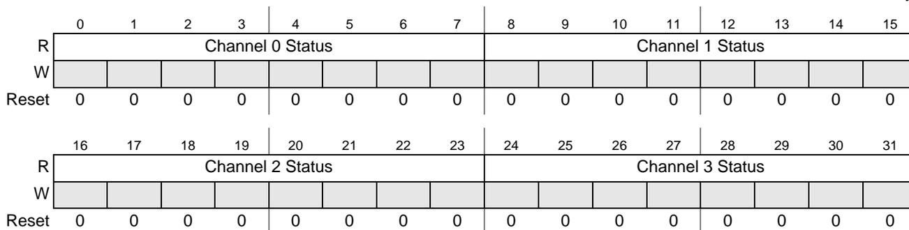
**Figure 28-75. DMA General Status Register (PCI\_DMAGSR)**
