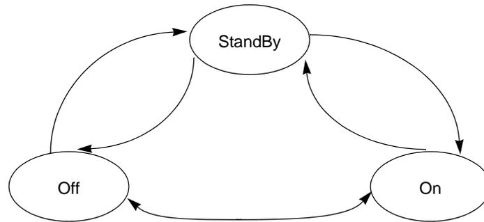
Figure 36-22. FIFO Auto-Resync Controller State Machine
