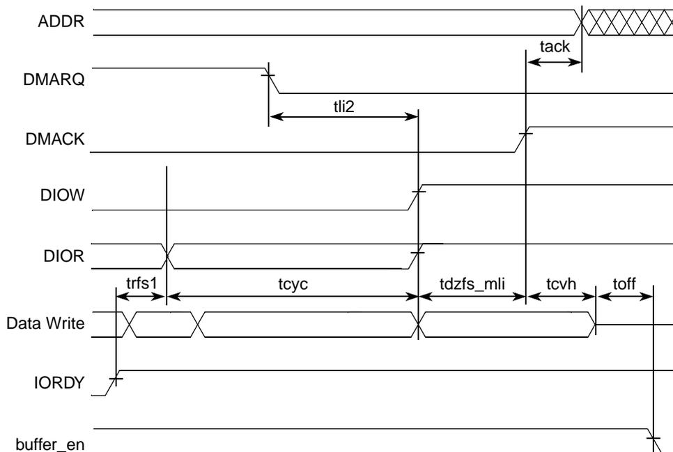
**Figure 27-25. UDMA Out Device Terminates Transfer**
