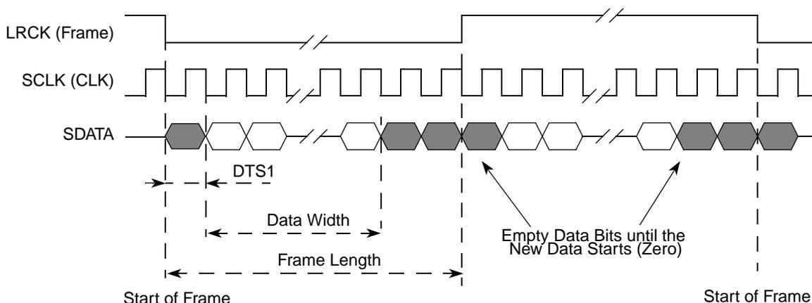
**Figure 30-48. I2S-Data Transmission**
