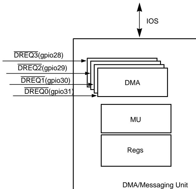
**Figure 28-59. PCI\_DMA Block Diagram**
