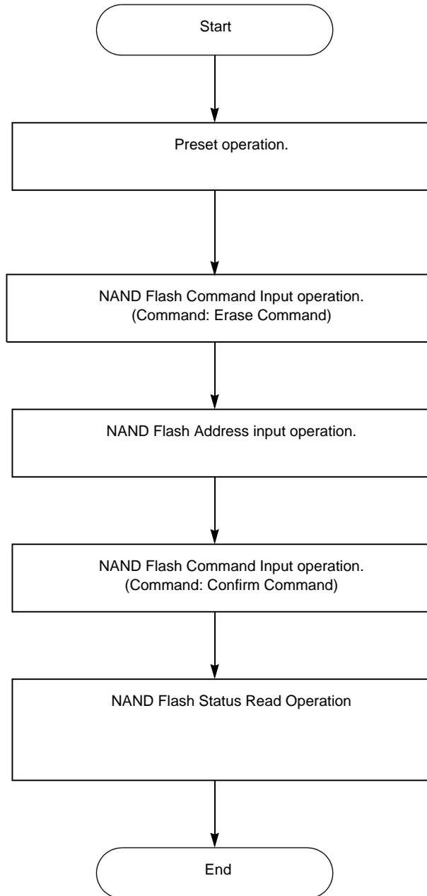
Figure 26-43. Flow Chart of Erase NAND Flash Operation
