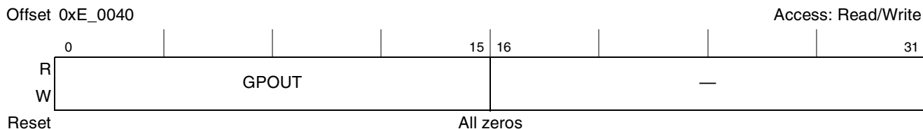
Figure 17-8. General-Purpose Output Data Register (GPOUTDR)
