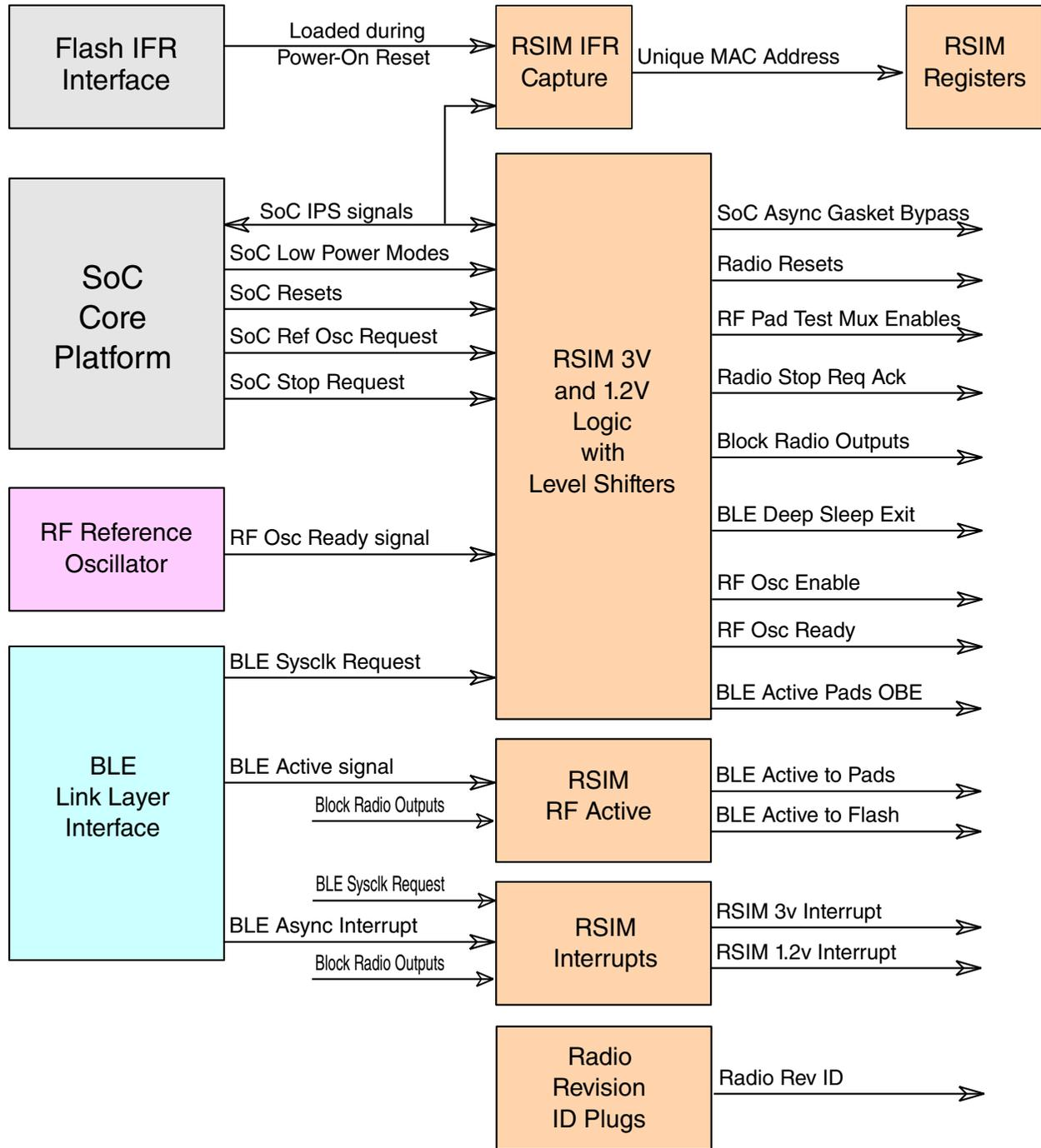
**Figure 44-2. Block diagram**
