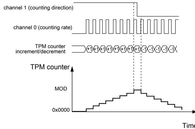
**Figure 32-28. Quadrature Decoder – Count and Direction Encoding mode**
