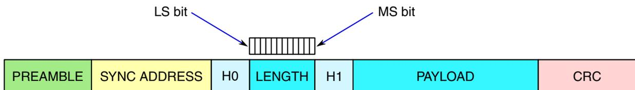
**Figure 44-73. LENGTH Bit Ordering (LSB First)**
