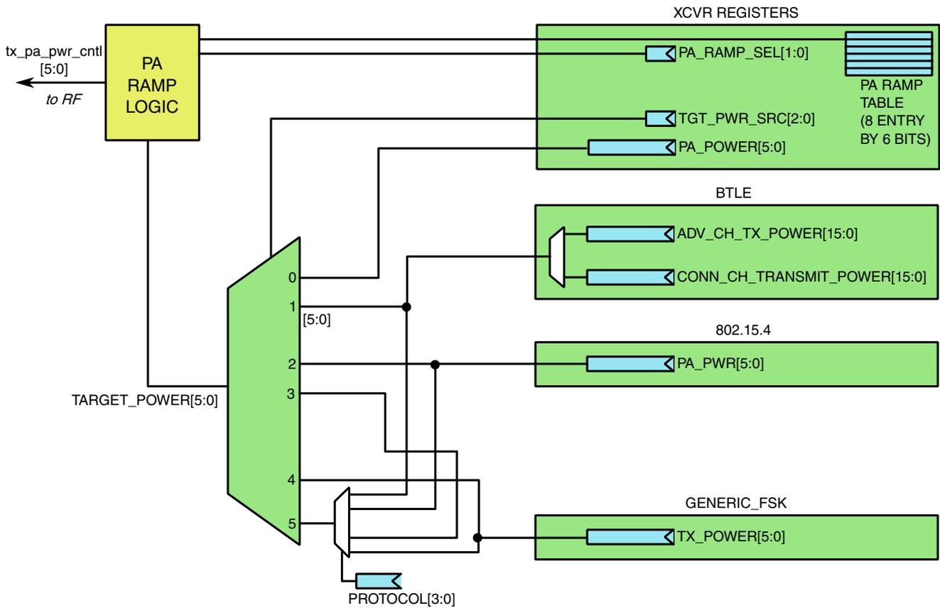
**Figure 44-55. PA Target Power Selection**
