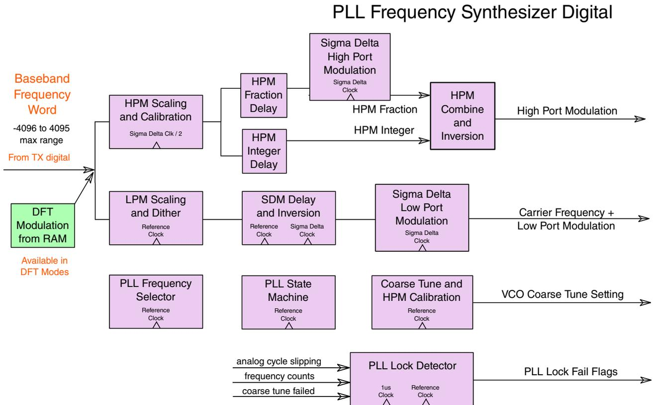
Figure 44-14. PLL Frequency Synthesizer
