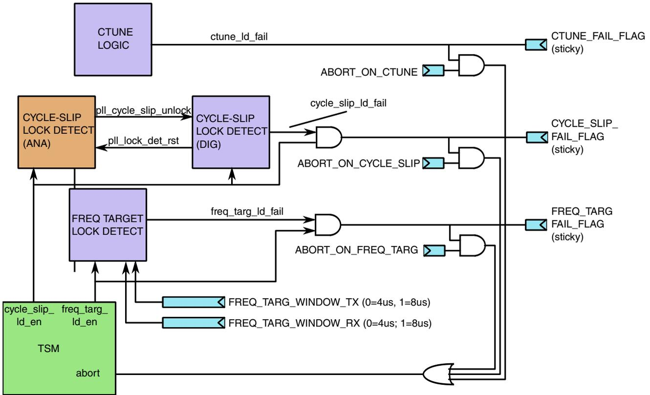
**Figure 44-51. PLL UNLOCK MONITORING AND ABORT LOGIC**
