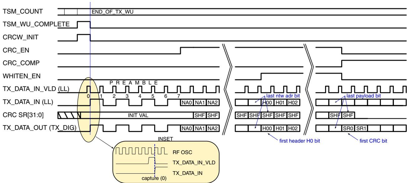
**Figure 44-82. BIT STREAM PROCESSING CRC AND WHITENING TX TIMING**
