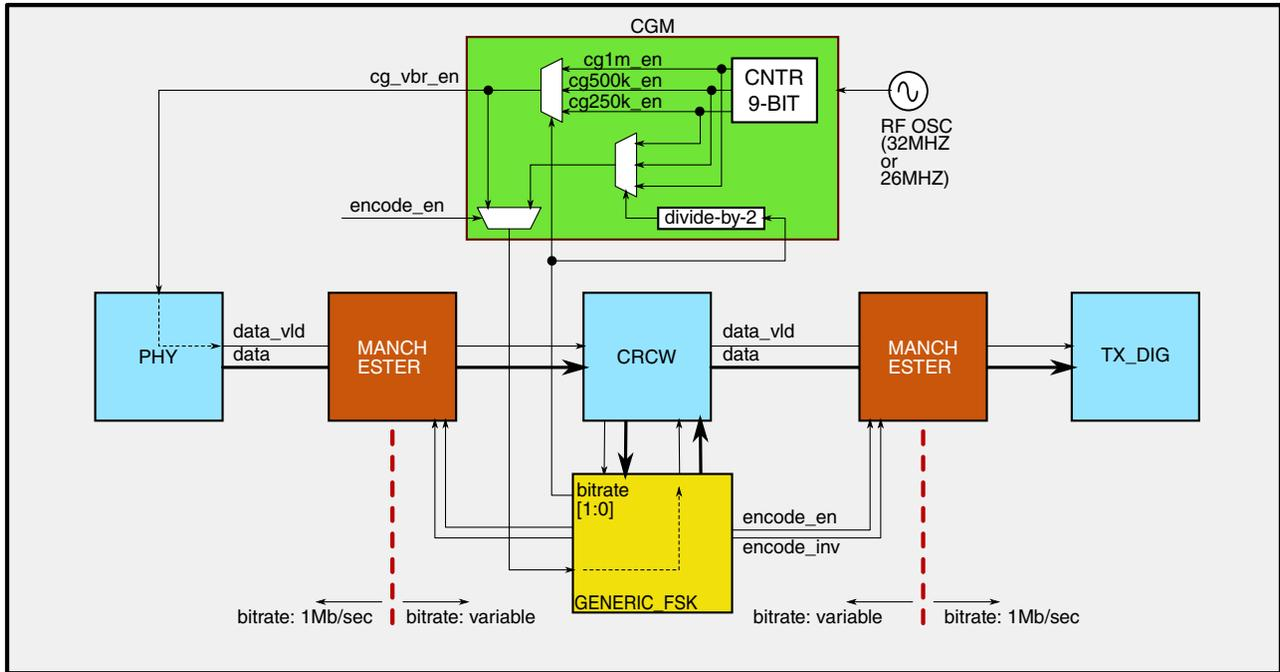
**Figure 44-86. BITSTREAM PROCESSING WITH MANCHESTER ENCODING**
