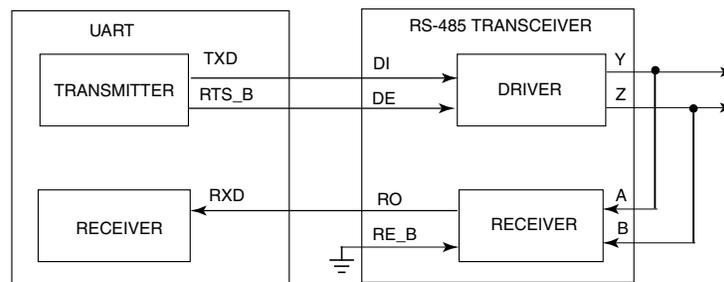
Figure 38-4. Transceiver driver enable using LPUART\_RTS
