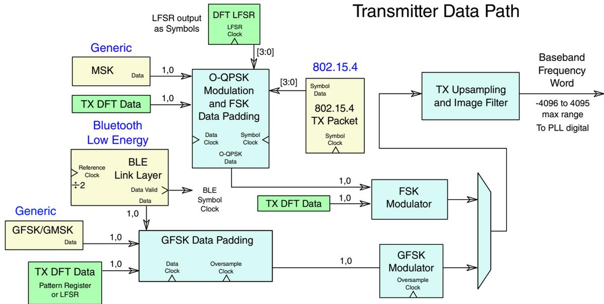
Figure 44-4. Transmitter Digital
