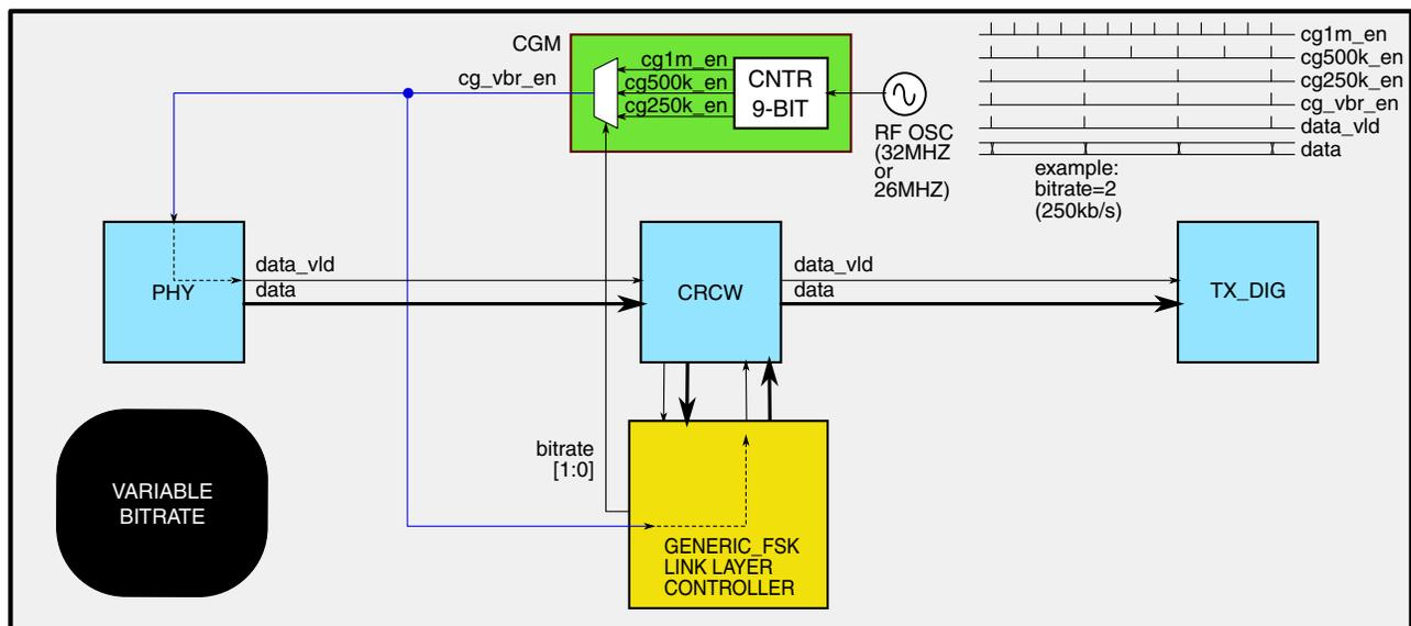
**Figure 44-84. BITSTREAM PROCESSING WITH VARIABLE BIT RATE**
