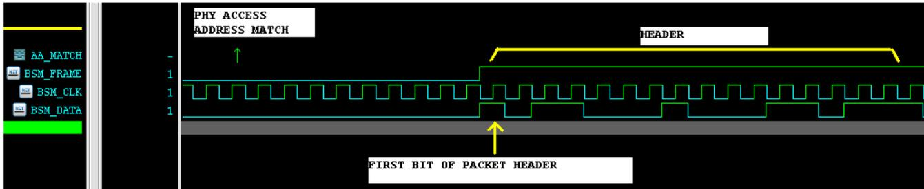
**Figure 44-47. BSM Timing Diagram**
