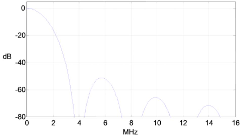
Figure 44-22. 4th order CIC (OSR=8) Decimation Filter Frequency Response
