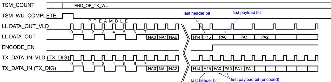
**Figure 44-87. BIT STREAM PROCESSING (WITH MANCHESTER) TX TIMING -- 1MBIT/SEC OTA**
