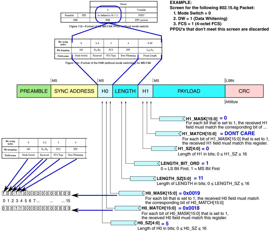
Figure 44-76. GENERIC FSK PACKET STRUCTURE AS APPLIED TO 802.15.4g PHR
