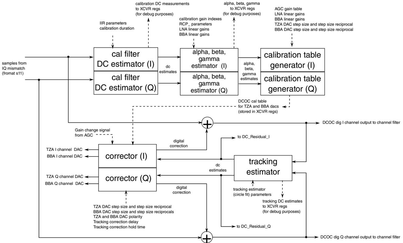
Figure 44-32. RX\_DIG DCOC Block Diagram
