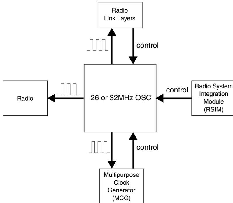
Figure 3-20. Reference OSC configuration
