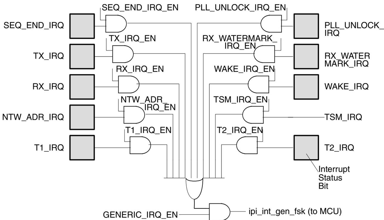
**Figure 44-92. GENERIC\_FSK Interrupt Architecture**
