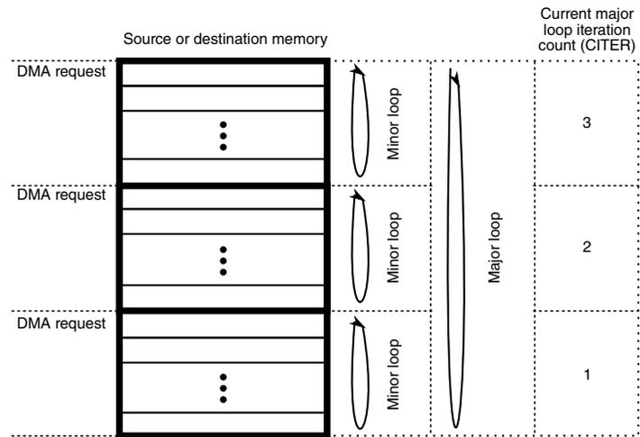
Figure 23-5. Example of multiple loop iterations
