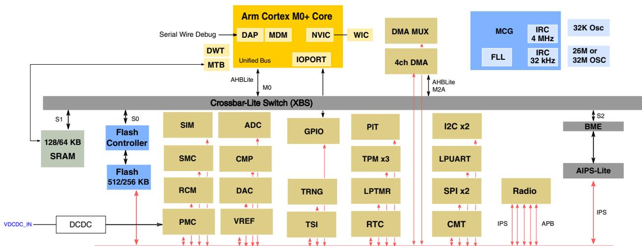
**Figure 1-1. MWPR1x24 Detailed Block Diagram**
