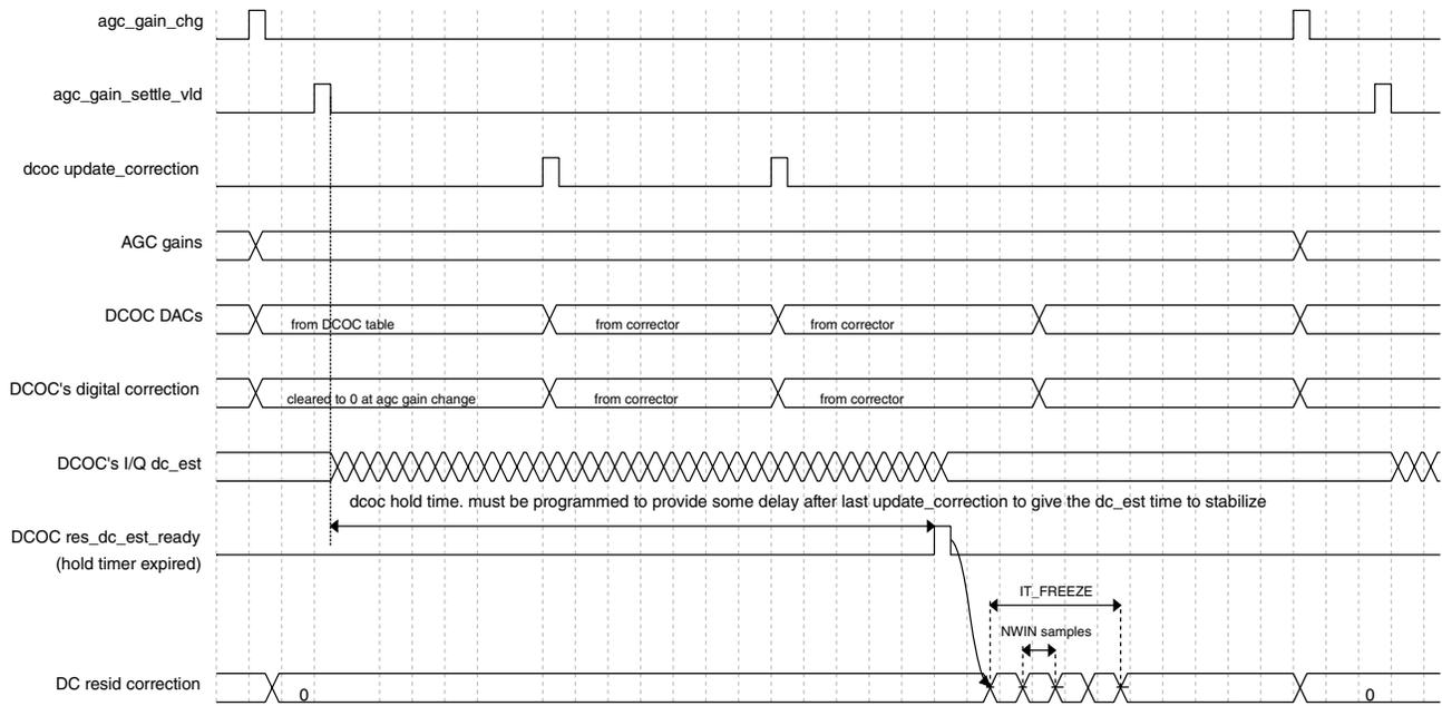
Figure 44-41. DC residual mode 2 timing
