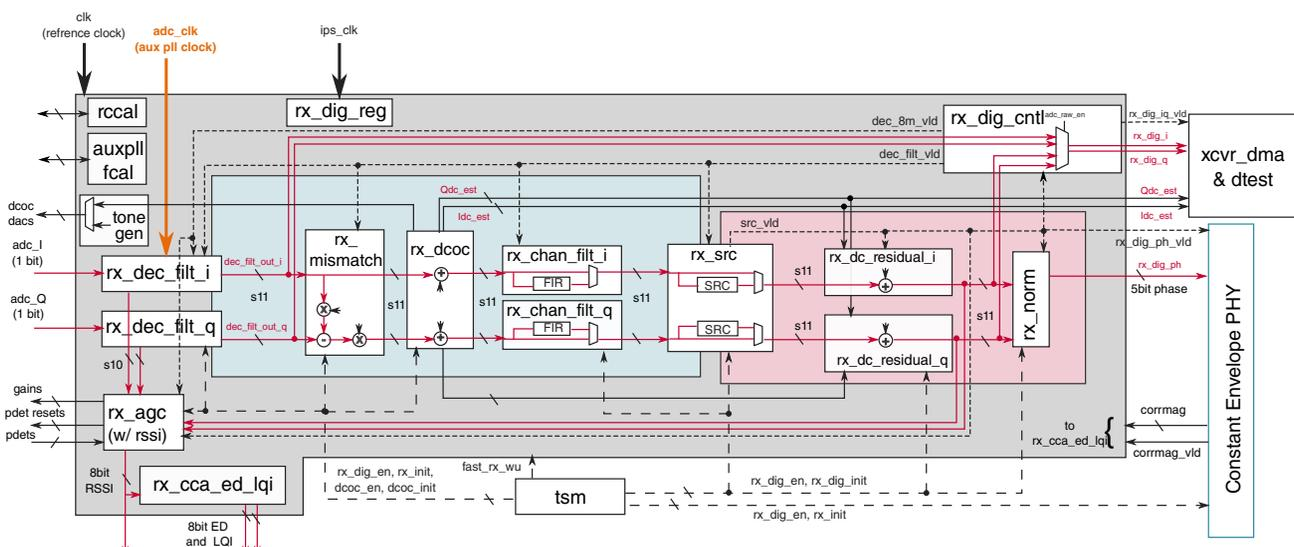
**Figure 44-20. RX DIG Block diagram**
