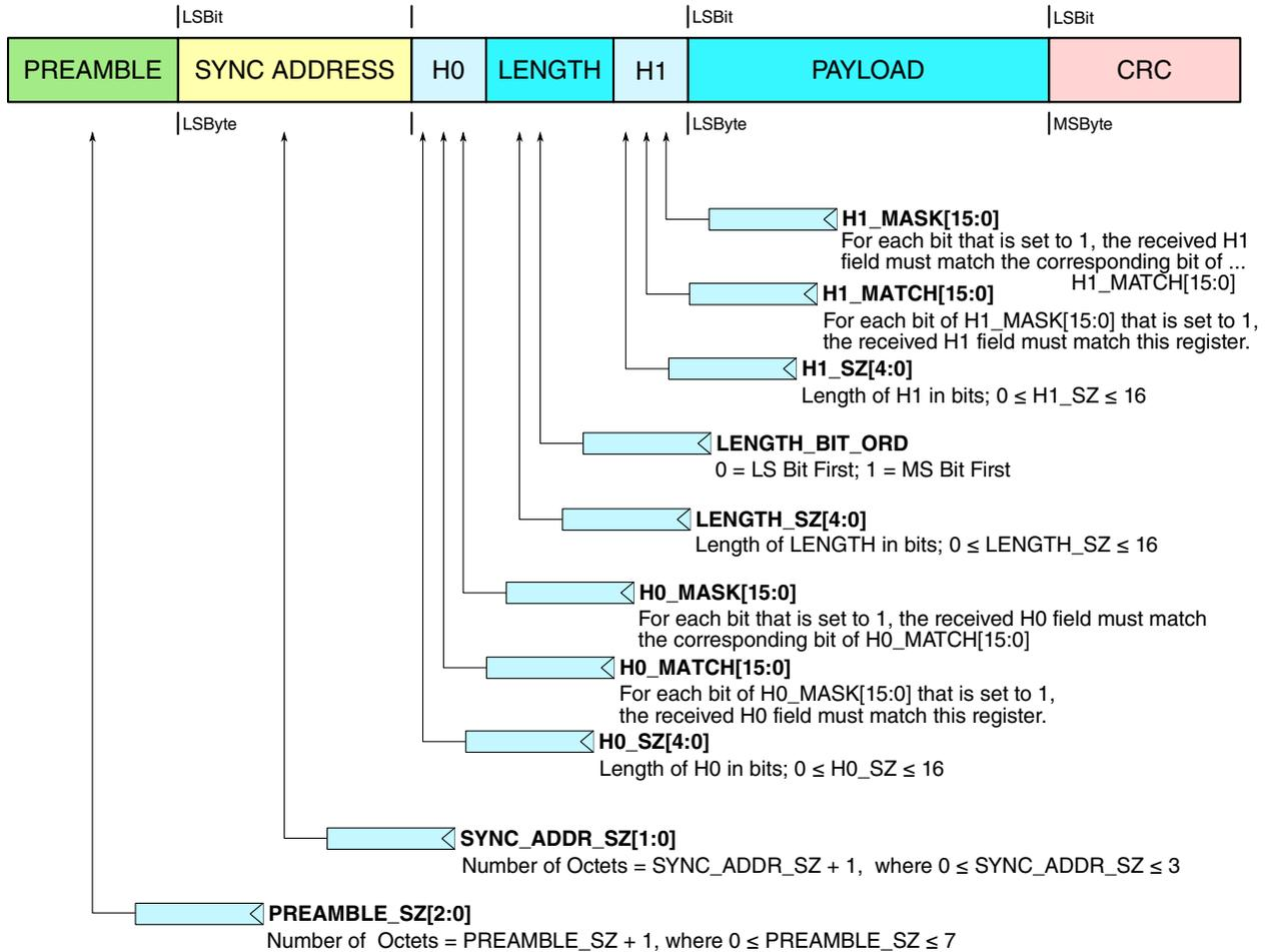
**Figure 44-69. Packet Structure Definitions (Part 1)**
