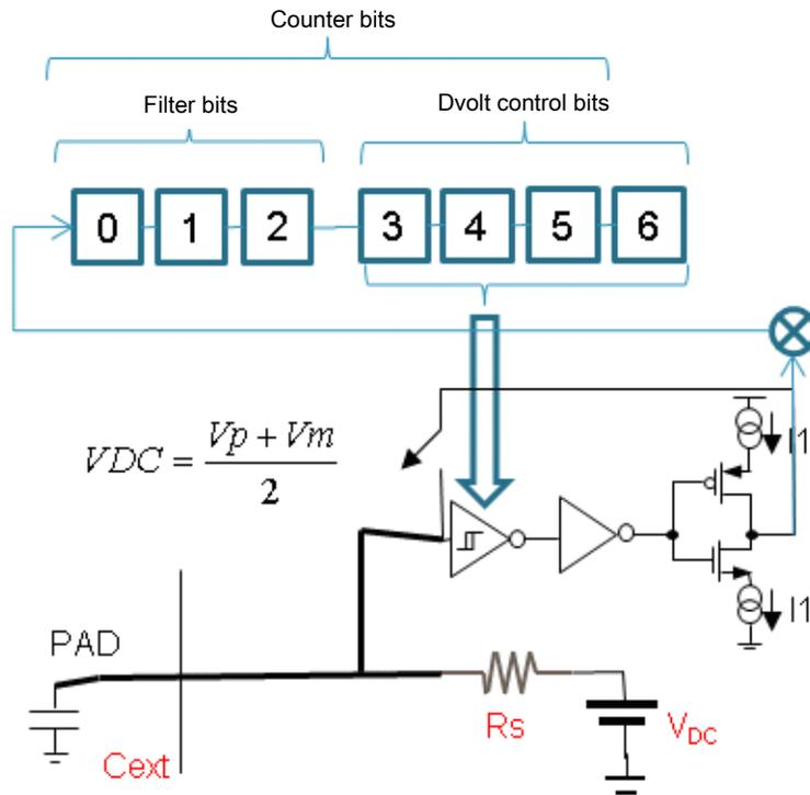
**Figure 41-9. Block diagram automatic noise threshold operation**
