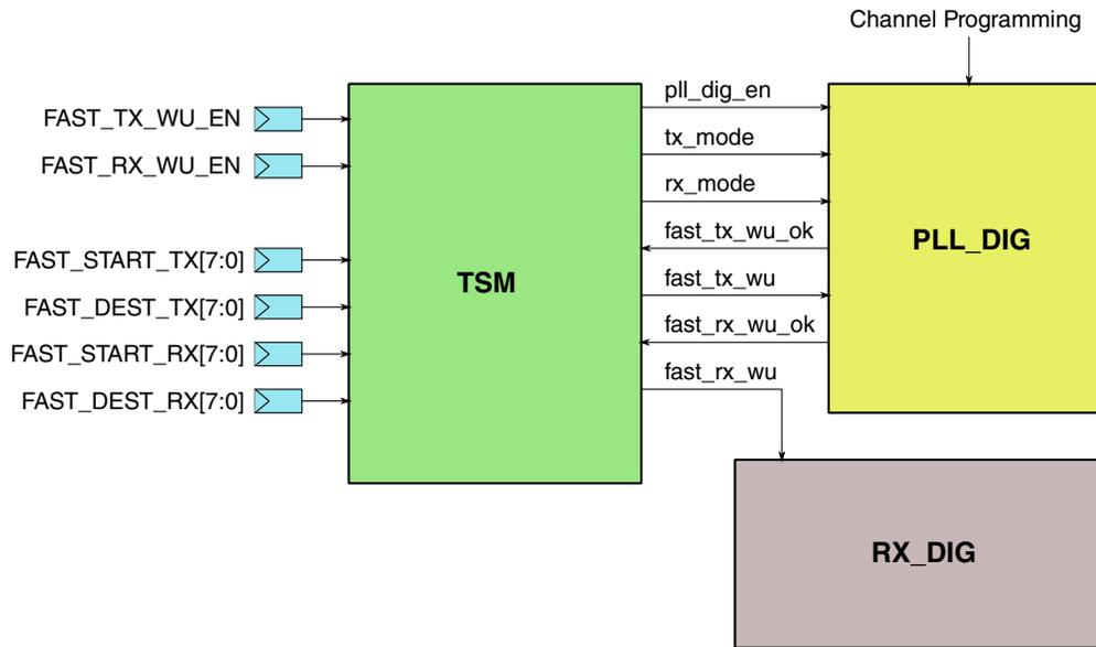
**Figure 44-59. Transceiver Signalling To Support TSM Fast Warmups**
