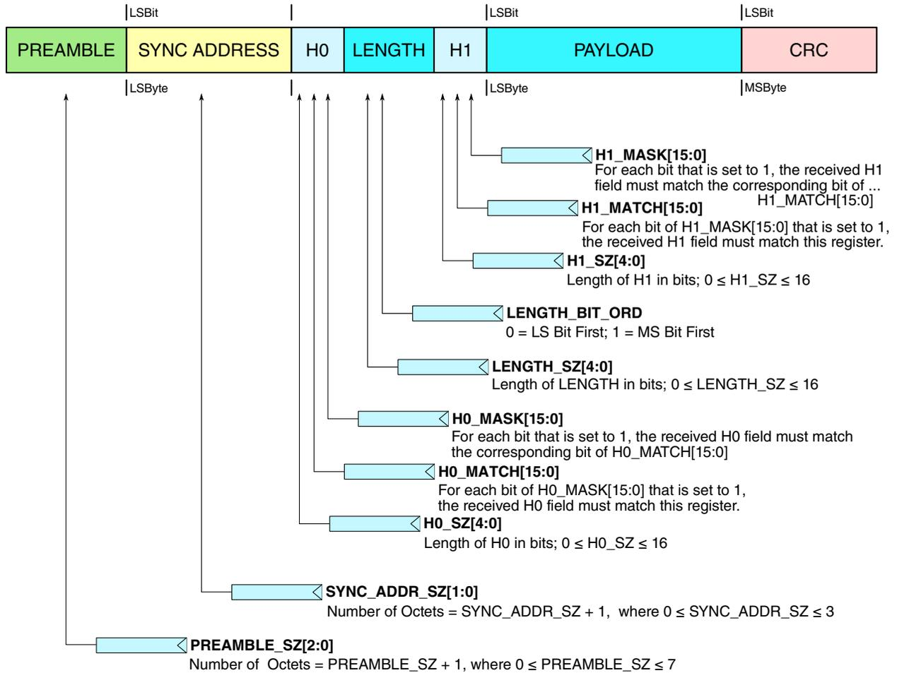
**Figure 44-70. Packet Structure Definitions (Part 2)**
