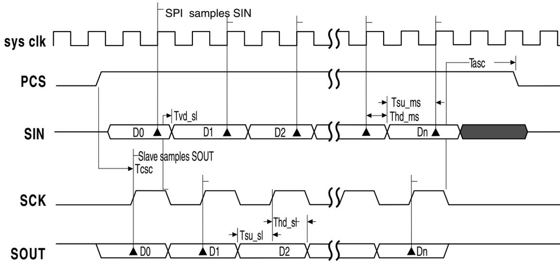
Figure 36-8. SPI Modified Transfer Format (MTFE=1, CPHA=0,  $f_{sck} = f_{sys}/2$ )
