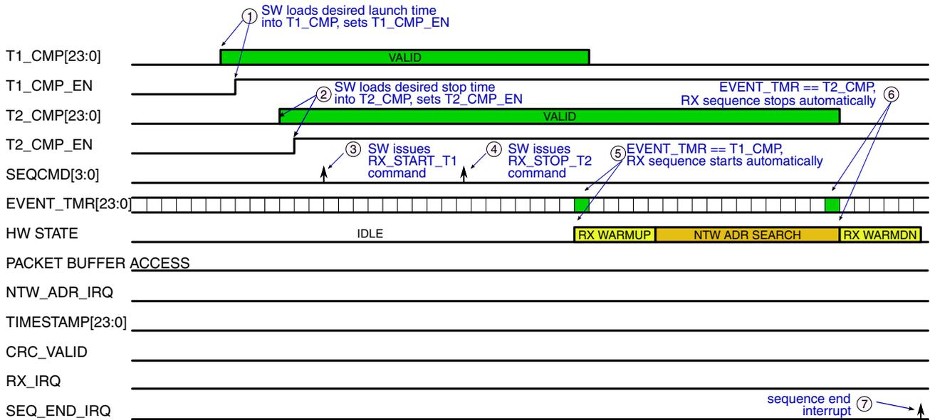
**Figure 44-97. GENERIC FSK RX SEQUENCE: SLAVE CHANNEL SEARCH, LAUNCH VIA T1, STOP VIA T2**
