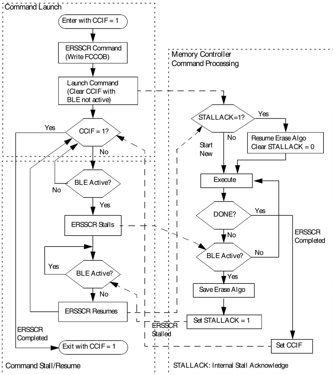
Figure 27-5. BLE Active Impact on Erase Flash Sector Operation
