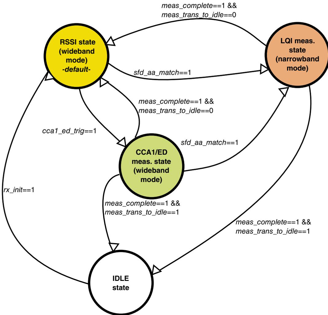
Figure 44-26. Module state machine
