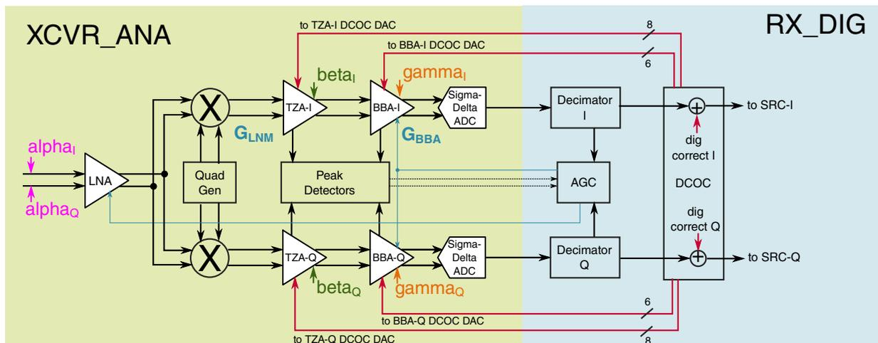
**Figure 44-38. Receiver model showing three contributors of DC offset**
