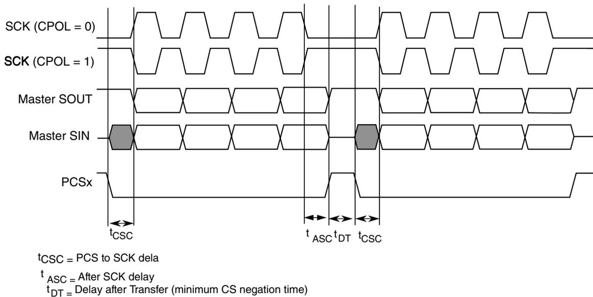
**Figure 36-13. Example of non-continuous format (CPHA=1, CONT=0)**
