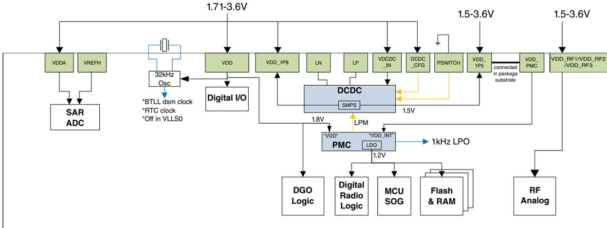
Figure 3-10. Bypass Power Tree
