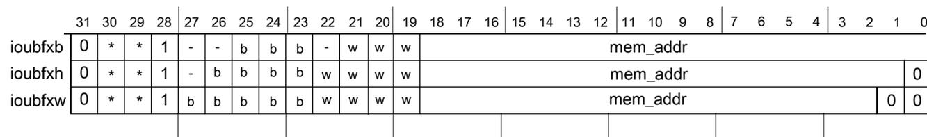
**Figure 17-11. Decorated load address: unsigned bit field extract**
