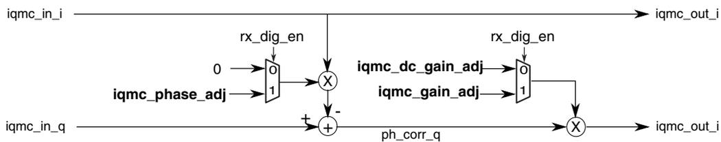
**Figure 44-31. I/Q Mismatch Correction Block Diagram**
