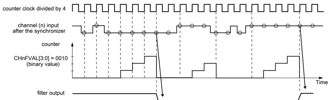
**Figure 32-24. Channel input filter example**
