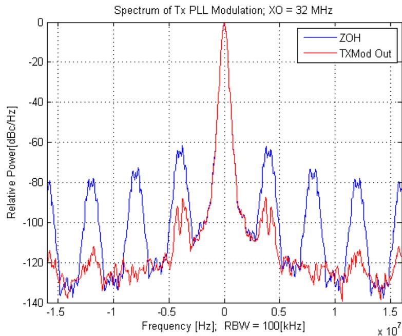
**Figure 44-12. Comparison of Transmit Modulation Images at the PLL Output for 500 kbps GMSK**
