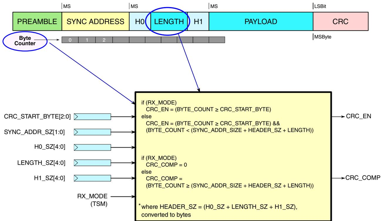
**Figure 44-78. GENERIC FSK: CONTROL OF CRC**
