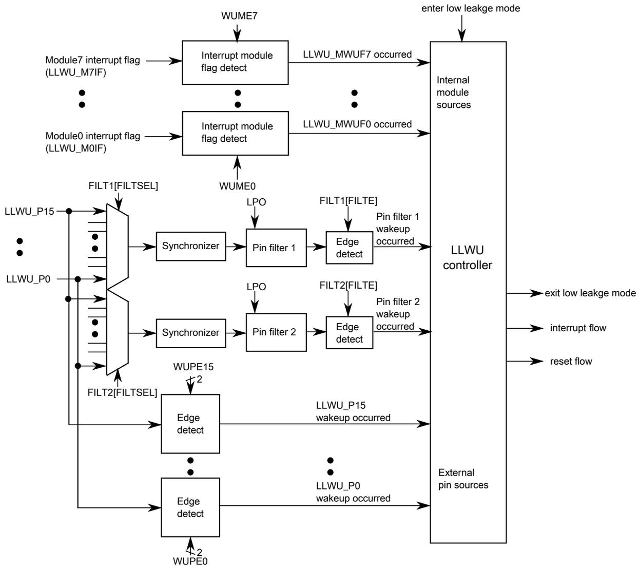
Figure 15-1. LLWU block diagram
