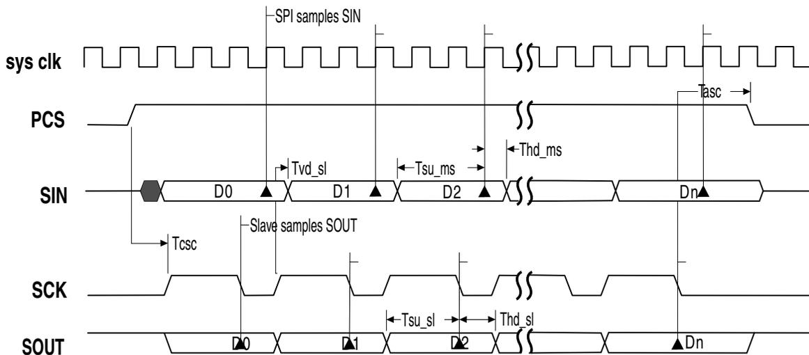
Figure 36-11. SPI Modified Transfer Format (MTFE=1, CPHA=1,  $f_{sck} = f_{sys}/3$ )
