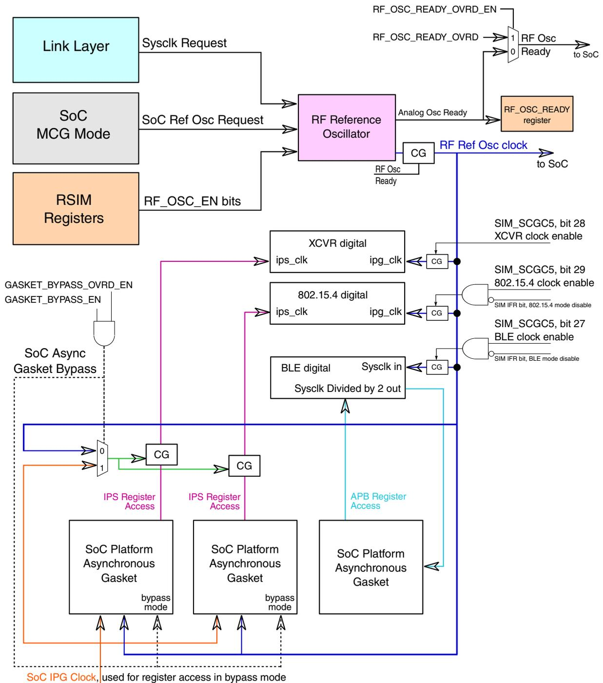
Figure 44-3. Radio Clocking Configuration
