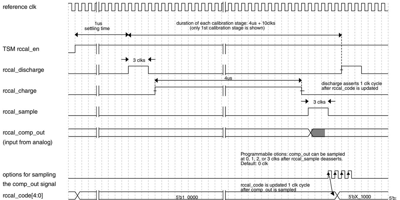
Figure 44-45. RX RCCAL timing
