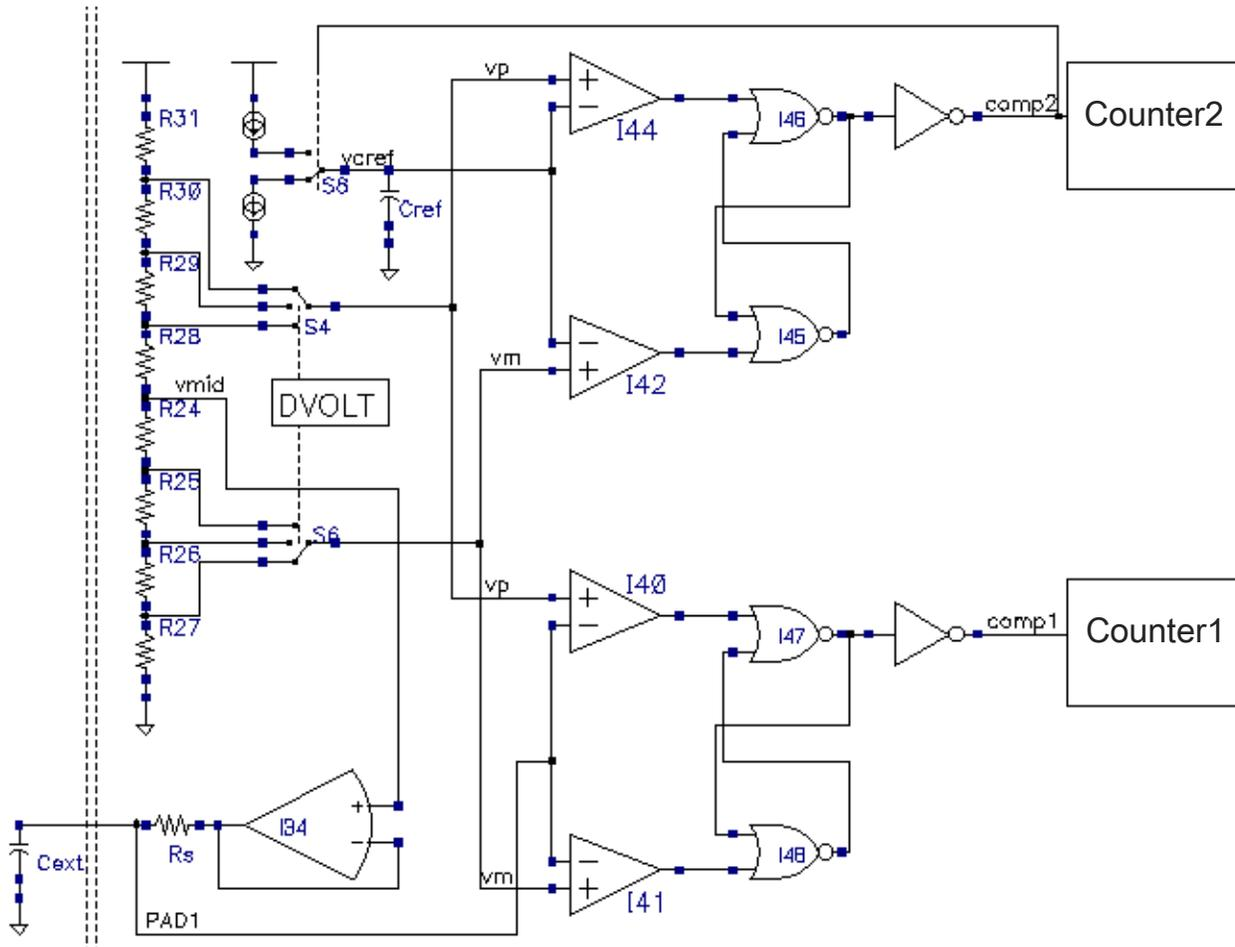
**Figure 41-5. TSI circuit in noise detection mode**
