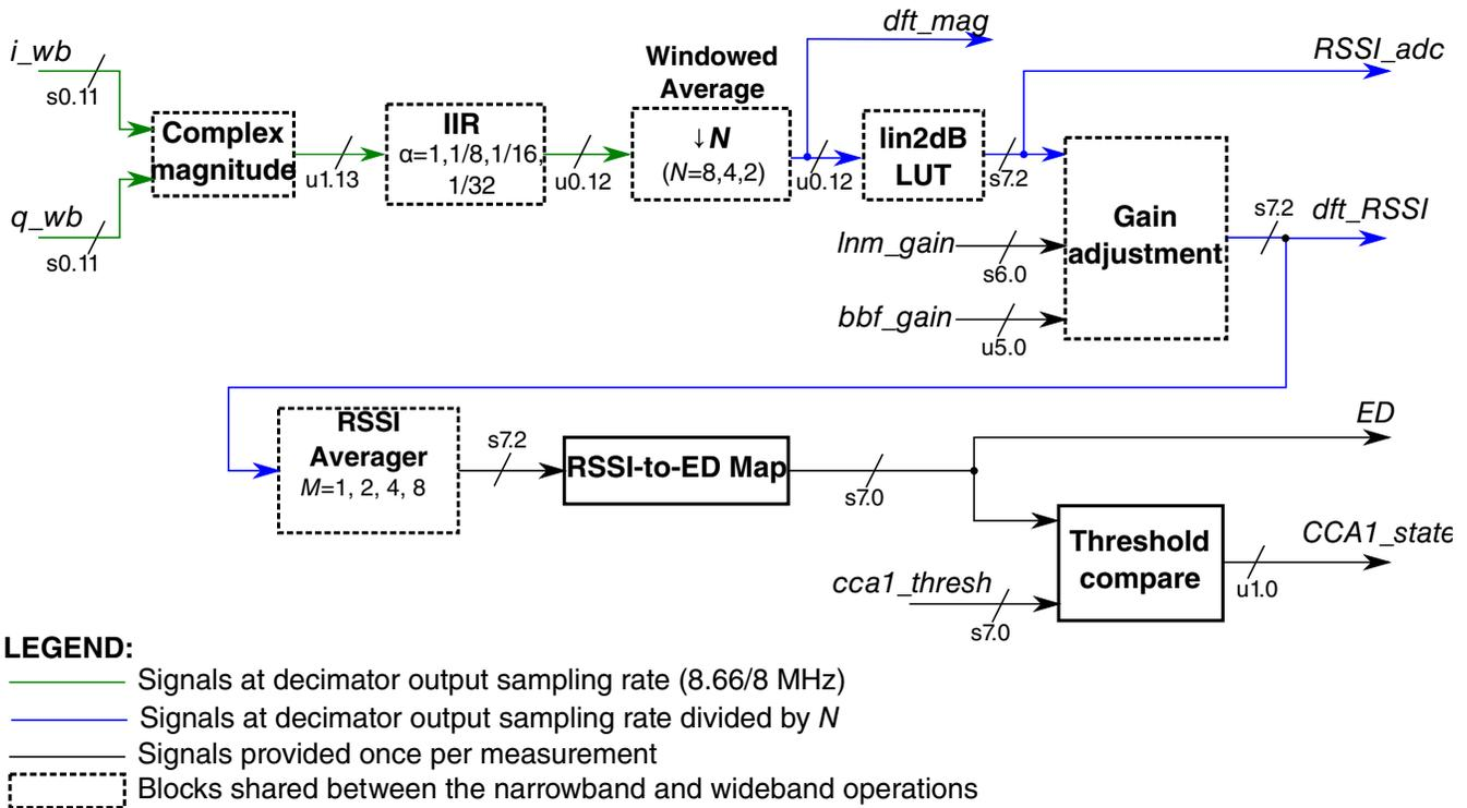
**Figure 44-27. Block diagram instantiated for wideband mode**
