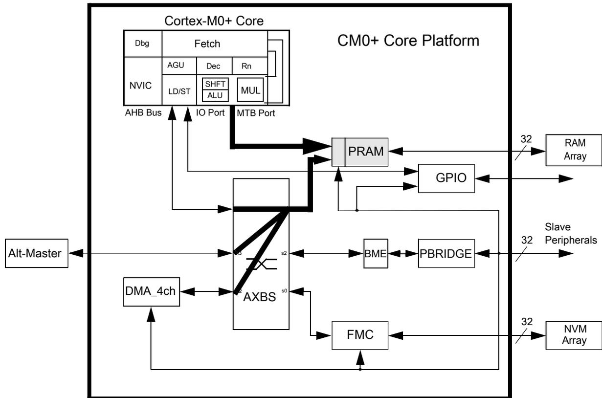
**Figure 19-1. Generic Cortex-M0+ core platform block diagram**
