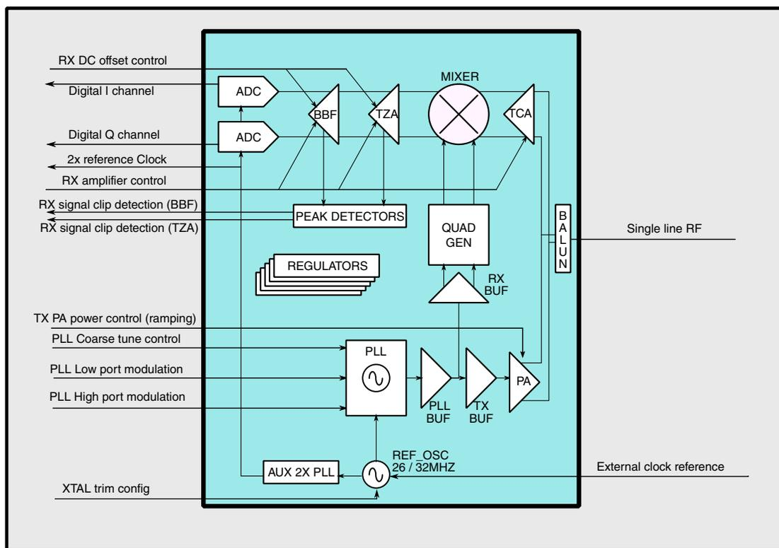
Figure 44-66. Analog Radio Block diagram
