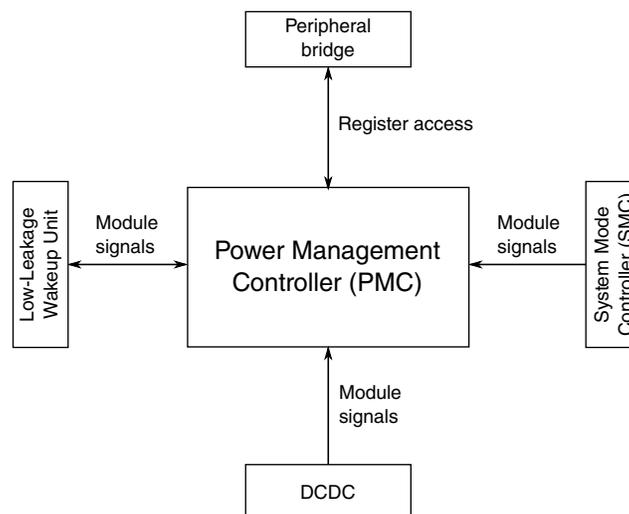
**Figure 3-6. PMC configuration****Table 3-12. Reference links to related information**
