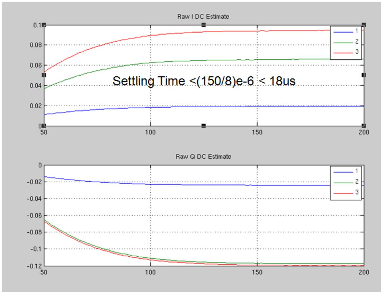
**Figure 44-37. 3-step {I,Q} DC estimation during calibration**
