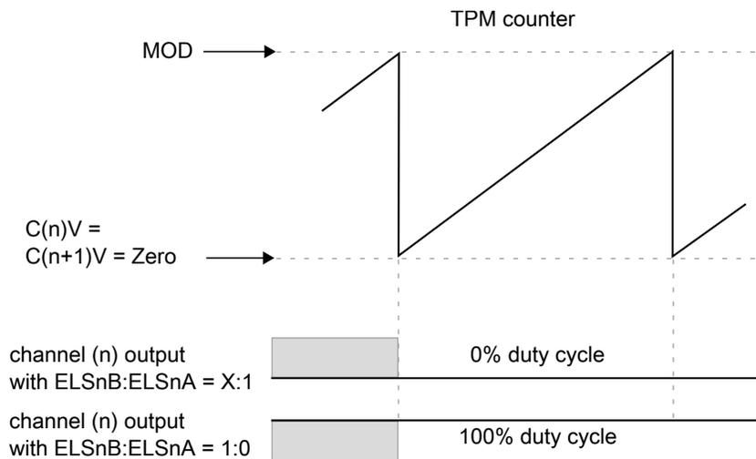
**Figure 32-20. Channel (n) output if  $(C(n)V = C(n+1)V = \text{zero})$**
