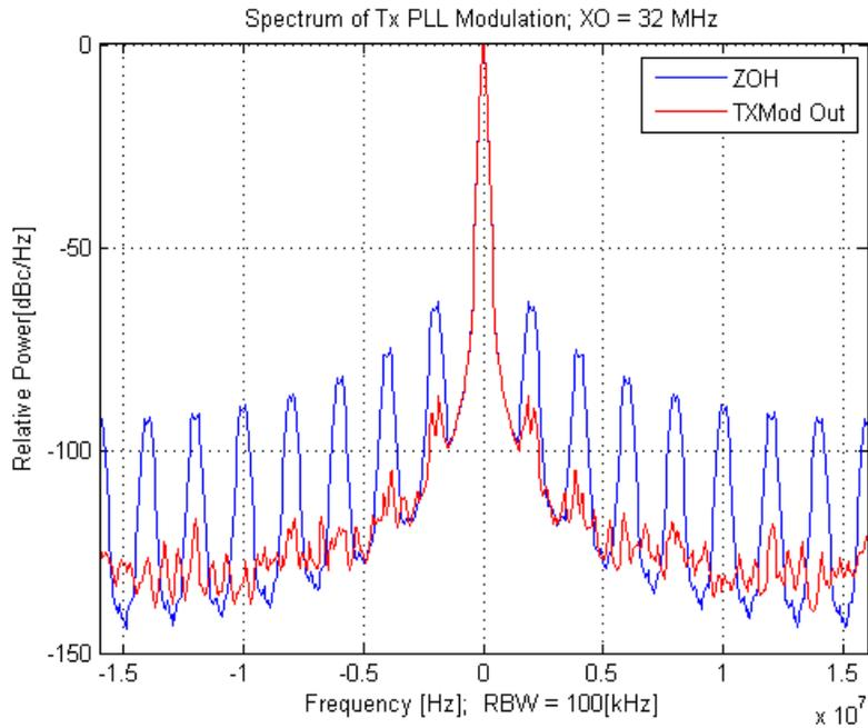
**Figure 44-13. Comparison of Transmit Modulation Images at the PLL Output for 250 kbps GMSK**
