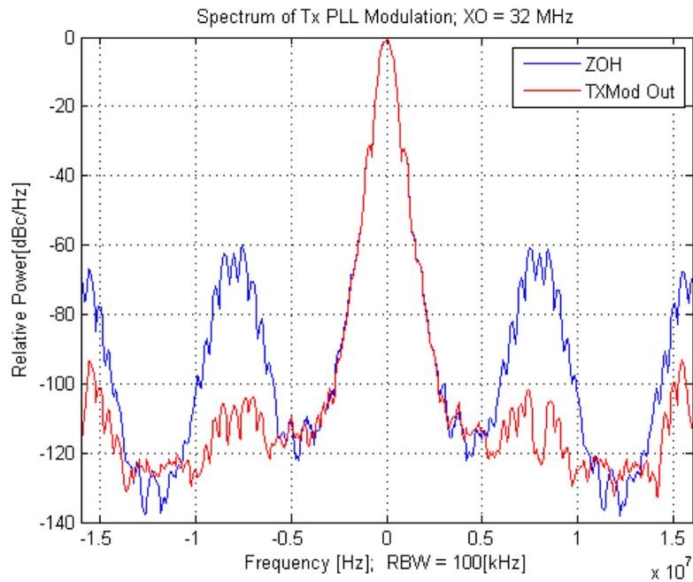
**Figure 44-11. Comparison of Transmit Modulation Images at the PLL Output for BLE (1 Mbps GMSK)**
