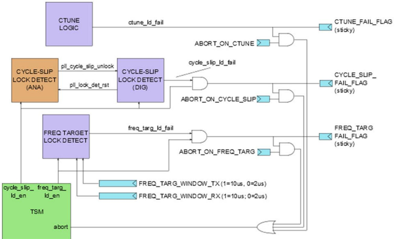
Figure 44-16. PLL Lock Detect Block Diagram
