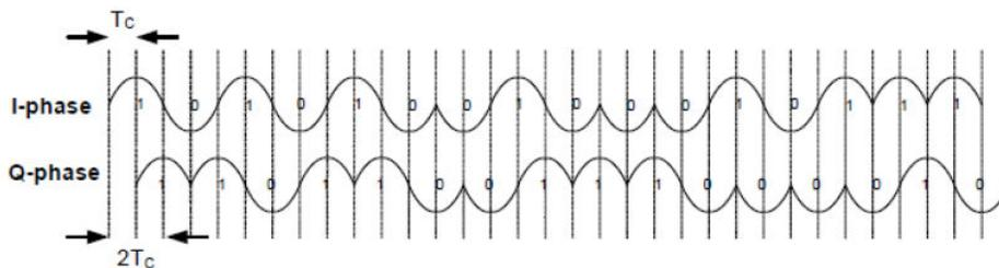
Figure 71—Sample baseband chip sequences with pulse shaping
