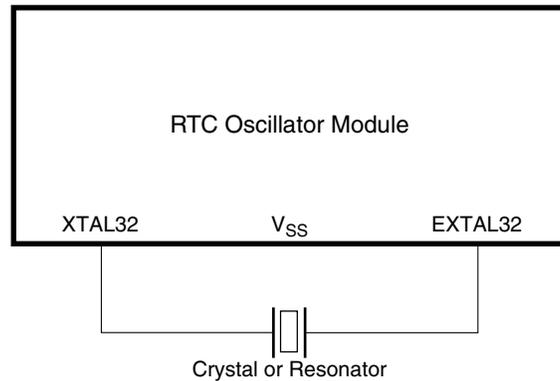
**Figure 25-2. Crystal Connections**
