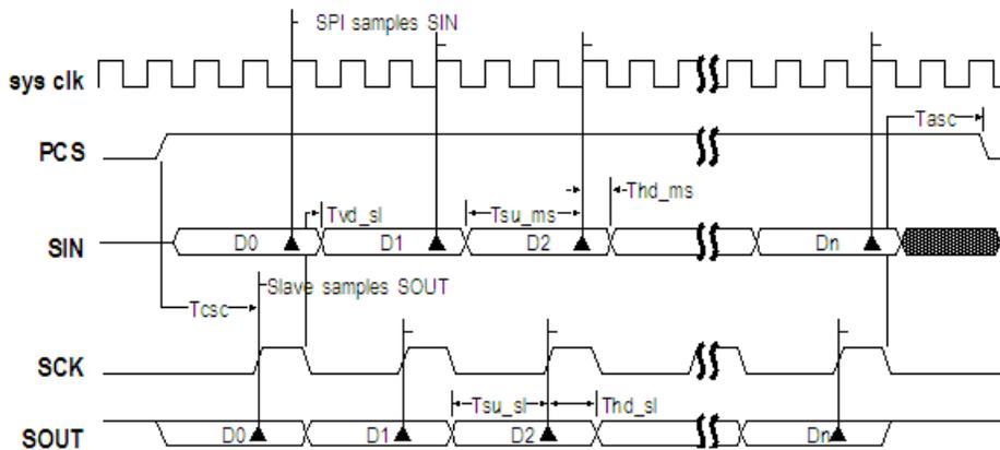
Figure 36-9. SPI Modified Transfer Format (MTFE=1, CPHA=0,  $f_{sck} = f_{sys}/3$ )
