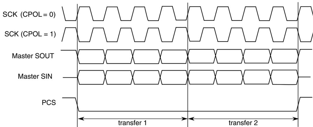
Figure 36-16. Continuous SCK timing diagram (CONT=1)
