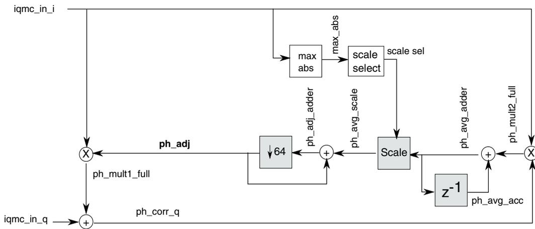
Figure 44-30. I/Q Phase Mismatch Calibration Block Diagram
