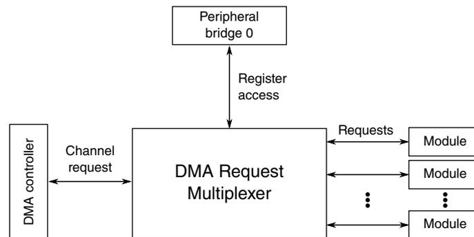
**Figure 3-15. DMA request multiplexer configuration**
