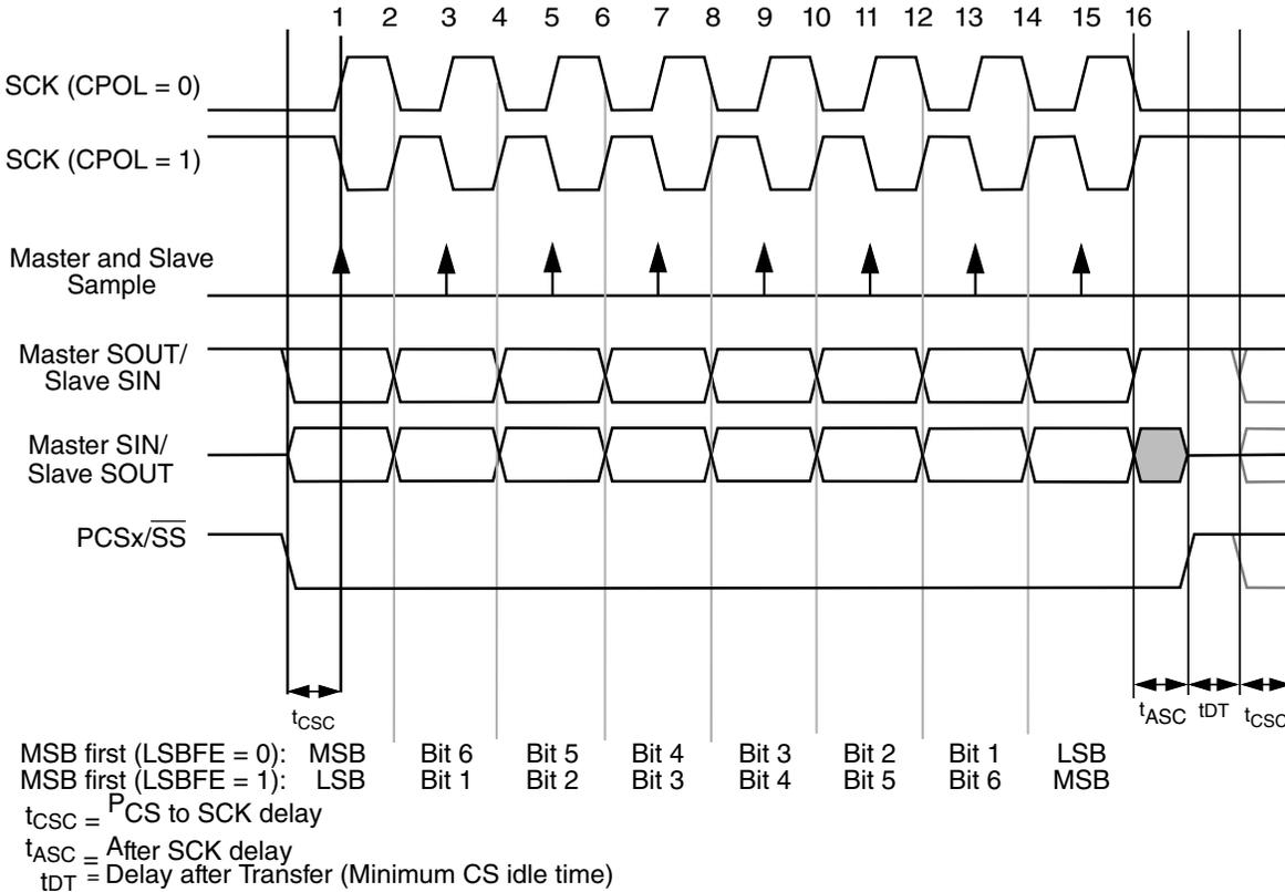
**Figure 36-5. Module transfer timing diagram (MTFE=0, CPHA=0, FMSZ=8)**
