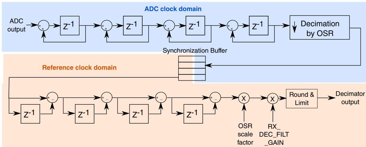
**Figure 44-21. Decimation Filter Block Diagram**
