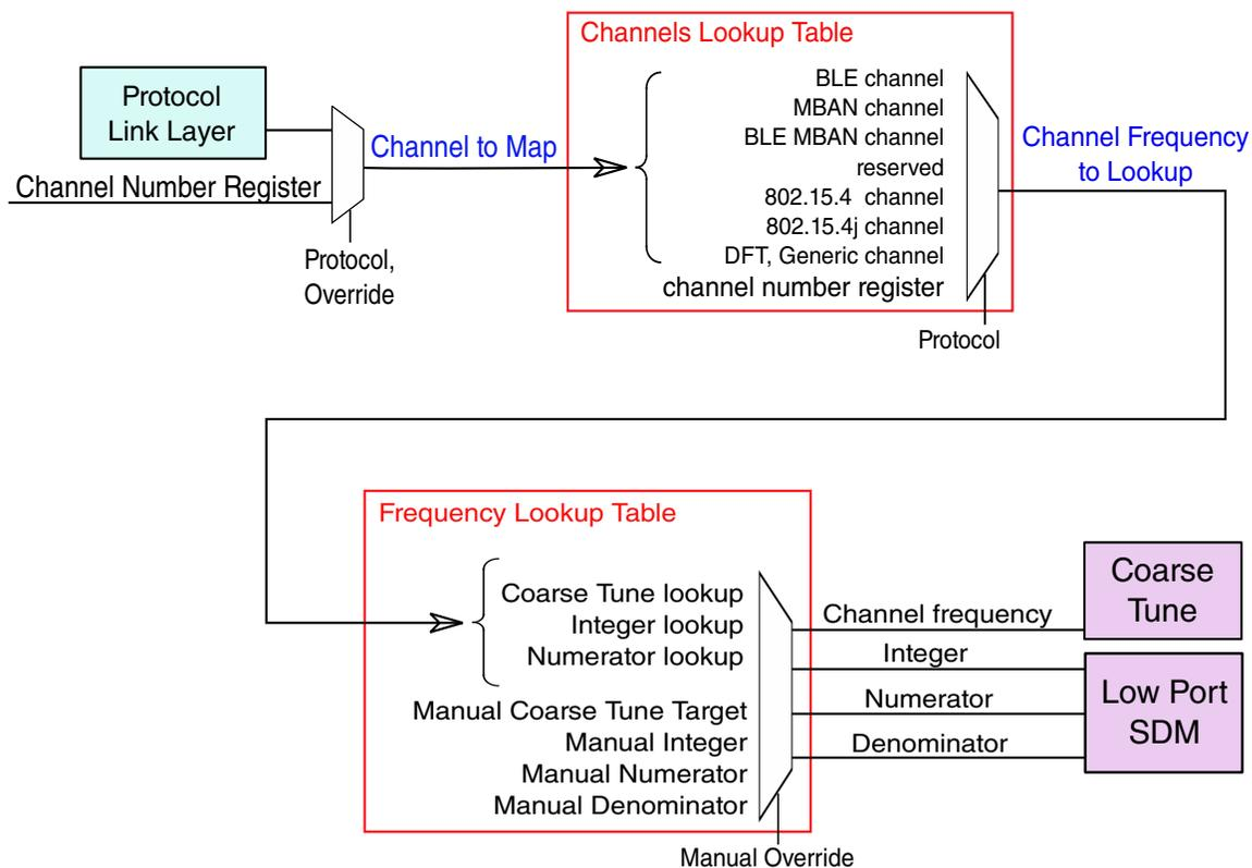
**Figure 44-15. Radio Frequency Selection**
