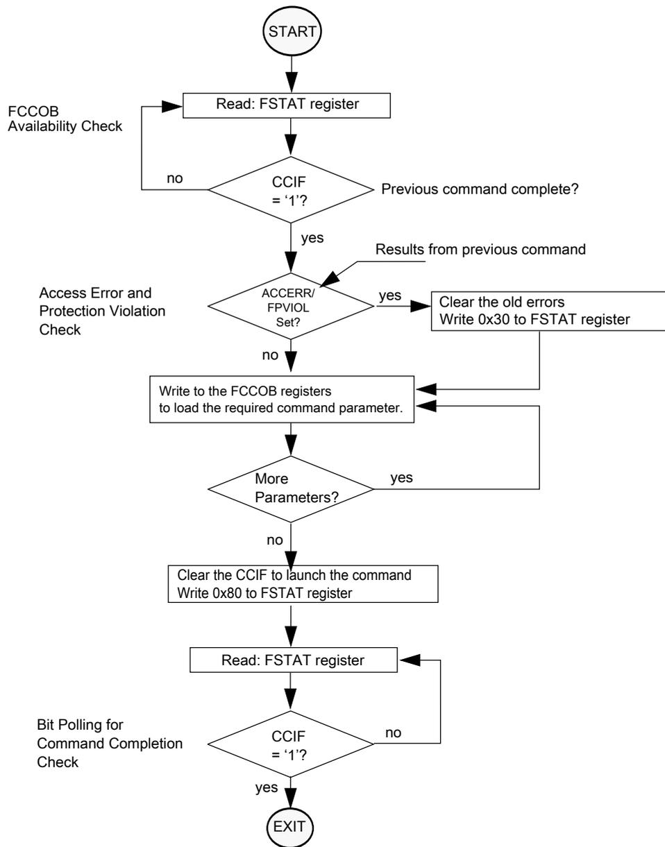
Figure 27-3. Generic flash command write sequence flowchart
