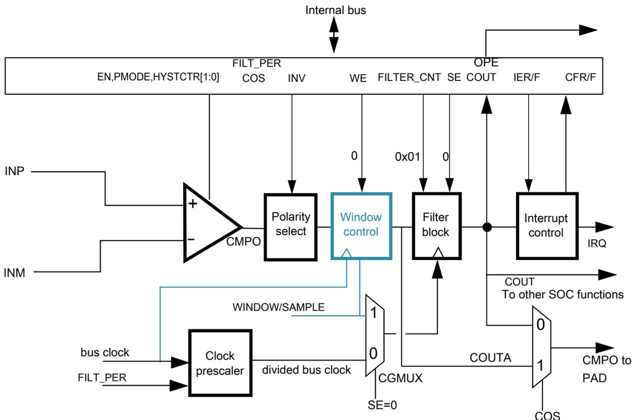
Figure 29-4. Sampled, Non-Filtered (# 3B): sampling interval internally derived
