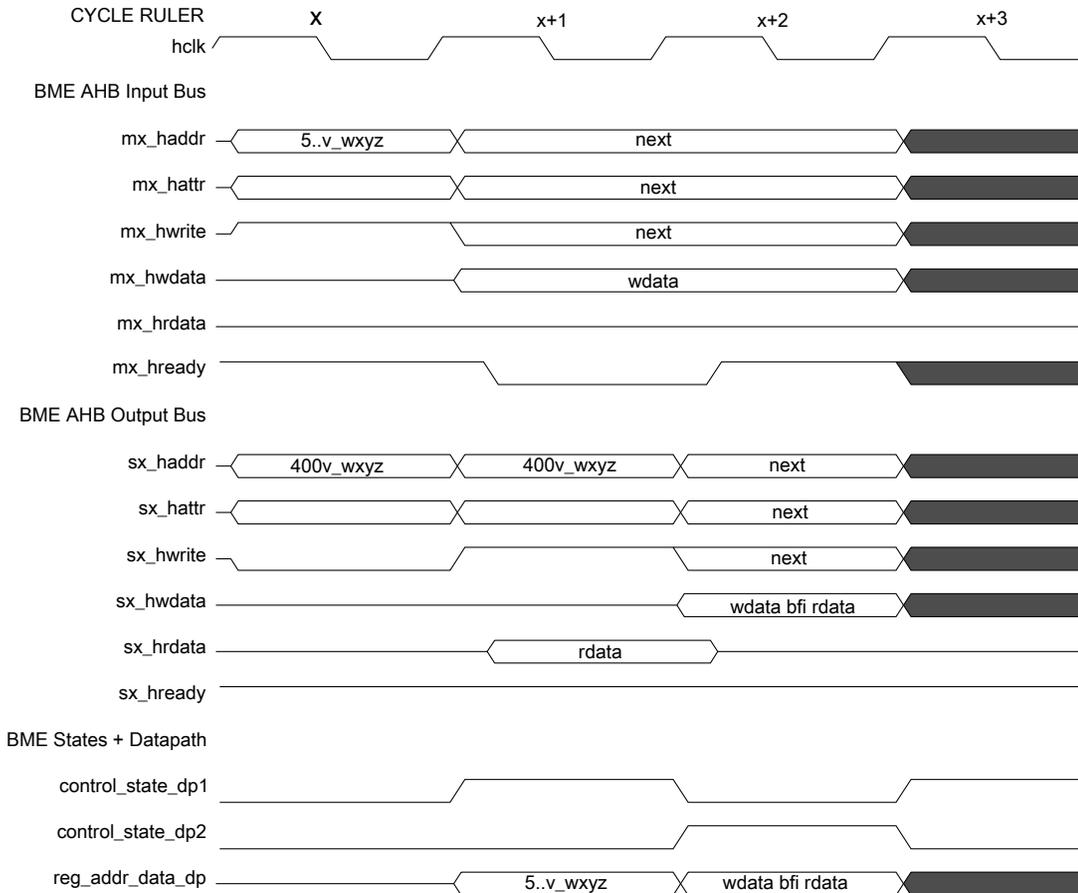
**Figure 17-2. Decorated store: bit field insert timing diagram**
