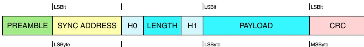
**Figure 44-68. GENERIC\_FSK Packet Structure**
