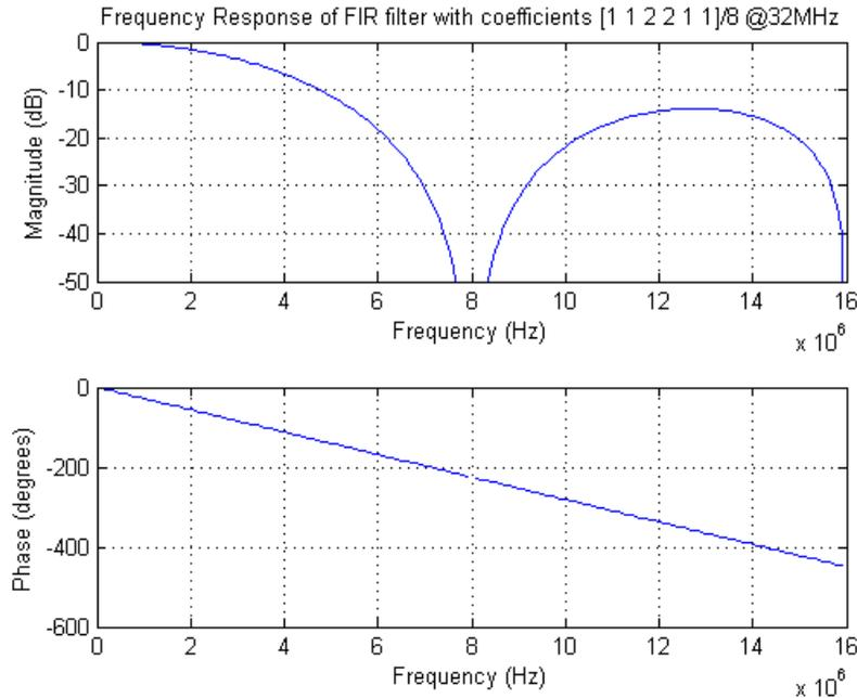
**Figure 44-9. Frequency response of the 6-Tap FIR Transmit Image Suppression filter**
