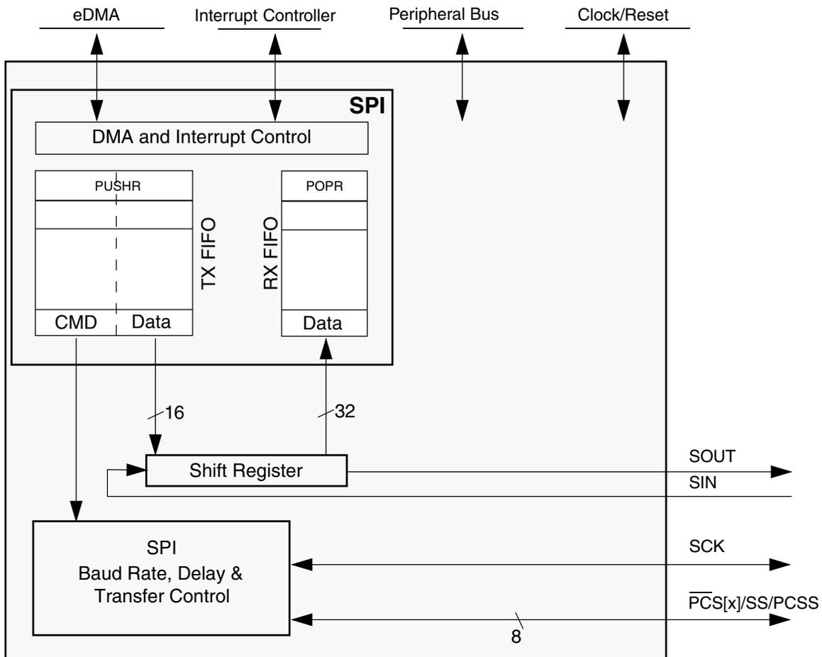
Figure 36-1. SPI Block Diagram
