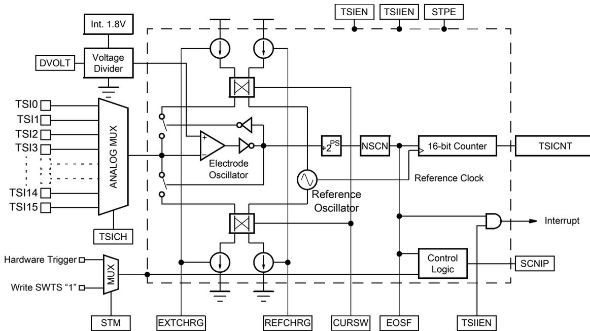
Figure 41-1. TSI module block diagram
