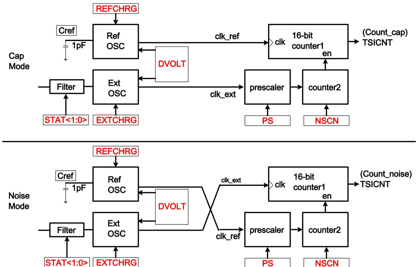
Figure 41-4. TSI noise detection mode block diagram
