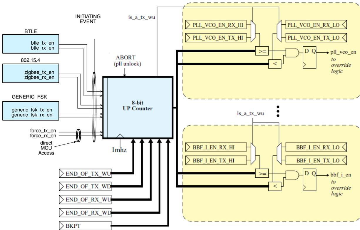
Figure 44-50. 2.4GHZ RADIO TSM BLOCK DIAGRAM
