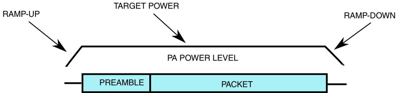
**Figure 44-54. PA Target Power**
