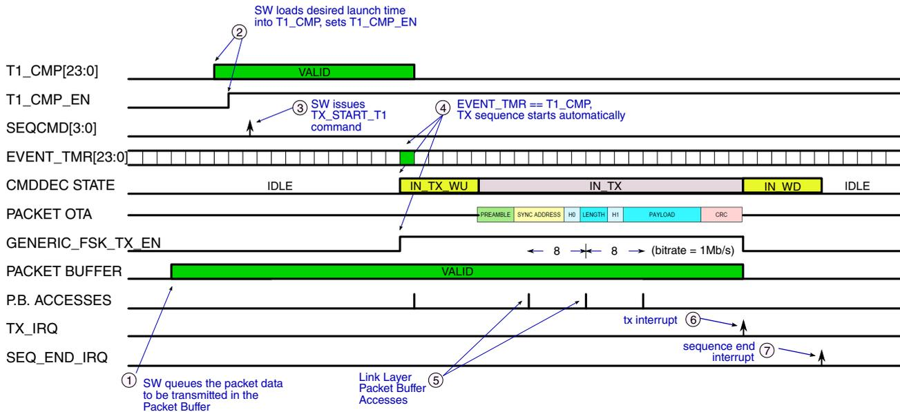
**Figure 44-94. GENERIC\_FSK TX SEQUENCE: LAUNCH VIA T1 TIMER**
