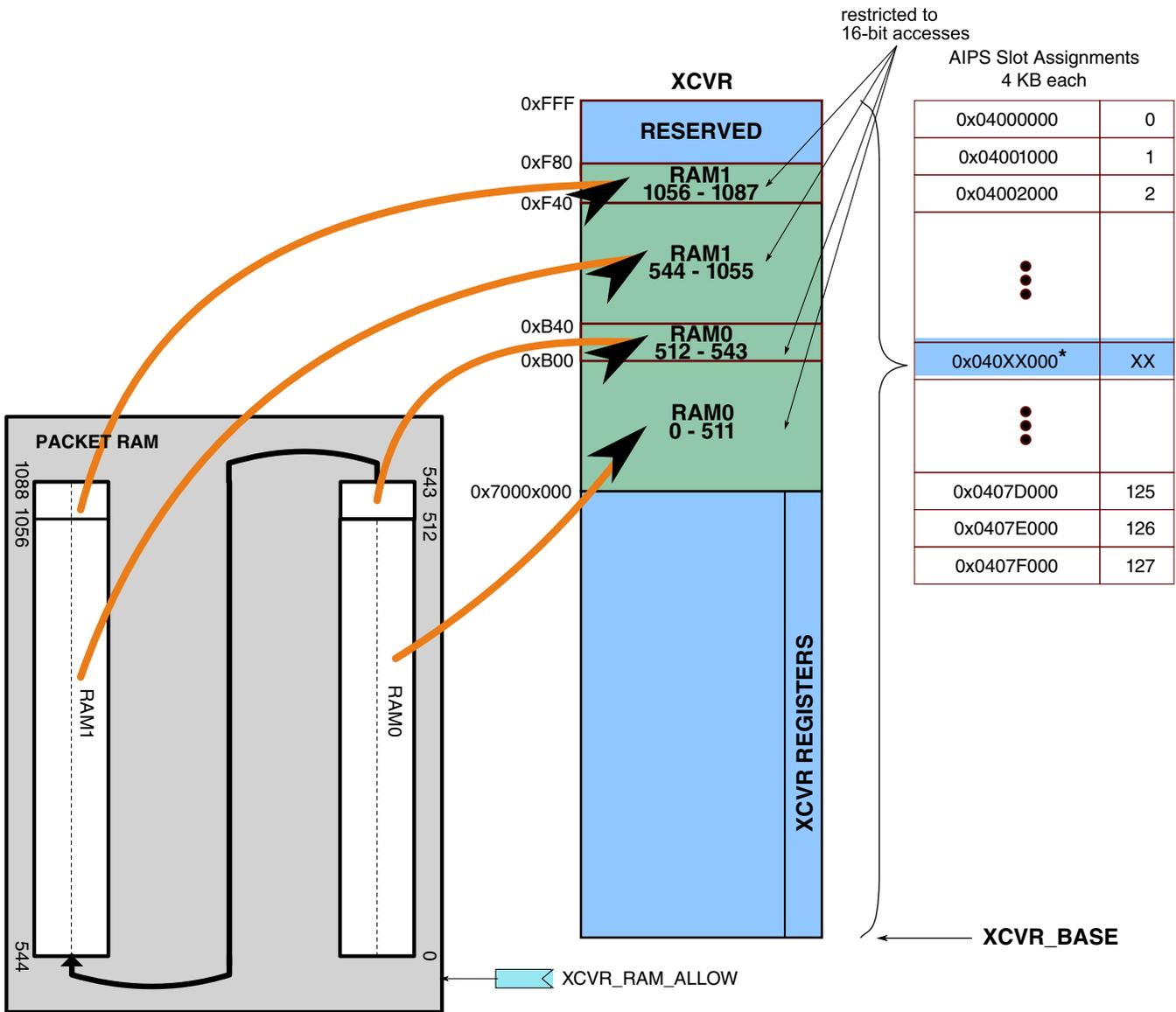
Figure 44-65. Packet RAM Memory Mapping in XCVR Space
