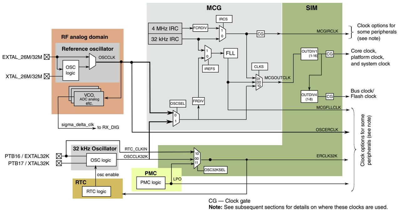
**Figure 5-1. Clocking diagram**
