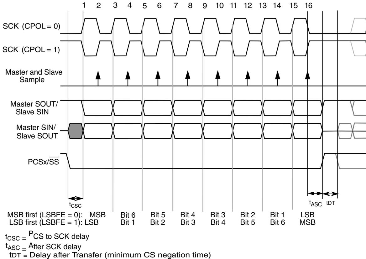
**Figure 36-6. Module transfer timing diagram (MTFE=0, CPHA=1, FMSZ=8)**
