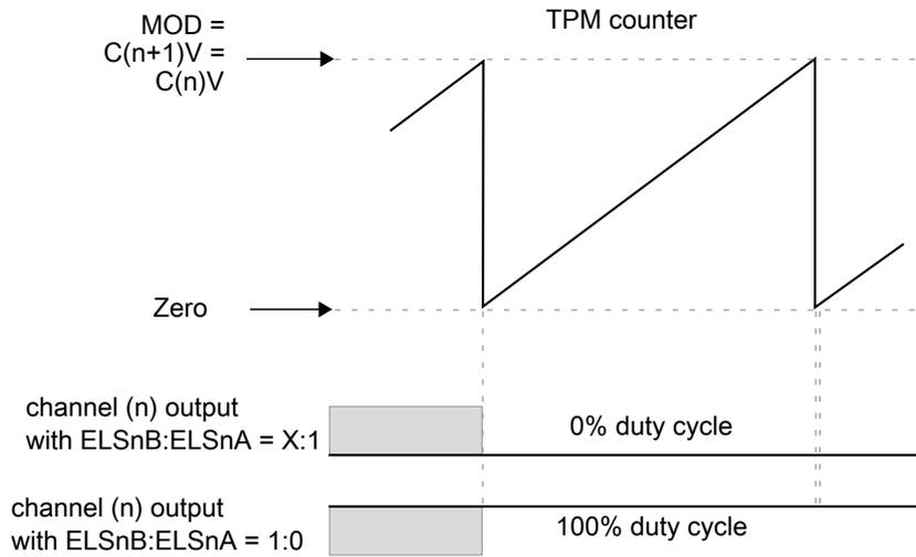
Figure 32-21. Channel (n) output if  $(C(n)V = C(n+1)V = MOD)$
