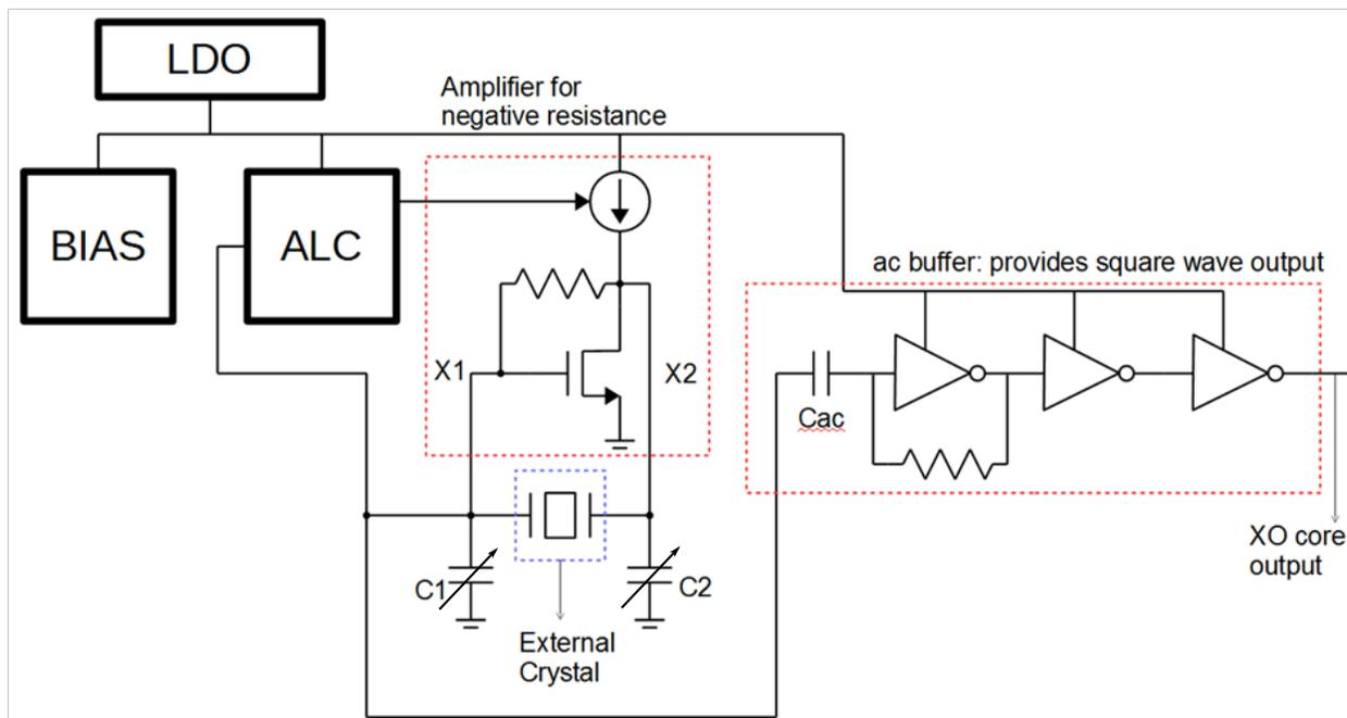
Figure 44-67. XO circuit diagram
