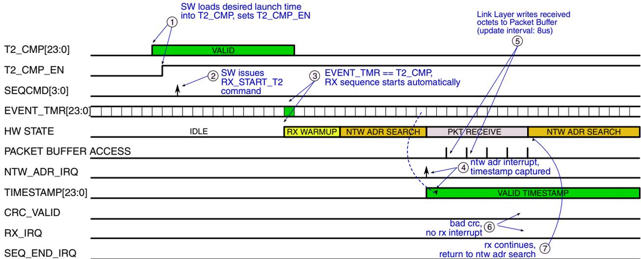
**Figure 44-96. GENERIC FSK RX SEQUENCE: LAUNCH VIA T2 TIMER, BAD PACKET, RX RECYCLE**
