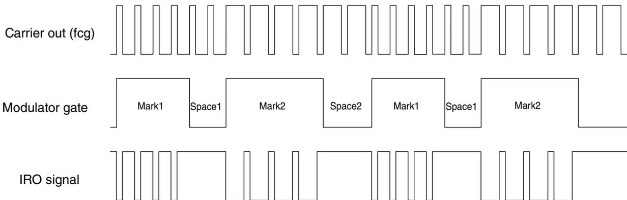
**Figure 39-6. Example: CMT output in FSK mode**
