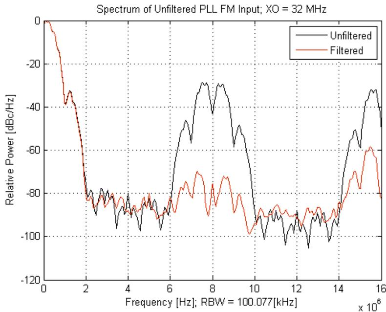
**Figure 44-10. Comparison of Transmit Modulation Images at the PLL Input for BLE**
