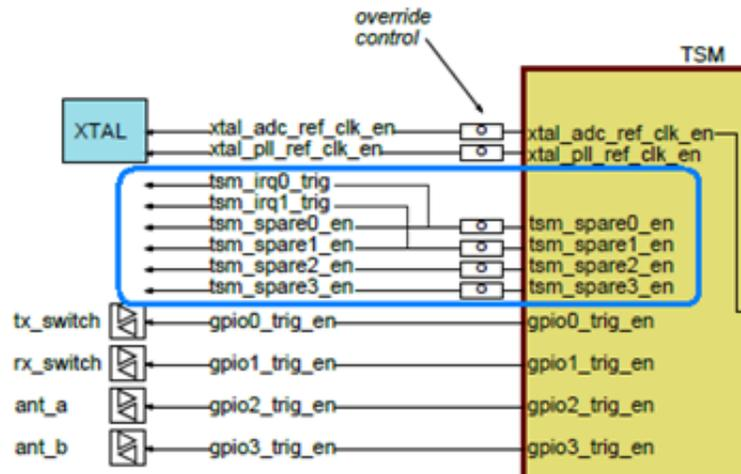
**Figure 44-62. TSM Interrupt Re-use Scheme**
