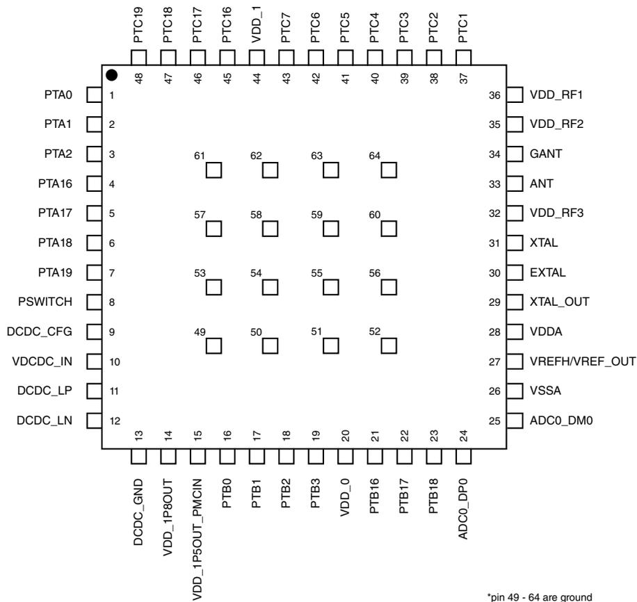
Figure 2-1. 48-pin Laminated QFN pinout diagram
