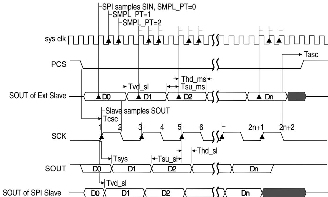
**Figure 36-7. SPI Modified Transfer Format (MTFE=1, CPHA=0,  $f_{\text{sck}} = f_{\text{sys}}/4$ )**
