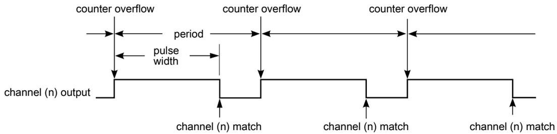
**Figure 32-9. EPWM period and pulse width with  $ELSnB:ELSnA = 1:0$**
