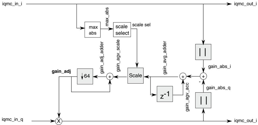
Figure 44-29. I/Q Gain Mismatch Calibration Block Diagram
