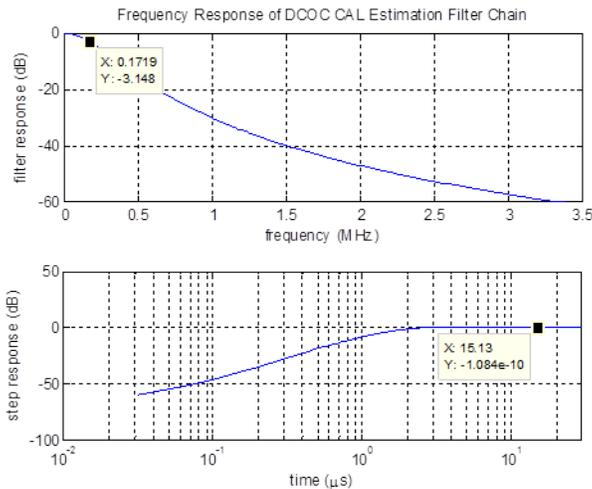
**Figure 44-36. Magnitude and Step response of DC Offset Calibration Estimator**
