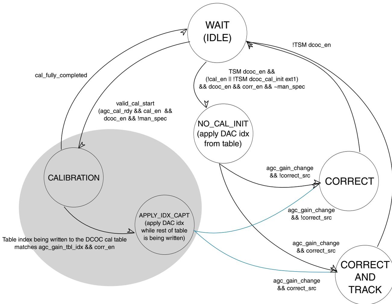
Figure 44-33. DCOC State Diagram
