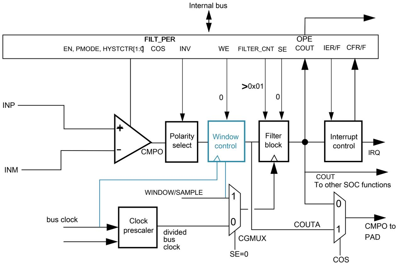
**Figure 29-5. Sampled, Filtered (# 4B): sampling point internally derived**
