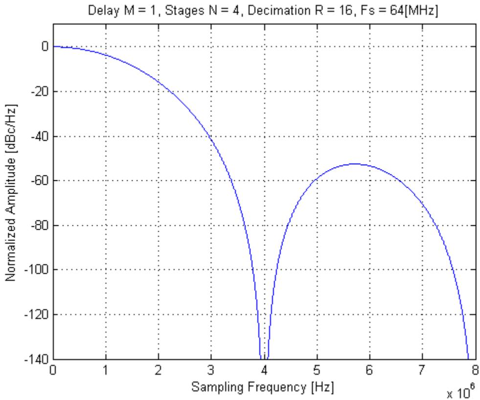
Figure 44-23. 4th order CIC (OSR=16) Decimation Filter Frequency Response
