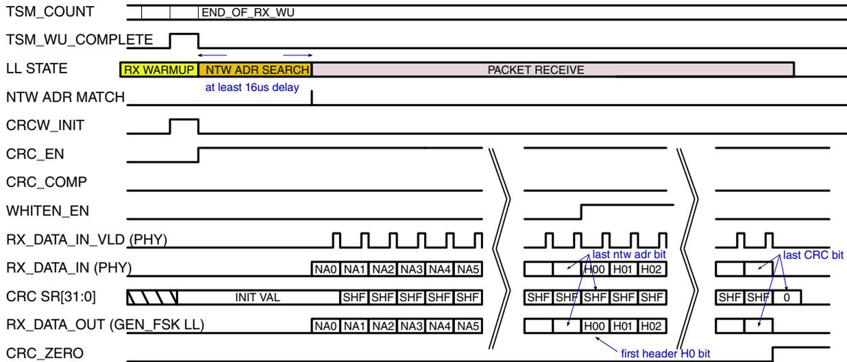
**Figure 44-83. BIT STREAM PROCESSING CRC AND WHITENING RX TIMING**
