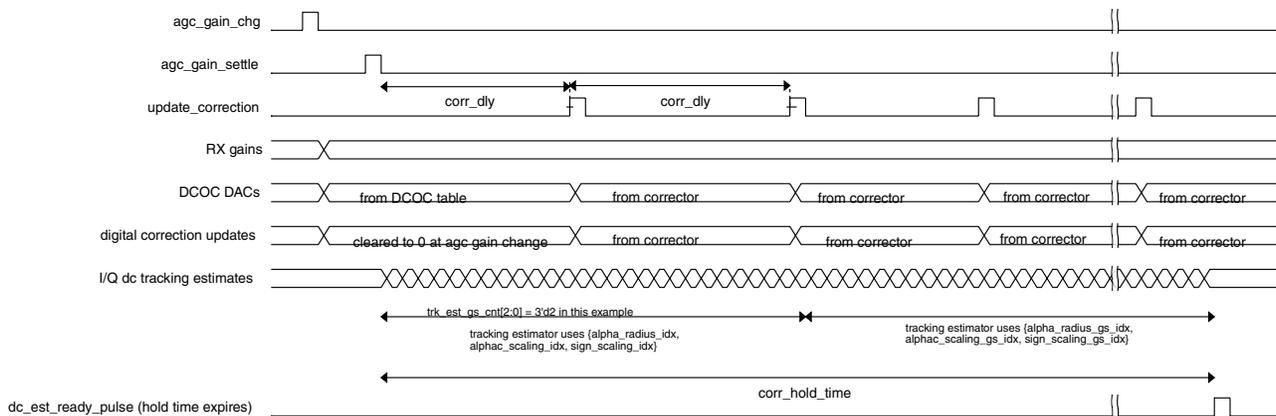
**Figure 44-39. DC Offset Tracking Correction Timing**
