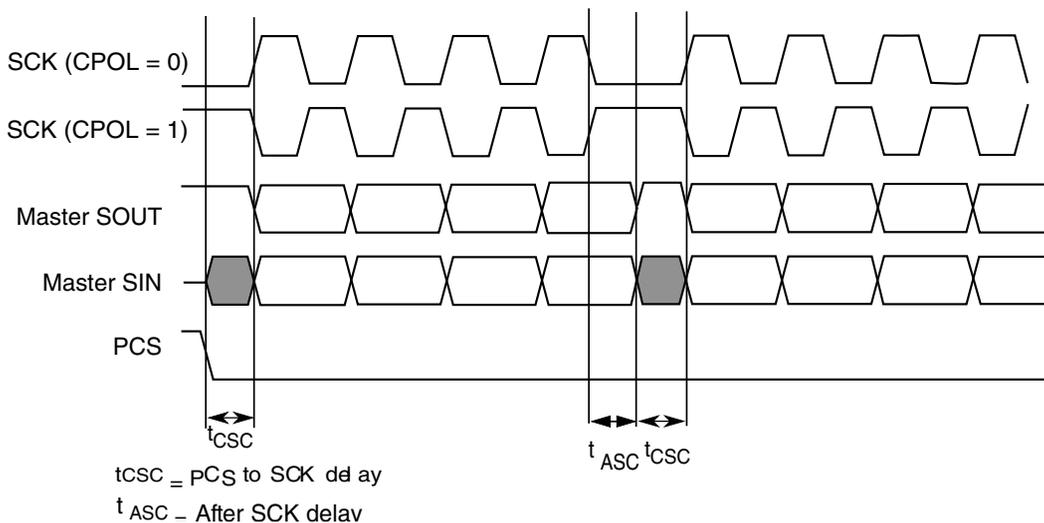
**Figure 36-14. Example of continuous transfer (CPHA=1, CONT=1)**
