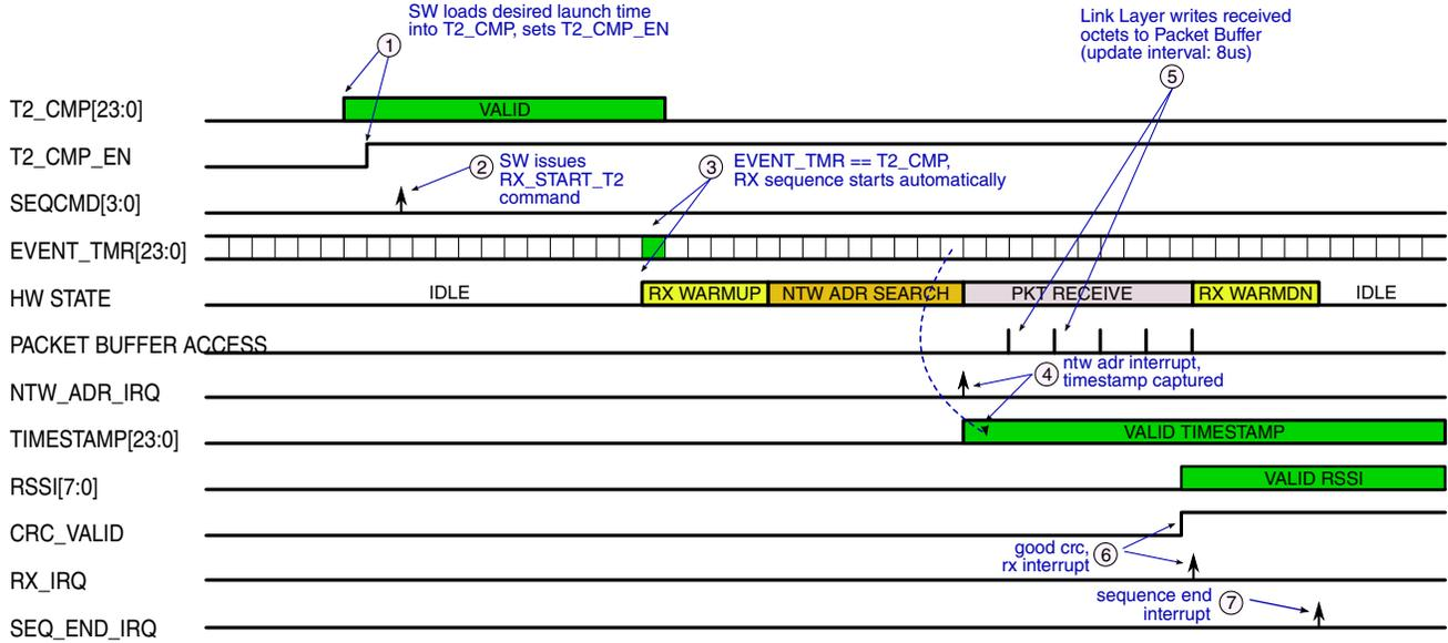
**Figure 44-95. GENERIC FSK RX SEQUENCE: LAUNCH VIA T2 TIMER, GOOD PACKET**
