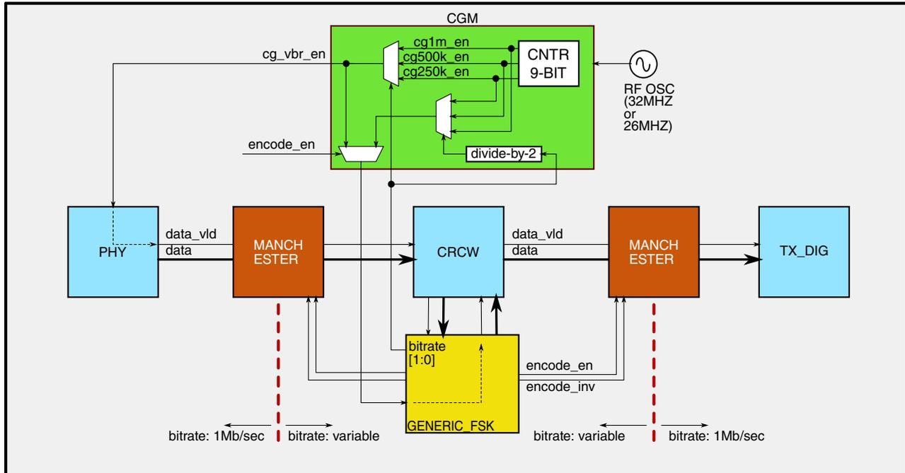
**Figure 44-77. BITSTREAM PROCESSING WITH MANCHESTER ENCODING**
