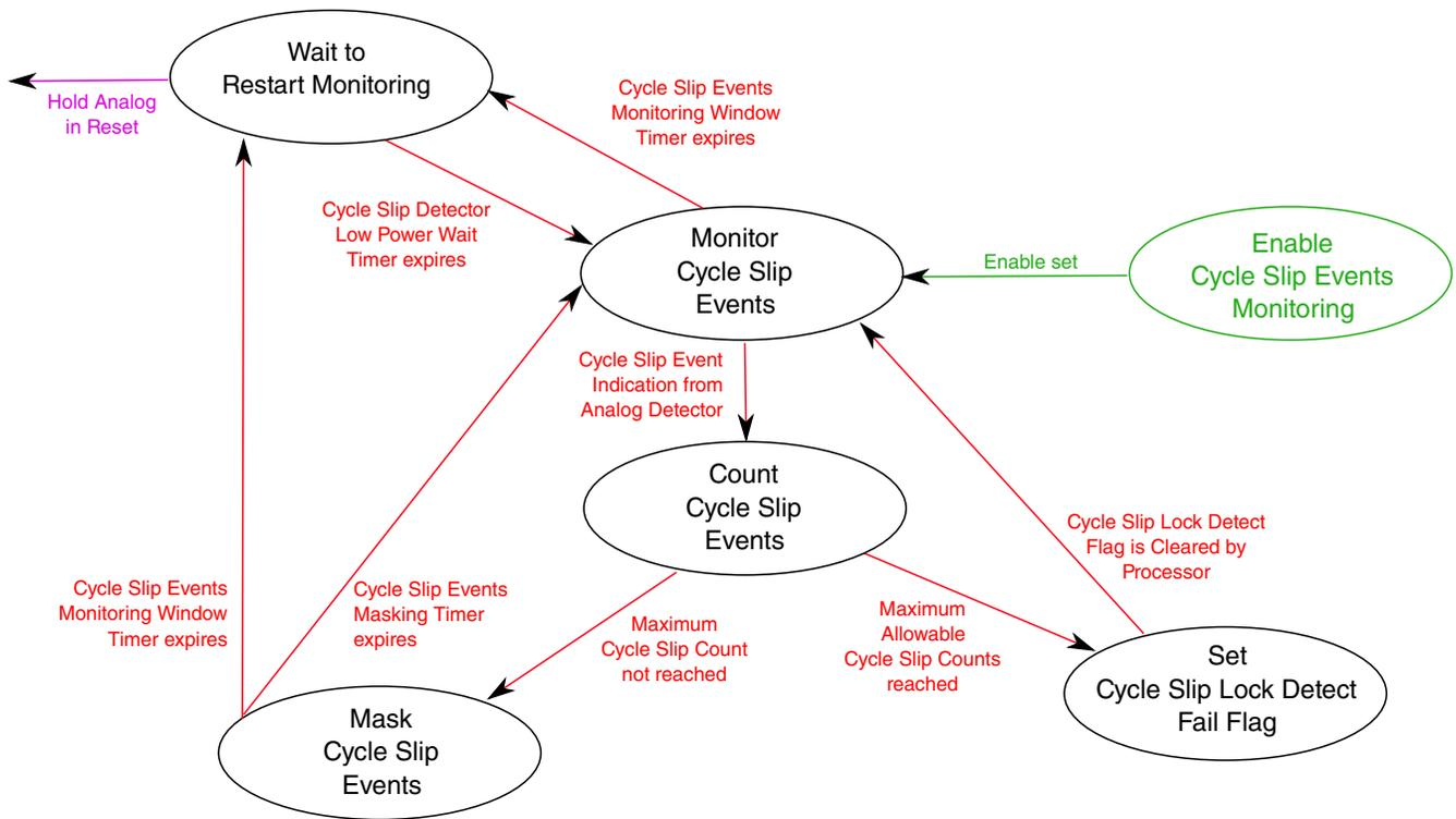
**Figure 44-17. PLL Lock Detect State Machine**
