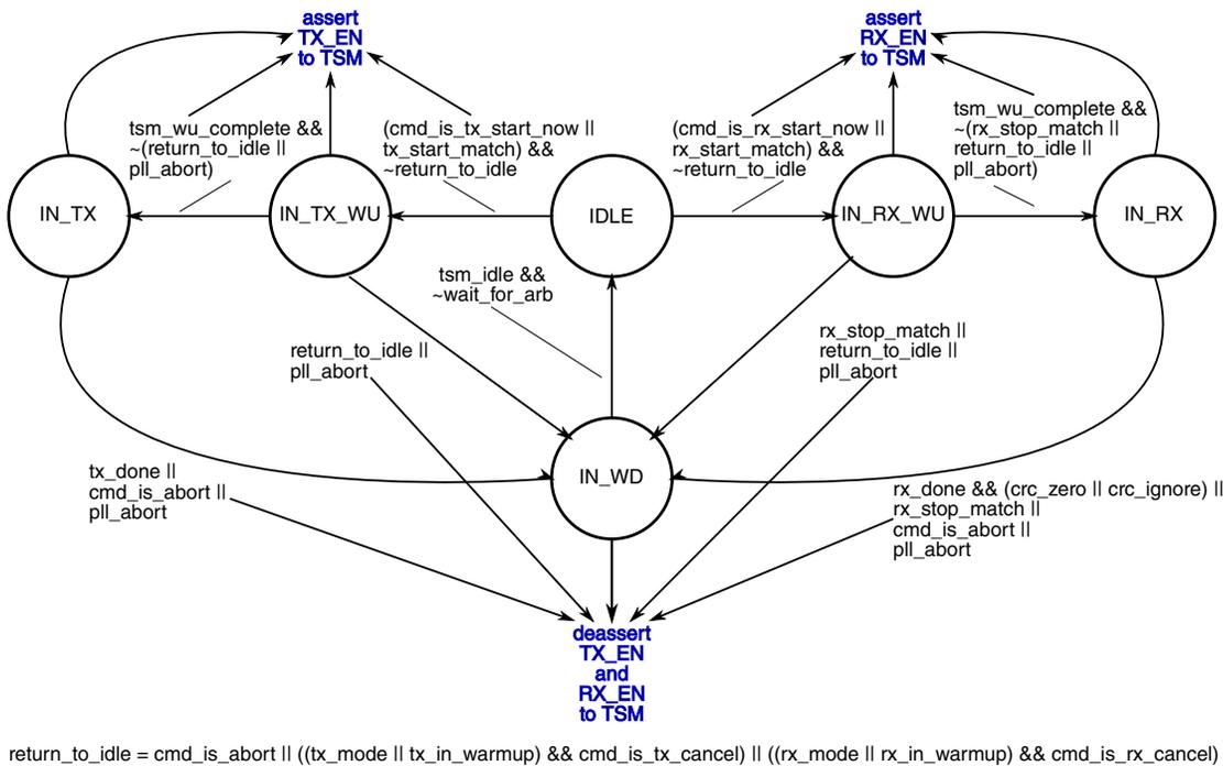
**Figure 44-90. GENERIC COMMAND DECODER FSM**
