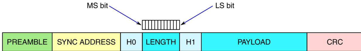
**Figure 44-74. LENGTH Bit Ordering (MSB First)**
