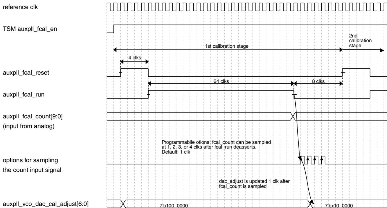
Figure 44-44. RX AuxPLL FCAL timing
