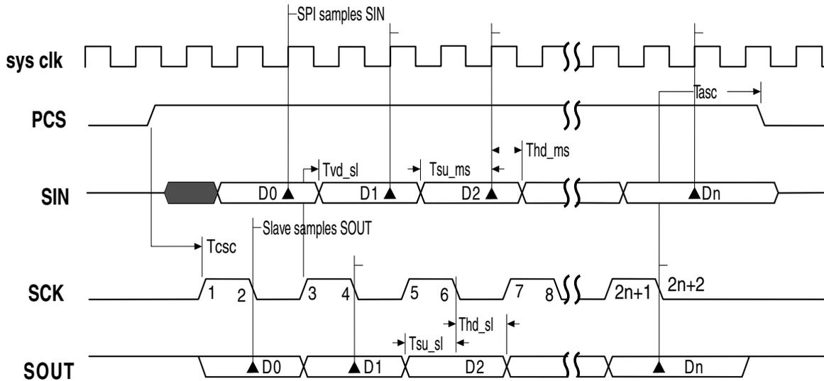
Figure 36-10. SPI Modified Transfer Format (MTFE=1, CPHA=1,  $f_{sck} = f_{sys}/2$ )
