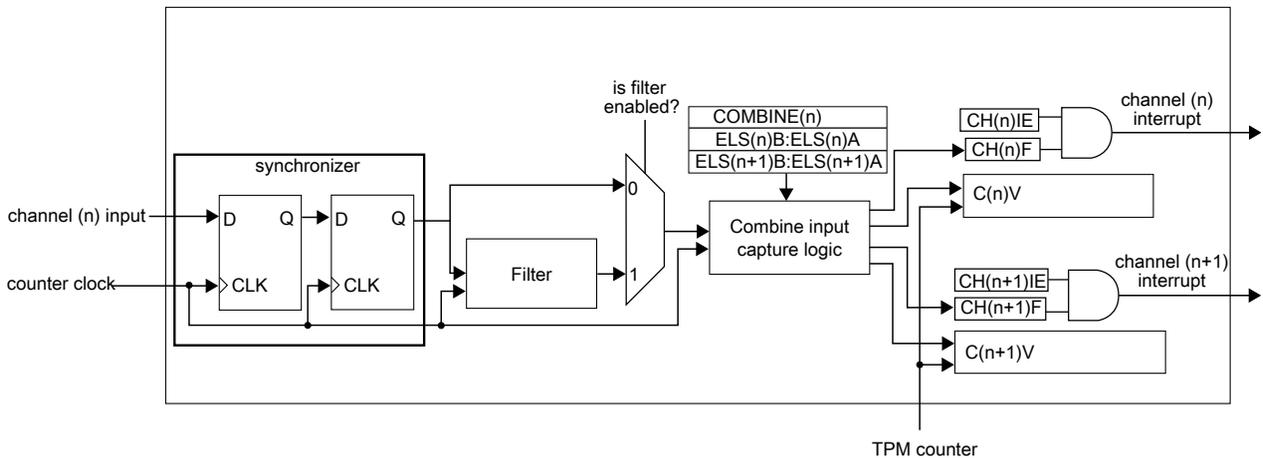
Figure 32-22. Combine Input Capture mode block diagram
