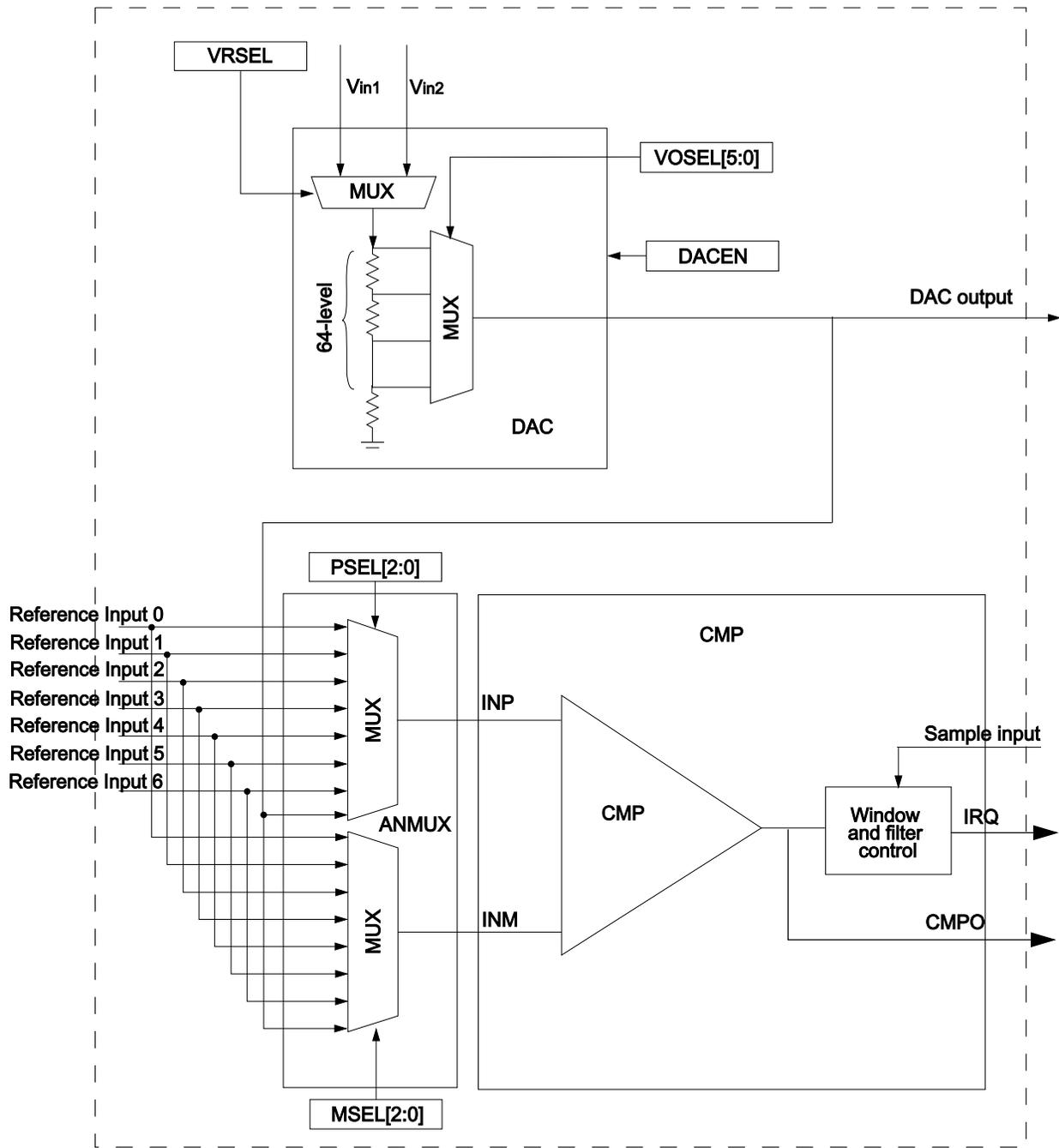
Figure 29-1. CMP, DAC and ANMUX block diagram
