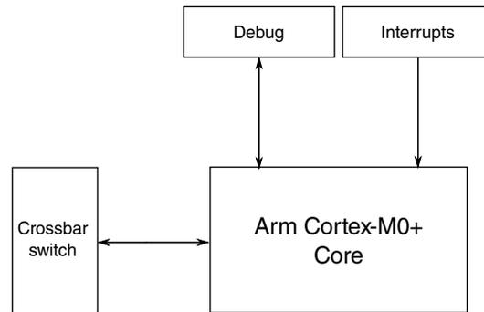
Figure 3-1. Core configuration
