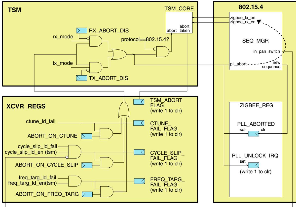
Figure 44-52. 802.15.4 PLL UNLOCK HANDLING
