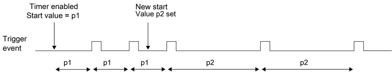
**Figure 33-4. Dynamically setting a new load value**
