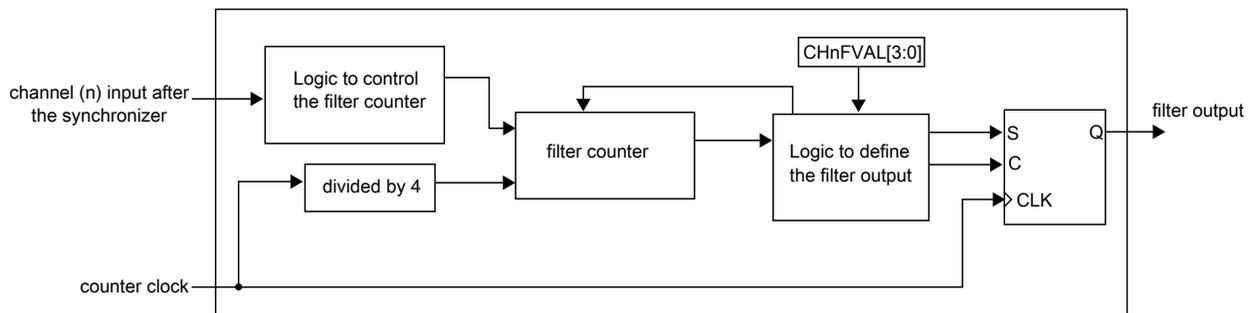
**Figure 32-23. Channel input filter**
