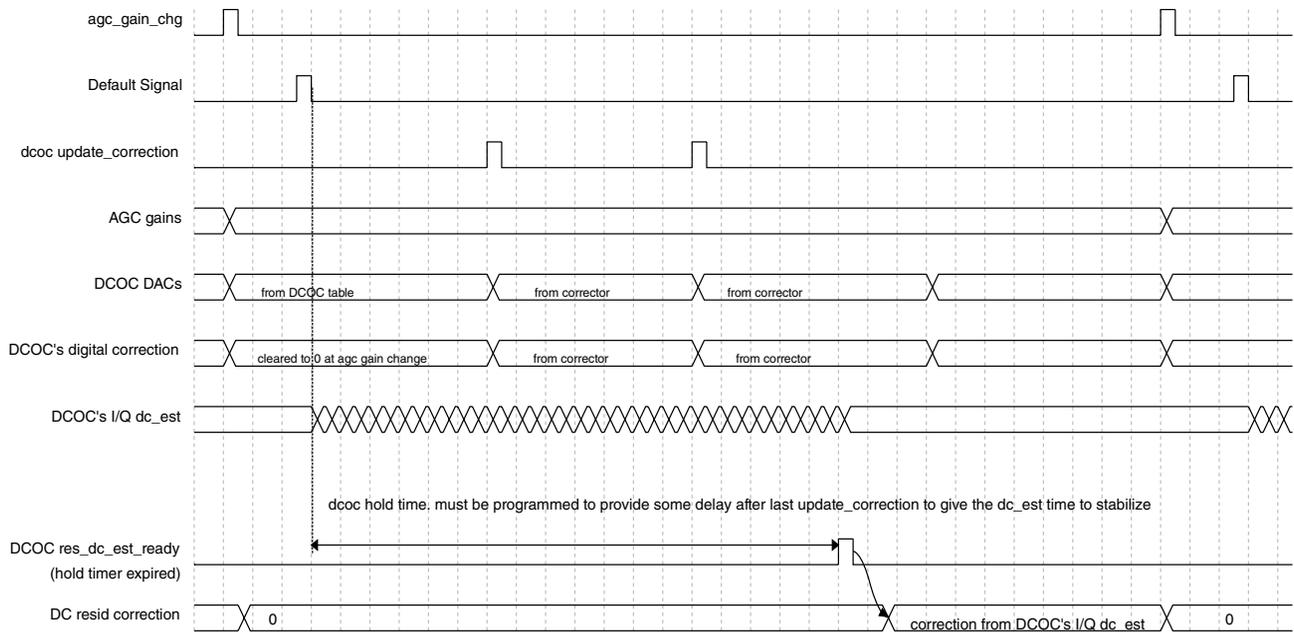
Figure 44-42. DC residual mode 3 timing
