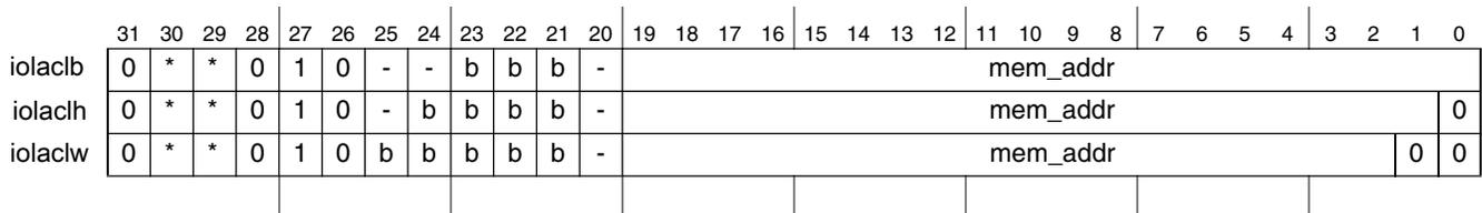
**Figure 17-9. Decorated load address: load-and-clear 1 bit**
