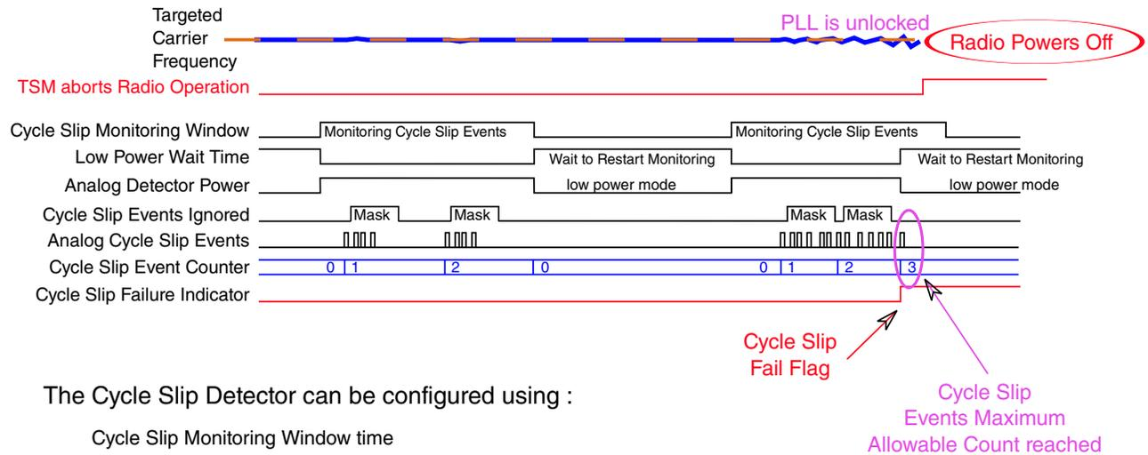
The Cycle Slip Detector can be configured using :
