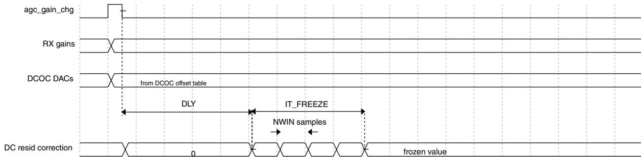
**Figure 44-40. DC residual mode 1 timing**
