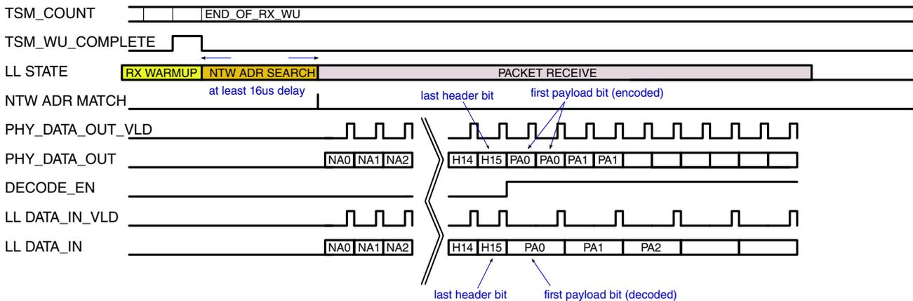
**Figure 44-88. BIT STREAM PROCESSING (WITH MANCHESTER) RX TIMING -- 1MBIT/SEC OTA**
