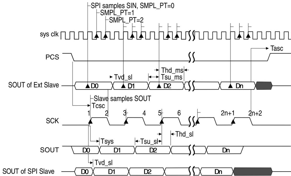
**Figure 36-12. SPI Modified Transfer Format (MTFE=1, CPHA=1,  $f_{sck} = f_{sys}/4$ )**
