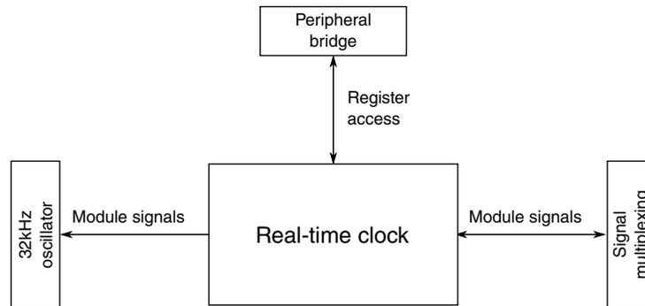
Figure 3-36. RTC configuration
