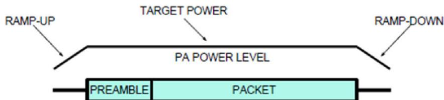
**Figure 44-5. Power Amplifier Ramping**
