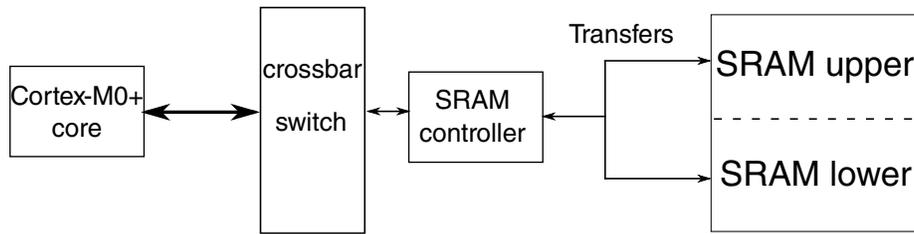
Figure 3-24. SRAM configuration
