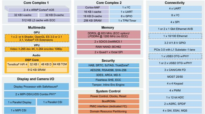
\* Each single PHY can either be a 1× 4 lane MIPI-DSI or a 1×1 channel LVDS interface for a total of 2 display interfaces. In combination, the two PHYs can be configured to be a single 2-channel LVDS interface.
