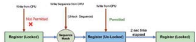
Figure 4 – Write protection sequence
