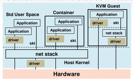
HW devices can be directly accessed by containers, VMs, and processes— not just the host kernel. It means load/store to device, use DMAs, etc.
