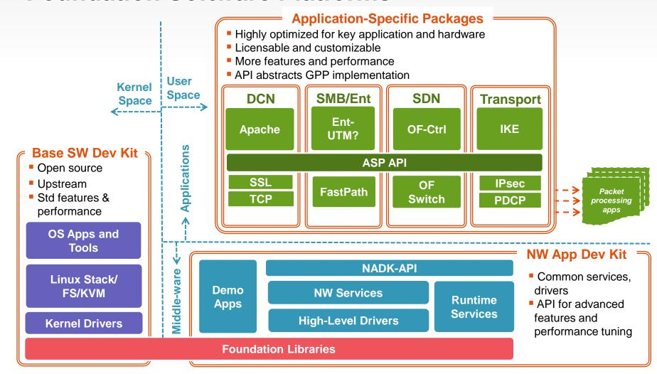
Freescale Platforms—QorlQ processors built on Layerscape architecture
