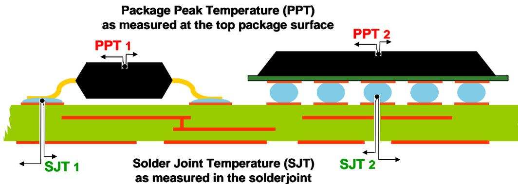
**Figure 1:** Solder Joint Temperature (SJT) and Package Peak Temperature (PPT) have to be determined for critical components on the boards.
