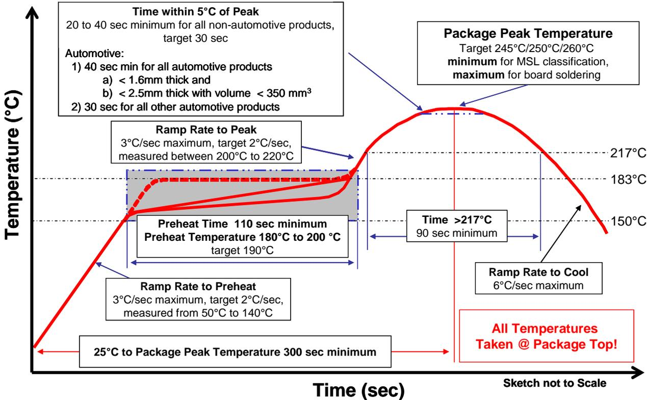
**Figure 2:** Package Peak Temperature (PPT) characterization for determination of components' Moisture Sensitivity Level (MSL) and the parts' processability per J-STD-020 and including customer board soldering requirements. This is not a soldering profile showing the solder joint temperature!
