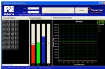
11. The red waveform is the X-axis, the green waveform is the Y-axis, and the blue is the Z-axis data. As you rotate the Tower System at various dimensions, the waveforms will also move up or down. The on-board accelerometer is a Freescale product. Please search “MA7361L” online for the data sheet. The data sheet outlines the corresponding output voltages based on the various orientations.
