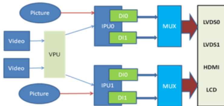
Block Diagram of the IPU DI Port for Multiple Display
