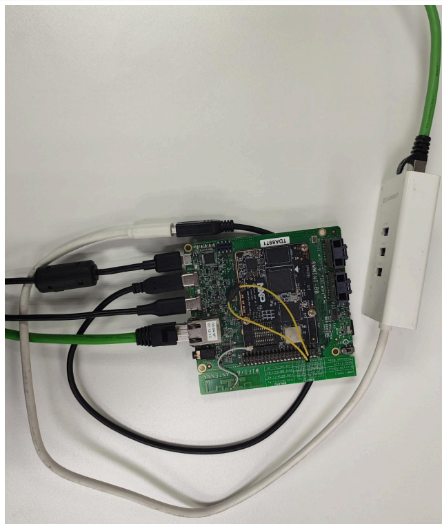
Figure 131. i.MX 8M Mini board connection
