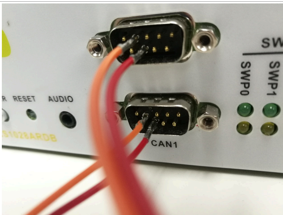
Figure 150. Physical connection for CAN using LS1028ARDB
