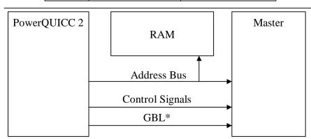
If the asserted address is in a page or block with M=1, the GBL\* signal is asserted. This notifies other masters to snoop their data cache(s). If the page or block has M=0, GBL\* is not asserted.
