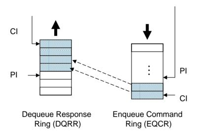
► Each entry in the TX ring (EQCR) can contain a DCA for the corresponding entry on the RX (DQRR) ring
