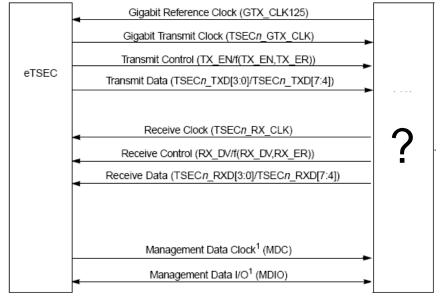
The management signals (MDC and MDIO) are common to all of the gigabit Ethernet controllers module connections in the system, assuming that each PHY has a different management address.
