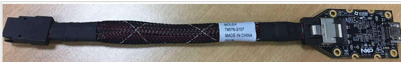
Figure 8. i.MX mini SAS cable with DSI-to-HDMI adapter
