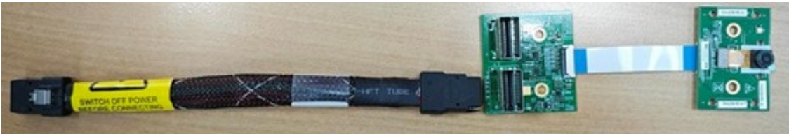
Figure 55. i.MX CSI MIPI Camera AP1302
