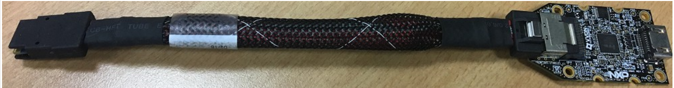
Figure 15. i.MX mini SAS cable with LVDS-to-HDMI adapter
