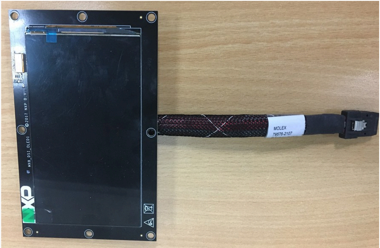
Figure 40. MX8-DSI-OLED1 MIPI panel
