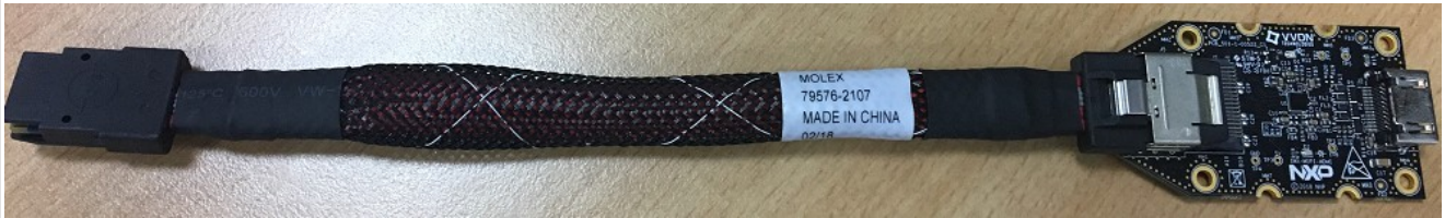
Figure 3. i.MX Mini SAS cable with DSI-to-HDMI adapter
