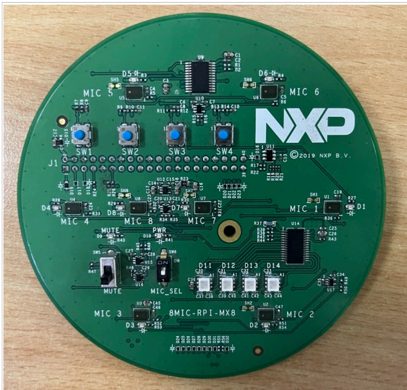
Figure 11. i.MX 8MIC PDM Microphone board
