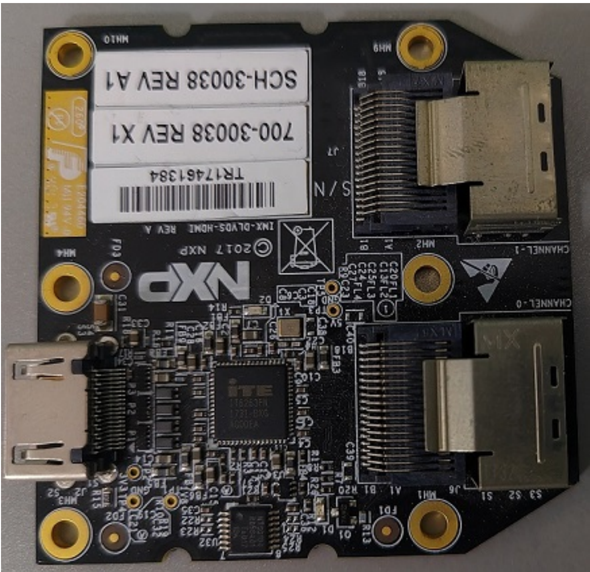
Figure 18. i.MX dual-channel LVDS-to-HDMI adapter
