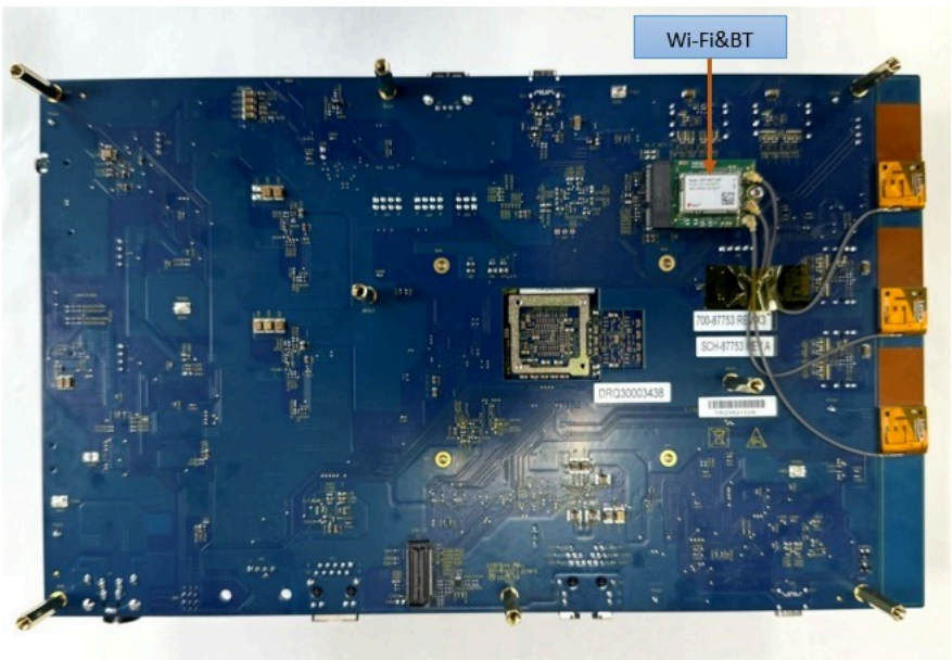
Figure 49. i.MX 95 EVK board back view
