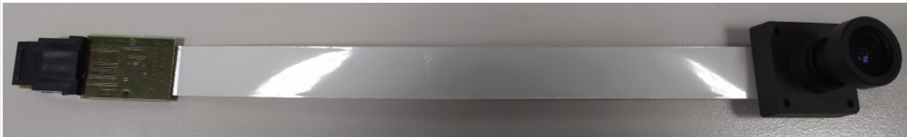
Figure 20. Basler CSI MIPI camera
