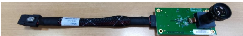
Figure 21. OS08A20 CSI MIPI camera
