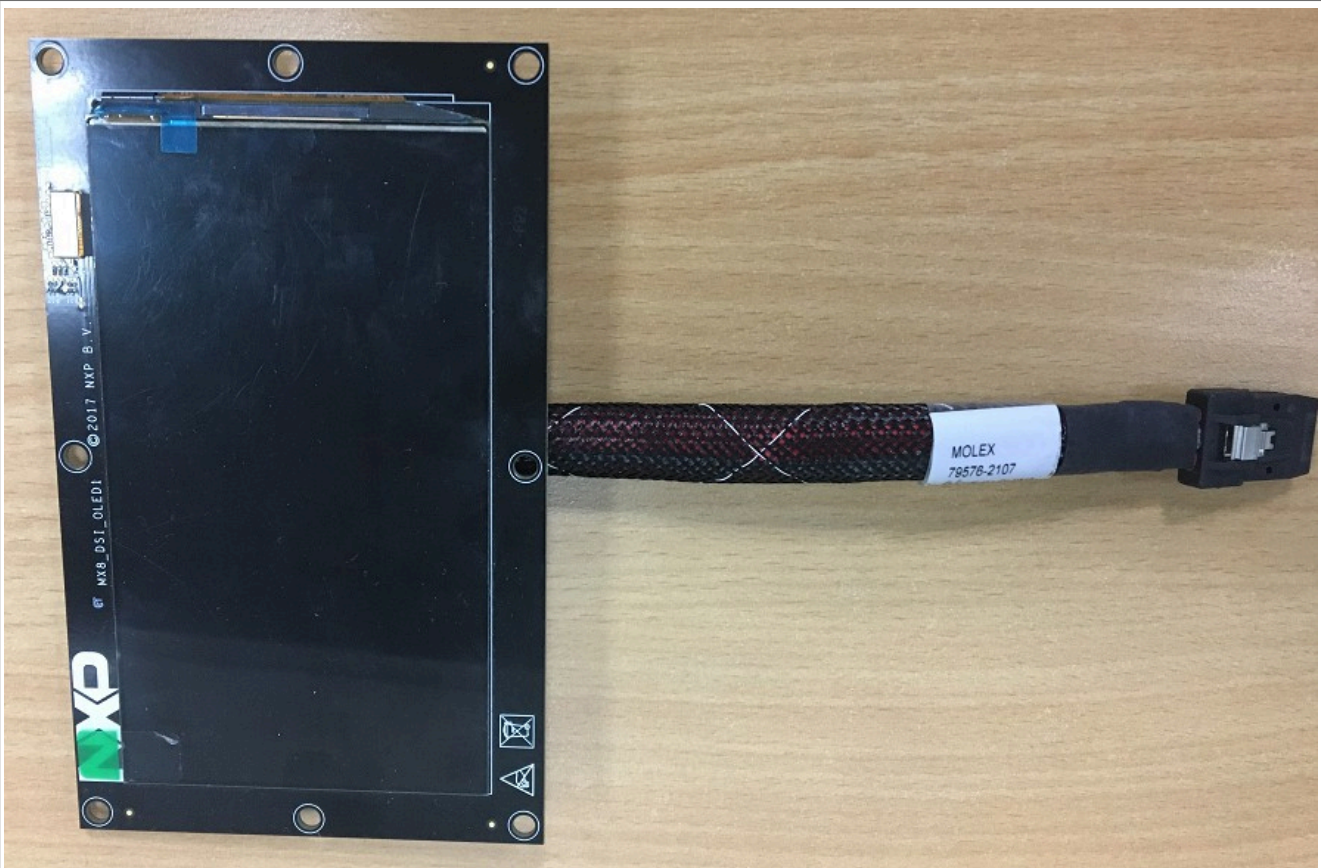
Figure 9. MX8-DSI-OLED1 MIPI panel
