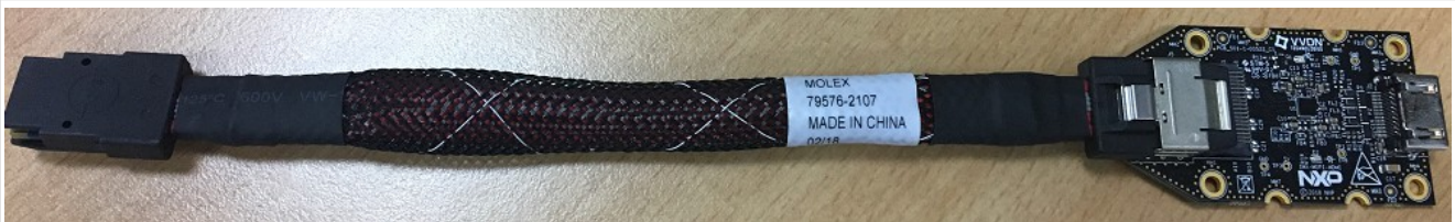
Figure 38. i.MX mini SAS cable with DSI-to-HDMI adapter
