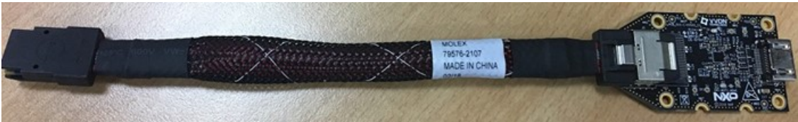
Figure 50. i.MX mini SAS cable with DSI-to-HDMI adapter
