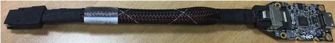
Figure 51. i.MX mini SAS cable with LVDS-to-HDMI adapter
