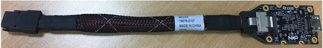
Figure 44. i.MX mini SAS cable with DSI-to-HDMI adapter
