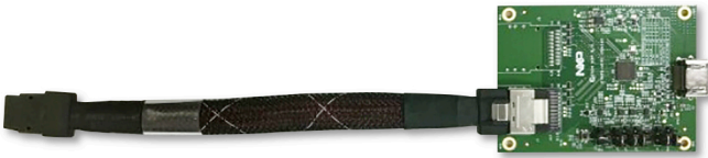
Figure 56. i.MX mini SAS cable with DSI-to-HDMI4K adapter
