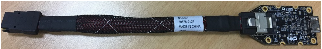
Figure 43. i.MX mini SAS cable with DSI-to-HDMI adapter
