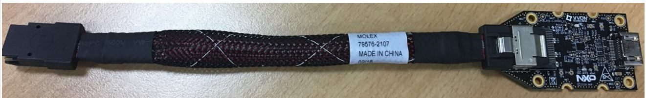
Figure 26. i.MX mini SAS cable with DSI-to-HDMI adapter
