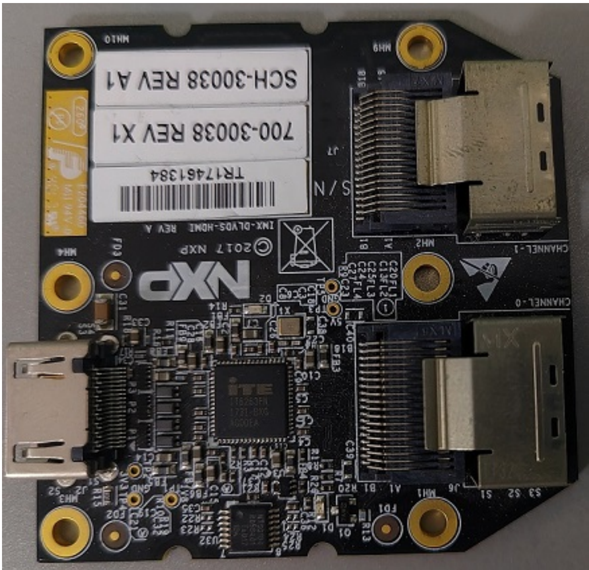
Figure 18. i.MX dual-channel LVDS-to-HDMI adapter
