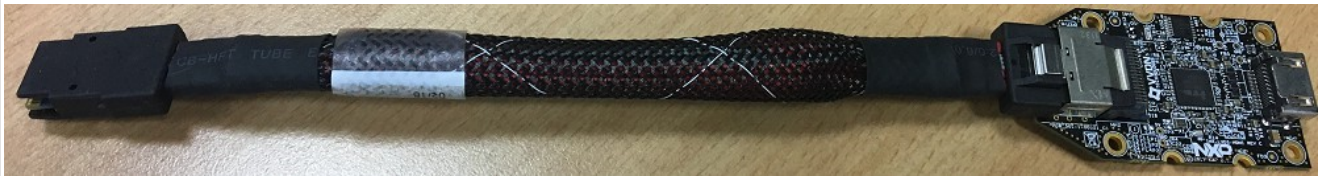
Figure 15. i.MX mini SAS cable with LVDS-to-HDMI adapter
