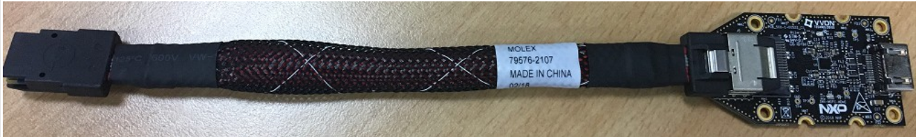
Figure 37. i.MX mini SAS cable with DSI-to-HDMI adapter
