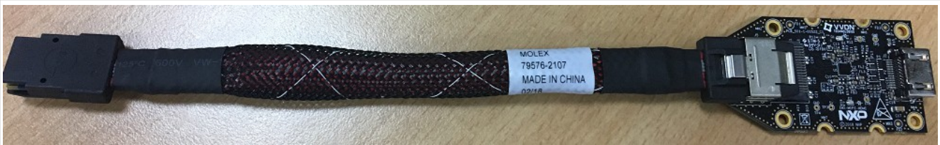
Figure 14. i.MX mini SAS cable with DSI-to-HDMI adapter
