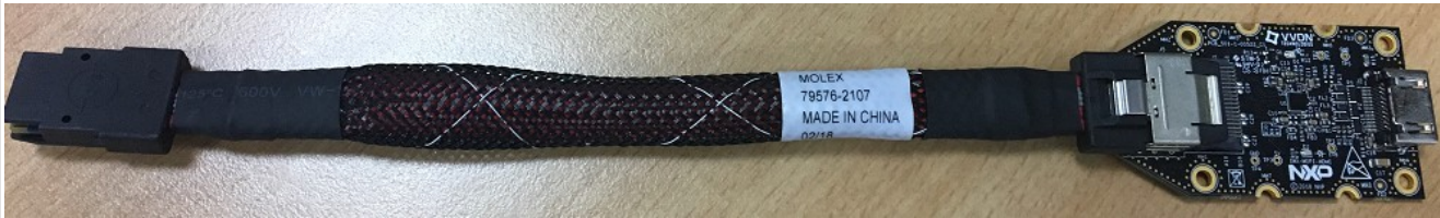
Figure 3. i.MX Mini SAS cable with DSI-to-HDMI adapter
