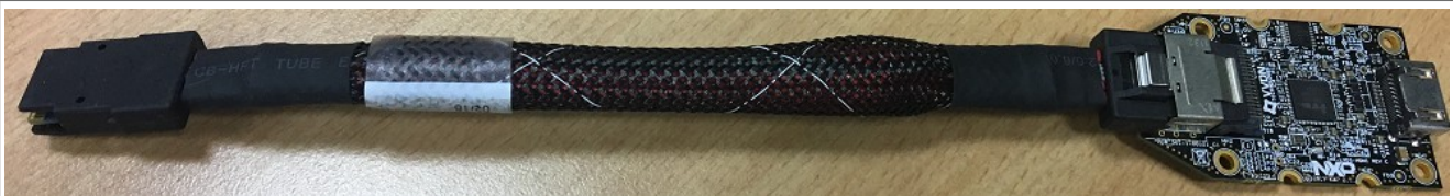
Figure 44. i.MX mini SAS cable with LVDS-to-HDMI adapter
