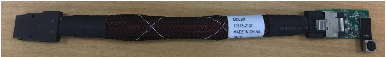
Figure 33. i.MX CSI MIPI camera
