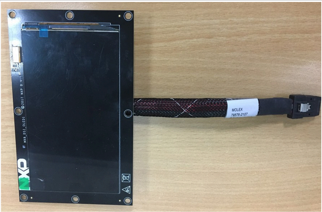
Figure 16. MX8-DSI-OLED1 MIPI panel
