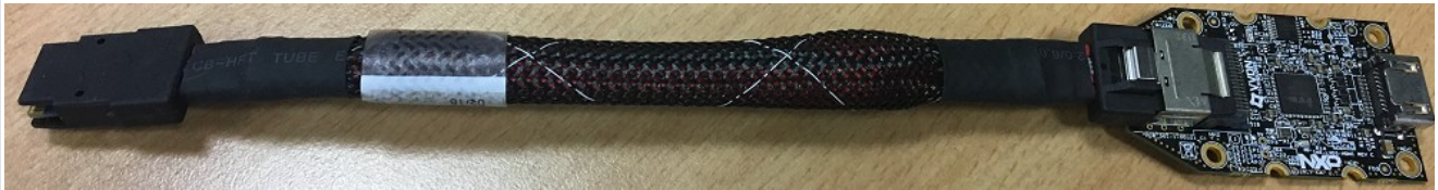
Figure 38. i.MX mini SAS cable with LVDS-to-HDMI adapter
