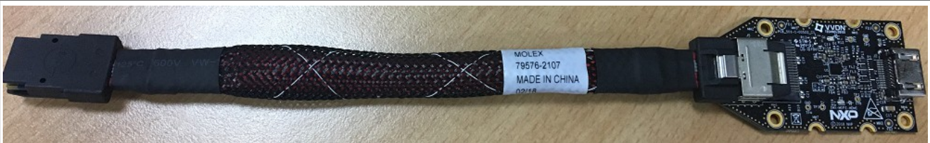
Figure 8. i.MX mini SAS cable with DSI-to-HDMI adapter
