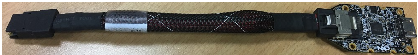
Figure 3. i.MX mini SAS cable with LVDS-to-HDMI adapter
