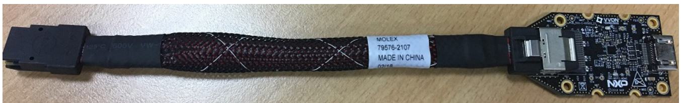
Figure 3. i.MX mini SAS cable with DSI-to-HDMI adapter
