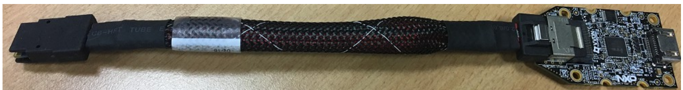
Figure 4. i.MX mini SAS cable with LVDS-to-HDMI adapter
