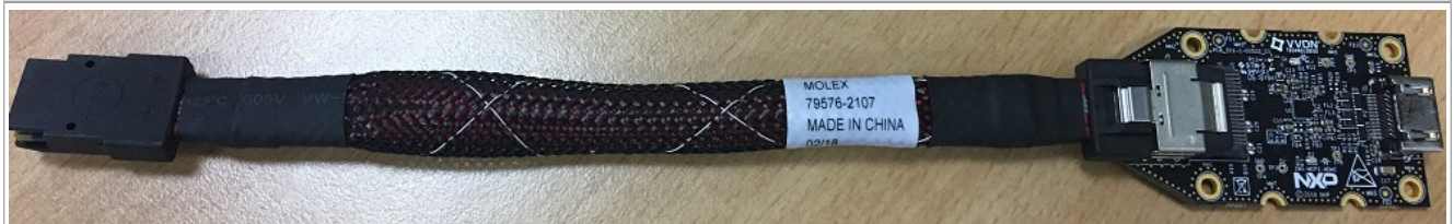
Figure 3. i.MX mini SAS cable with DSI-to-HDMI adapter
