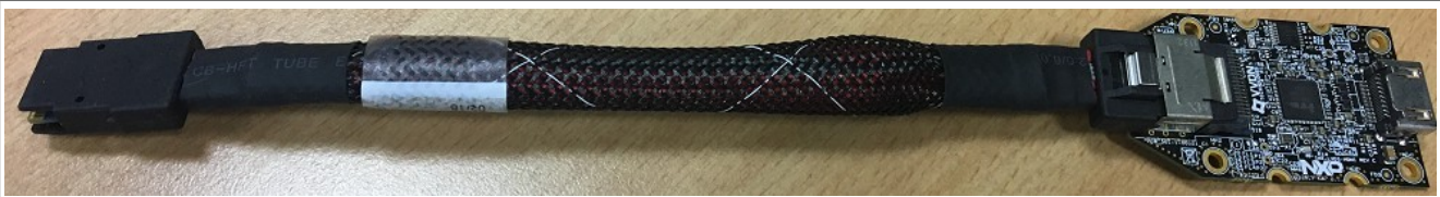
Figure 4. i.MX mini SAS cable with LVDS-to-HDMI adapter
