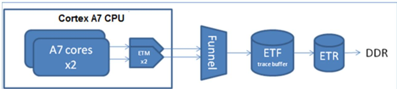
The UI Platform Configurator configures the ARMv7 cores Embedded Trace Macrocell (ETM), Funnel, Embedded Trace FIFO (ETF), and Embedded Trace Router (ETR) modules. The ETF stores and forwards trace data using a dedicated RAM buffer. This reduces trace loss by absorbing spikes in trace data. The ETR redirects trace to the system bus for collection from alternative channels. For ARMv7, it is DDR memory.
