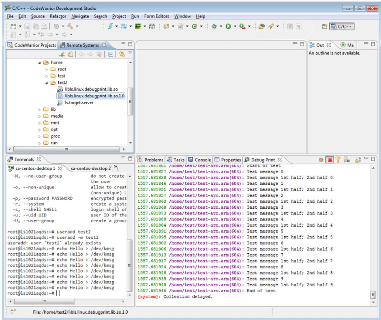
3. The dynamic library cross-compiled for ARM is located in CodeWarrior directory at: `[CWInstallDir]/CW_ARMv7/ARMv7/sa_ls/linux.armv7.debugprint/lib`, which needs to be copied on the target. This library must be loaded by the Linux loader before the C runtime, when you are running the user space applications that need to be monitored by setting the environment variable, `LD_PRELOAD`.
