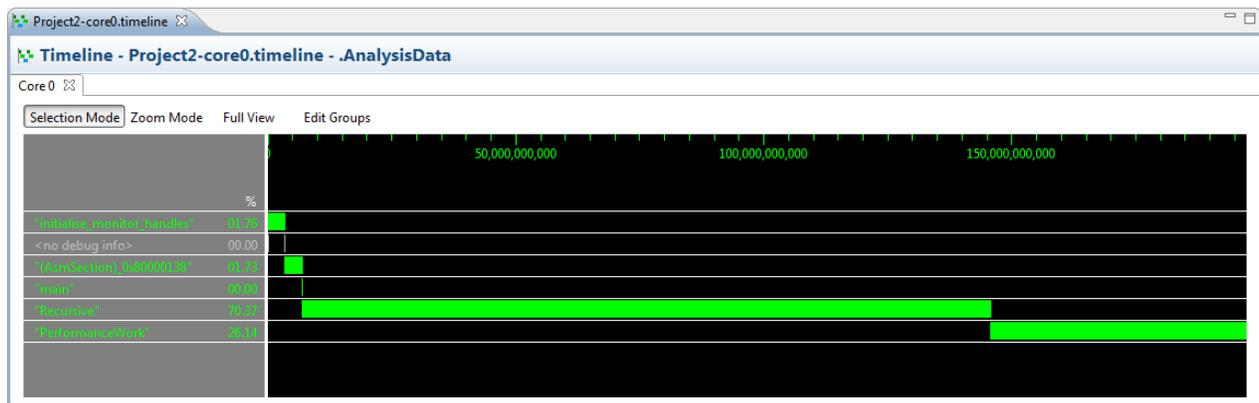
The **Timeline** viewer shows a timeline graph in which the functions appear on y-axis and the number of cycles appear on x-axis. The green-colored bars show the time and cycles that the function takes.
