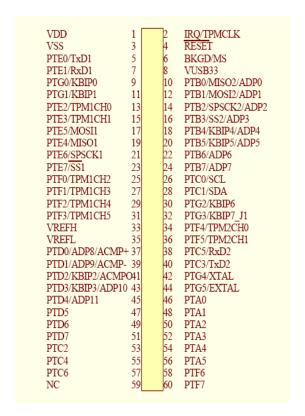
Figure 2-2: MCU Port Connector Pinout
