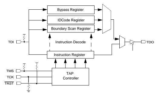
Figure 14-1. Test Access Port (TAP) Block Diagram
