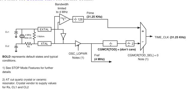
Figure 6-3. Using an External Crystal
