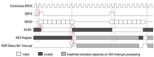
Figure 11-20. Normal Mode Receive Timing—Continuous Clock (WL=8 bit words, DC=1)
