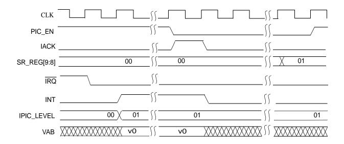
Figure 8-24. Interrupt Handshake Timing
