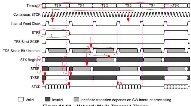
Figure 11-22. Network Mode Transmit Timing
