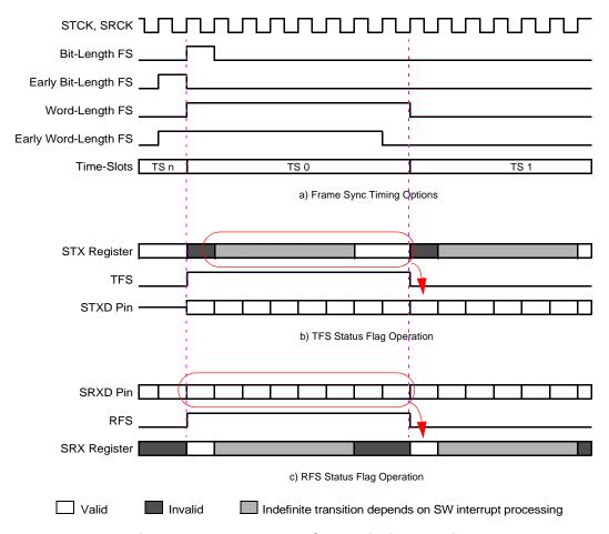
Figure 11-14. Frame Sync Timing Options
