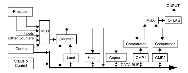
Figure 12-1. TMR Module Block Diagram
