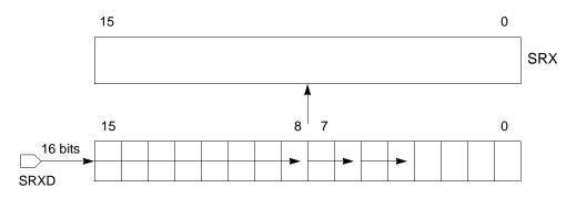
Figure 11-10. Receive Data Path (RSHFD=1)
