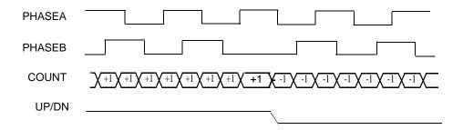
Figure 12-2. Quadrature Incremental Position Encoder
