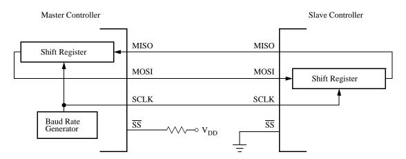
Figure 10-3. Full-Duplex Master/Slave Connections
