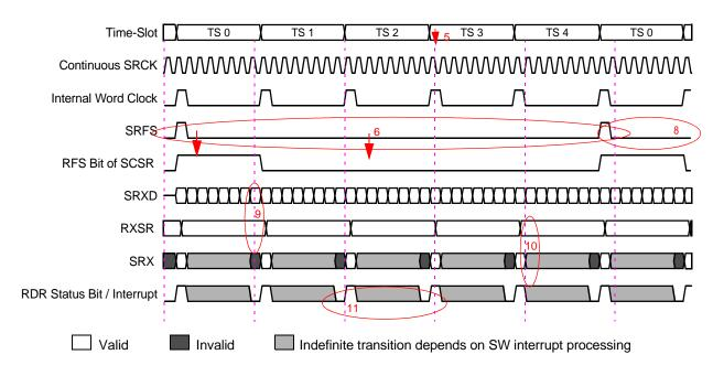
Figure 11-23. Network Mode Receive Timing
