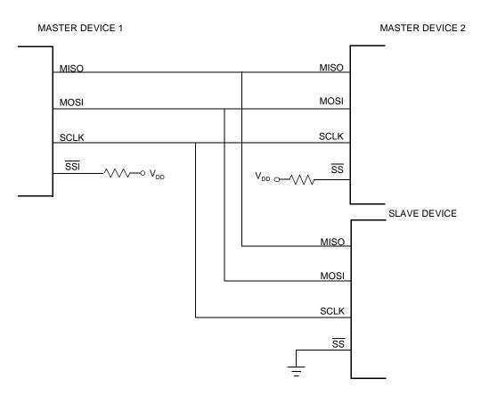
Figure 10-4. Sharing of a Slave by Multiple Masters
