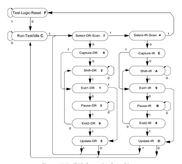
Figure 14-7. TAP Controller State Diagram
