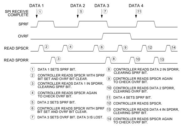
Figure 10-11. Clearing SPRF When OVRF Interrupt Is Not Enabled
