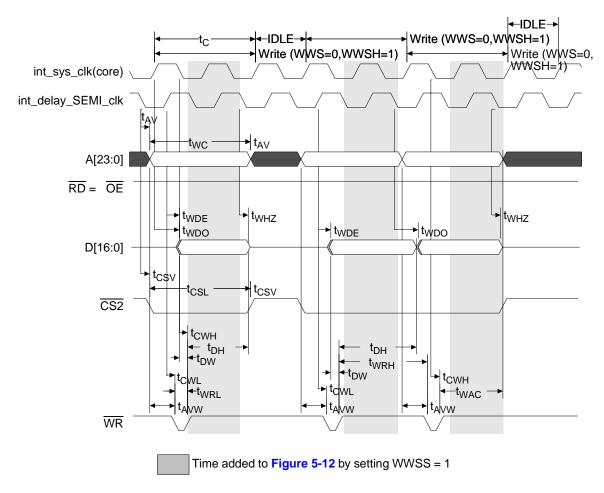
Figure 5-15. External Write Cycle with WWS = 0, WWSH = 1, WWSS = 0
