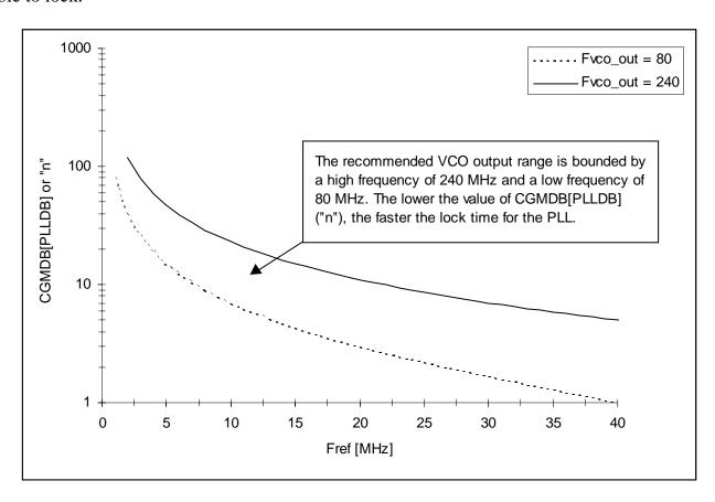
Figure 6-7. PLL Output Frequency vs. Input Frequency
