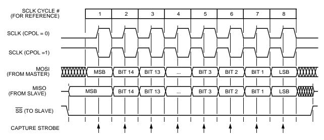
Figure 10-5. Transmission Format (CPHA = 0)
