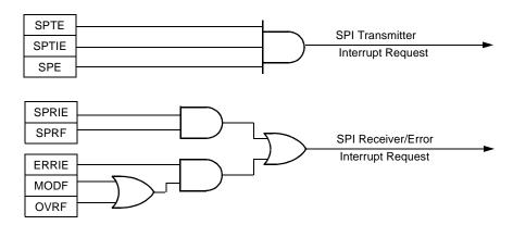
Figure 10-17. SPI Interrupt Request Generation
