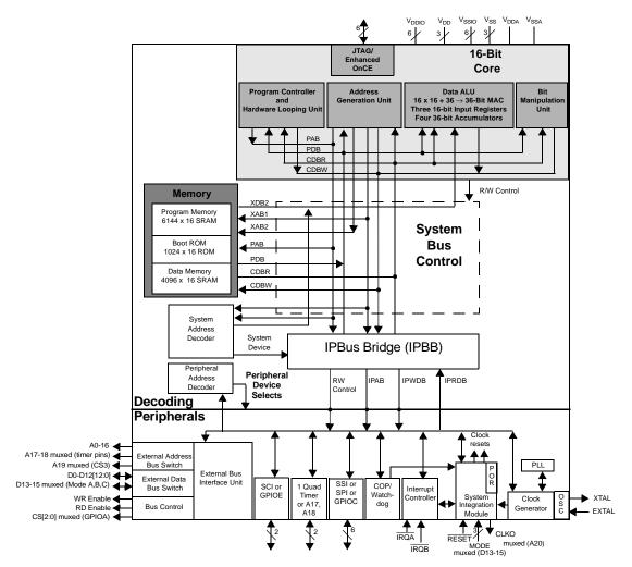
Figure 1-3. 56852 Functional Block Diagram
