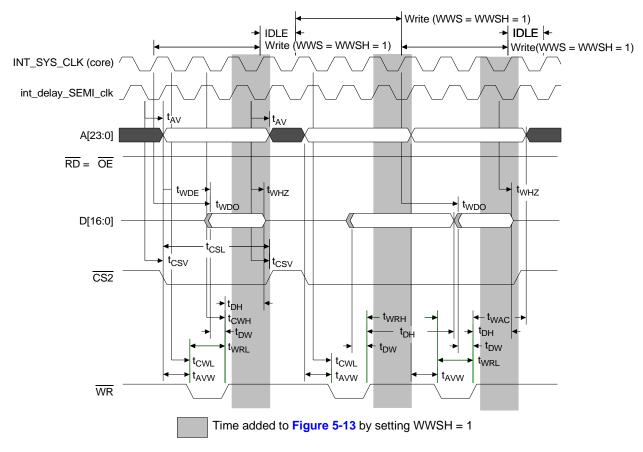
Figure 5-17. External Write Cycle with WWS = WWSH = 1 (WWSS = 0)
