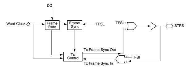
Figure 11-28. ISSI Transmit Frame Sync Generator Block Diagram
