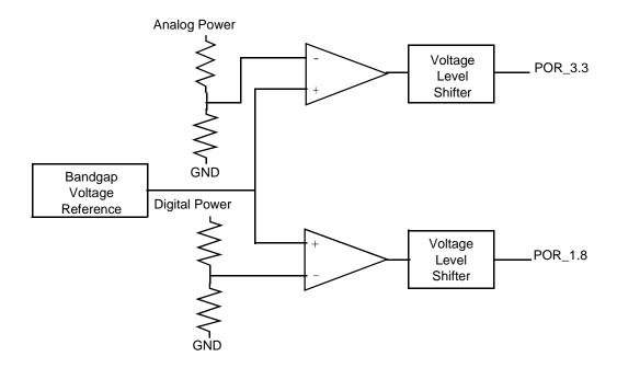
Figure 7-1. POR Module Block Diagram
