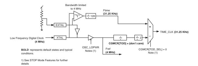
Figure 6-4. Using an External Active Low Frequency Clock, < 4MHz
