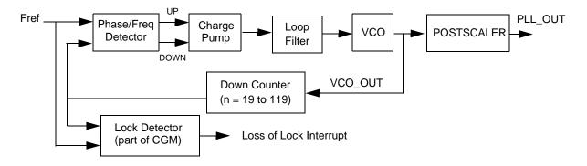
Figure 6-6. PLL Block Diagram
