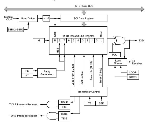
Figure 9-3. SCI Transmitter Block Diagram
