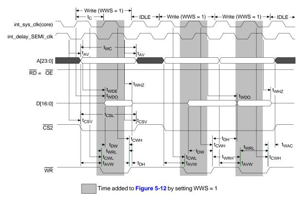
Figure 5-13. External Write Cycle with WWS = 1, WWSH = 0, and WWSS = 0
