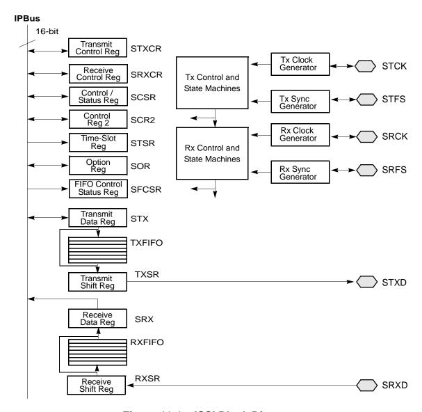
Figure 11-1. ISSI Block Diagram
