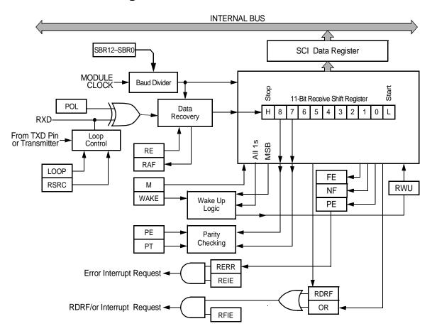
Figure 9-4. SCI Receiver Block Diagram
