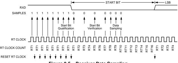
Figure 9-5. Receiver Data Sampling
