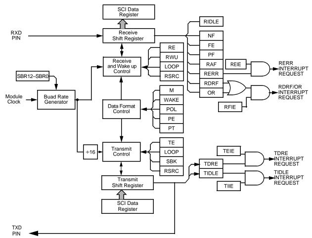
Figure 9-1. SCI Block Diagram
