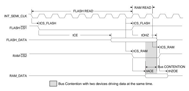
Figure 5-6. Data Bus Contention Timing Requiring MDAR Field Assertion
