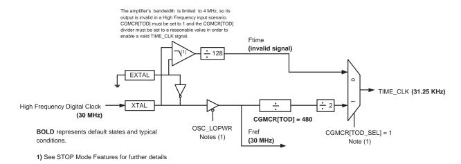
Figure 6-5. Using an External Active High Frequency Clock, > 4MHz
