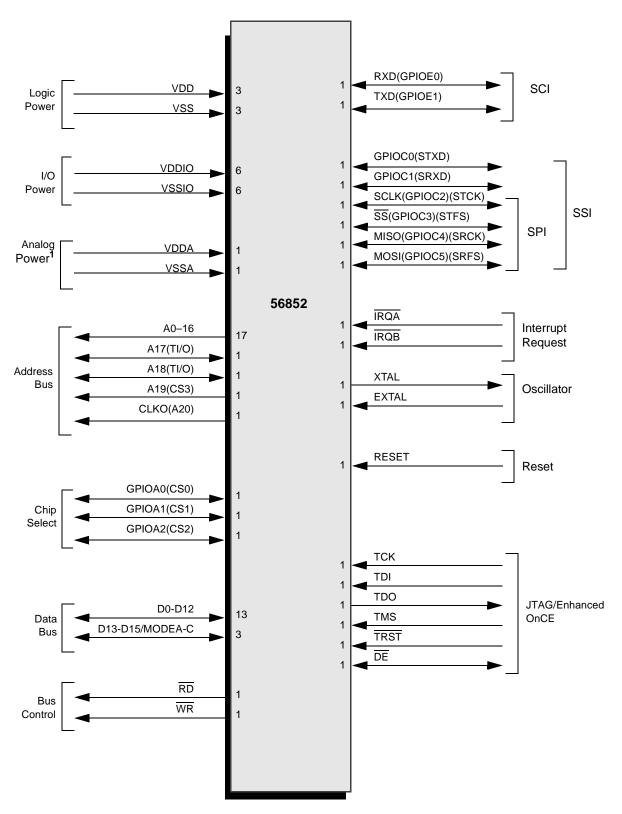
Figure 2-1. 56852 Signals Identified by Functional Group
