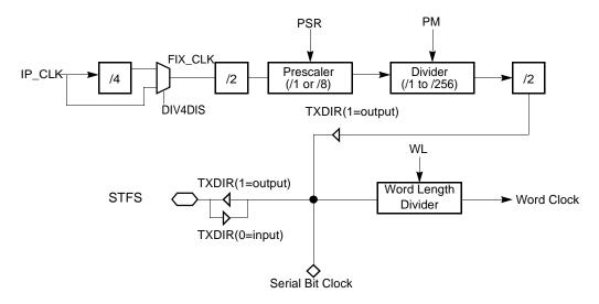
Figure 11-27. ISSI Transmit Clock Generator Block Diagram
