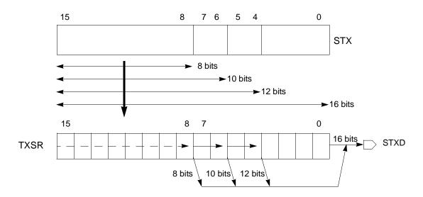
Figure 11-7. Transmit Data Path (TSHFD = 1)
