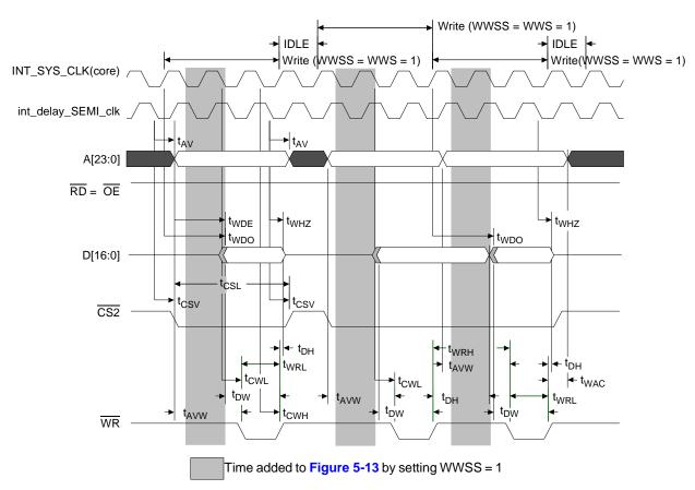
Figure 5-16. External Write Cycle with WWSS = WWS = 1 and WWSH = 0
