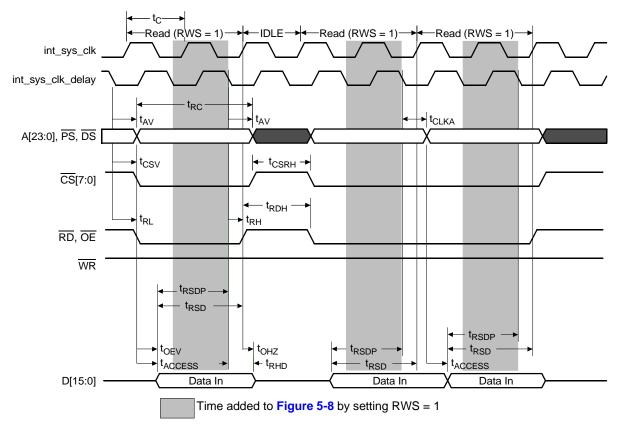
Figure 5-9. External Read Cycle with RWS = 1, RWSH = 0 and RWSS = 0
