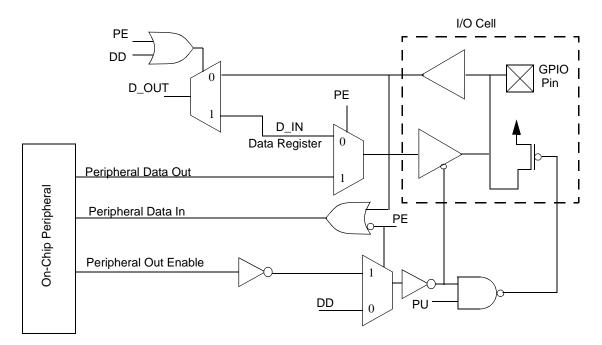
Figure 13-1. Bit-Slice View of GPIO Logic
