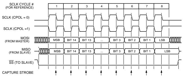
Figure 10-7. Transmission Format (CPHA = 1)
