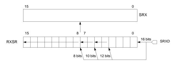
Figure 11-9. Receive Data Path (RSHFD=0)
