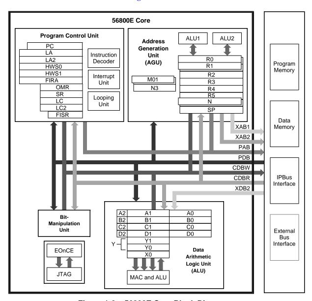
Figure 1-2. 56800E Core Block Diagram
