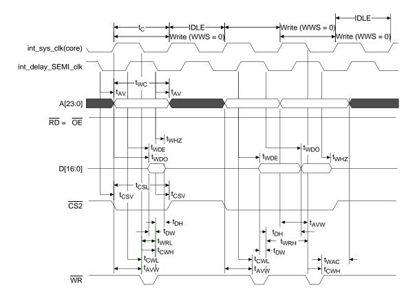
Figure 5-12. External Write Cycle
