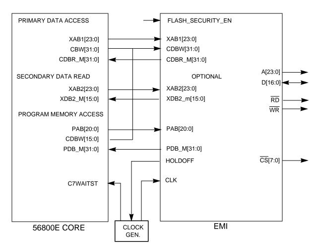
Figure 5-1. EMI Block Diagram
