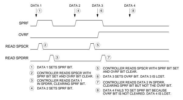
Figure 10-10. Missed Read of Overflow Condition
