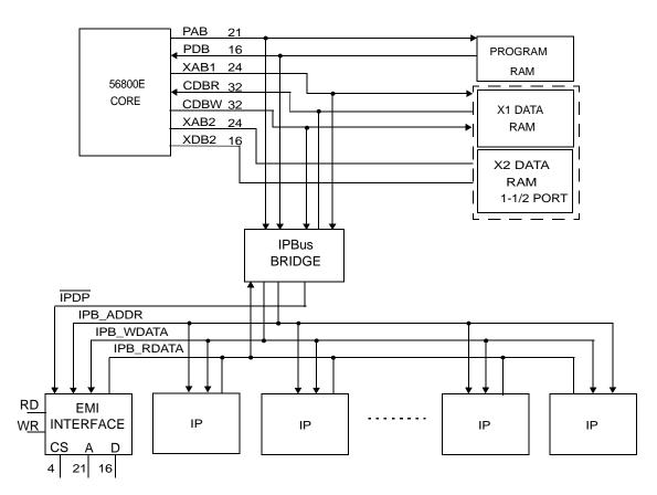
Figure 1-1. IPBus Bridge Interface With Other Main Components
