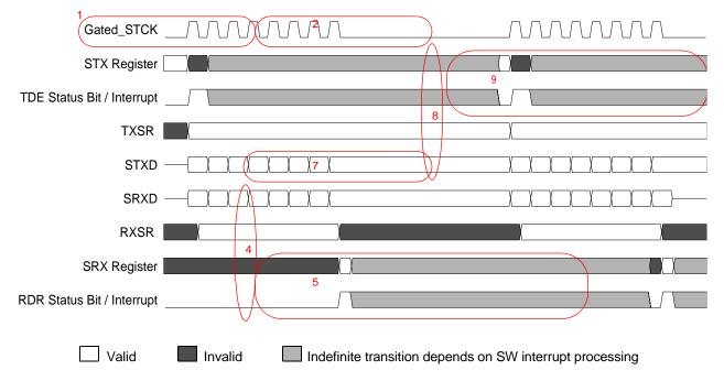
Figure 11-21. Normal Mode Timing—Gated Clock
