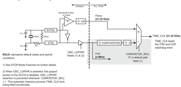
Figure 6-2. OSC Supplying Clocks to PLL/CGM
