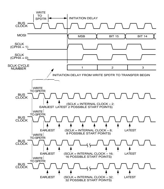
Figure 10-8. Transmission Start Delay (Master)
