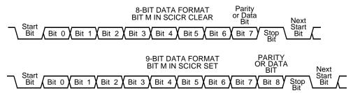
Figure 9-2. SCI Data Frame Formats
