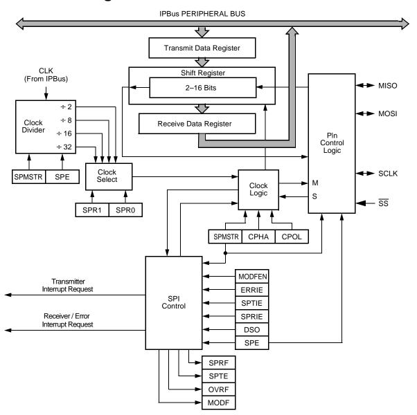
Figure 10-1. SPI Block Diagram
