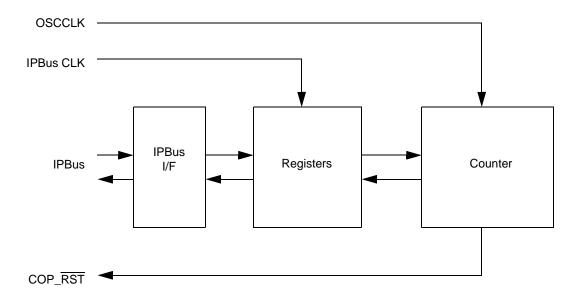
Figure 7-2. COP Module Block Diagram and Interface Signals
