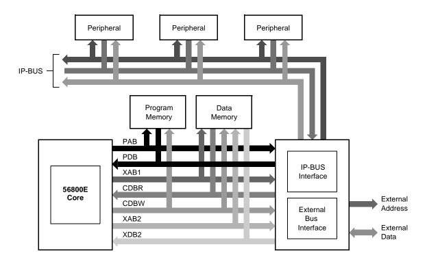
Figure 1-1. 56800E Chip Architecture with External Bus
