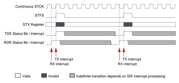
Figure 11-24. Synchronous Mode Interrupt Timing
