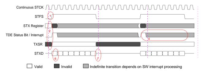
Figure 11-19. Normal Mode Transmit Timing—Continuous Clock (WL=8 bit words, DC=1)
