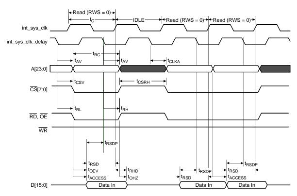
Figure 5-8. External Read Cycle with Clock and RWS = 0
