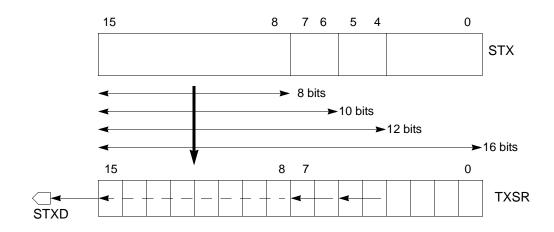
Figure 11-6. Transmit Data Path (TSHFD = 0)
