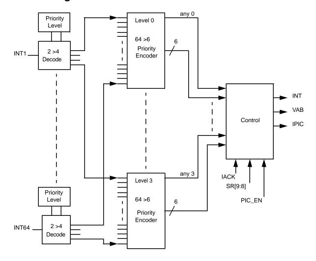
Figure 8-1. Interrupt Controller Block Diagram
