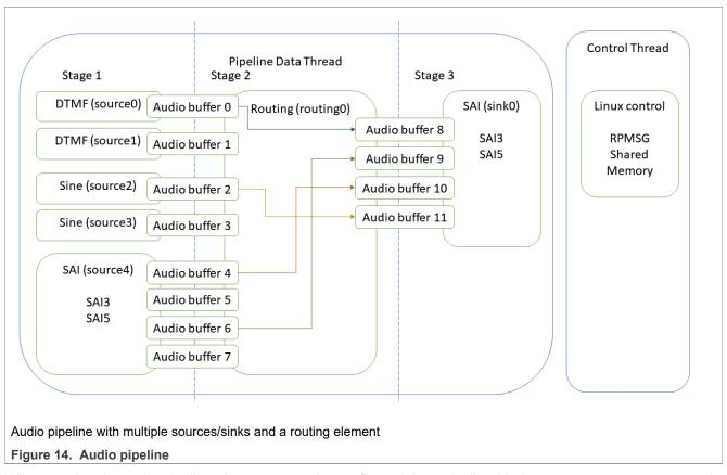
When running the audio pipeline, the routes can be configured dynamically with the <code>harpoon\_ctrl</code> command. This command uses source and sink indexes to connect elements.
