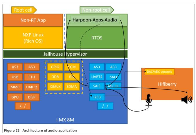
The DAC and ADC on the HiFiBerry card are controlled by the audio application. Control is done through I2C3 and data throughput through SAI5.
