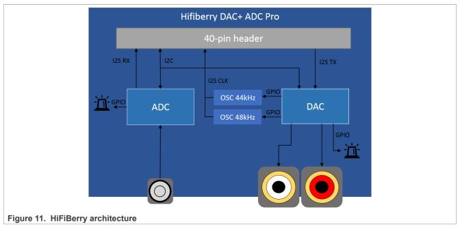
The PCM1863 and the PCM5122 use the same signal for I2S word select by using SAI synchronous mode.
