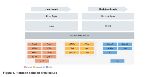
The bottom box shows the hardware partitioning between Jailhouse cells.
