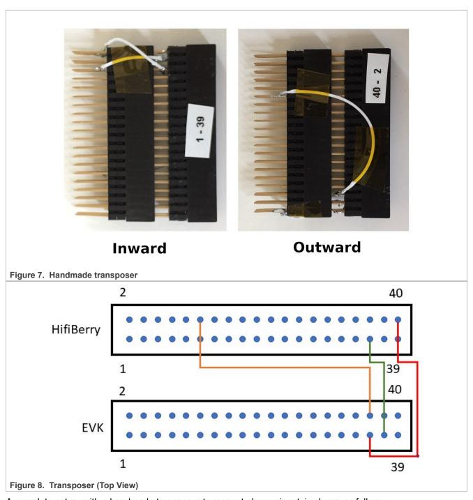
A complete setup, with a handmade transposer to respect above pinout, is shown as follows.
