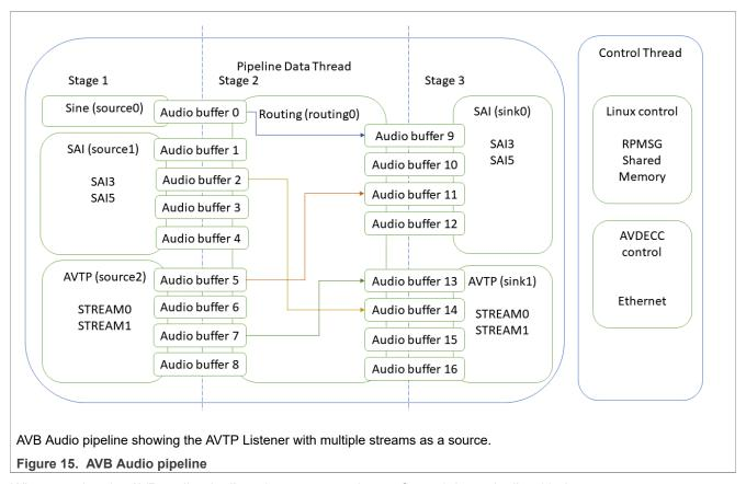
When running the AVB audio pipeline, the routes can be configured dynamically with the harpoon\_ctrl command. This command uses source and sink indexes to connect elements.
