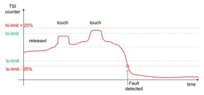
Figure 34. TSI input test fault detection
