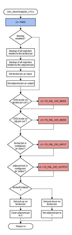
Figure 12. Block diagram of FS\_DIO\_ShortToAdiSet\_LPC() function IEC60730\_B\_CM0\_Library\_UG\_v4\_3, Rev. 0, 30. September 2022
