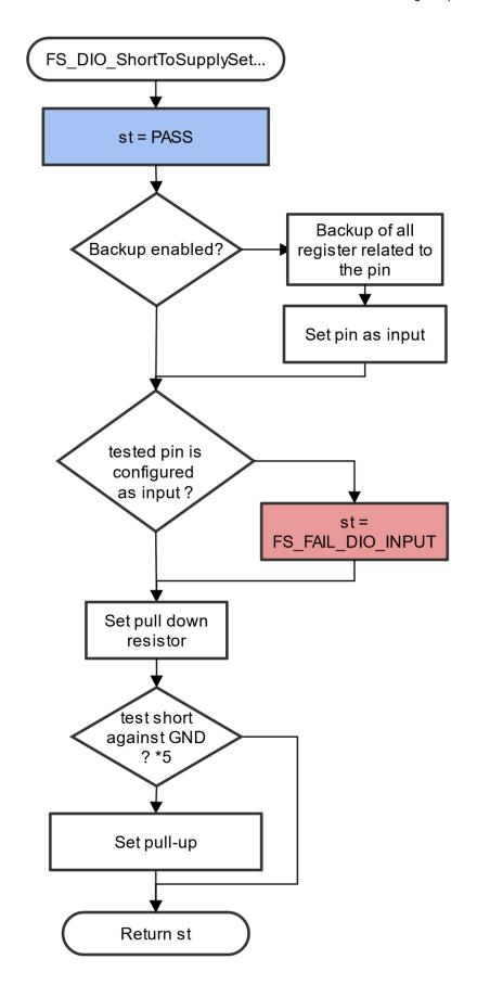
Figure 8. Block diagram of FS\_DIO\_ShortToSupplySet function IEC60730\_B\_CM0\_Library\_UG\_v4\_3, Rev. 0, 30. September 2022
