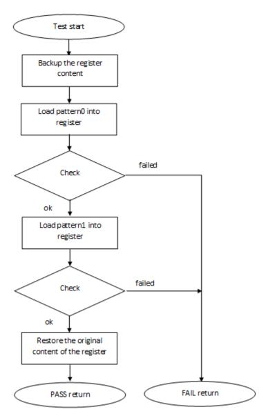
Figure 31. Block diagram for PRIMASK and CONTROL registers test
