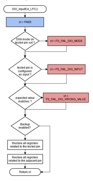
Figure 18. Extended digital input test for LPC devices
