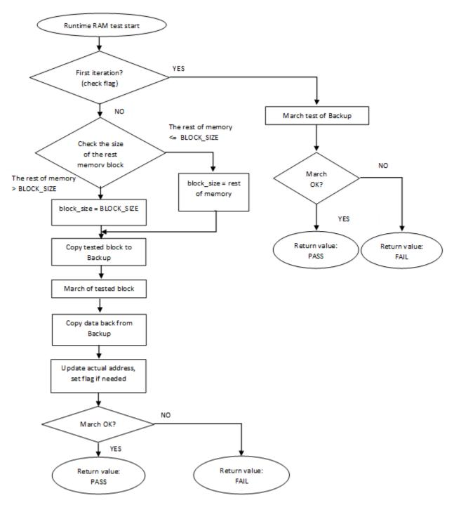
Figure 28. Block diagram for runtime test of RAM
