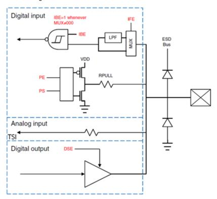
Figure 33. I/O simplified block diagram
