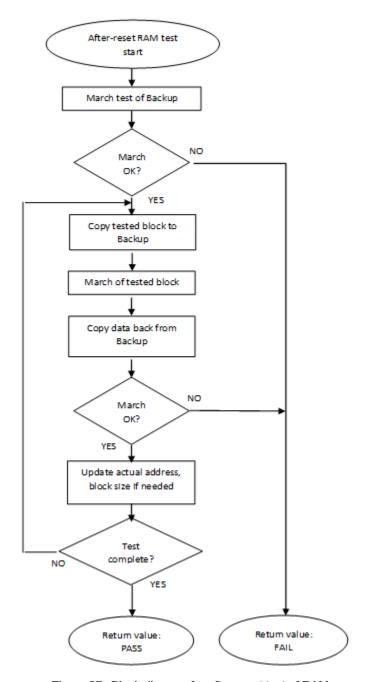
Figure 27. Block diagram for after-reset test of RAM
