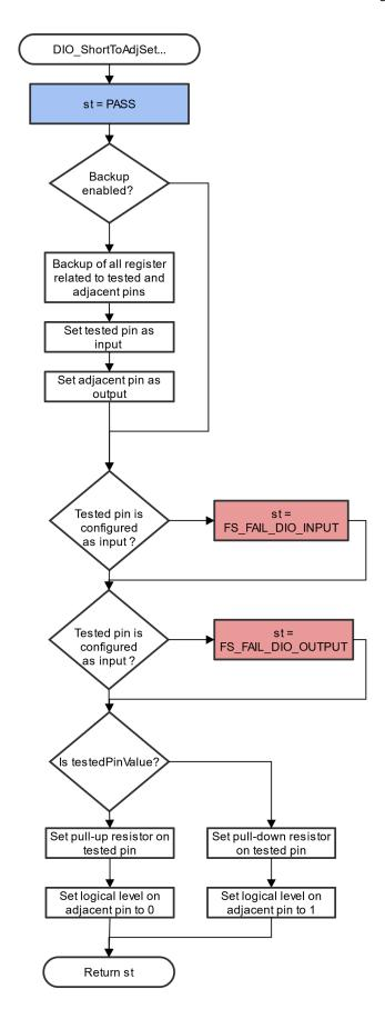
Figure 23. Block diagram of FS. DIO\_ShortToAdjSet\_RGPIO() function IEC60730\_B\_CM0\_Library\_UG\_v4\_3, Rev. 0, 30. September 2022
