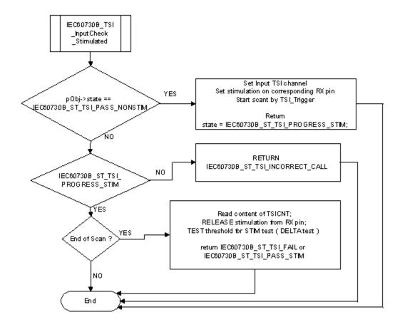
Figure 38. Software program flow for TSI input test with stimulated inputs
