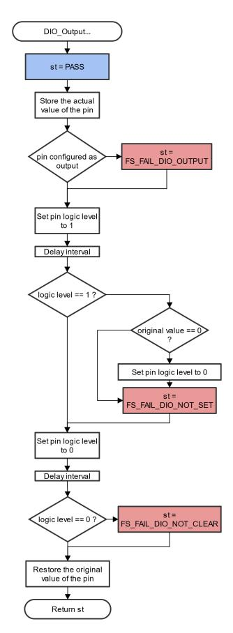
Figure 15 Block diagram for digital output test IEC60730\_B\_CM0\_Library\_UG\_v4\_3, Rev. 0, 30. September 2022
