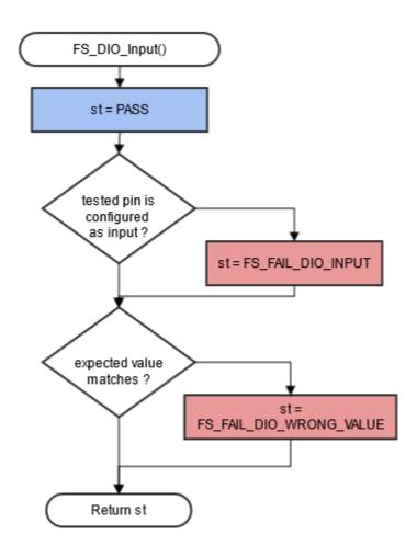
Figure 4. Block diagram for digital input test
