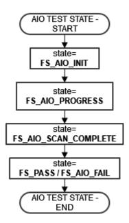
Figure 2. ADC Test Code flow
