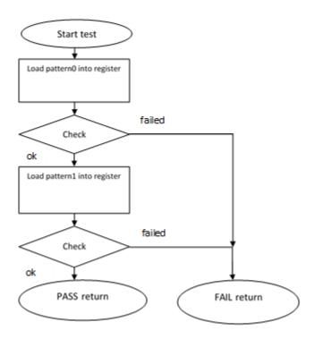
Figure 29. Block diagram for R2 – R12 registers test
