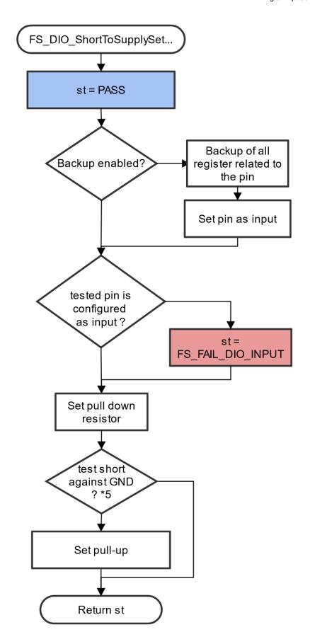
Figure 17 Block diagram of FS\_DIO\_ShortToSupplySet\_IMXRT() function IEC60730\_B\_CM0\_Library\_UG\_v4\_3, Rev. 0, 30. September 2022
