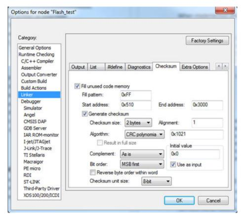
Figure 25. Checksum settings for linker
