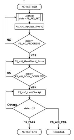
Figure 1. Block diagram for analog input test
