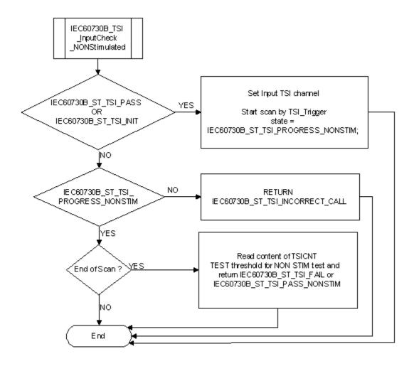
Figure 35. Software program flow for TSI input test with non-stimulated inputs
