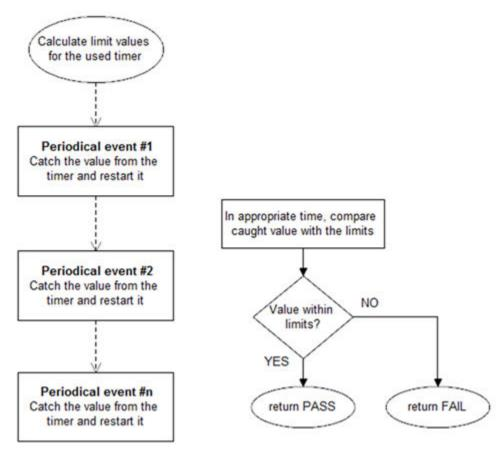
Figure 3. Block diagram for clock test
