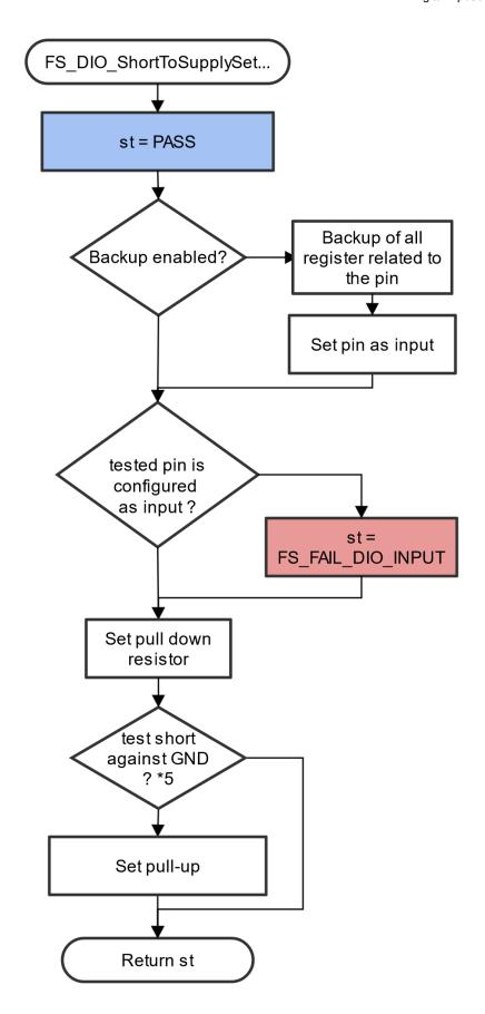
Figure 13. Block diagram of FS\_DIO\_ShortToSupplySet\_IMX8M() function IEC60730\_B\_CM0\_Library\_UG\_v4\_3, Rev. 0, 30. September 2022
