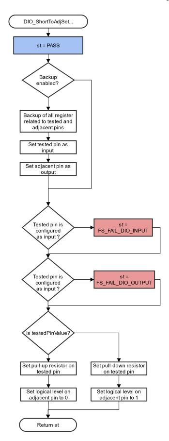
Figure 11 Block diagram of FS\_DIO\_ShortToAdjSet\_IMX8M() function IEC60730\_B\_CM0\_Library\_UG\_v4\_3, Rev. 0, 30. September 2022
