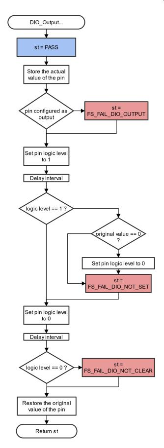
Figure 10. Block diagram for digital output test IEC60730\_B\_CM0\_Library\_UG\_v4\_3, Rev. 0, 30. September 2022
