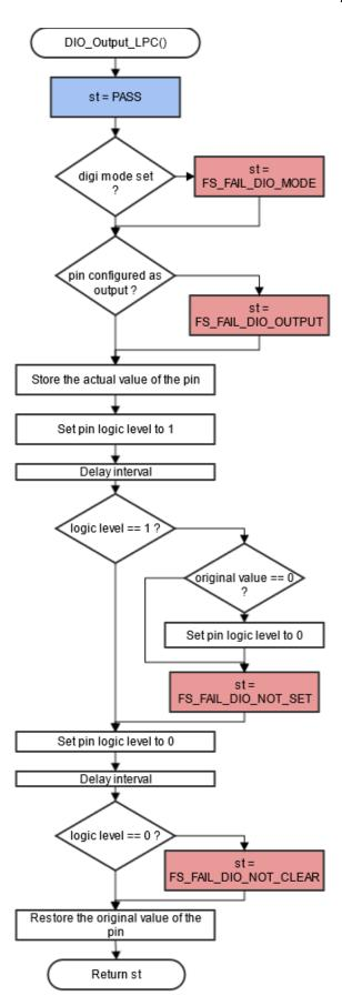
Figure 19 Block diagram for digital output test IEC60730\_B\_CM0\_Library\_UG\_v4\_3, Rev. 0, 30. September 2022
