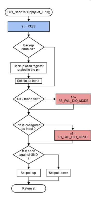
Figure 21. Block diagram of FS\_DIO\_ShortToSupplySet\_LPC function
