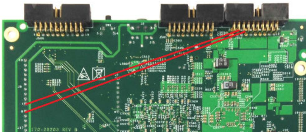
Figure 10. NFC hardware connection on LS1021A-IoT
