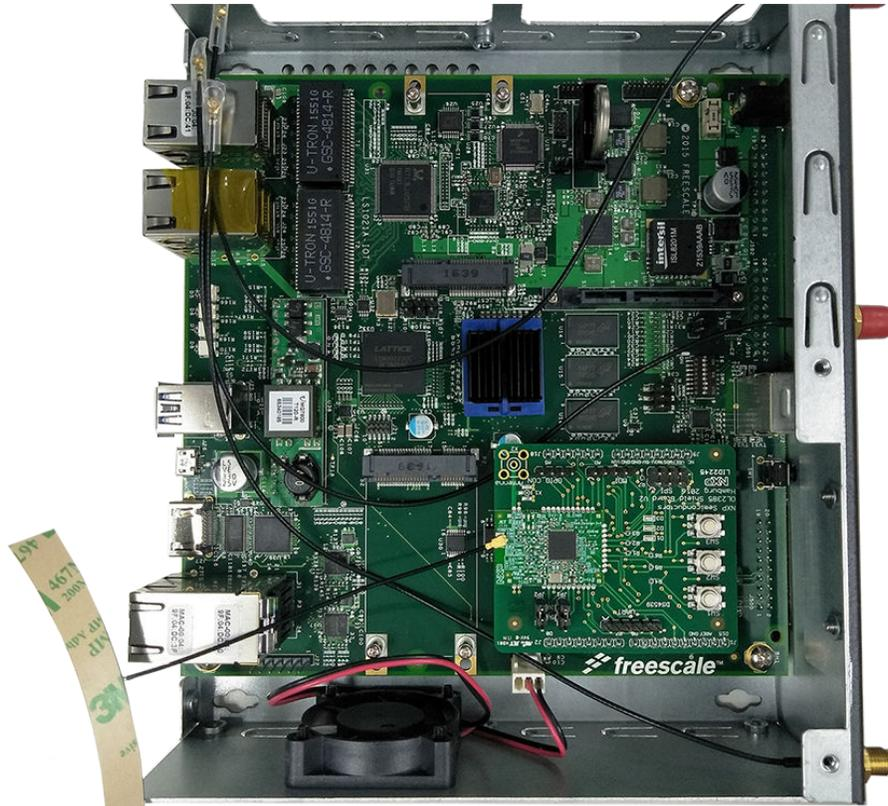
Figure 17. Using the  $\mu$ FL connector for Sigfox demo
