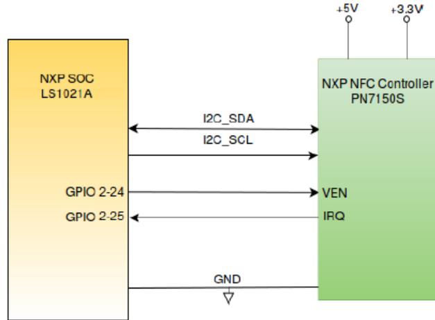
Figure 8. NFC connections to the LS1021A-IoT board
