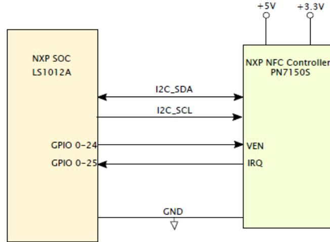
Figure 9. NFC connections to the LS1021A-IO board
