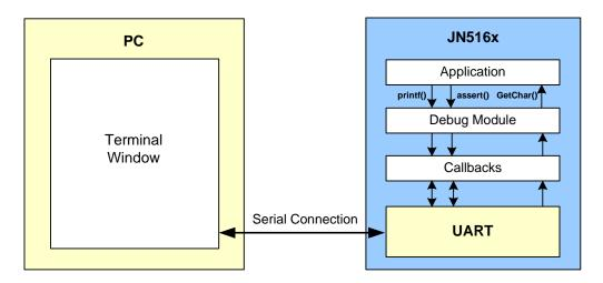
Figure 9: Typical Hardware Set-Up for Debugging
