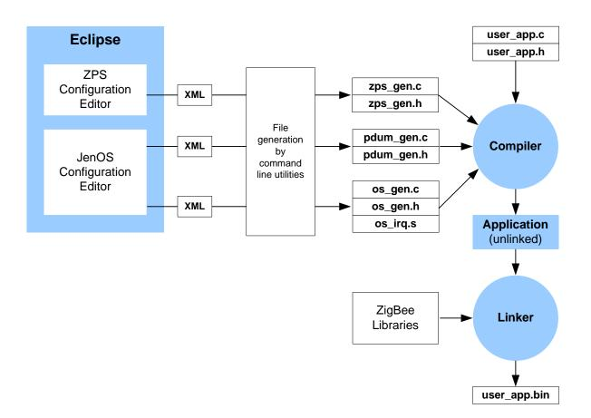
Figure 1: Application Build Process
