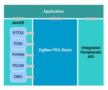
Figure 1: Basic Software Architecture
