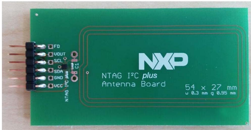
**Figure 31: NTAG I<sup>2</sup>C plus Antenna Board**
