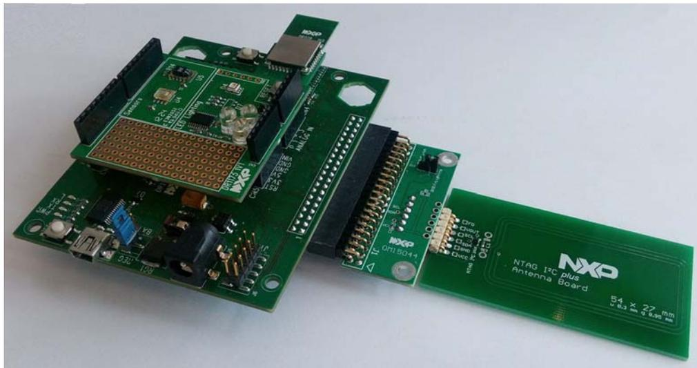
**Figure 32: Fully Assembled Board with NFC Tag**
