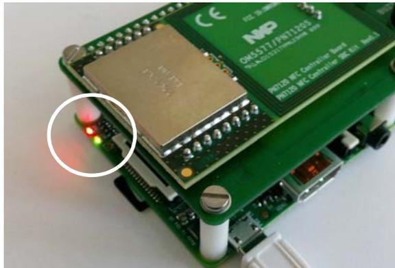
The IoT Gateway is then ready. When in this state, the green LED on the NFC Controller board flashes.
