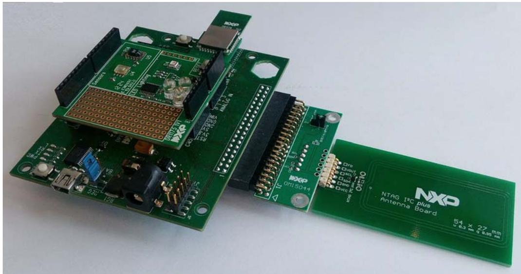
**Figure 12: Assembled Node**
