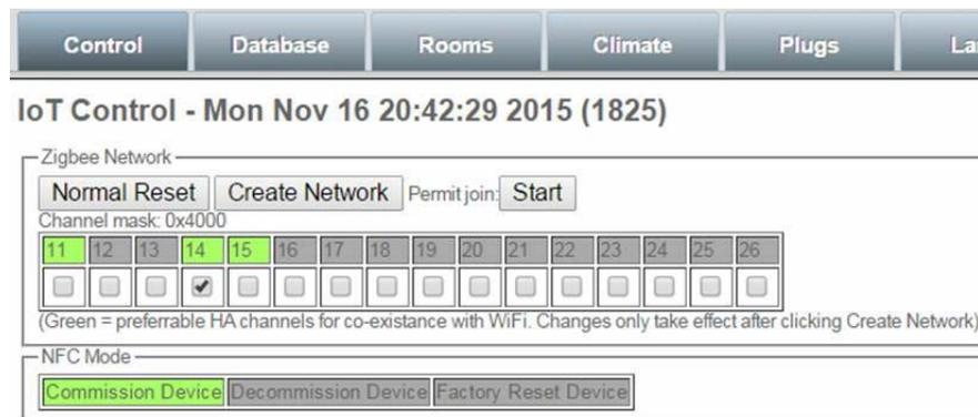
The ZigBee network will be created on channel 14. A successful network start will be indicated by the illumination of the green and orange LEDs on the JN5169 USB Dongle.
