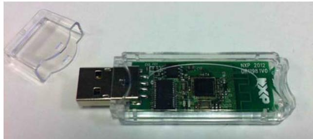
**Figure 28: JN5169 USB Dongle**
