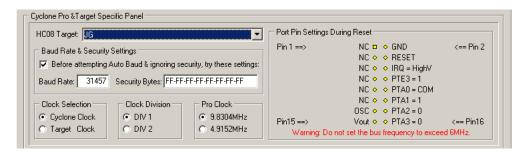
Figure 13-16: 68HC908JG Family MON08 Pinout
