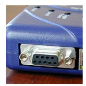
Figure 3-3: Cyclone PRO RS232 Connector
