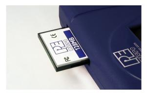
Figure 3-22: CompactFlash Port
