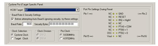
Figure 13-35: 68HC908RF Family MON08 Pinout
