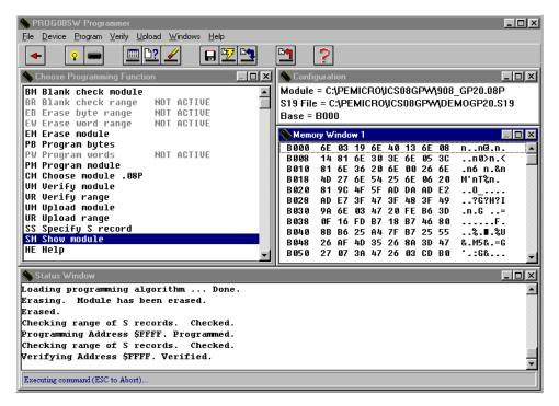
Figure 8-3: PROG08SZ Programmer Screen Snapshot
