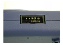
Figure 3-17: Jumper Settings for Target Power Connection via Cyclone PRO Board Power and Pin 15 of Cyclone PRO MON08 Connector
