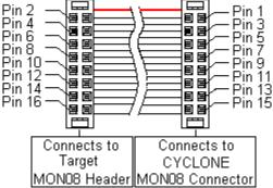
Figure 3-10: Ribbon Cable Diagram When Looking Into IDC Socket
