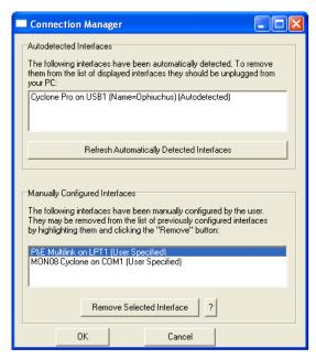
Figure 8-13: Remove A Manually Configured Multilink/Cyclone Pro Interface
