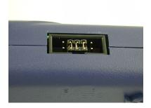
Figure 3-19: Jumper Settings for Target Power Connection via Cyclone PRO Board Power and Pin 6 of Cyclone PRO BDM Connector
