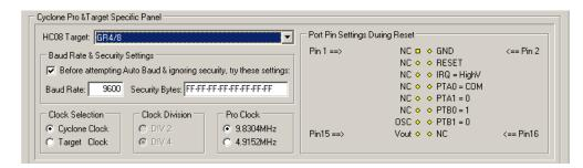
Figure 13-10: 68HC908GR4/8 MON08 Pinout
