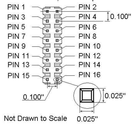
Figure 3-8: 16-Pin Header Mechanical Drawing
