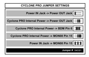
Figure 3-11: Jumper Settings (Rev. C)
