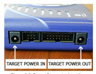
Figure 3-6: Power Connector Locations
