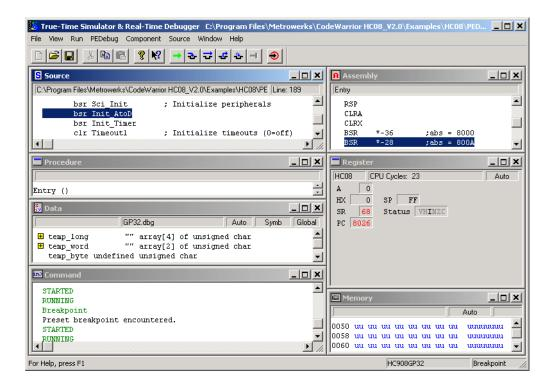
Figure 8-5: True-Time Simulator & Real-Time Debugger Window
