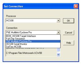
Figure 8-27: HCS08 P&E Multilink/Cyclone Pro Connection Setting
