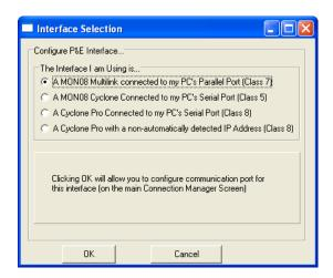
Figure 8-12: P&E Multilink/Cyclone Pro Manual Interface Selection
