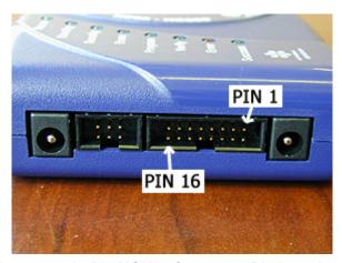
Figure 3-9: 16-Pin MON08 Connector Pin Locations
