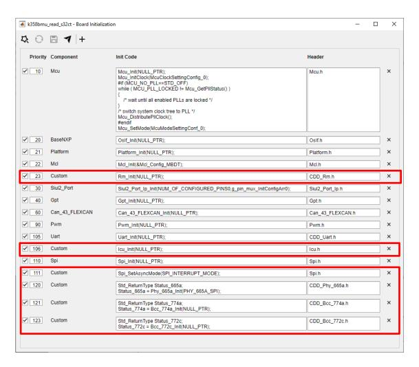
For this example, all the Components marked as **Custom** were added. Note that the Priority column specifies the order in which the code will be generated. An External Board Initialization Template can also be provided. For more details on how to provide an initialization template, please check the MBDT for S32K3xx Release Notes and Quick Start Guides.
