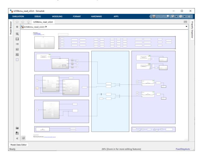
Open the FreeMASTER project associated with the model, and connect to the BMU. If successful, the BMU.General tab shows the pack voltage and the pack current measured by the battery management system.
