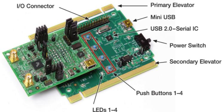
Connect the TWR-RF-MRB USB connector (J2) to the USB of the PC.
