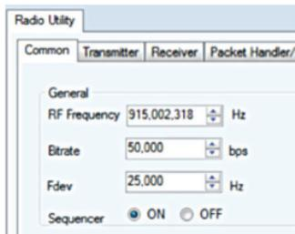
Do this separately to both boards and they will both be on the same correct frequency. (The above image is targeting 915 MHz.)
