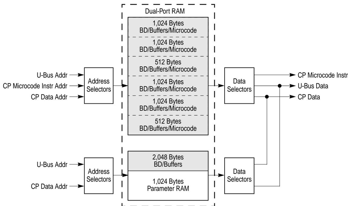
Shaded area is system RAM. Note that in this figure, the area is not contiguous memory. For an accurate representation of the physical implementation, see Figure 1-4.
