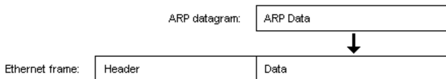
Figure A-3. ARP Datagram in an Ethernet frame
