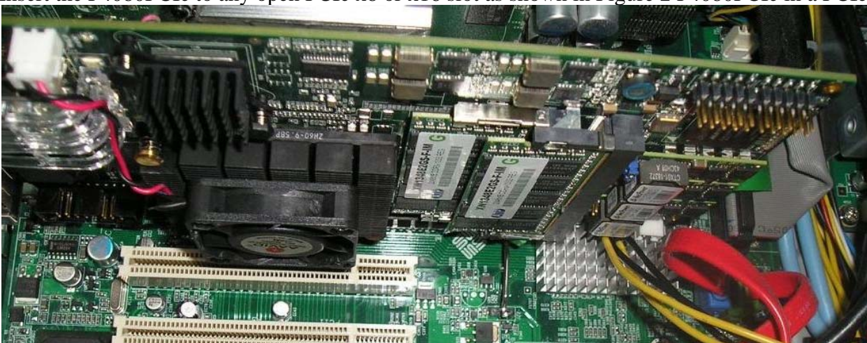
Figure 2 P4080PCIe in a PCIe x8 slot.
