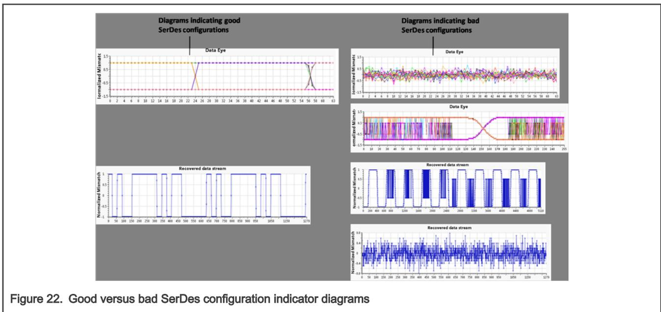
Figure 22. Good versus bad SerDes configuration indicator diagrams
