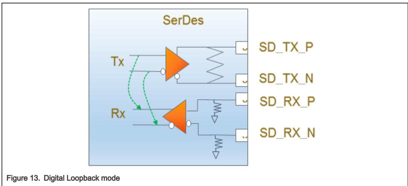
Figure 13. Digital Loopback mode
