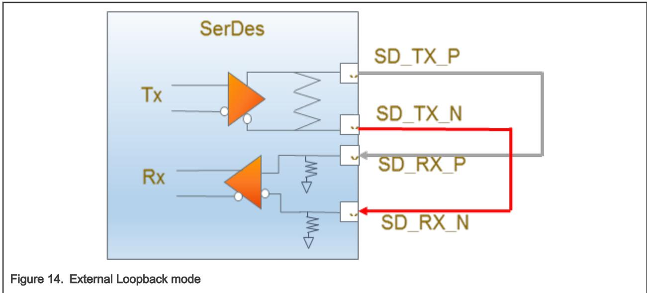
Figure 14. External Loopback mode
