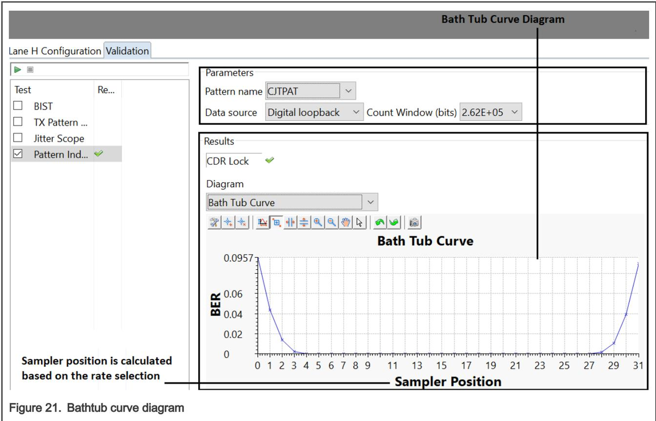
Figure 21. Bathtub curve diagram
