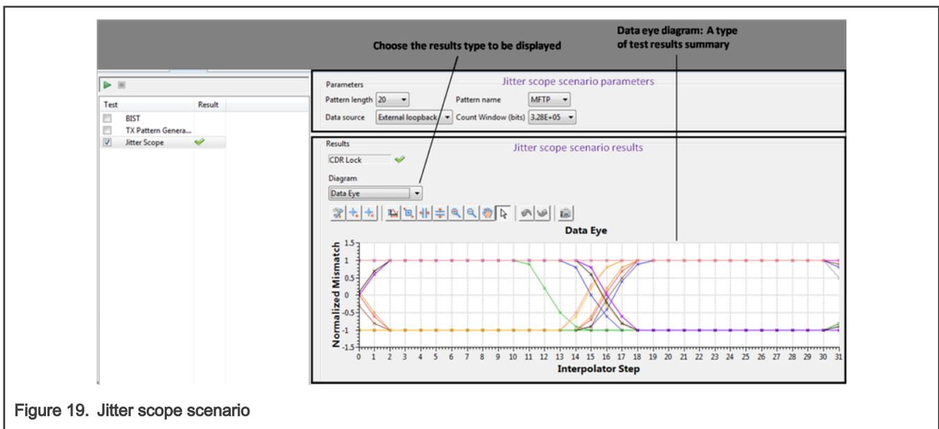
The figure below describes the data eye and recovered data stream diagrams.
