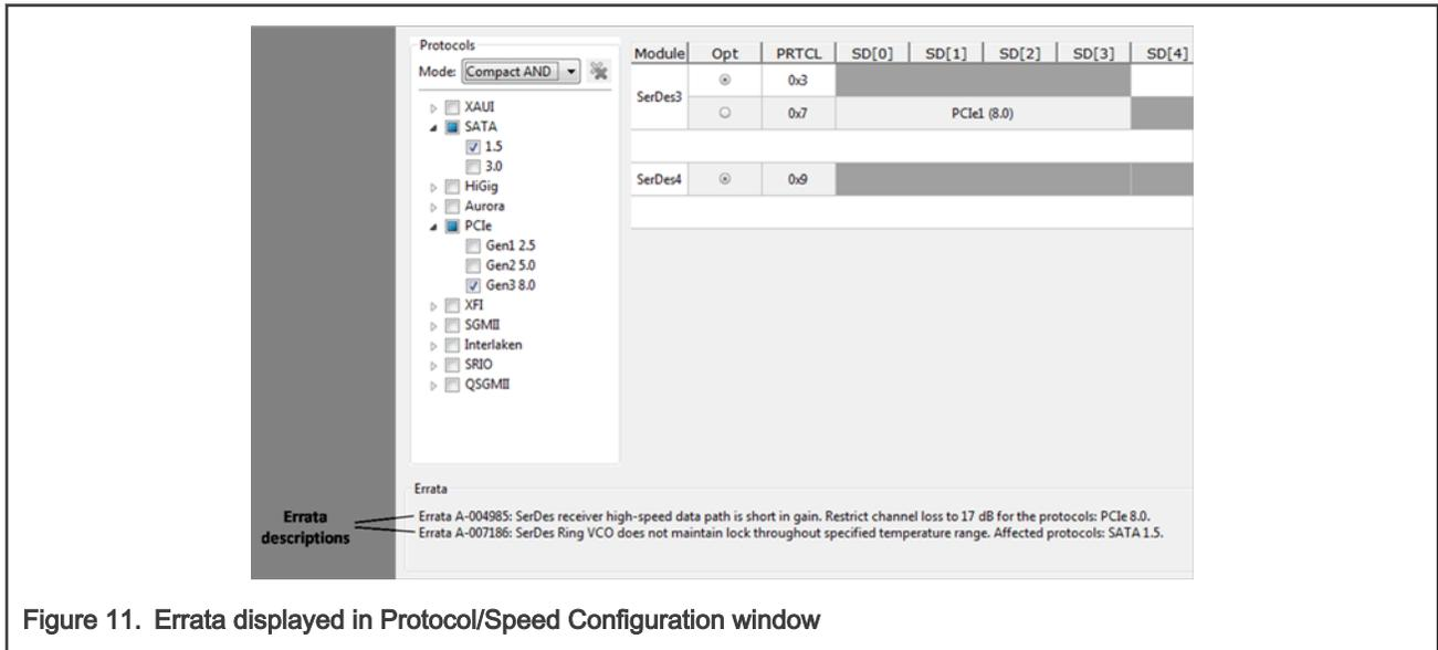
Figure 11. Errata displayed in Protocol/Speed Configuration window
