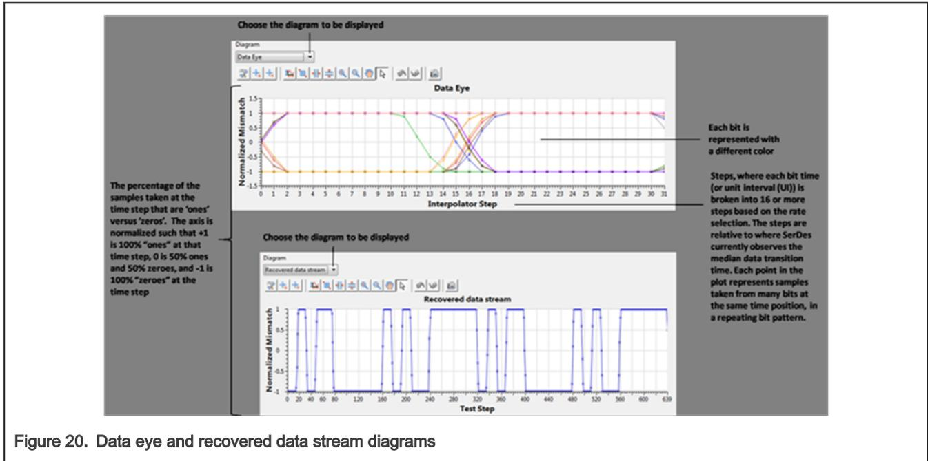
Figure 20. Data eye and recovered data stream diagrams
