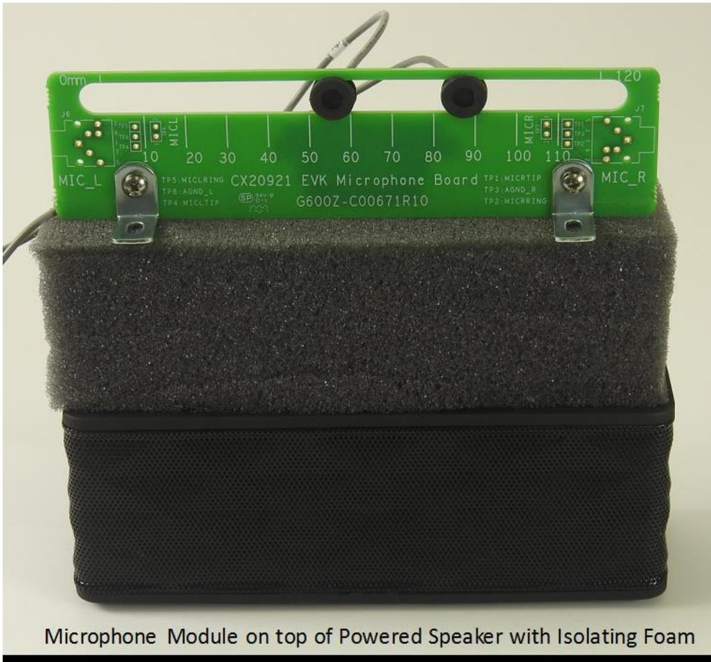
Microphone Module on top of Powered Speaker with Isolating Foam
