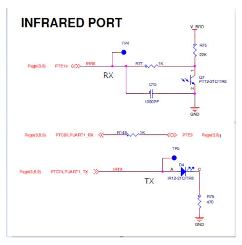
Figure 9. Infrared port
