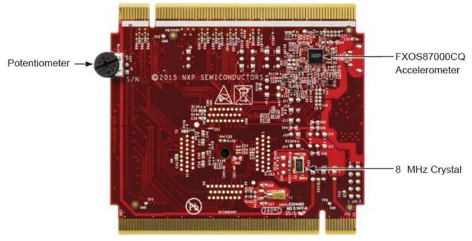
Figure 3. Back Side of TWR-KE18F
