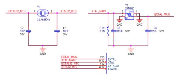
Figure 5. TWR-VF65GS10 external clock options
