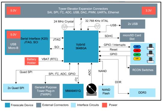
Figure 4. TWR-VF65GS10 block diagram
