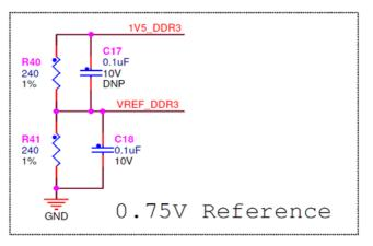
Figure 11. DDR3 0.75V reference supply
