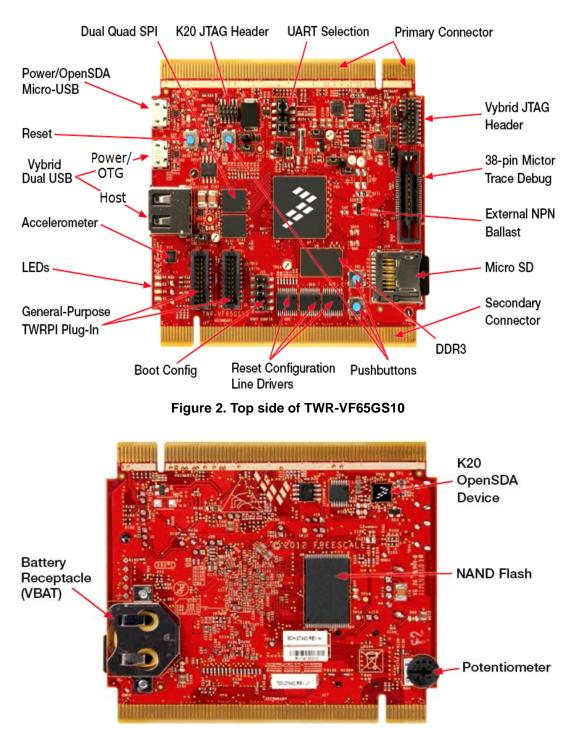
Figure 3. Bottom side of TWR-VF65GS10
