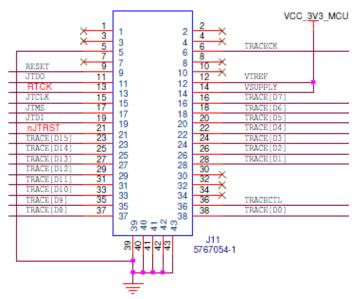
Figure 10. 38-pin Mictor connector
