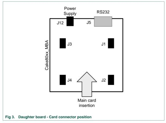
With respect to this card connector position, the following figures give the position of the different daughter boards.
