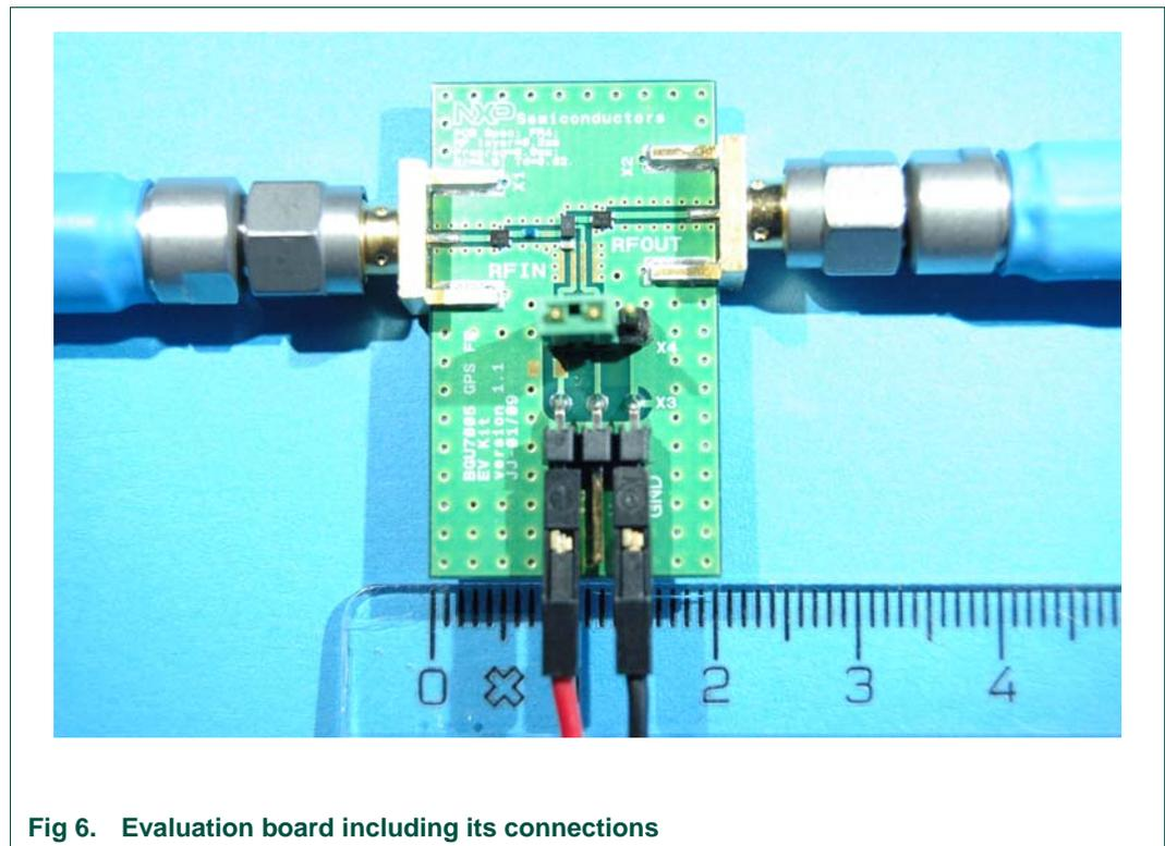
Fig 6. Evaluation board including its connections
