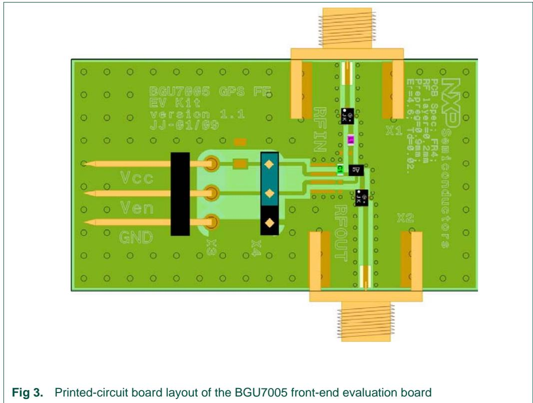
Fig 3. Printed-circuit board layout of the BGU7005 front-end evaluation board
