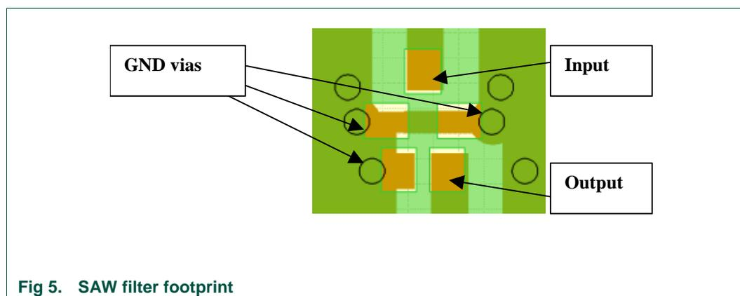
Fig 5. SAW filter footprint
