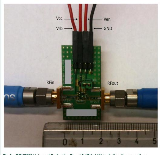
Fig 6. BGU7003 Universal Evaluation Board 2.4GHz LNA including its connections
