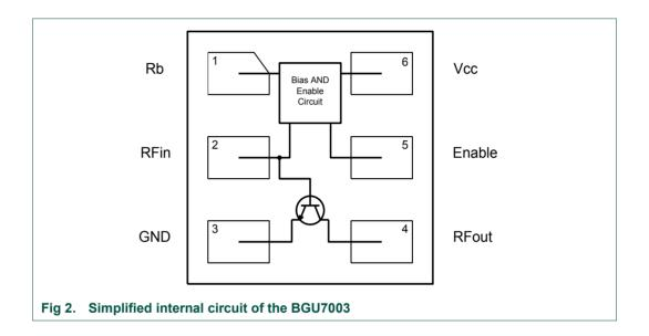
The BGU7003 is not internally matched so for both input and output a matching circuit needs to be designed. The fact that no internal matching is available makes the product suitable for different application/frequency areas.
