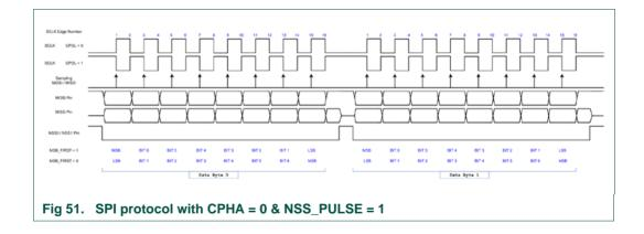
The SPI master automatically generates NSS signal. Its polarity can be configured, and it can be chosen to generate a pulse on NSS between each byte. If more flexibility is needed, then FW can program itself the value to output to NSS, using NSS\_CTRL=1 (override internal value), and choosing the value to output to NSS\_VAL.
