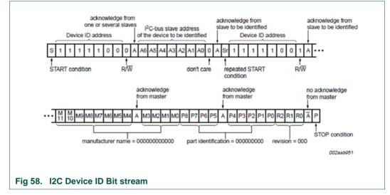
If HOSTIF\_I2C\_CONTROL\_REG.I2C\_DEVID\_ENABLE is logic low, the Host Interface will respond to the Device ID Address and the I2C Slave Address with NACK.
