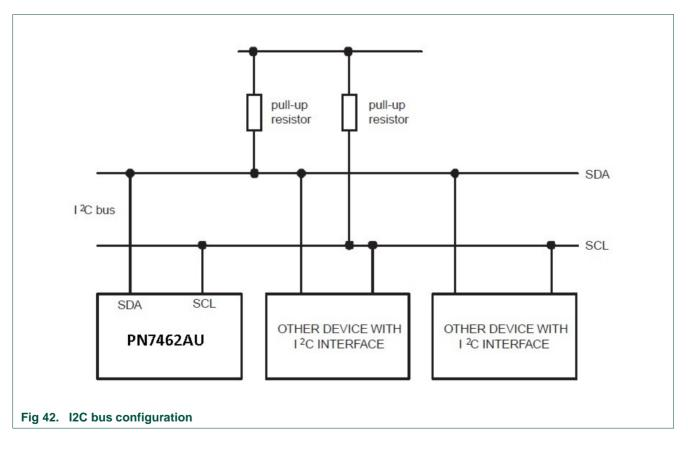
The I2C Master can operate in two modes: I2C Master Transmitter and I2C Master Receiver.
