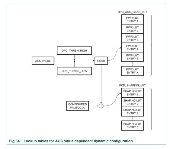
The AGC value is compared to a maximum and minimum threshold value which is stored in EEPROM.
