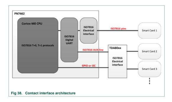
The external TDA is required to handle the smart card electrical interface. The connection between the PN7462 family and the TDA is composed of 2 parts:
