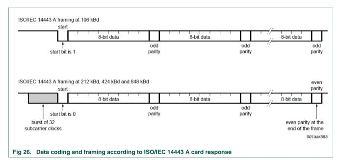
The internal CRC coprocessor calculates the CRC value based on the selected protocol. In card mode for higher baud rates, the parity is automatically inverted as end of communication indicator.
