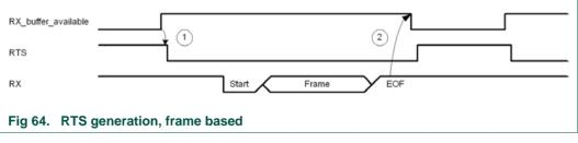
Note that in case the host sends a frame longer than buffer size, a buffer\_overflow interrupt will be sent to the firmware. The RTS will not toggle to high. Data received after the error are not stored into memory. The error is signaled to the firmware by an interrupt.
