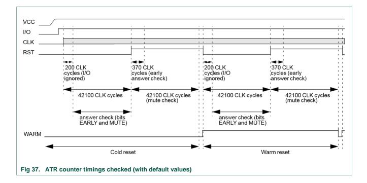
The bits EARLY and MUTE signal an interrupt when set to logic level one (see the registers description).
