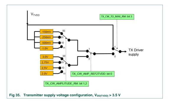
transmitter supply voltage configurations - can be defined by the application, up to 15 gears are available.
