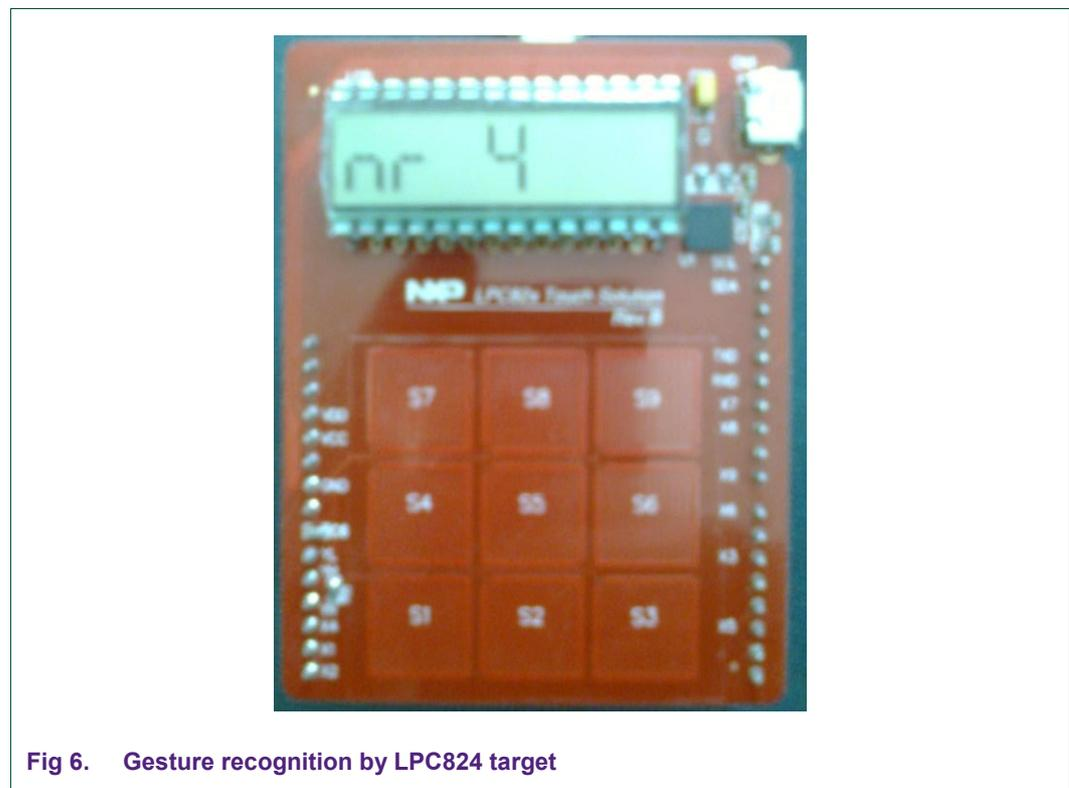
**Fig 6. Gesture recognition by LPC824 target**
