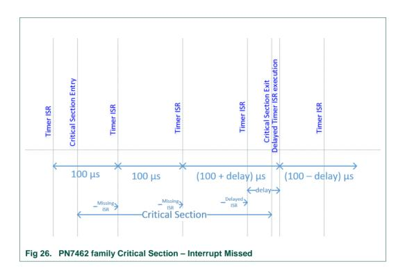
As presented in the Fig 26 there is a possibility of missing interrupts when the interrupt is configured to occur every 100  $\mu$ s and if the interrupt arrives when the "phhalRf\_Receive()" API is executing the critical section in passive target mode, the interrupt gets missed couple of times.
