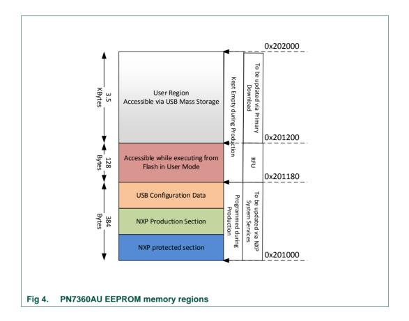
Note: The RFU section of 128 bytes is kept hidden from the aperture of USB mass storage. But this area is used by the HAL executing from the user flash for internal purposes. As of now, there is no special use case for this region and hence in the default examples of PN7462 family, this region remains unused.
