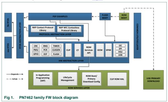
The FW can be divided into NXP FW and user FW. The NXP FW is placed in ROM memory region and protected flash memory region. The user FW is placed in the user flash memory region. The protected flash memory region is primarily used to place ROM patches.
