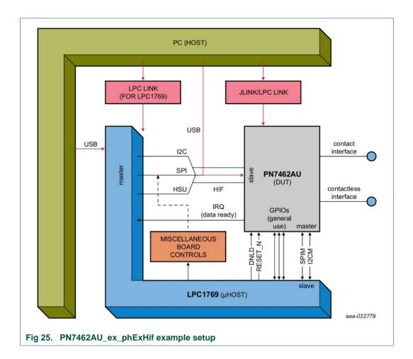
The GPIOs of LPC and PN7462AU are used to determine which functionality of this example has to be executed. It is also used to select the host interface or master interface to be used. For each different functionality, a different LPCXpresso project is required for LPC1769 side while PN7462AU side has only the PN7462AU\_ex\_phExHif LPCXpresso project.
