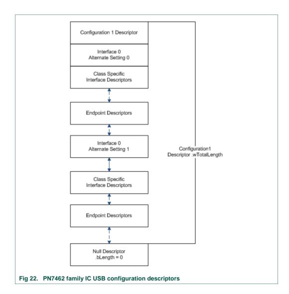
The following example shows the configuration descriptor for the USB CCID class device:
