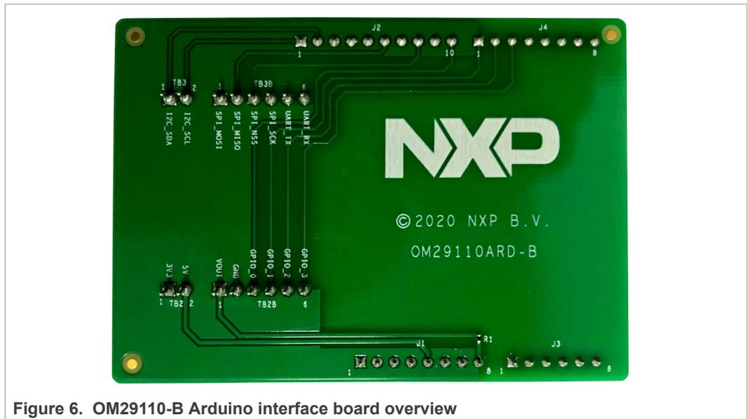
Figure 6. OM29110-B Arduino interface board overview
