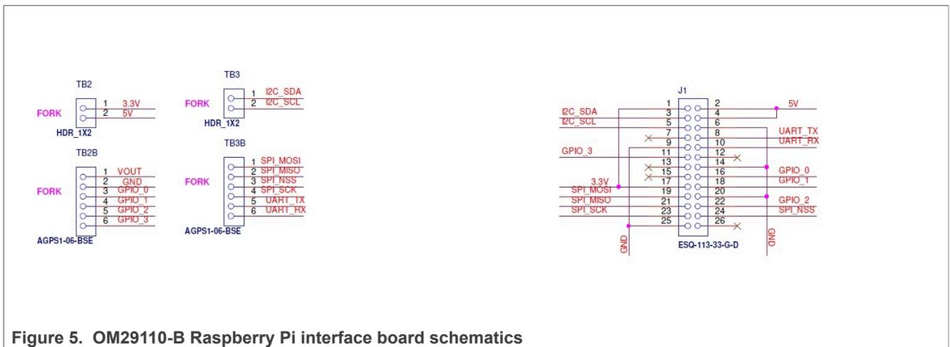
Figure 5. OM29110-B Raspberry Pi interface board schematics
