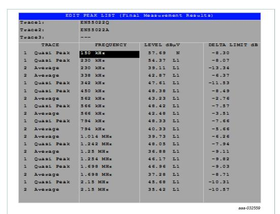
Figure 8. Conducted EMI peak list at full load 230 V (AC)/50 Hz and 20 V (DC)/3 A
