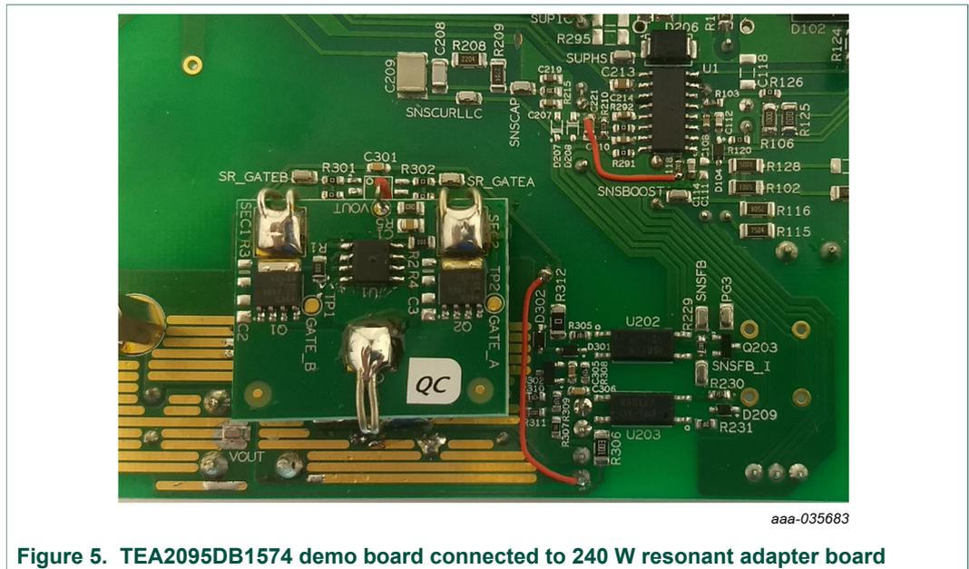
Figure 5. TEA2095DB1574 demo board connected to 240 W resonant adapter board
