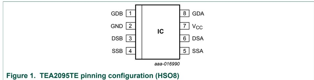
Figure 1. TEA2095TE pinning configuration (HSO8)
