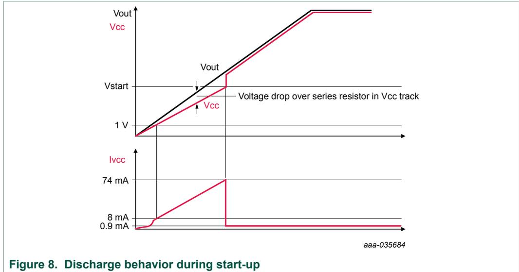
Figure 8. Discharge behavior during start-up
