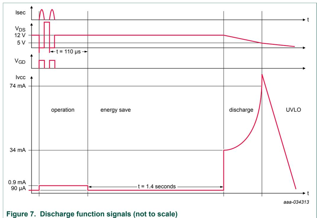
Figure 7. Discharge function signals (not to scale)
