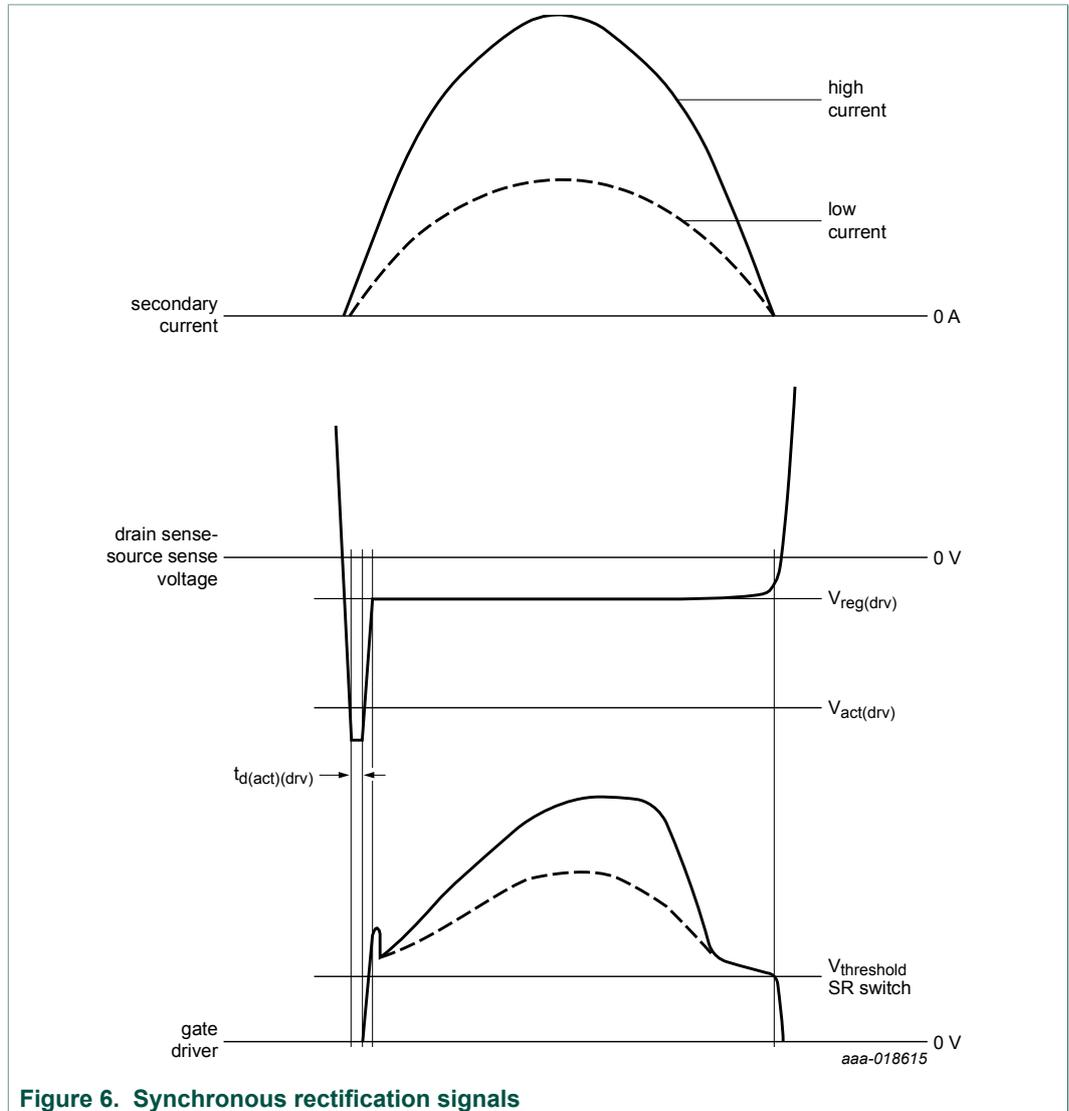
Figure 6. Synchronous rectification signals
