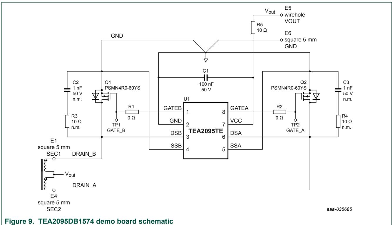
Figure 9. TEA2095DB1574 demo board schematic
