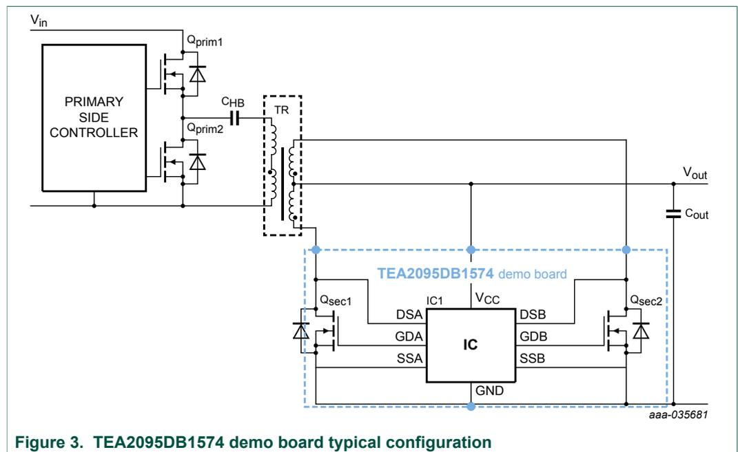
Figure 3. TEA2095DB1574 demo board typical configuration
