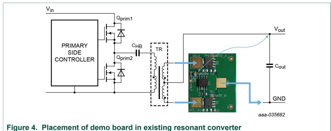
Figure 4. Placement of demo board in existing resonant converter
