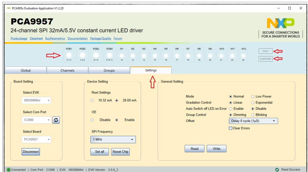
Figure 10. Graphical user interface — Settings tab activated
