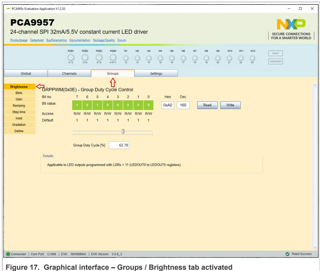
Figure 17. Graphical interface – Groups / Brightness tab activated
