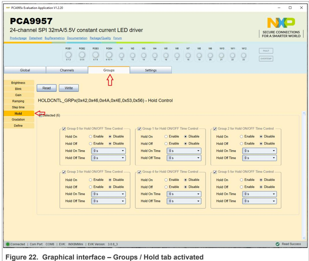
Figure 22. Graphical interface – Groups / Hold tab activated
