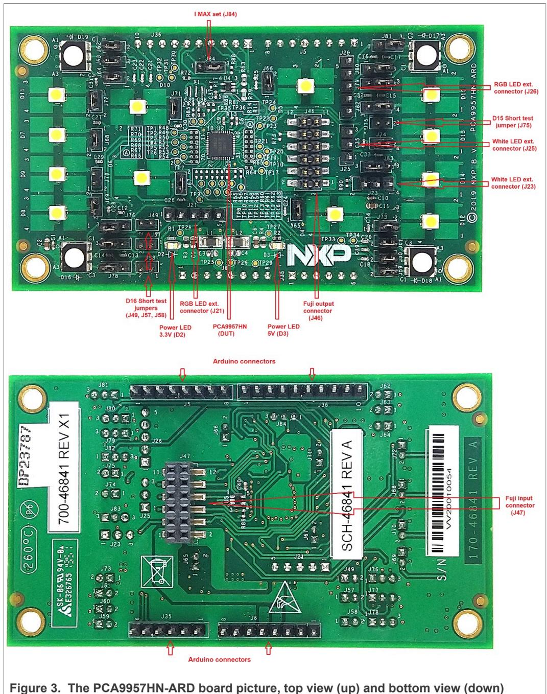
Figure 3. The PCA9957HN-ARD board picture, top view (up) and bottom view (down)
