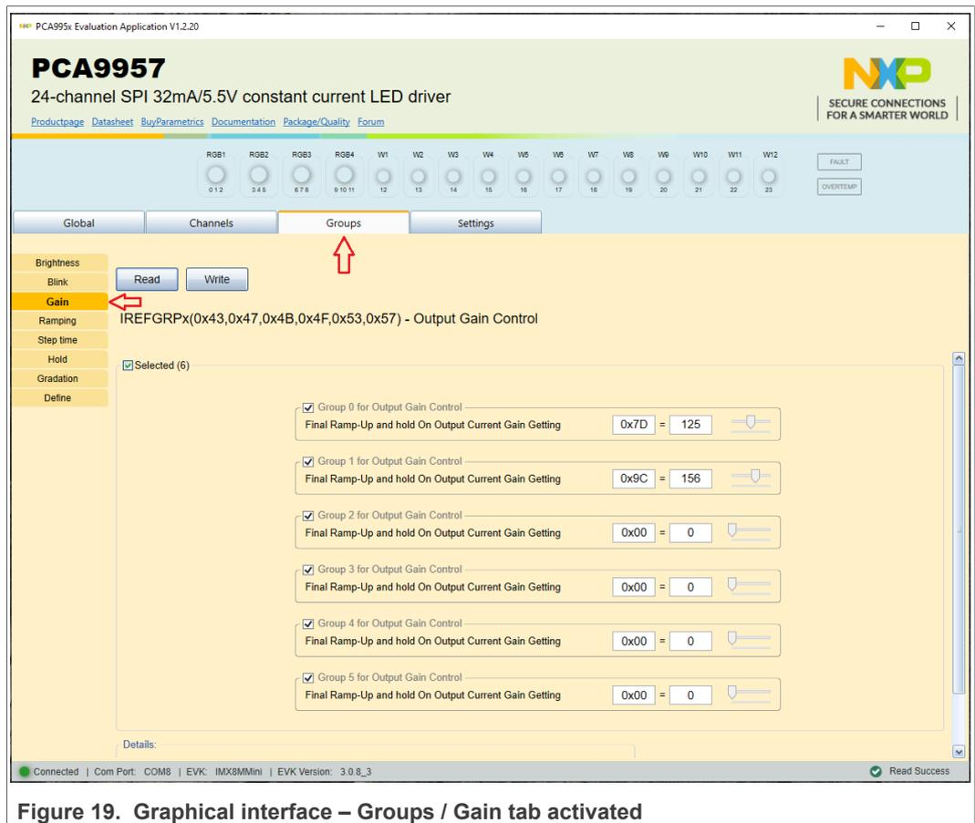
Figure 19. Graphical interface – Groups / Gain tab activated
