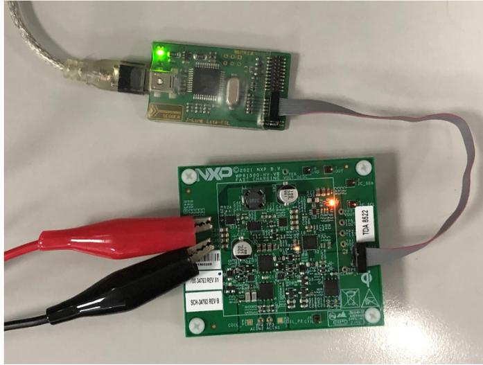
Figure 5. Downloading and debugging connections
