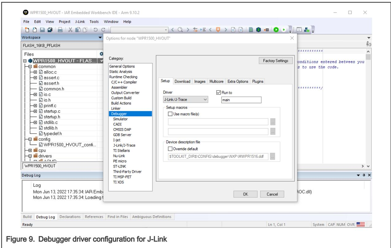
Figure 9. Debugger driver configuration for J-Link
