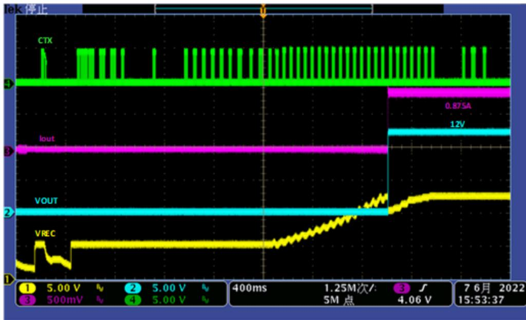
Figure 19. WPR1500-HV board system start wave
