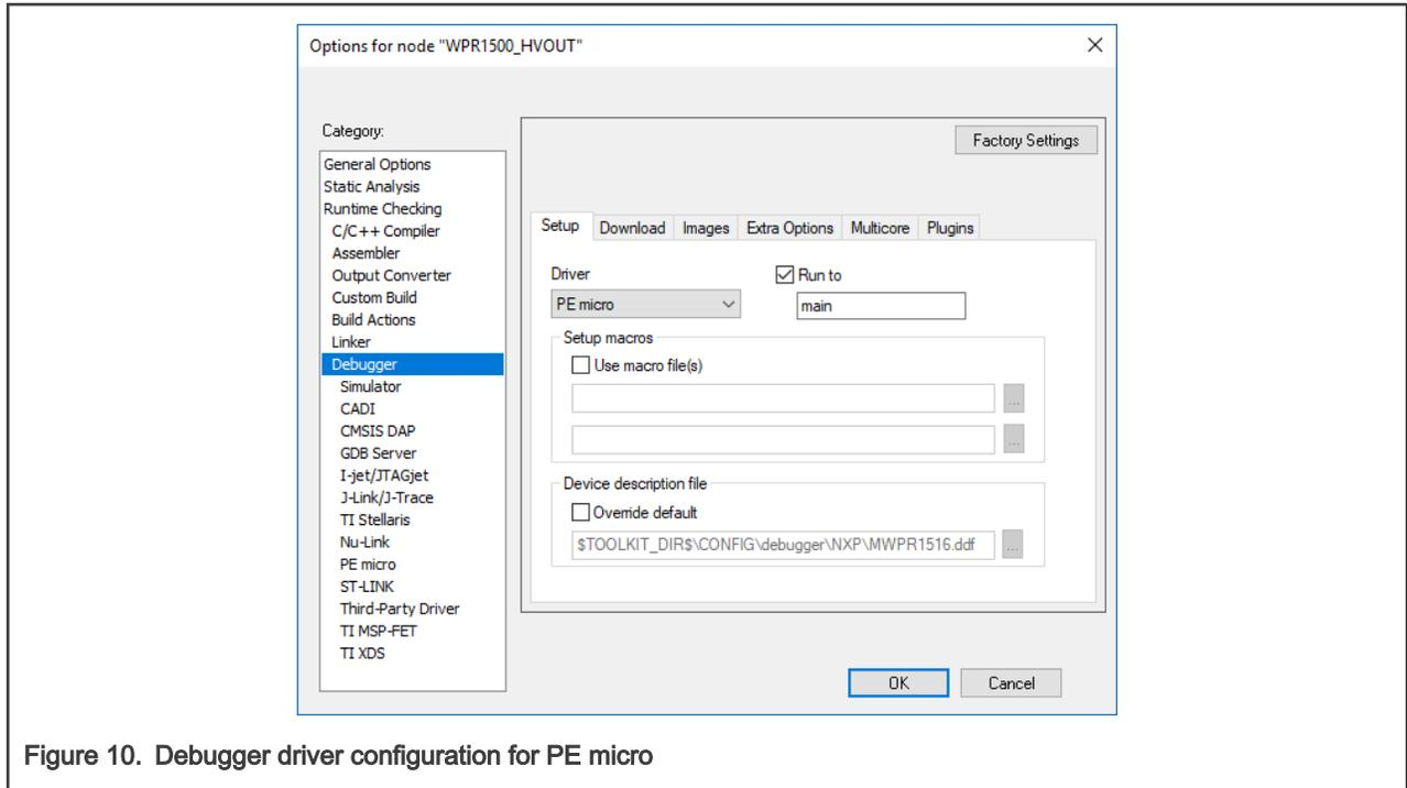
Figure 10. Debugger driver configuration for PE micro
