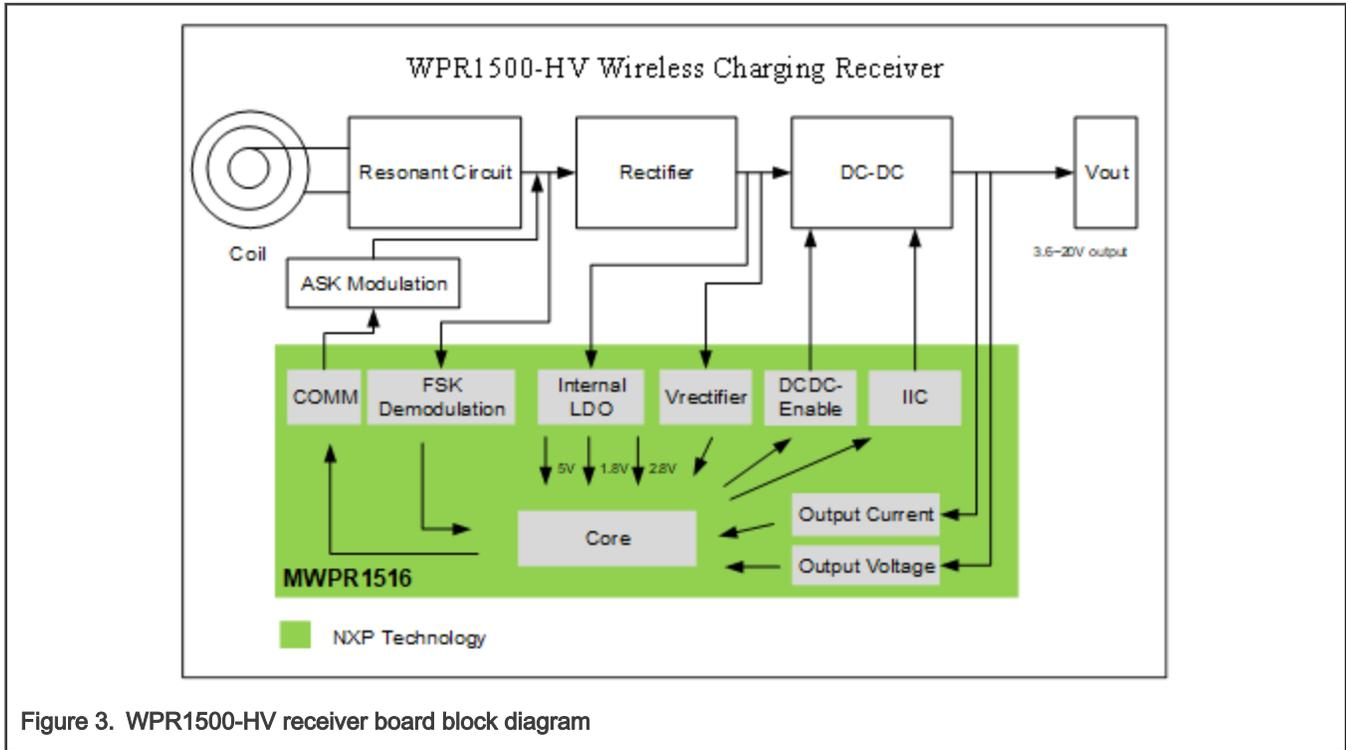
Figure 3. WPR1500-HV receiver board block diagram
