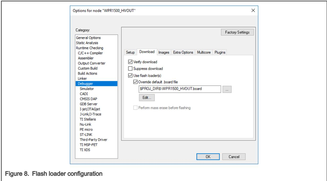
Figure 8. Flash loader configuration
