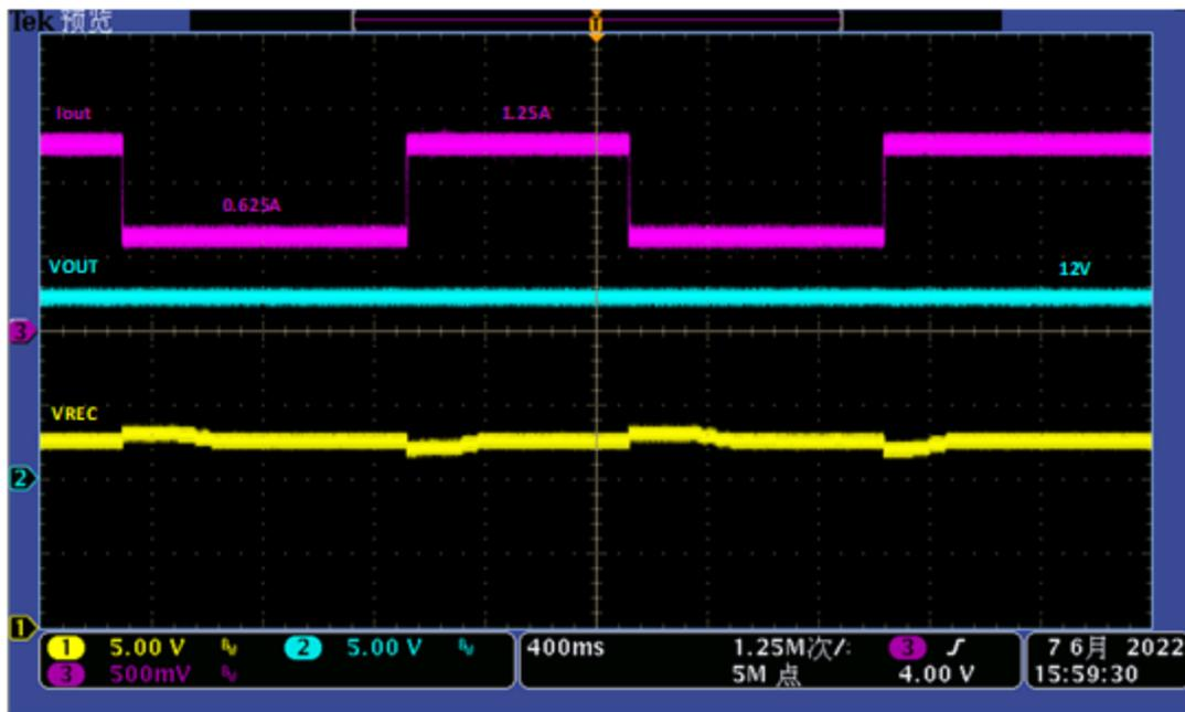
Figure 20. WPR1500-HV board load Step/Dump wave
