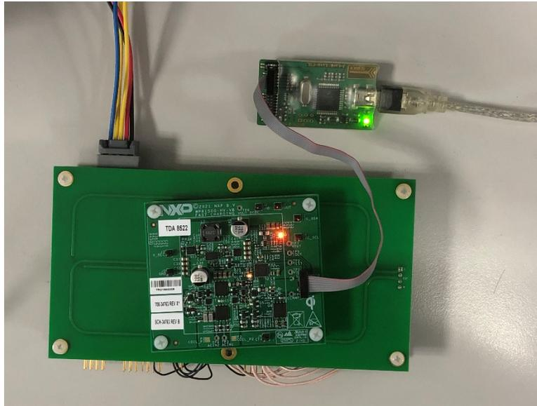
Figure 14. FreeMASTER debugging connection
