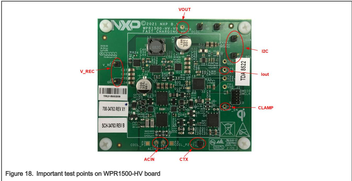
Figure 18. Important test points on WPR1500-HV board
